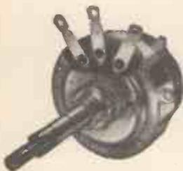
Thorough screening between switch and potentiometer. Concentric operating spindles give independent operation of switch or potentiometer with 'one-control' simplicity. Quick make-and-break action mains switch. Knob location to suit specified requirements. Type 154 with SPST switch, Type 155 with DPST switch.
