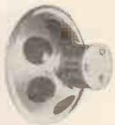
The small cone acts as a high note radiator for frequencies above 10,000 cycles and also as a diffuser for frequencies below 10,000 cycles from the large cone. The large cone itself acts as a low note radiator below 10,000 cycles, and as a reflector for the high notes above this frequency. The distribution of sound over the entire frequency range is thus much wider than on a normal loudspeaker. These loudspeakers have a very smooth response curve combined with a low resonance frequency.
