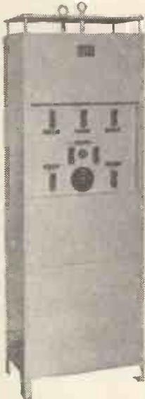
Specification: A.C. input 100-260 volts. 45-65 cycles. D.C. output 24 volts 11 amps. and 130 volts 600 m/a. very conservatively rated. L.T. and H.T. completely smoothed. All circuits fused. Mains on/off switch. Built in grey metal cabinet as illustrated. Height 5ft. 0in., width 1ft. 7½in. depth 1ft. 1½in. Weight 200 lb.
