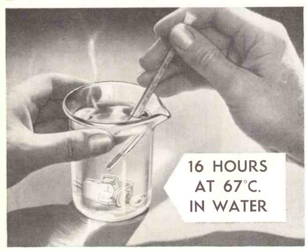
In a previous announcement we showed how ACOS GP61 Ceramic Pick-up Cartridges had passed the official BSI Test No. BF.2011, Class 112, "Basic Climatic and Durability Test for components for radio and allied equipment". Now our own laboratories have gone even further with climatic tests—and added a punishing mechanical test too. These new tests, which covered a batch of GP61s, gave average results as follows:—
