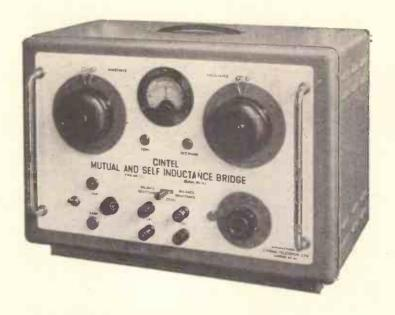
Designed for the accurate measurement of either mutual or self inductance and resistance in the range 0.001  $\mu H$  to 30mH and  $100\mu\,\Omega$  to 3000  $\Omega$  respectively.
