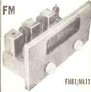
F.M. V.H.F. TUNER completely stable drift free tuning. Volume control, Tuning indicator, A.V.C. Sensitivity better than 4  $\mu\mathrm{V}$  for 20 db quieting. 21 gns. Tax paid.
