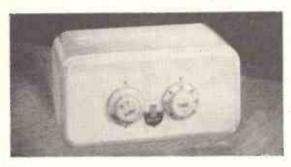
The Wolsey Convertor is a self-contained unit complete with power pack, comprising transformer with tapped primary for mains voltage selection, together with metal rectifier and R.C. smoothing.
