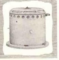
TYPE V 1000 - This vibrator is designed to produce a peak alternating thrust of ± 500 lbs. (unblown) at 1 kW. A forced draught into the vents provided in the base will allow increased input current for a correspondingly increased thrust. Unit construction has been adopted and careful attention to detail has produced a vibrator that can quickly and easily be stripped and reassembled should repairs become necessary—the design is such that no routine maintenance is required.
