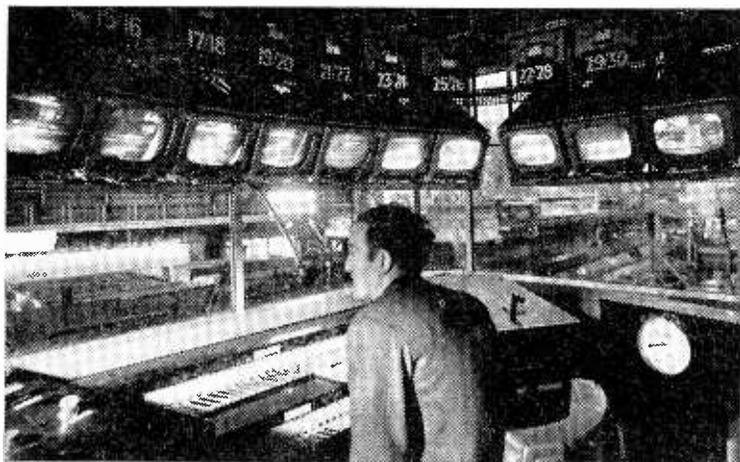
FIFTEEN closed-circuit television channels in the new rolling mill of the Steel Company of Wales at Port Talbot provide a composite view of about 700ft of railway track. This installation by Marconi's is for the remote observation of the conveyance of red-hot steel ingots from the soaking pits to the rolling mill.
