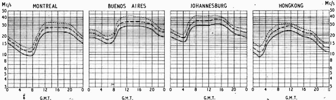
THE full-line curves indicate the highest frequencies likely to be usable at any time of the day or night for reliable communications over four long-distance paths from this country during September.
