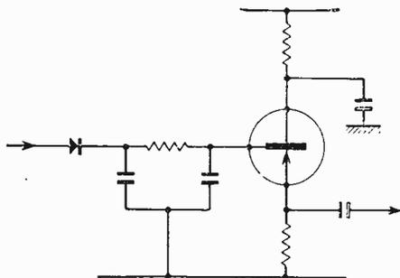
Fig. 8. Diode detector with emitter-follower audio stage.
