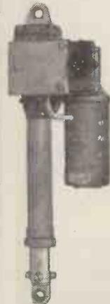
**AMERICAN AIRCRAFT 24-volt ACTUATOR UNITS.** Type ML-PM. Plunger opens and closes 4½ins., with limited switch. Will operate on 12 volts. Motor spec.: H.P. 1/6th. R. P. M. 7,500. Approx. overall size: 15 x 6 x 6in.
