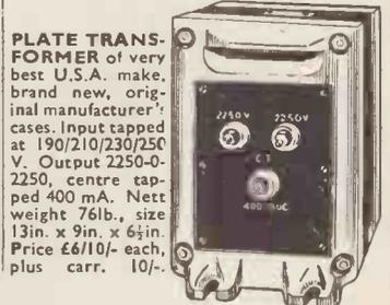
**PLATE TRANSFORMER** of very best U.S.A. make, brand new, original manufacturer's cases. Input tapped at 190/210/230/250 V. Output 2250-0-2250, centre tapped 400 mA. Nett weight 76lb., size 13in. x 9in. x 6 1/2in. Price £6/10/- each, plus carr. 10/-.
