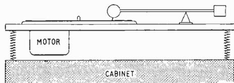
Fig. 1. Typical playing desk arrangement shown in front elevation.
