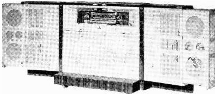
Siemens STR 30 stereo radio-gramophone with loudspeakers adjustable for spacing and angle.
