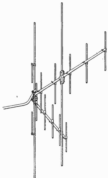
Labgear three-channel, two-direction aerial for channels 1, 8 and 9.
