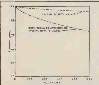
In his article (given at the 4th National Symposium of Reliability and Quality Control in Electronics in New York). Mr. R. Brewer\* describes the tests carried out on M-O.V. Special Quality valves. In comparing the reliability of these Special Quality valves with that of their commercial equivalents, he states:—"the Special Quality valves are about *seven times better* than their commercial equivalents."
