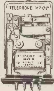
**NEW CARPENTER'S TYPE POLARISED RELAYS.** 2 x 9 500 turns at 1,685 ohms. Price 22/6 each. P. & P. 1/-.
