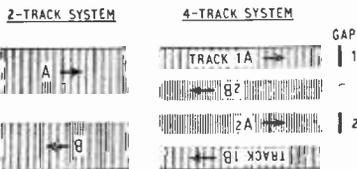
Four-track magnetic tape recording convention for single channel, compare with the two-track system. The two heads can be switched for simultaneous operation for stereo if required.
