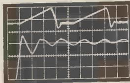
Same signal displayed simultaneously on slow sweep (upper beam) and fast sweep (lower beam) shows both coarse and fine structure of waveform. Delay range—0.5  $\mu$  sec. to 50 secs.
