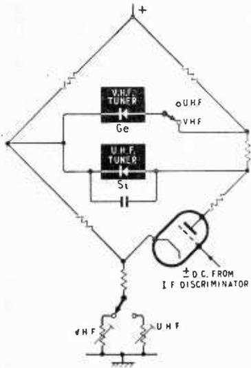
The high-impedance silicon diode is left in circuit when the set is switched to v.h.f. in the automatic tuning circuit developed by Graetz.
