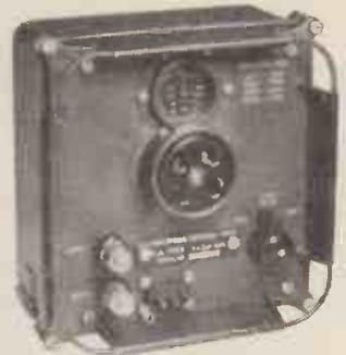
**FERRANTI TESTMETER TYPE Q.** An extremely compact self-contained multimeter. Volts 0 to 30, 150, 600 A.C./D.C., with additional 0.3 v. D.C. and 0-15 v. A.C. ranges; Milliamps 0 to 7.5, 30, 150 and 750 D.C.; ohms 0-25 K. Accuracy BSS first grade. 500 ohms per volt. Knife-edge pointer and clearly calibrated 2½in. scale. Complete with leads, prods, battery, and instructions in fitted velvet-lined 4 x 7 x 3in. case. Brand new condition, perfect working order. Bargain price. ONLY 59/6. Post 2/6.
