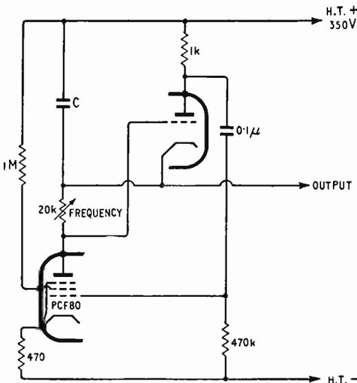
Fig. 3. Alternative method of coupling to triode.
