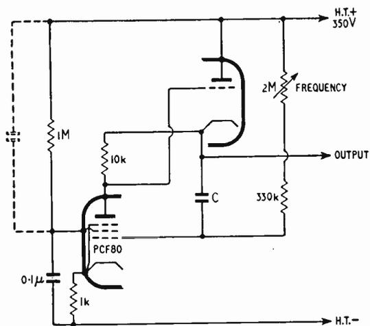
Fig. 5. Cathode coupling to pentode screen grid.
