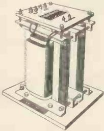
Saturable Reactors for controlling AC currents up to 220 A 100 kVA. Available for all standard AC supply voltages. Single-phase and three-phase. Standard DC control volts; 12, 24, 36 110 and 240 V.
