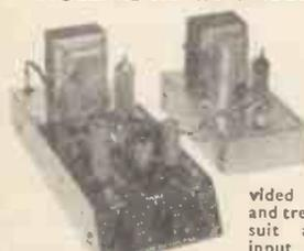
Our printed circuit version of this excellent amplifier, with ULTRA-LINEAR PUSH-PULL output stage, giving an exceptionally high quality output of 10 watts (max.). Built-in Controls are provided for independent bass and treble Tone correction to suit all types of signal input. Will match all crystal or high impedance
