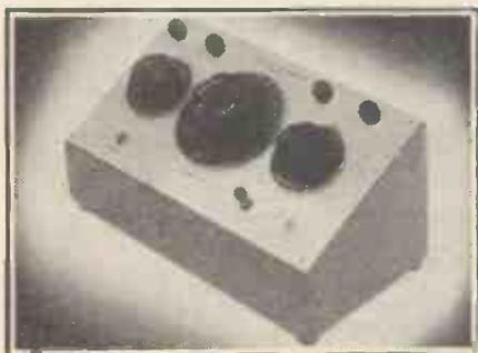
"The above, in conjunction with a Signal Generator and Valve Voltmeter, is capable of making a variety of measurements by the resonance method in the approximate frequency range of 50 Kc/s to 20 Mc/s."
