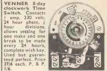
**VENNER 8-day clockwork Time Switch.** Contacts 1 amp. 230 volt. 24 hour phase, ½ hour divisions, allows setting for one make and one break to be made every 24 hours, complete with key. Used but guaranteed perfect. Price 27/6 each. P. & P. 1/6.
