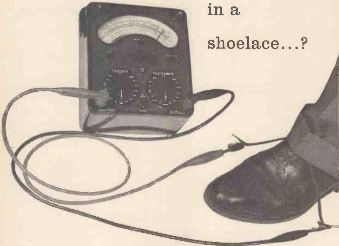
Fanciful? No, because as our photograph proves, a shoelace can be made electrically conducting by impregnating it with "dag"\* colloidal graphite.
