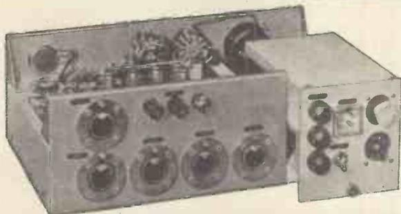
*The rear view of the Audio Mixing Unit (Type 3053) shows the A.C. mains unit partially withdrawn. Any of the power input units which can be supplied as accessories (shown below) to the mixer can be inserted in the position shown. As well as the mains input socket and fuses, the picture shows the 4 channel input sockets, the output sockets and terminals.*
