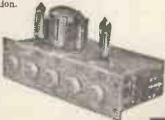
Two Mullard ECL 82 Triode Pentode Valves are incorporated in the design, they form a "CLASS A" single ended output stage in each channel. The input sensitivity is 300 mV/vo, therefore when used with most STEREO Crystal Pick-Ups, or Radio Tuning Units, an output of 2 Watts per channel is achieved, or similarly when switched to MONAURAL Pick-up position a combined output of 4 Watts is produced.
