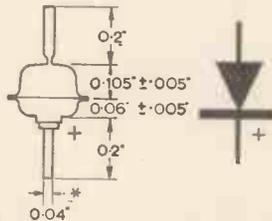
The can is covered with a plastic sleeve of wall thickness 0.01in. which is not included in the above dimensions.
