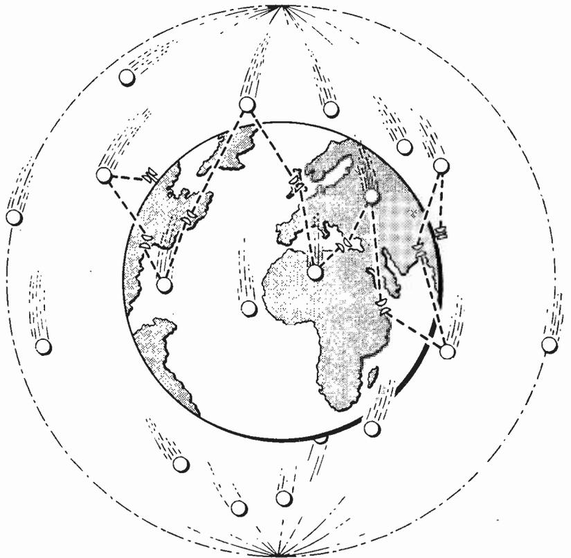
Fig. 1. Round-the-world communication by passive satellites in 3,000-mile polar orbits.
