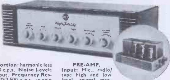
12-20 watt output. Distortion: harmonic less than .1% at 10 watts/700 c.p.s. Noise Level: 85 D.B. below rated output. Frequency Response: within 2D.B., 20/2,500 c.p.s., within .5 D.B., 10/6,000 c.p.s. Feedback: 40 D.B. total. Output Impedance: 3.4 ohms, 7 ohms and 15 ohms. Spare Power: 295 v./45 M.A. and 6.3 v. 2.5 amps. for pre-amp, radio tuner and tape amp. A.C. Input: 100/150 v. and 200/250 v. Valve Line-up: two EF86, two KT66 one GZ32. Dimensions: 16½ x 8 x 7½ in. Weight: 32lb.
