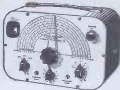
Covering 100 Kc/s-100 Mc/s. on fundamentals and 100 Mc/s to 200 Mc/s on harmonics. Metal case 10in. x 6 1/2in. x 5 1/2in., grey hammer finish. Incorporating three miniature valves and Metal Rectifier, A.C. Mains 200/250 v. Internal Modulation of 400 c.p.s. to a depth of 30%. Modulated or unmodulated R.F. output continuously variable 100 millivolts C.W. and mod. switch, variable A.F. output. Incorporating magic-eye as output indicator. Accuracy plus or minus 2%.
