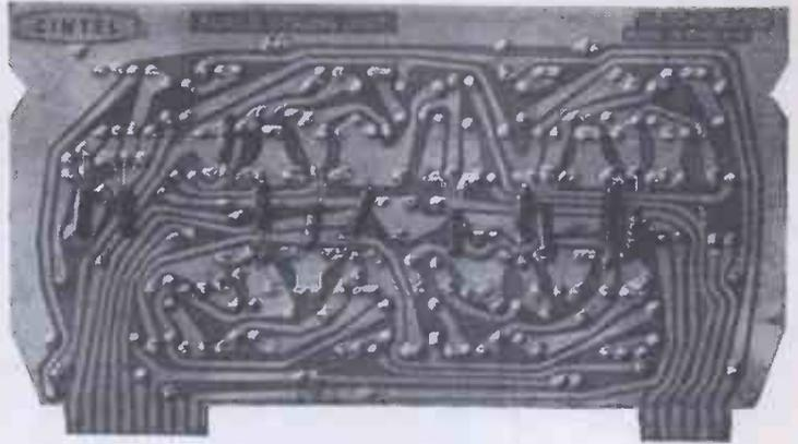
A complete range of transistorized counter panels of common size, fixing method and electrical connexion, designed to provide a flexible unit system whereby any special requirements in the counting or data processing fields can be quickly built up.
