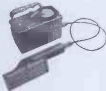
Model PAC-1S. Alpha Counter-Scintillation Type. Designed for surveying alpha contamination over a wide range of activity levels and under wide temperature variations. Consists of a probe, a single conductor 36 inch shielded cable, and rate meter. All units waterproof. Controls and scale selector, etc., are conveniently grouped around handle and can be operated by one finger of the carrying hand even when wearing protective gloves.
