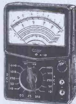
MODEL A-10 (500 Micro-amp. Movement). D.C. (2k per volt) 0/10/50/250/500/1,000 v. A.C. (2k per volt) 0/10/50/250/500/1,000 v. D.C. current 0/0.5/25/250 mA. Resistance: 0/10K/1 Meg. Size: 5 1/2 x 3 3/8 x 1 1/2 in. Weight: 17 ozs. Price £4/17/6. P.P. 1/6 inclusive of Test Prods, Instruction Book and Batteries.
