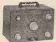
Measures capacity 10pF. to 1,000 $\mu$ F, resistance 100 $\Omega$  to 5 megohms and power factor. 5-450 v. test voltages. Safety switch provided.
