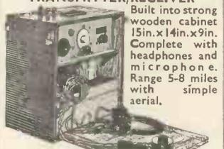
Built into strong wooden cabinet 15 in. x 14 in. x 9 in. Complete with headphones and microphone. Range 5-8 miles with simple aerial.
