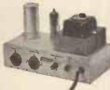
Compact, general purpose unit suitable for FM Tuners, Tape Recording Amplifiers and general Laboratory use. Input 100/120V,  $\sim$ 0/250V, 40-60 c/s. Output 6.3V 2.5A A.C.; 200, 250 270V. 120 mA. max D.C.,
