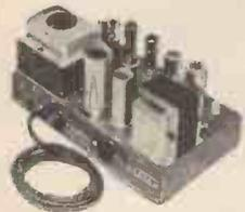
A compact high fidelity power amplifier (including auxiliary power supply). 12 watts output. Wide frequency range and low distortion. A variable sensitivity control is fitted enabling it to be used with an existing amplifier in a stereo-phononic system. Other applications include
