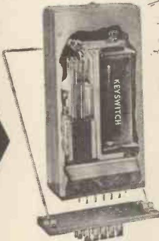
This relay incorporates 15 amp. Micro Switch, 5 amp. Mercury Switch and Standard 0.3 to 8 amp. contacts.
