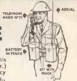
and operates from a Standard Dry Battery—HT/LT. 94/1. 3 v. (i.e. Ruben Mallory Type I). 14 of the current series of B7G valves are employed: 1-3A4, 6-1L4, 4-1T4, 1-1S5. 2-1A3. Each set is in first class condition.
