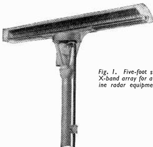
Fig. 1. Five-foot slotted X-band array for a marine radar equipment.
