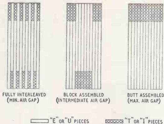
Fig. 3. Methods of assembling core laminations.
