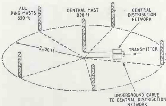
Fig. 1. Schematic diagram of the Motala ring aerial system.
