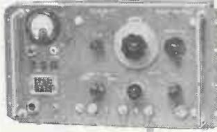
8.9 to 300 megacycles. Output 1 micro-volt to 10 millivolts. 2 1/2 in. Flush mounting. Five position switched attenuator. Variable multiplier 1 to 10, calibrated 0-20 db. C.W. square wave and sine wave outputs. Vernier tuned, 6 Band Coil turret, Potted 'C' core Transformers, Stabilised H.T. All voltage supplies including mains, R.F. filtered. External mod. by sine wave from 50 c.p.s. to 10 kc/s. or pulses down to 1/2 sec. Complete with all valves and charts.
