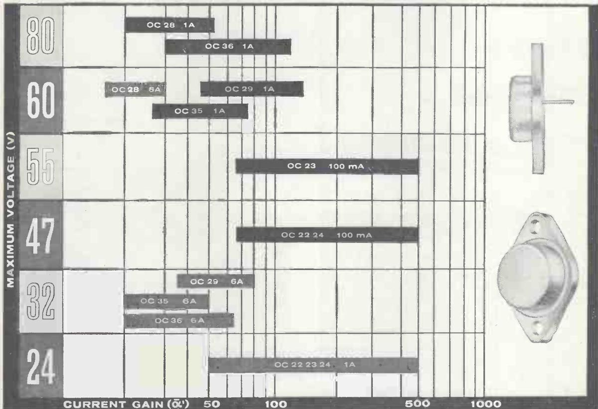
GREY is maximum allowable collector-emitter voltage at maximum continuous current.
