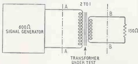
Fig. 5. Arrangement of circuit for testing a transformer.
