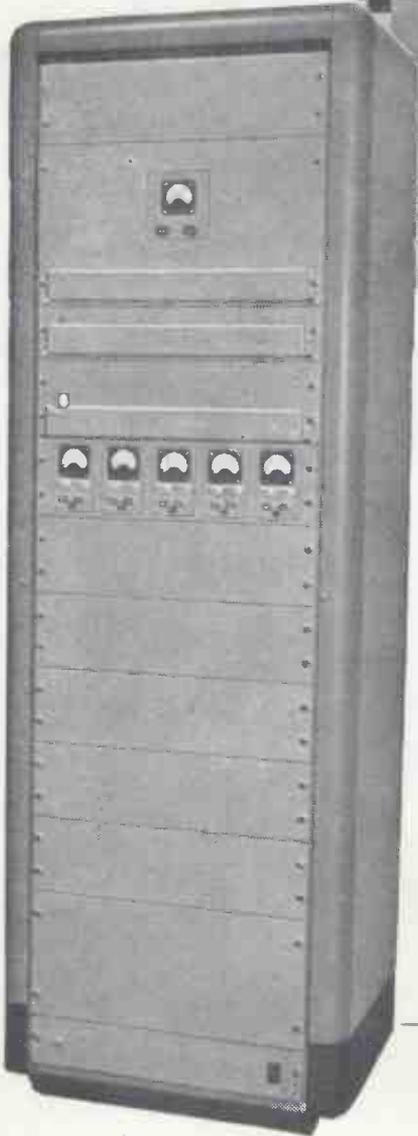
For efficient full scale servicing—the Telequipment Monoscope test card generator.
