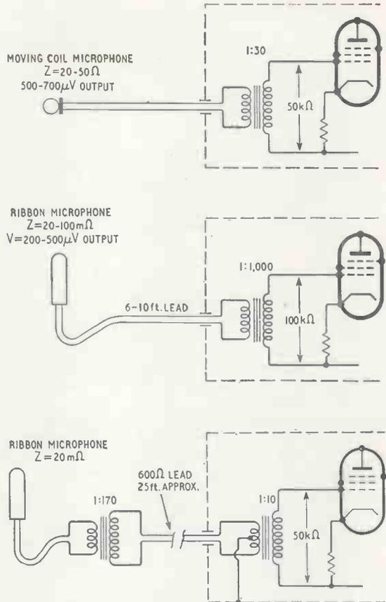
Fig. 6. Matching microphone to input of amplifier
