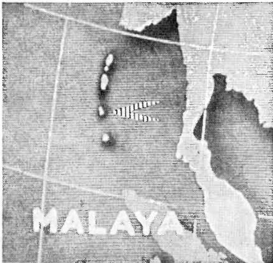
requirements, Pye, Ltd., have developed an electronic pointer generator by means of which an arrow can be superimposed on the picture and moved to any desired point by a remote-control "joystick," which carries a push-button for switching on or off. An auxiliary switch reverses the direction of the pointer.
