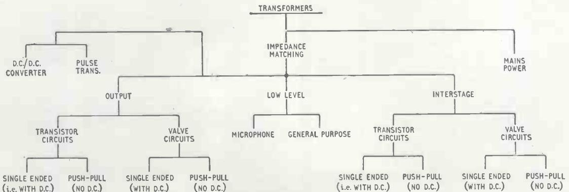
Fig. 1. Transformer family tree showing some of its numerous applications
