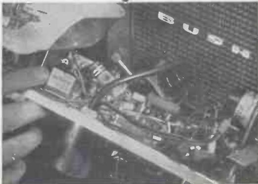
SenTerCel Contact Cooled Rectifiers have been selected by Bush for H.T. supply circuits in their domestic radio receivers. These belong to a comprehensive range of rectifiers which offer important reductions in size, weight and cost over the conventional metal rectifiers. In addition greater facility in chassis layout is permitted since they can be mounted at any angle. A table of ratings is shown below
