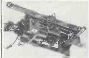
As used in many famous makes car radios. A permeability tuned Coil Pack covering medium and long wavebands, with tuned R.F. stage and complete with dial and pointer. Needs no ganged condenser. Its compact construction and small size, 7 1/2 x 5 x 1 1/2 in. enables it to be used in the smallest of car radios.
