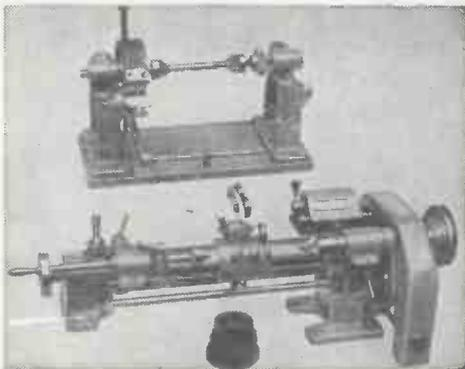
**MODEL 'E' SEMI-AUTOMATIC COIL WINDING MACHINES**
