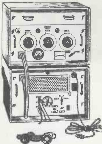
**TRANSMITTER TYPE 36.** A complete 50 watt TX for phone or CW. Covers 10-40 Mc/s. (10-15-20m.). Crystal or stabilised VFO. Push-pull 807's plate and screen modulate parallel 807's. Tested and ready to plug into AC mains. Complete with 16 valves, handset, operating instructions and circuit. Wooden cabinets may be somewhat damaged. £15 Carr. England and Wales £2.
