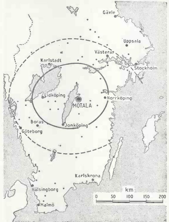
Fig. 2. Fading limits of the old (solid line) aerial system at Motala together with estimated limits of the new ring aerial. This map is reproduced from Magnusson and Stranden's article in the E.B.U. Review.
