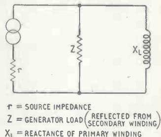
Fig. 4. Equivalent transformer primary circuit.
