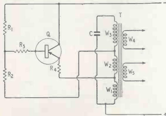
Fig. 1. Driver oscillator circuit for frequency-stabilized inverter.
