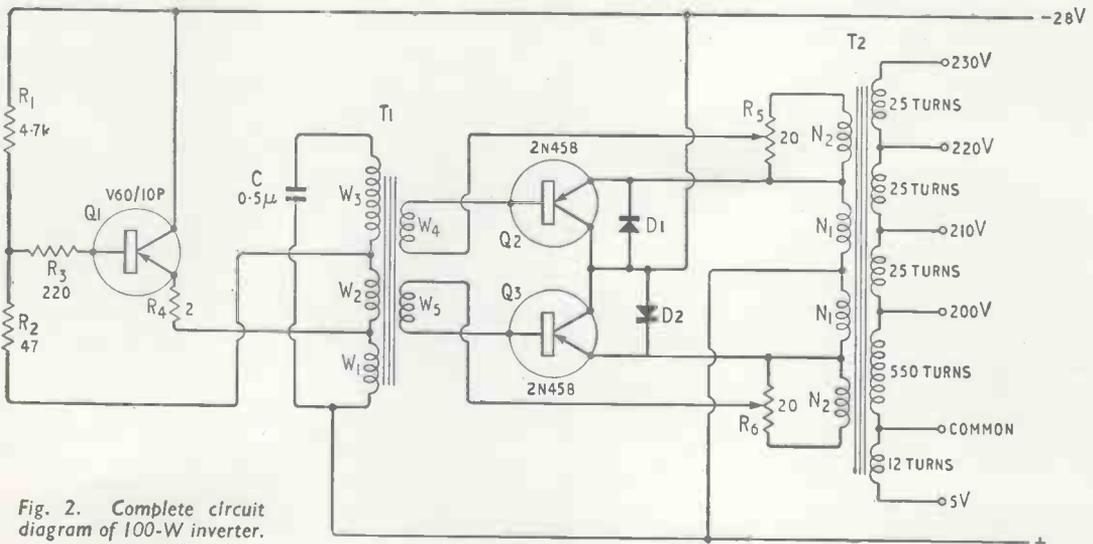
Fig. 2. Complete circuit diagram of 100-W inverter.
