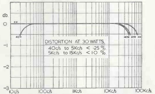
TYPICAL FREQUENCY RESPONSE OF 30W. AMPLIFIER USING AVEL TRANSFORMER TYPE NO. TO30A.
