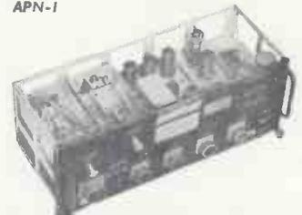
This is the attractive lightweight American Radio Altimeter that superseded the British version. A complete 14-valve radar set covering 420-460 Mc/s it is ideal for conversion to radio control of models or 70 cm. work. It embodies three self-contained sub-units in separate detachable aluminium cases, as follows:
