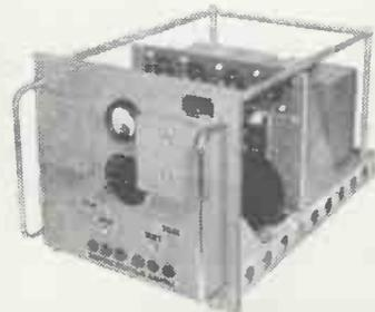
**LOW VOLTAGE POWER UNIT TYPE 15** D.C. unregulated power unit providing two separate smoothed outputs of -50V, 4A. each (+ wired to chassis). Output impedance 4.3 ohms, ripple 1 Volt R.M.S. at full load Input 230V, 50 cycles. Switched metering of current, output voltage on each channel and also A.C. input voltage. Size 13½in. x 12in. x 20½in.
