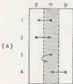
(Left): Fig. 2 A transistor consists of two diodes back-to-back, and here are shown the typical movements of (a) electrons and (b) holes.
