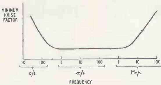
Fig. 4 Typical noise/frequency characteristic for a transistor.
