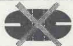
In the conventional grommet, only one thickness of plate and only one size of cable can be accommodated. No effective seal is afforded by the parallel groove.
