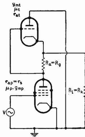
Fig. 7. Single-ended pentode-b.f. triode combination. Simplified circuit neglecting direct voltages.
