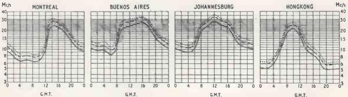
THE full-line curves indicate the highest frequencies likely to be usable at any time of the day or night for reliable communications over four long-distance paths from this country during January.
