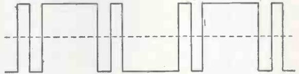
Fig. 3. Inverter output waveform with inductive load.
