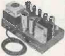
A compact high fidelity power amplifier (including auxiliary power supply). 12 watts output. Wide frequency range and low distortion. A variable sensitivity control is fitted enabling it to be used with an existing amplifier in a stereophonic system. Other applications include sound reinforcing systems, transmitter modulators, for use with tape recorders, also as a general purpose laboratory amplifier.
