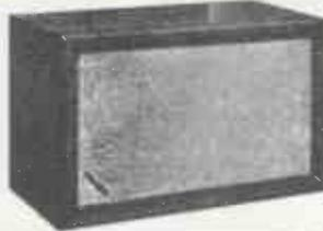
A complete 15 watt three-way high fidelity loudspeaker system, comprising a precision built 12in. unit oo-axially mounted mid-range radiator and pressure driven HF unit, providing performance from 35-20,000 c/s. Power handling capacity 15 watts. Size: 24in. wide, 11½in. deep, 14½in. high.
