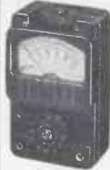
The KAPURA Mdl. U1. MULTI-RANGE TEST METER, incorporating 3in. rectangular meter. Sensitivity: 1,000 ohms per volt A.C. and D.C. Ranges: (A.C. and D.C.) 0-10-50-250-500-1,000 v D.C. current 0-100-500 m/a. 0-1 m/a. (used at 0-10 v. range).
