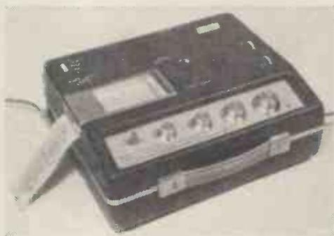
Devices R.1. recorder, with hot stylus unit in use. This may quickly be interchanged with an ink pen system.
