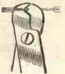
This 3-in-1 tool strips insulation without nicking the wire, cuts wire cleanly and splits extruded plastic twin flex. Adjustable to most wire thicknesses. 3/6 each (subject).
