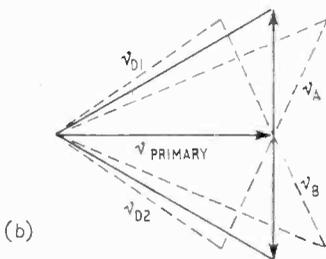
Left: Fig. 2. Common type of tuned discriminator shown at (a). Varying voltages on diodes shown in (b).
