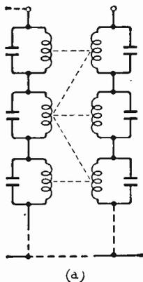
Left:—Fig. 8. Each atom has, in fact, several levels which split when the atoms are coupled.
