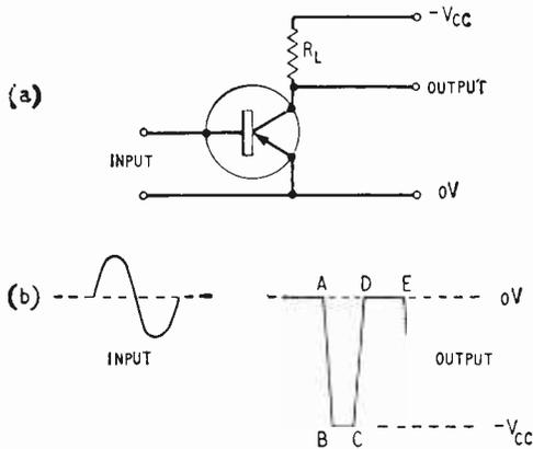
Fig. 65. Overdriven amplifier as amplified clipper.
