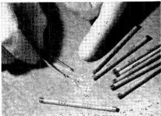
▲ STC miniature selenium rectifiers showing some of the 150 small discs used in the assembly of the components.
