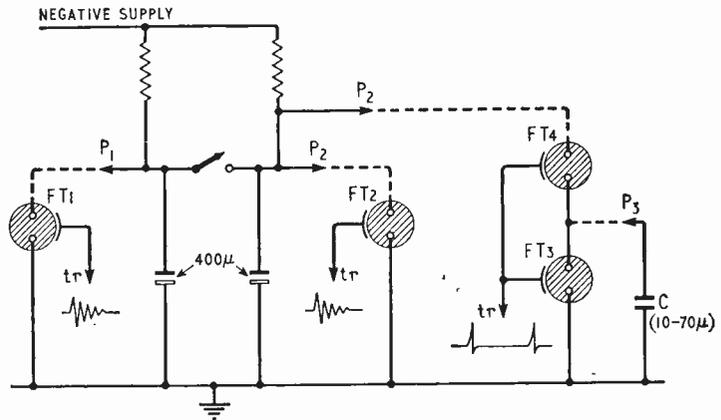
Fig. 1. Basic circuits for single, double or stroboscopic flashes. The points  $P_1$ ,  $P_2$  and  $P_3$  refer to the corresponding points in Figs. 4 and 5.
