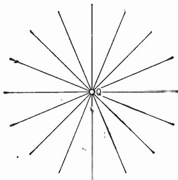
Fig. 1. Conventional representation of an electric field by lines of force takes this form around a concentrated charge in space.
