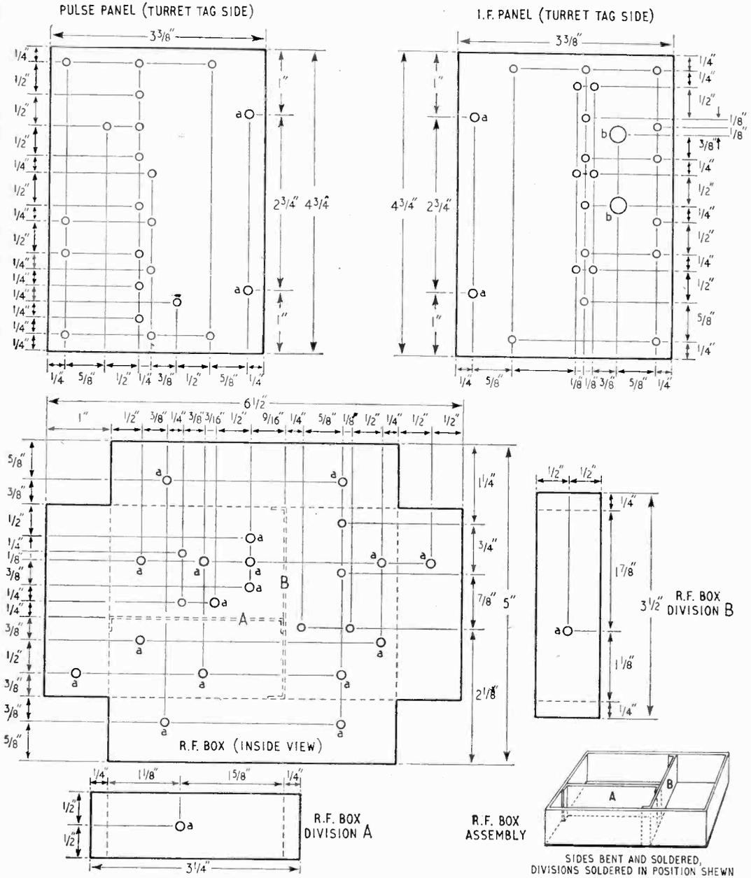
PULSE AND I.F. PANELS MADE FROM  $\frac{1}{16}$ in PAXOLIN HOLES MARKED a, DRILLED  $\frac{1}{8}$ in DIA. R.F. BOX AND DIVISIONS MADE FROM THIN TINPLATE HOLES MARKED b, DRILLED  $\frac{1}{4}$ in DIA. REMAINDER DRILLED  $\frac{3}{32}$ in DIA.
