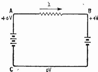
Fig. 4. Unlike the p.d. across a resistance, the p.d. across a source of e.m.f. does not reverse with direction of current.
