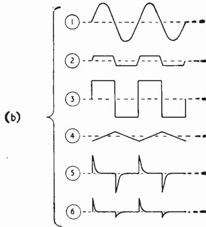
Fig. 66. Typical example of waveshaping of pulse train for computer.
