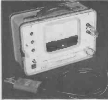
S.T.C. Type 74251 millivoltmeter introduced for general purpose and telecommunications use.
