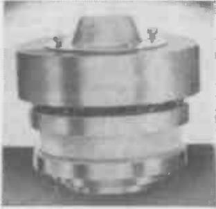
Mullard YL1230 metal-ceramic tetraode for s.s.b. applications at frequencies up to 200 Mc/s.
