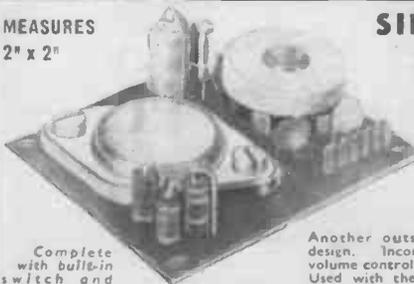
Complete with built-in switch and volume control.
