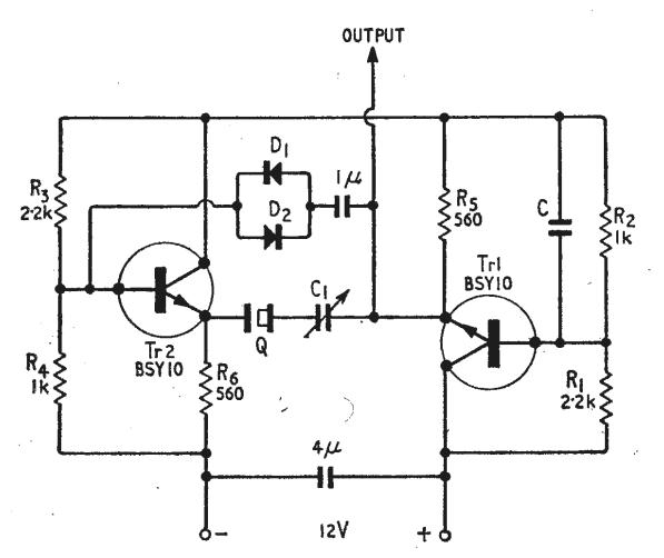
Fig. 4. Series bootstrap crystal oscillator.
