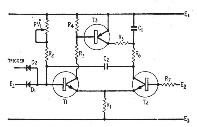
Fig. 4. Re-arrangement of Fig. 1 to use n-p-n transistors.
