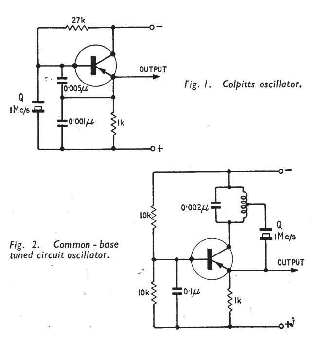
use in a frequency standard, as a clock source or as the drive oscillator for a frequency synthesizer. The oscillator works particularly well over the frequency range 100 kc/s to 5 Mc/s with the crystal operating on its fundamental frequency, as distinct from an overtone mode. Standard frequency sources commonly operate at 100 kc/s, 1 Mc/s, 2.5 Mc/s or 5 Mc/s so that any of these crystals would be suitable for use in the oscillator with no (or only minor) circuit changes.
