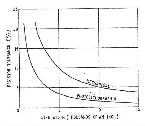
Fig. 3. Relationship between resistor tolerance and line width in Welwyn resistors produced by mechanical and photolithographical techniques.
