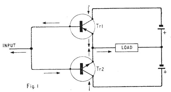
the collector-base junction of Tr1 is conducting in the forward direction and supplying a base current to make Tr2 conduct in spite of the opposing input current. Since Tr2 has approximately the full supply voltage across it the dissipation problems mentioned by Mr. Salmain occur.
