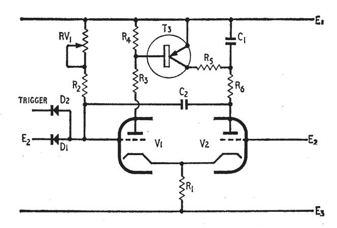
Fig. 5. Hybrid version of Fig. 1 circuit.
