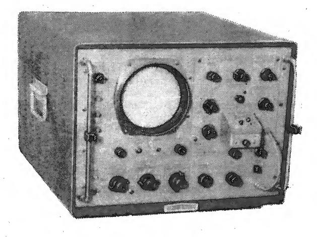
fitted with a number of alternative preamplifier plug-in units, one of which gives a d.c.-40Mc/s bandwidth at 50mV/cm. As it appears in the photograph, the instrument is fitted with a TM6456A dual-trace preamplifier module, which has a 35Mc/s bandwidth at 50mV/cm and which incorporates an electronic switching arrangement whereby two inputs can be displayed together.
