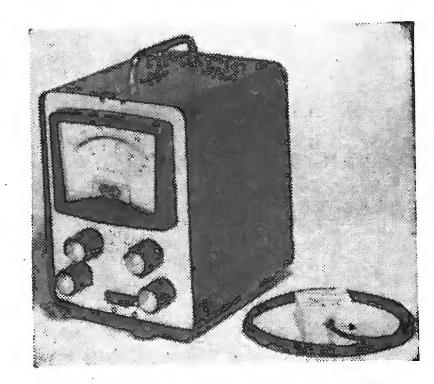
Portable gaussmeter from Preformations.
