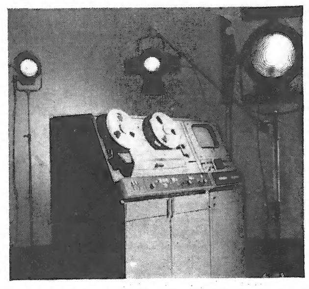
Ampex VR-2000 video tape recorder provides a 6 Mc/s vision bandwidth with automatic timebase and colour saturation control.
