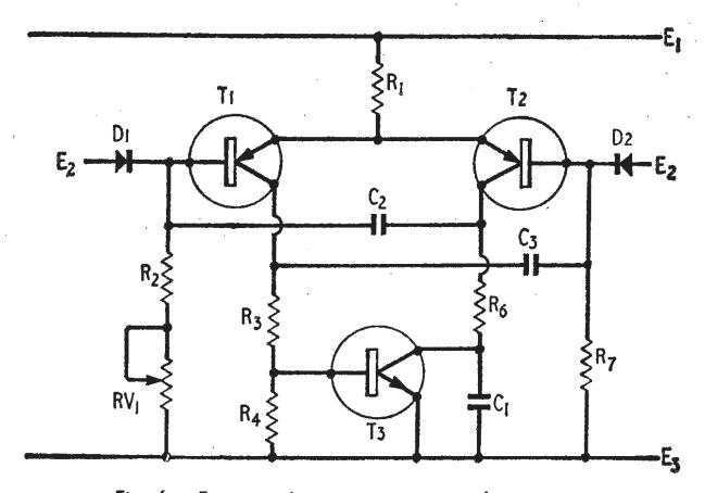
Fig. 6. Free-running ramp or sawtooth generator.
