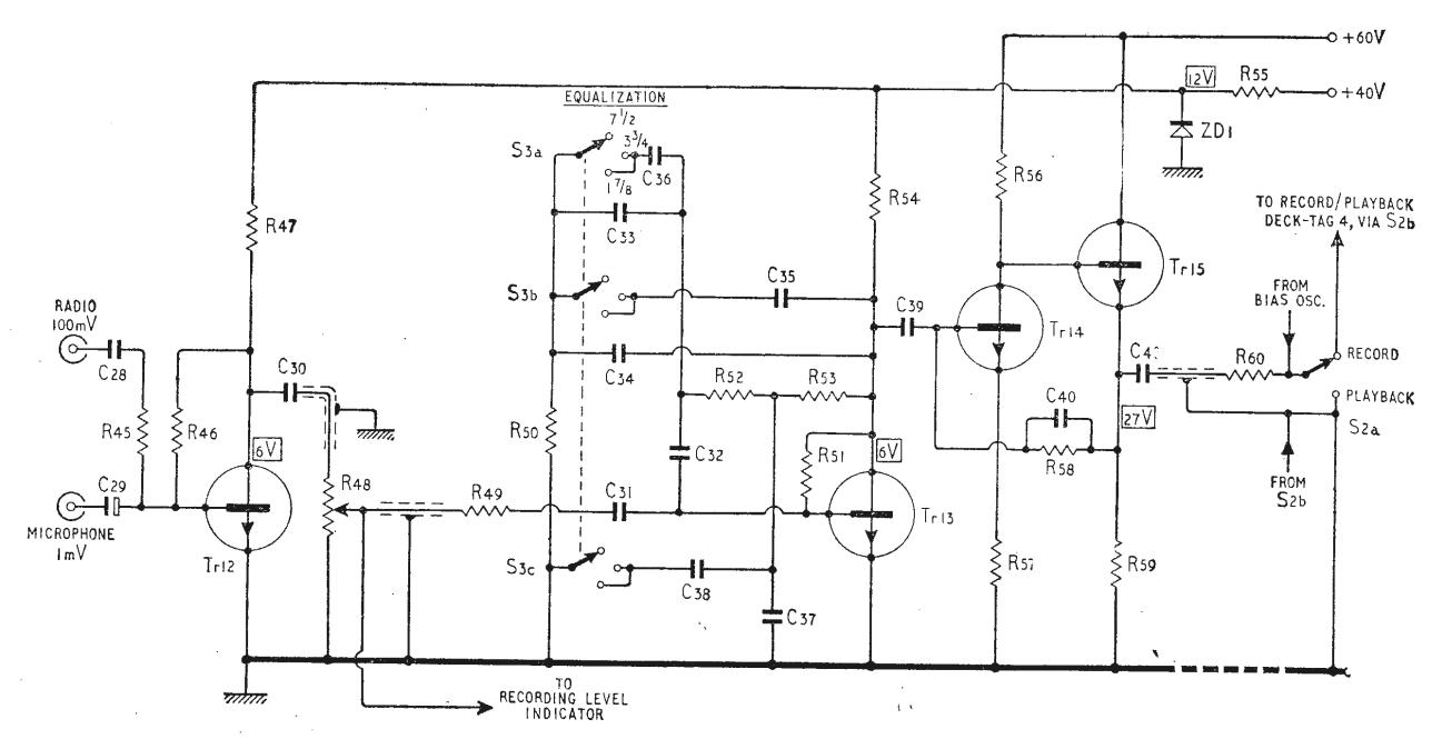
Fig. 5. Recording amplifier circuit.
