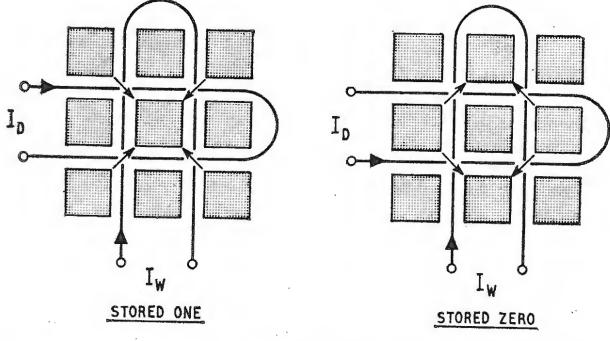
Waffle-iron thin-film store showing (above) principle of construction and (below) method of holding information by diagonal magnetization components in film.
