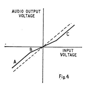
age. A similar shift occurs in the audio output voltage, since this is essentially just the average value of the voltage taken over one pulse cycle. In case B the shift in audio voltage is intermediate between the shifts in A and C. The resulting amplifier characteristic is shown by the continuous line in Fig. 4. If more realistic waveforms are used in place of those shown in Fig. 3, the effect is to round off slightly the sharp corners in Fig. 4.
