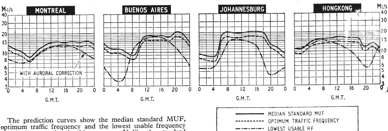
The prediction curves show the median standard MUF, optimum traffic frequency and the lowest usable frequency (LUF) for reception in this country. Unlike the standard MUF, the LUF is closely dependent upon such factors as transmitter power, aerials, and the type of modulation. The LUF curves shown are those drawn by Cable and Wireless Ltd. for commercial telegraphy and assume the use of transmitter power of several kilowatts and aerials of the rhombic type.
