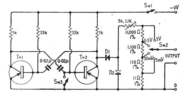
Fig. 54. Vertical sensitivity calibrator circuit for oscilloscope. Trl and Tr2 are germanium alloy 7 Mc/s r.f. types (e.g. NKT 128); D1 is a germanium diode (e.g. NKT 149 B30); and D2 is a 6V (approx.) low power zener diode.
