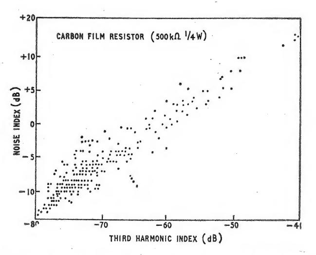
Correlation between third harmonic index and noise index in a large group of carbon film resistors (Welwyn). Correlation coefficient is 0.9.
