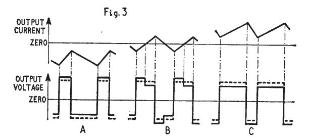
through the load. The amount of distortion is of the same order as that of the corresponding class B amplifier having the same quiescent current, and it would appear to render the open-loop system unsuitable for applications which require the lowest distortion figures, whereas with the closed-loop system the distortion can be made as low as is desired by increasing the foodback
