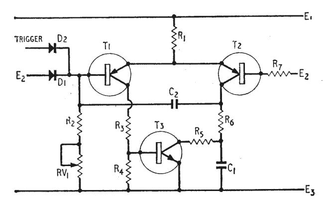
Fig. 1. Basic circuit of ramp generator.
