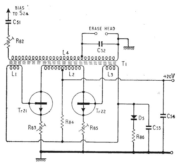
Fig. 8. Erase and bias oscillator designed for Collaro Studio tabe deck.
