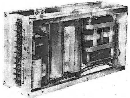
Modular power supply unit with stabilized d.c. output from Advance Electronics.
