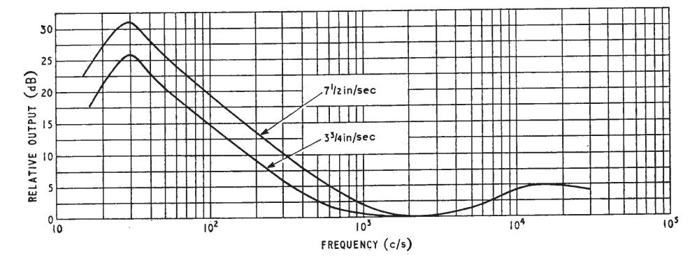
Fig. 2. Playback preamplifier amplitude-frequency response.
