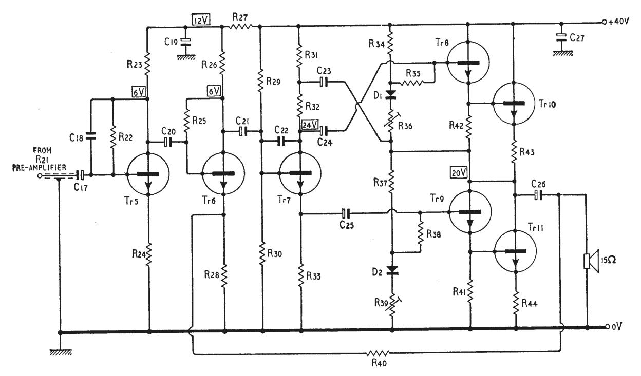
Fig. 3. 7-watt power amplifier. Tr10 and Tr11 are mounted on  $2\times2\times\frac{1}{16}$  in copper or aluminium heat sinks insulated from the chassis. Alternatively, the chassis may serve as a heat sink, from which Tr10 and Tr11 are electrically insulated by 0.002in mica washers.
