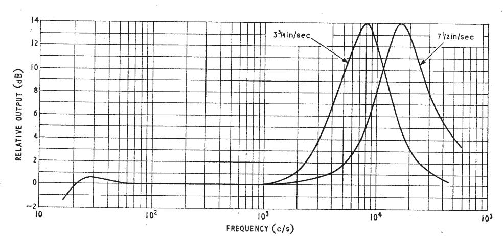
Fig. 6. Record amplifier amplitude-frequency response.
