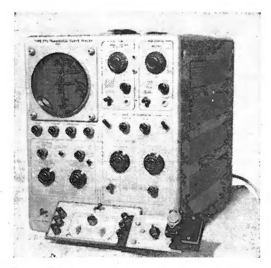
Fig. 52. Transistor curve-tracer scope system: Tektronix Type 575
