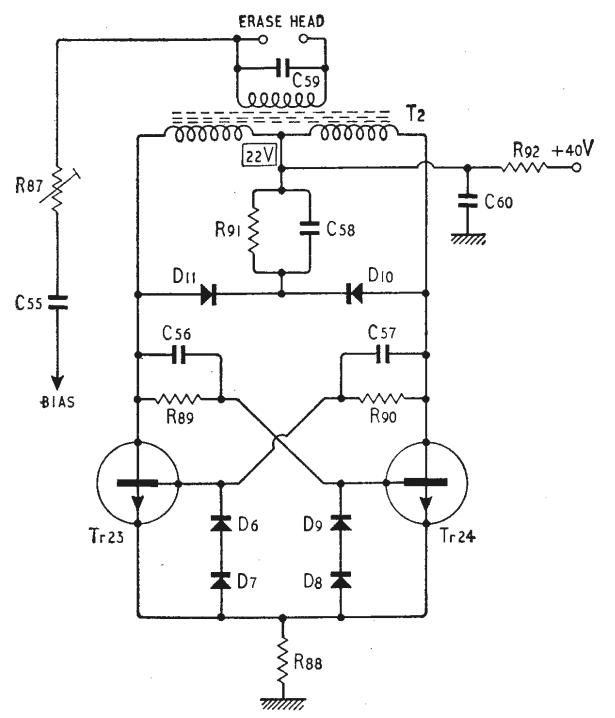
Fig. 9. Class D oscillator designed for use with Wearite deck, model 4B.
