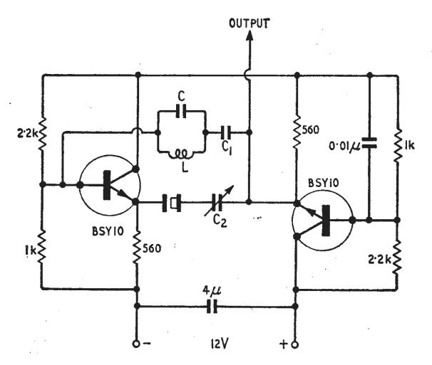
Fig. 5. Suppression of undesired oscillations by frequency-selective feedback.
