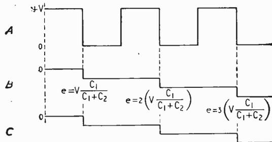
Fig. 3(a). Diode-transistor pump (original version). D<sub>1</sub> is replaced by the emitter follower Tr1 so that the voltage at B follows that at C. (b) Voltage waveforms at points A, B and C in (a).
