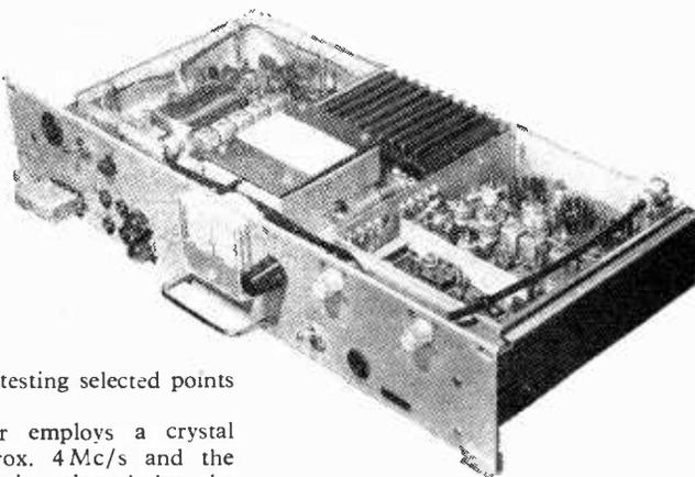
This is the first point-to-point equipment to be produced by Cossor Communications Co., Ltd., of Elizabeth Way, Harlow, Essex. It is designed to provide one or two speech channels with or without supervisory control tones.
