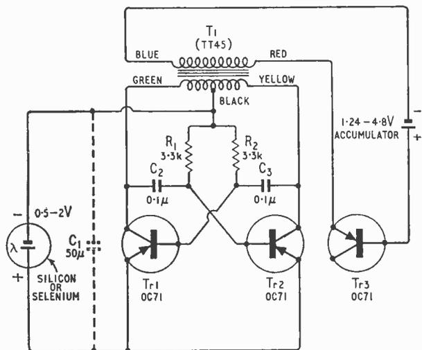
Fig. 3. Circuit of the converter charger. Suppliers of some of the components are listed in the panel on this page.
