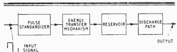
Fig. 1. Basic pump arrangement.
