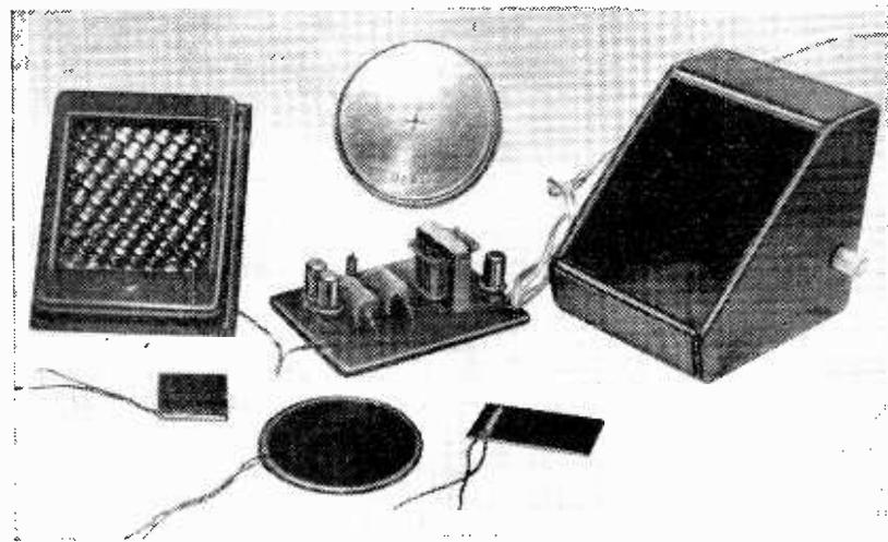
Details of the solar battery charger. In the foreground selenium wafers. Left to right: four-cell silicon sun battery, converter and box. In the background: 1,000 DKZ Deac cell.
