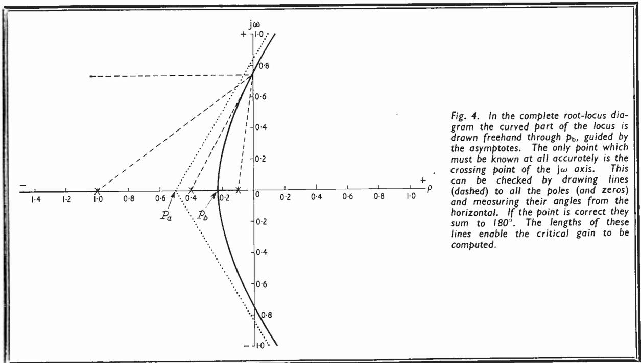
Fig. 4. In the complete root-locus diagram the curved part of the locus is drawn freehand through  $p_b$ , guided by the asymptotes. The only point which must be known at all accurately is the crossing point of the  $j\omega$  axis. This can be checked by drawing lines (dashed) to all the poles (and zeros) and measuring their angles from the horizontal. If the point is correct they sum to  $180^\circ$ . The lengths of these lines enable the critical gain to be computed.
