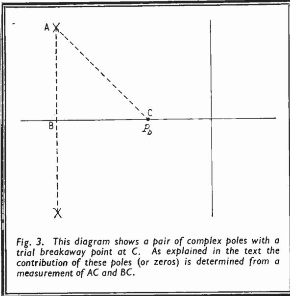
Fig. 3. This diagram shows a pair of complex poles with a trial breakaway point at C. As explained in the text the contribution of these poles (or zeros) is determined from a measurement of AC and BC.
