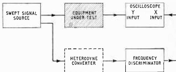
Fig. 9. "Frequency base" generation for oscilloscope displays.
