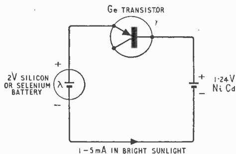
Fig. 1. Circuit of a simple charger.
