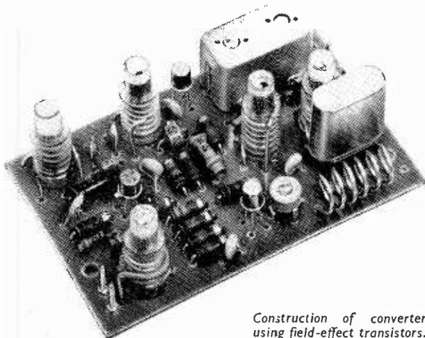
Construction of converter using field-effect transistors.
