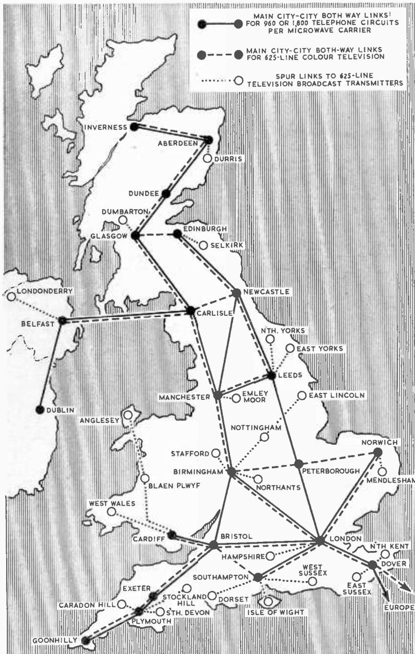
To meet expected trunk telephone and television traffic the Post Office plans this microwave network for 1970. Relay stations at intervals of 25-30 miles are being built along each route.
