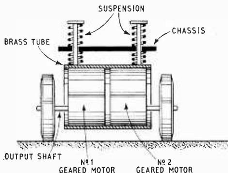
so that the whole tube can absorb shocks, etc. (As a three-wheeler suspension is used, springing is not primarily necessary to hold the wheels in contact with the ground on rough surfaces.) The Graupner motors are equipped with integral 60:1 reduction ratio gearheads, and the road wheels are fitted directly to the gearhead output shafts. The front wheel is mounted as shown below. In the prototype the height of the shaft, and
