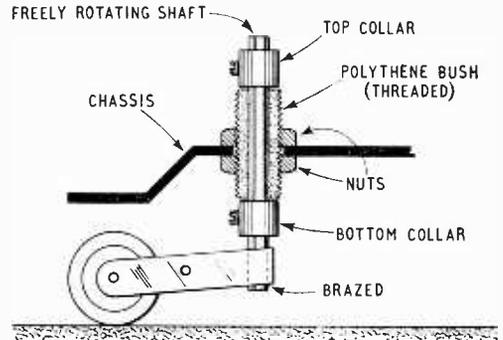
hence the clearance given to the dummy front wheels is adjustable, as is the effective length of the castor arm.
