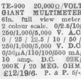
**TE-900 20,000Ω/VOLT GIANT MULTIMETER**
