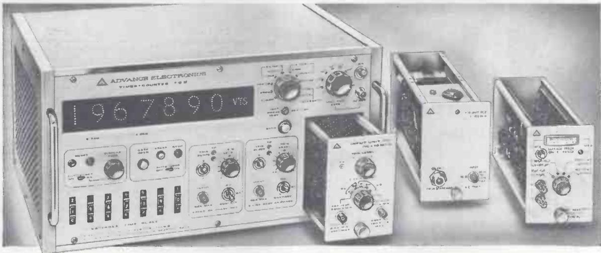
Measures frequency, period, phase angle, pulse width, time, resistance, or capacity.
