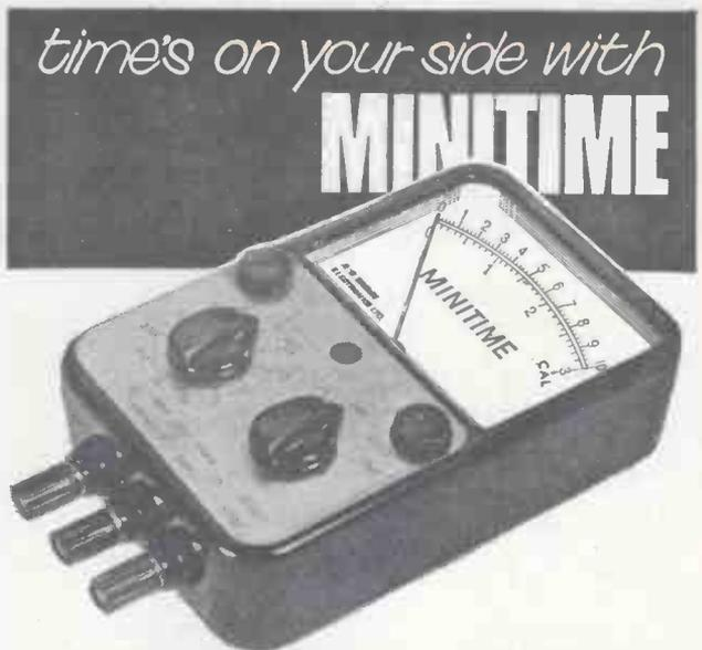
High accuracy, wide range, low cost. These are among the many advantages of MINI TIME. Comprising a pocket size black moulded case with contrasting front panel and 3in. meter. MINI TIME is designed to measure the time interval between the opening and/or closing of contacts, or width of pulses in active circuits. Range: 1 milli-10 secs.
