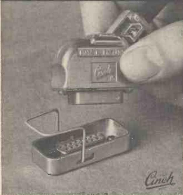
Designed to comply with D.E.F 5325 PAT. 110, these connectors consist of one-piece Diallyl Phthalate moulding with hard gold plated plug pins, socket contacts, and beryllium copper contact clips. Closed entry contact design eliminates the risk of damage to the sockets by test probes. The shells are of passivated cadmium plated steel and the covers and cable clamps are of die-cast aluminium Grade LM6.
