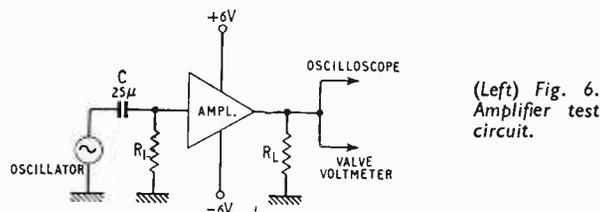
(Left) Fig. 6. Amplifier test circuit.
