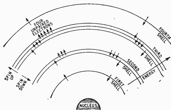
Fig. 2. Showing the relative energy levels of electrons in an iron atom.
