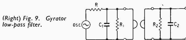
(Right) Fig. 9. Gyrator low-pass filter.
