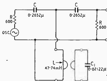
(Left) Fig. 10. Gyrator high-pass filter (cut-off frequency 1kc/s).
