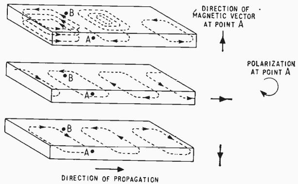
Fig. 5. Magnetic field of the  $TE_{10}$  mode in rectangular waveguide.
