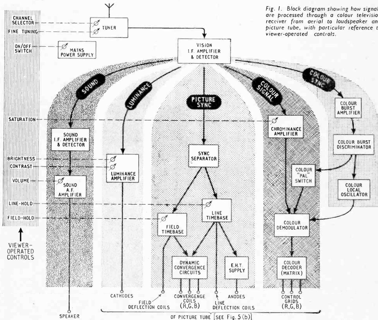
Fig. 1. Block diagram showing how signals are processed through a colour television receiver from aerial to loudspeaker and picture tube, with particular reference to viewer-operated controls.
