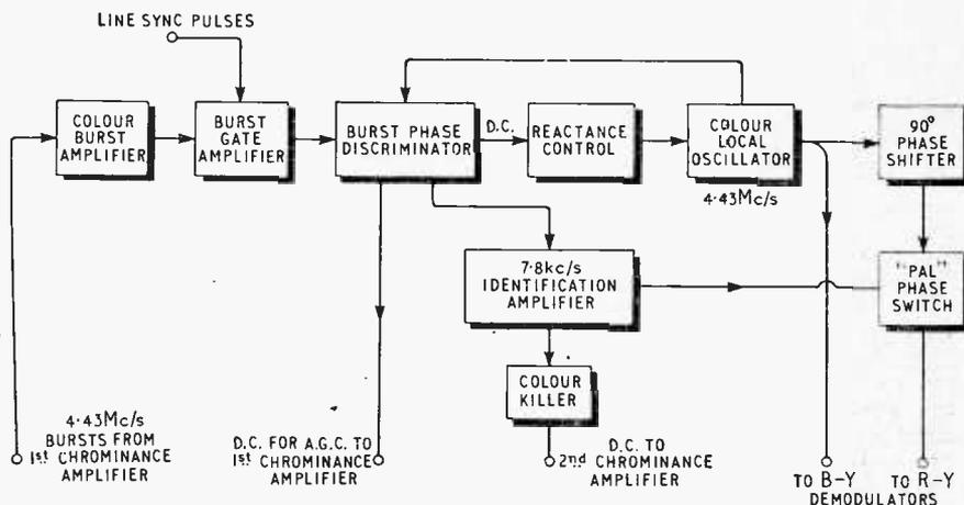
into two streams of 4.43 Mc/s r.f. signals. These have now to be demodulated to recover the original modulation to control the picture tube.
