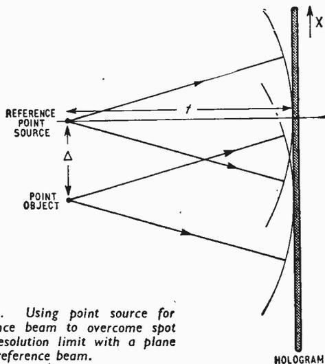
Fig. 8. Using point source for reference beam to overcome spot size resolution limit with a plane wave reference beam.
