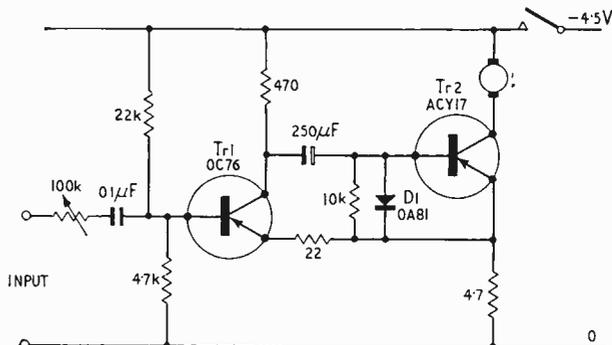
stage amplifies the input signal fairly linearly until switching occurs. D1 is to shorten the paralysis time on switching back. Without this diode the device remains insensitive for about two seconds after the knob has moved and fails to indicate any overloads during this time. The high sensitivity obtained by this system enables the device to be connected to low level monitor outputs of relatively high impedance.
