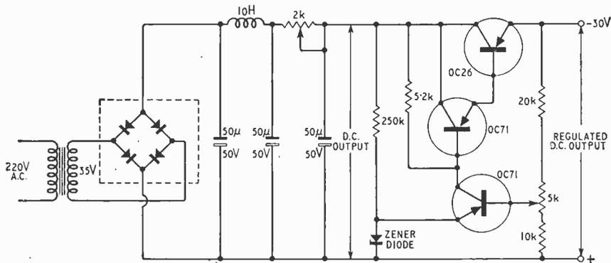
Fig. 4. Power supply unit for the tachometer.
