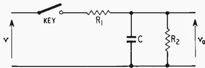
Fig. 2. Equivalent keying circuit.
