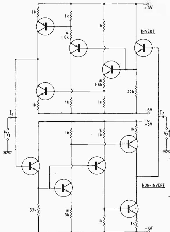
Fig. 4. Simple gyrator. (Below) Fig. 5. High-grade gyrator.
