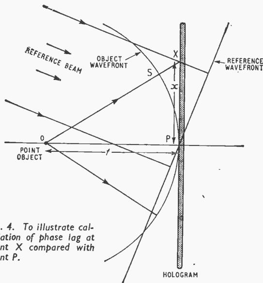
Fig. 4. To illustrate calculation of phase lag at point X compared with point P.
