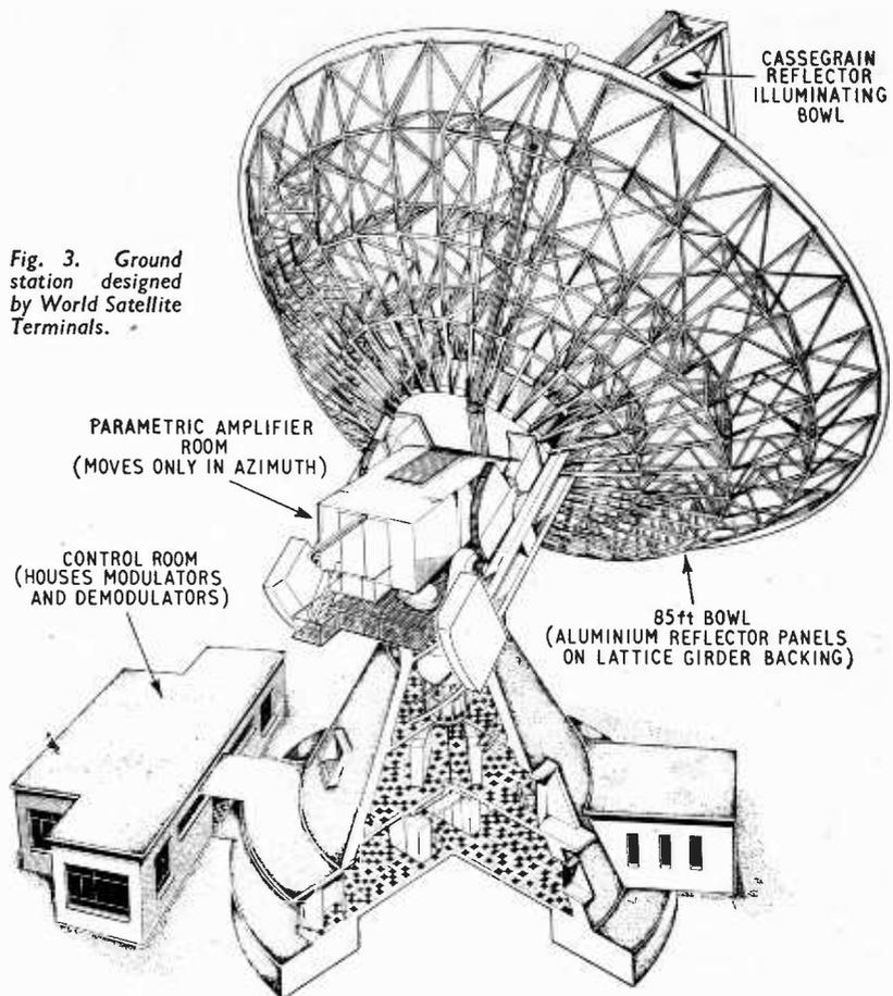
Fig. 3. Ground station designed by World Satellite Terminals.
