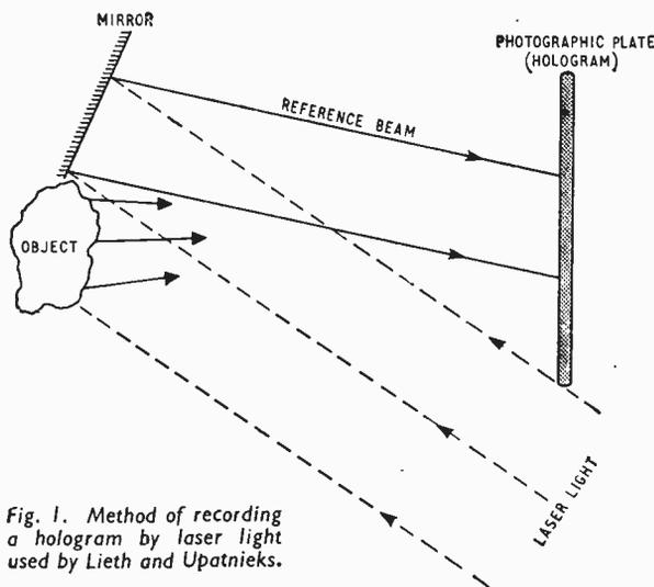
Fig. 1. Method of recording a hologram by laser light used by Lieth and Upatnieks.
