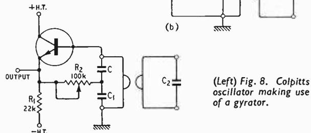
(Left) Fig. 8. Colpitts oscillator making use of a gyrator.
