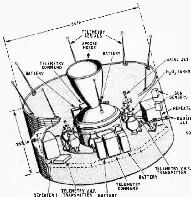
Fig. 2. Construction of the Hughes Intelsat II satellite.
