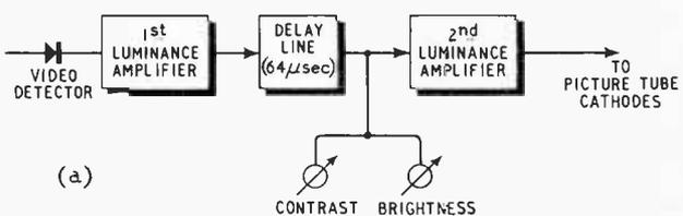
Fig. 5. (a) Main features of the luminance amplifier which isolates the brightness (black-and-white) information from the composite video signal after the video detector and drives the cathodes of the colour picture tube (British 625-line system). The graphical symbol of the picture tube at (b).
