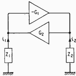
(Left) Fig. 3. Gyrator using back-to-back parallel amplifiers.
