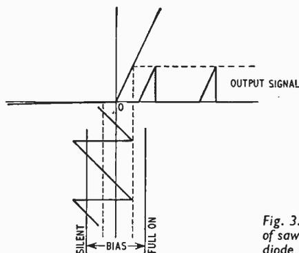
Fig. 3. Distortion of sawtooth during diode keying.
