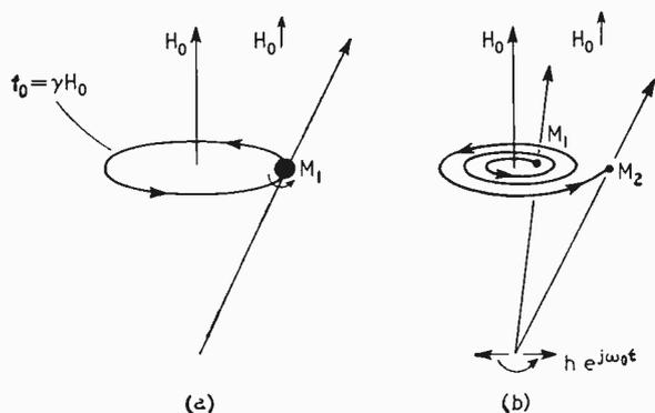
Fig. 3. Precession of an unpaired electron under the influence of external magnetic fields. At (a) is shown the precession with an external steady magnetic field  $H_0$ . A clockwise polarized r.f. field will have no effect. At (b) is the precession under the influence of a steady field  $H_0$  plus an anti-clockwise polarized r.f. field  $h e^{j\omega_0 t}$ .
