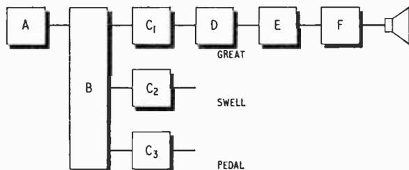
Fig. 1. Block diagram of an electronic organ, A, main oscillators; B, dividers; C<sub>1</sub> C<sub>2</sub> C<sub>3</sub>, keying systems; D, voicing networks; E, summing system and pre-amplifier; and F, power amplifier.
