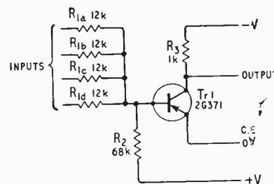
Fig. 4. Circuit of NOR gate. (Cost per gate: 1s 3d as for NOT gate plus 2d per extra input)
