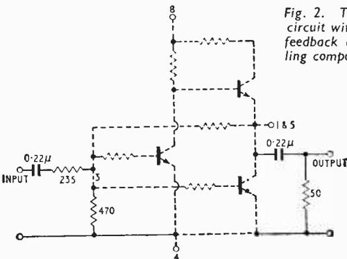
Fig. 2. The  $\mu$ L900 circuit with additional feedback and decoupling components.
