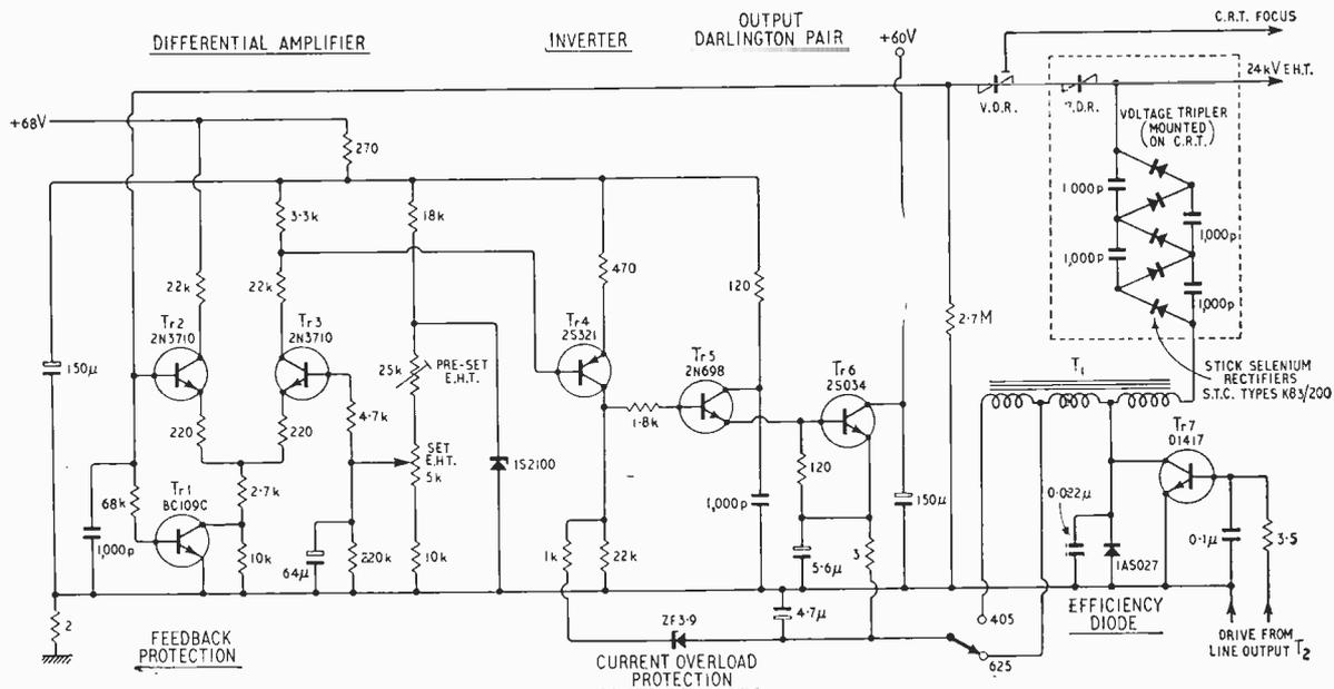
Fig. 2. Circuit of e.h.t. unit. The e.h.t. generator itself is on the right and the closed-loop voltage-regulation circuitry on the left.
