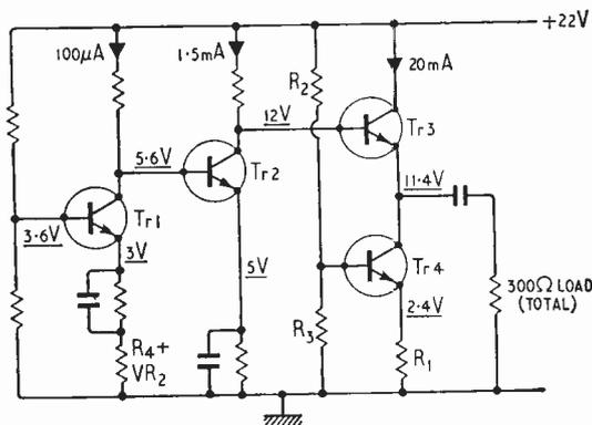
Fig. 1. Basic circuit of amplifier section.
