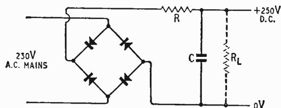
Fig. 5. Basic circuit of mains-derived h.t. d.c. supply for colour receiver.
