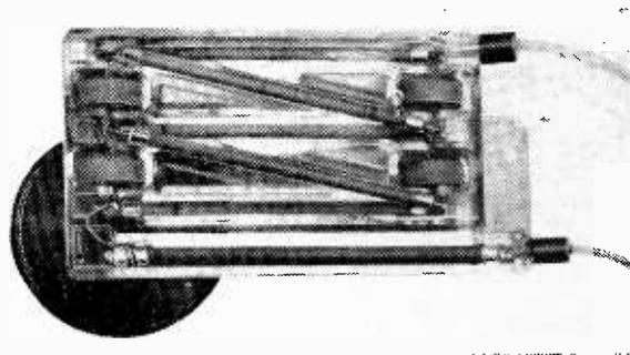
The e.h.t. Cockcroft-Walton voltage tripler is a separate sealed unit which is attached directly to the c.r.t. final anode by a clip connector (in the centre of a black circular insulating cover which can be seen underneath)
