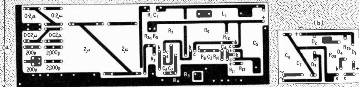
Fig. 5. Suitable printed board layouts. The smaller is the power supply board.
