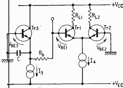
Fig. 5. Current switch biasing in which Tr1, Tr2 and Tr3 are on the same silicon slice.
