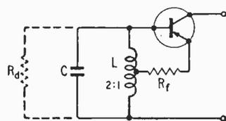
Fig. 2 Essentials of the Q multiplying circuit.
