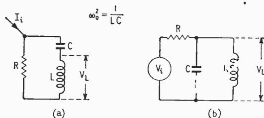
Fig. 1 Basic filter circuits. Variable selectivity can be obtained by cascading several.
