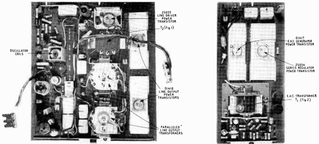
Left: Layout of line timebase unit on replaceable printed-circuit module. Right: The e.h.t. unit on its replaceable printed-circuit module.
