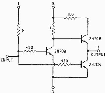
Fig. 1. Circuit of the Fairchild  $\mu$ L900 buffer.
