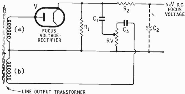
Fig. 3. Obtaining 5-kV d.c. supply for adjustable focus voltage on second anodes of shadow-mask colour picture tube.
