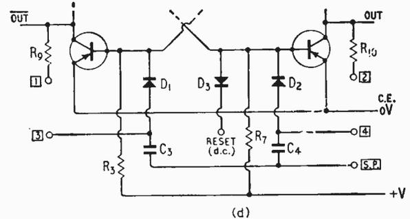
Fig. 11. (a) Set/reset d.c. bistable circuit (Cost per d.c. bistable: 8 resistors at 2d each, 2 transistors at 9d each = 3s 6d). At (b), modifications to (a) to produce set/reset a.c. bistable. (Cost per a.c. bistable = 4s 11½d). At (c), modifications to (a) to produce counter bistable. (Cost per counter bistable: 5s 3½d). At (d), modifications to (a) to produce shift register bistable. (Cost 5s 3½d)
