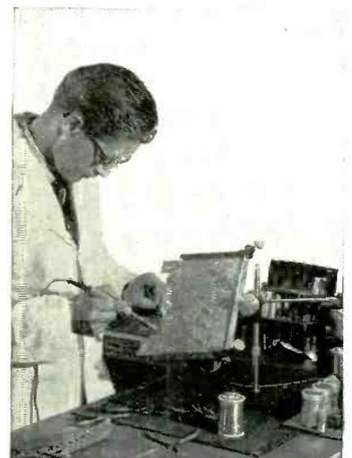
**H. J. Leak & Co. Ltd.** Ersin Multicore Savbit alloy is shown in use in the wiring construction of the Leak Integrated Stereo 30 Transistor Amplifier. In order to ensure the utmost reliability, the Leak High Fidelity equipment has been made with Ersin Multicore Solder for more than 20 years.
