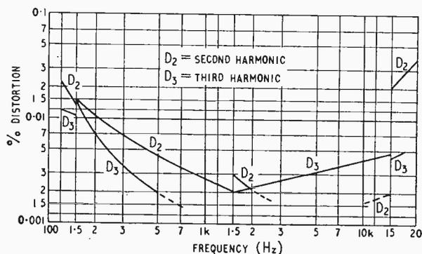
Fig. 6. Distortion characteristics.
