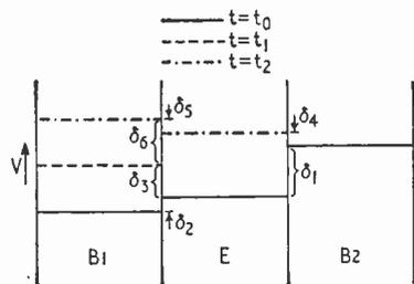
Fig. 2. D.C. behaviour of current switch of Fig. 1. Full line represents condition at each node when  $t=t_0$  ( $Tr_1$  off,  $Tr_2$  on). Broken line corresponds to  $t=t_1$  ( $t_1 > t_0$ ) when  $Tr_1$  is on verge of conduction. For  $t_1 > t > t_2$ ,  $Tr_1$  is fully on and  $Tr_2$  is off, shown by chain line.
