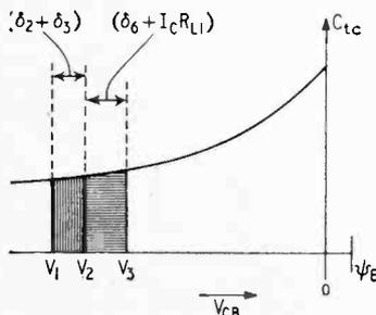
Fig. 4.  $C_{te}$  as a function of  $V_{CB}$ . Collector-base junction is always reverse-biased in current steering circuits.
