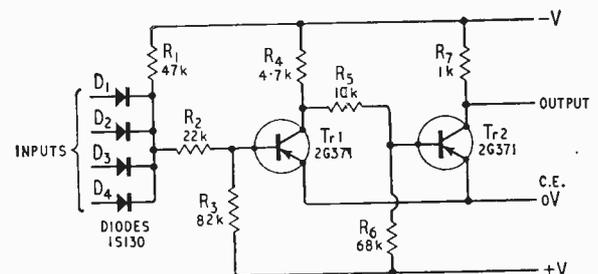
Fig. 5. Circuit of AND gate. (Cost per gate: 7 resistors at 2d each, 4 diodes at 4½d each, 2 transistors at 9d each = 4s 2d)
