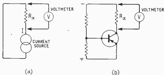
Fig. 1. (a) The measuring technique employed.
