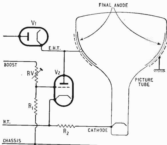
Fig. 2. Basic e.h.t. regulation circuit
