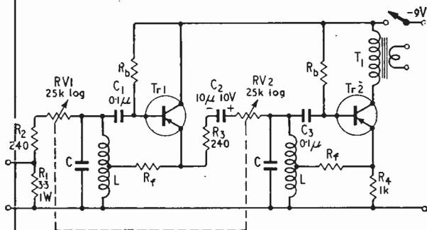
Fig. 3. Complete Q multiplier circuit. All resistors are  $\frac{1}{10}$ W  $\pm 10\%$  unless stated otherwise. Transistors are OC7's or similar l.f. types.
