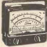
0.5/2.5/10/50/250/500/1,000 v. D.C. 0.3/10/50/250/500/1,000 v. A.C. 0/10/100μA/10/100/500 mA / 2.5/10 Amp. 0/1K/10K/100K/10M/100MΩ. -10 to 49.4 dB. £16/16/- P. & P. 5/-
