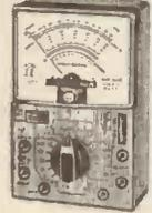
**MODEL AF-105, 50KΩ/Volt.** Mirror scale, built-in meter protection. 0/3/12/60/120/300/600/1,200 v. D.C. 0/6/30/120/300/600/1,200 v. A.C. 0/30μA/6/60/300 mA. 12 Amp. 0/10K/1M/10M/100 MΩ -20 to +17 dB. £8/10/- P. & P. 3/6.
