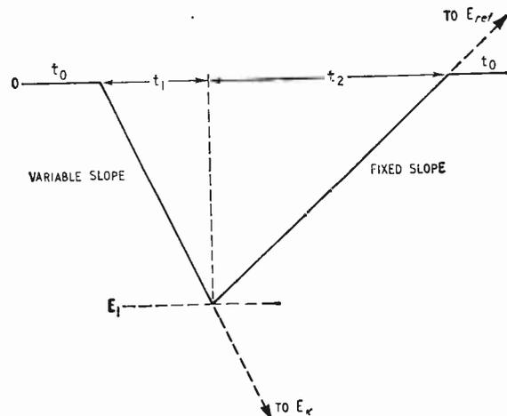
Fig. 6. Showing the charge and discharge of the integrating capacitor.
