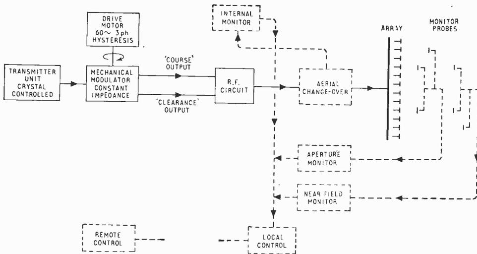
Fig. 3. I.L.S. "quadrature clearance" system; block schematic of the localizer transmitter equipment.
