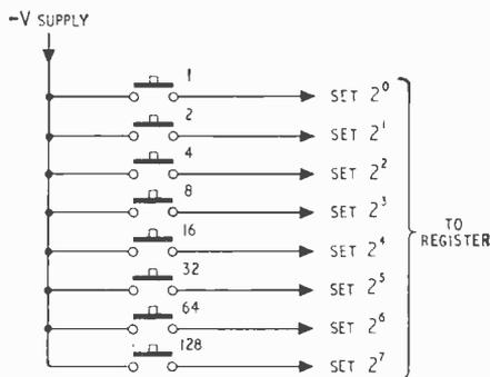
Fig. 34. The input unit for entering data.
