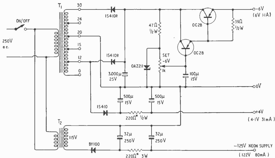
Fig. 33. The computer power supply. If a double wound 115 V transformer ( $T_3$ ) cannot be obtained, use an isolating transformer and an auto-transformer ( $T_3$  &  $T_4$ ) as shown in inset. Resistors marked \* must be increased in value when the power supply is used for test purposes.
