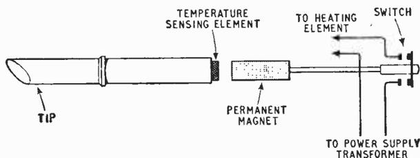
Using the Curie point principle, and operating as described, the tip temperature controls the switching of the iron. The switch and permanent magnet are housed in the handle of the iron.
