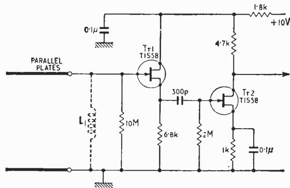
Fig. 2. The broadband amplifier circuit.
