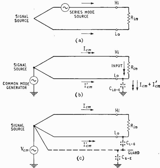
Fig. 14. (a) series mode (b) common mode without guard (c) common mode with guard—equivalent circuits.
