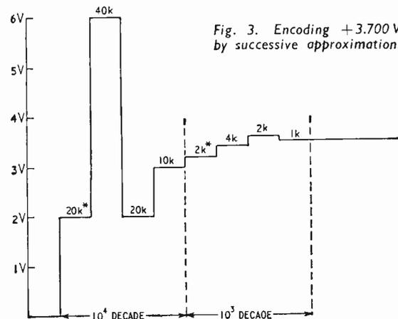
Fig. 3. Encoding +3.700 V by successive approximation.
