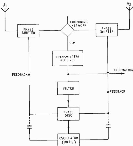
Fig. 5. Showing how the gain of the receiver is used in the control loop of the active aerial system.
