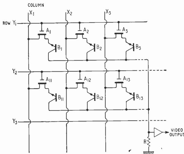
Fig. 1. Schematic arrangement of Fairchild solid-state imaging array. Each photo-element point consists of an m.o.s.f.e.t. (A) and a photo-transistor (B).
