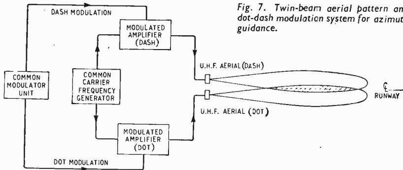
Fig. 7. Twin-beam aerial pattern and dot-dash modulation system for azimuth guidance.
