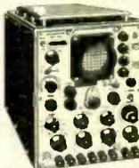
An extremely high quality oscilloscope originally costing £400. Switched beam. Identical Y1, Y2 Amplifiers D.C. to 9 Mc/s. Bandwidth 3mV/cm to 100 V/cm. Time base 10 μsec. to 10 m/sec. Calibrator. X amplifier D.C. to 2.5 Mc/s. 2 Modulation. 110/200/250V. A.C. Supplied in good working order. £65 carriage £2, or available as received from Ministry non-serviced £50. carriage £2. (Handbook £2 extra.)
