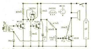
Fig. 1. The circuit diagram is drawn in the usual way, except that the transistor electrode connections are positioned so as to correspond with the transistor header. In this circuit the only transistor which requires special treatment is the 2N3702, which has its leads in a straight line with the collector in the middle.
