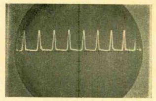
Fig. 5. Output palse waveform.  $x = 0.6 \mu s/div$ . y = 0.5 V/div.
