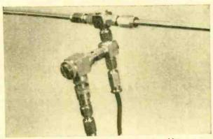
The transmitter, dipole aerial and light source assembly.
