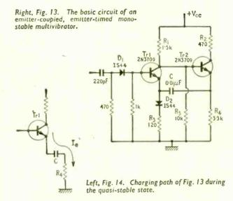
ensure that the transistor ratings are not exceeded. The following are some useful design equations; The pulse width is given by the approximate relationship
