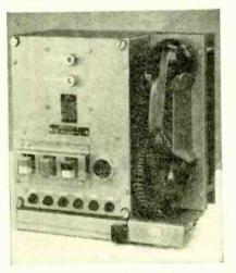
Drivers on the London Transport Victoria line and its Brixton extension will be able to communicate directly with other trains using a v.h.f. radio link. So far Nelson Tansley Ltd., 144 Holland Park Avenue, W.II, have received orders for about 170 communication systems as shown in the photograph. These, in addition to inter-train communications, offer passenger address and cab-to-cab intercom facilities.
