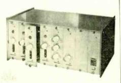
±12 dB at 100 Hz, gain control. Distortion is less than 1% for full output on 10 W, 25 W and 75 W models. Response for microphone is ±2 dB 50 Hz—10 kHz and music ±2 dB 40 Hz—12 kHz. Noise on microphone is better than 50 dB and on music it is better than 60 dB. The dimensions are standard free-standing unit 16½×7×10 in deep; rack mounting model 19×7×10 in deep. Associated Electronic Engineers Ltd., Dalston Gardens, Stanmore, Middlesex.
