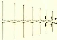
Schematic diagram of log-periodic dipole aerial showing the phasing.
