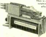
This is a 3000 type relay capable of latching in the energised position after the supply is removed until a suitable releasing current is applied in the opposite direction. This releasing current is controlled with a single coil, by reducing the operating current in reverse or with a double
