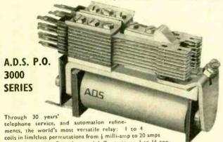
(0.1 to 400 volts); Fast, slow, and A.C. versions; I to 16 contact units (36 springs max.); Standard contacts 0.3 to 1 amp; Alternatives for switching Dry-state, Inductive, and 10 amp circuits. Insulation from 100 to 4,000 volts; Life up to 100 million operations; Plain or tropical finishes; Approx. dimen" sions 1 31" × 31" × 21" max. An A.D.S. 3000 Type to meet all specifications-G.P.O., E.I.D. C.E.G.B., ADMIRALTY, U.K.A.E.A., ALL COMMERCIAL, ETC.
