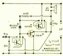
Fig. 5. Complementary a.f. amplifier. With sine-wave drive this delivers 60 mW to an  $8\Omega$  load. Speakers of any higher impedance may be connected.
