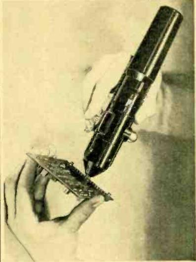
THE DIOTESTER detects faulty diodes and transistors when still in circuit without need for unsoldering.
