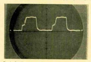
Fig. 4. Sampling gate waveform.  $x = 1 \mu s/div.$  y = 2 V/div.
