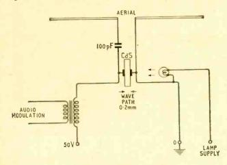
Fig. 2. Circuit of the v.h.f. transmitter, showing light control.
