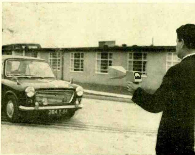
(left) Portable radar speedometer being used to measure the speed of a car. The battery-operated microwave Doppler radar set has a range of about 200 yards on a large vehicle.
