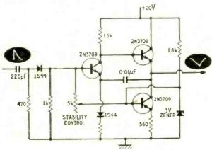
Fig. 20. A linear sawtooth generator circuit.
