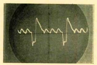
Fig. 3. Frequency divider waveform.  $x = 1 \mu s/div.$  y = 1 V/div.
