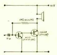
Fig. 4. Simple two-stage class A amplifier. The current drain is 8-35 mA, depending on the speaker impedance. A power output of about 10 mW is delivered to a load of  $20\text{-}40\,\Omega$  and loads up to  $200\,\Omega$  may be used without change of component ralues. For higher loads, or headphones, the bias resistor is 8.2 M $\Omega$ , and the current taken is 1.5 mA.
