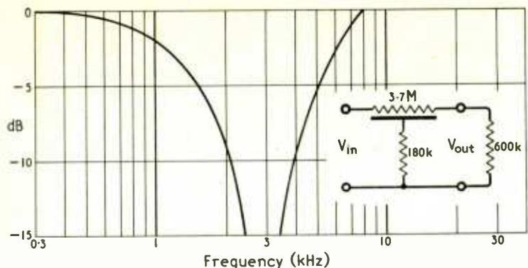
Fig. 3. Notch filter. A complete null is obtained only for one combination of frequency and earth-lead resistance.
