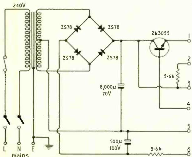
The circuit diagram of the module given in Fig. 2 shows a number of different supply rails which may be related to Fig. 1 as detailed below:
