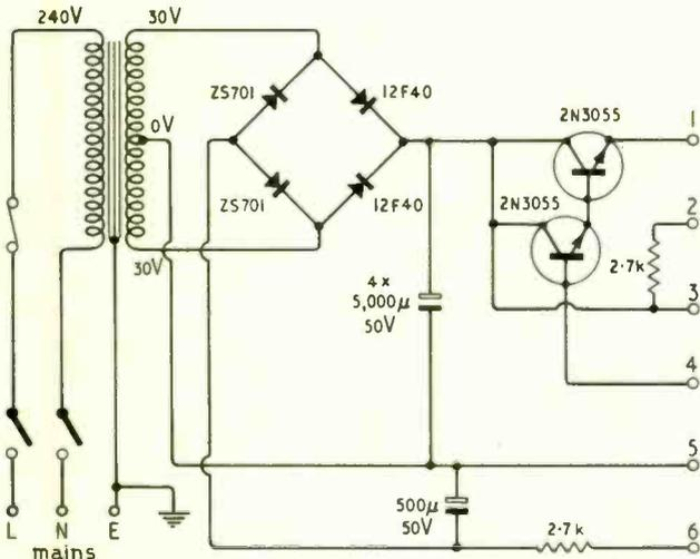
Fig. 4. Power supply giving an output of 24 V at 5 A. Output is taken from pins 1 and 5.
