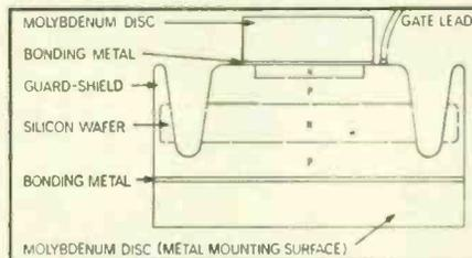
During manufacture, the silicon wafer for epitaxial thyristors is contoured to improve the high-voltage characteristics of the device. This illustration shows the cross-section of a typical contoured silicon wafer.
