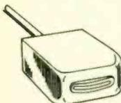
Built into a deep drawn mumetal case ensures complete shielding. Type T is the protruding pole type with special narrow track (as narrow as .002 in.) and can be made as a Record/Playback or Erase Head, or combined Record / Playback / Erase Head, or even Record/Playback and self-oscillatory Erase Head. The
