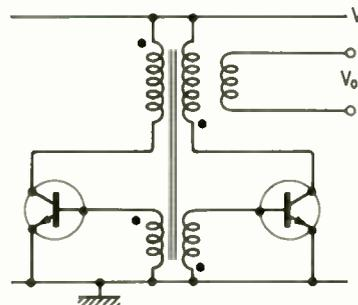
Fig. 8. Conventional single-transformer d.c. inverter circuit.
