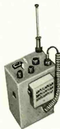
"Mariner", 6 Ch. VHF FM, RF Output power 1W, Portable Transceiver
