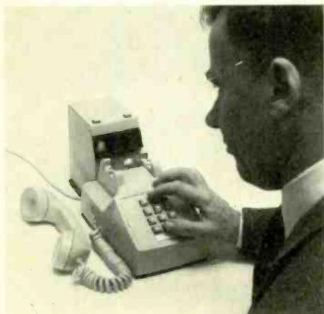
to display the 36 digits required and two small windows show that coding is in process and the end of word and end of sentence periods.
