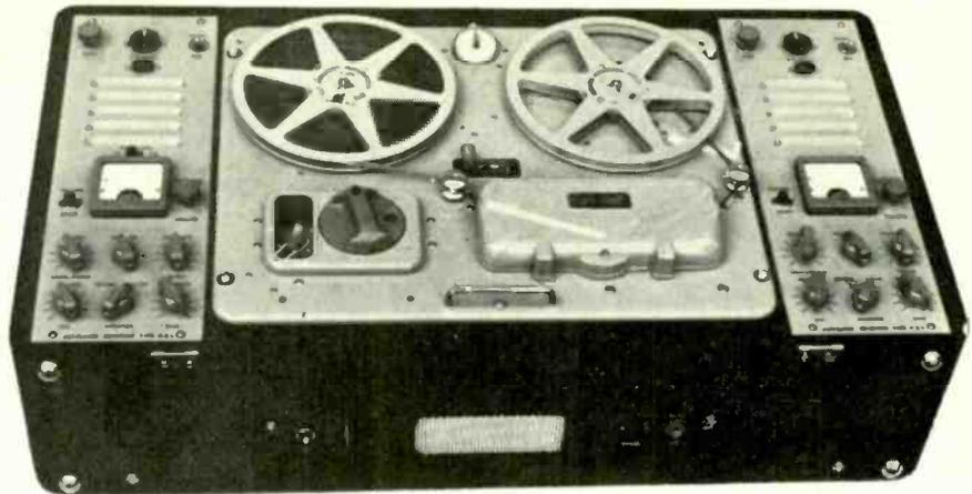
**W.V.B. TAPE RECORDER.** Similar to above but mono only. Professional quality recordings, checked by after record monitor during recording. Echo and superimpose facilities, 600 $\Omega$  balanced or unbalanced output and  $3\frac{1}{2}$  watts output to internal or external speaker.
