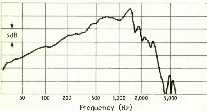
Fig. 5. Axial frequency characteristic of Bextrene cone from first mould, fitted with p.v.c. surround of shape shown in Fig. 4.
