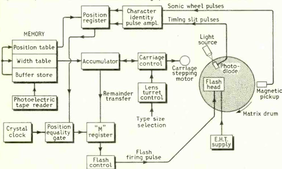
exposed on the film; its position has been determined only by its width and the widths of the characters preceding it in the line, and is thus typographically correct.
