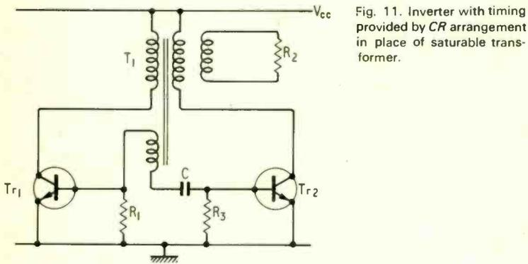
Fig. 11. Inverter with timing provided by CR arrangement in place of saturable transformer.
