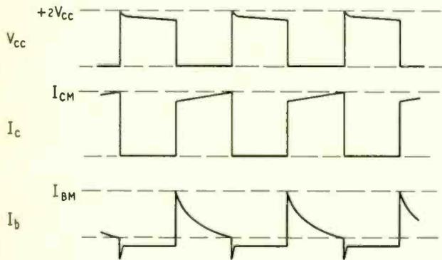
Fig. 12. Voltage and current waveforms in the inverter with CR timing.
