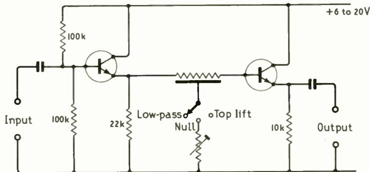
Fig. 5. Practical circuit giving low-pass, notch, and top-lift responses. Any good high-gain low level planar transistors (2N3707, BC109, BC168B, etc.) may be used.
