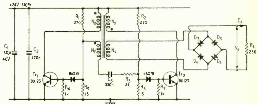
likely to occur when the base-emitter voltage is high. The reverse base-emitter voltage could be limited by a shunt diode placed across the base-emitter junction. The diode, however, would not eliminate the reverse base current. Series diodes are therefore used in each transistor base lead together with the shunt resistor to provide a path for leakage current.
