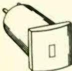
Size is  $\frac{7}{16}$  in. square at the front with body  $\frac{3}{8}$  in. dia. by  $\frac{3}{8}$  in. long. Curved front  $1\frac{1}{4}$  in. radius. This head is available in a wide range of Record/Playback impedances. Also available as Erase. This novel design possesses many advantages over comparable types—higher output—lower losses—extremely good H.F. response—very low noise pick up—has internal mumetal screen. Round body aids mounting arrangements—easy azimuth alignment.
