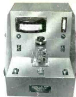
Incorporates many new features, including semi-automatic electrical timing, proportional temperature control, remote controlled specimen lowering system and a temperature meter calibrated to an accuracy of 0.25% full scale deflection at the test temperature.
