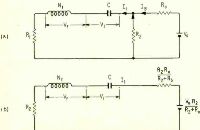
Fig. 8<sup>2</sup>. The transformer can either be of a non-saturable type, or of a saturable type. In the case of the non-saturable transformer circuit, a considerable variation of frequency with load will be experienced and the transformer size required to handle the same power will be three to four times as big as one using a saturable transformer. The circuit with single non-saturable transformer is therefore regarded as not suitable for practical purposes.
