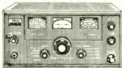
4 band receiver covering 550 Kc/s to 30 Mc/s. continuous and electrical band spread on 10, 15, 20, 40 and 80 metres. 8 valve plus 7 diode circuit. 4/8 ohm output and phone jack. 88B-CW • ANL • Variable BFO • 8 meter • Sep. band spread dial • 1F 455 Kc/s audio output 1.5 W • Variable RF and AF gain controls. 115/250 v. A.C. Mains. Beautifully designed. Size: 7 x 15 x 10in. With instruction manual and service data. £310/0. Carriage 12/6.
