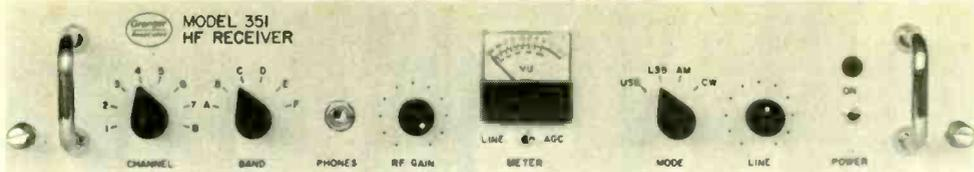
105 MHz) and an h.f. oscillator (range 4.65–43 MHz)—are used in a double frequency conversion that cancels out the drift of the v.h.f. oscillator. A fine frequency control is provided for each crystal. Frequency stability is  $\pm 20$  Hz up to 20 MHz, and 1 p.p.m. above 20 MHz.
