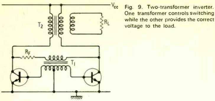
Fig. 9. Two-transformer inverter. One transformer controls switching while the other provides the correct voltage to the load.
