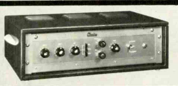
For mounting in Cabinet Rack or Console on 19" standard panels—finished gun, metal two tone blue or to requirements—Microphone, Tape, Gramophone, Radio and Priority Tone Signal Modules.
