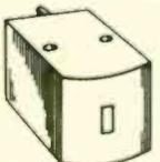
Exactly as Type R except body is  $\frac{7}{16}$  in. square along its length providing simple mounting arrangements. The Erase versions of R and DR types are double field heads. These are not just double gaps but two Erase heads in one, giving better than 60dB erasure of a saturation (+6dB on full record level), 1 k/c recording at  $3\frac{3}{8}$  l.p.s.
