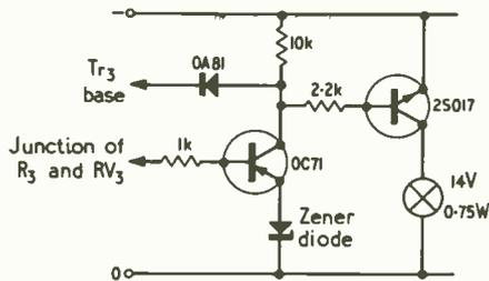
Mr. Hubbard's overload protection circuit
