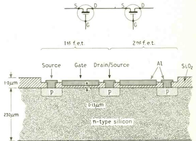
Fig. 1. Basic structure of a field-effect device in an m.o.s. integrated circuit (not to scale), showing how two of the devices can be easily connected in series by making one p-type region common to both.
