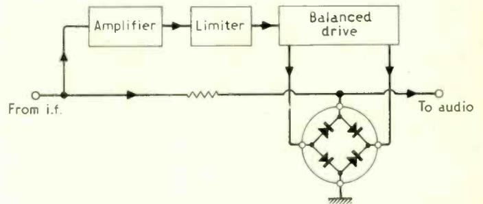
Fig. 6. Zero-crossing detection system.
