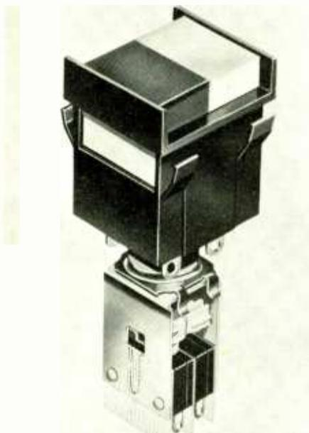
suitable for horizontal or vertical matrix mounting requiring individual rectangular holes 1.00 in. by 1.14 in. for single units and additional 1.250 in. per switch for matrix mounting. One- to four-pole momentary or maintained snap-on switch modules are available as standard, each pole being s.p.d.t. or two circuit. The basic two-circuit microswitches are rated at 10 A., 125/250 V a.c., 30 V d.c.
