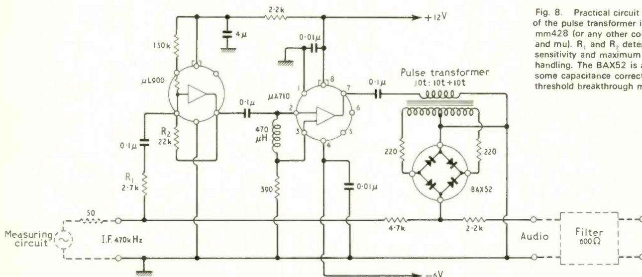
Fig. 8. Practical circuit for detector. The core of the pulse transformer is a Ferralex type mm428 (or any other core of similar size and  $\mu$ ).  $R_1$  and  $R_2$  determine threshold sensitivity and maximum linear signal handling. The BAX52 is a matched quad, but some capacitance correction for minimum threshold breakthrough may be necessary.
