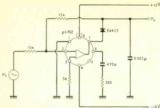
Fig. 3. Amplifier/diode envelope detector.
