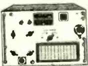
**COLLINS (U.S.A.) RECEIVER.** 7 valve super-heterodyne (411t Octal valves); exceptionally stable for 88B. Frequency coverage 1.5-12 Mc/s. Power required, 200 v. D.C. 80 mA. 12 v. A.C. 1.25A. Excellent condition. £12.
