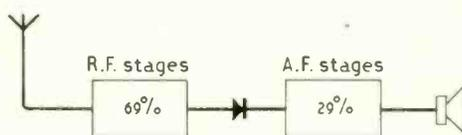
Fig. 1. Basic block schematic of a.m. broadcast receiver.
