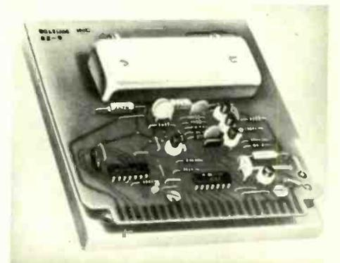
continuously. An address counter is not required or sequential write-in and readout of data, making the module suitable for c.r.t. display and offer memory applications. The memory has a maximum storage of capacity of 10,000 bits at a delay of 10 ms and a clock rate of 1 MHz.
