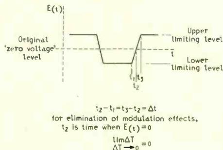
Fig. A. Condition for elimination of a.m. effects.
