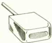
Built into a deep drawn mumetal case ensures complete shielding. Type T is the protruding pole type with special narrow track (as narrow as .002in.) and can be made as a Record/Playback or Erase Head, or combined Record / Playback / Erase Head, or even Record/Playback and self-oscillatory Erase Head. The Erase track can be made wider than the R/P track on the Combo Head, a fully screened lead is incorporated as part of the head.
