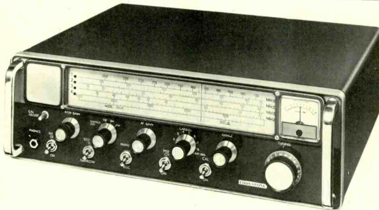
The '990R' when used in conjunction with the matching '990S' provides continuous AM/FM coverage from 27 to 870MHz. A common Panoramic Display Unit is available for use with both receivers.
