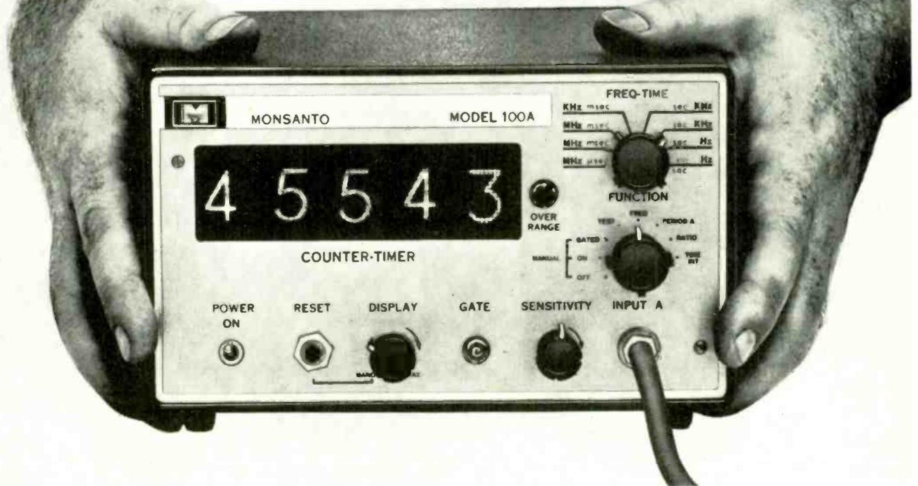
Integrated circuit construction plus completely original design concepts, result in high-quality 12.5 MHz counter/timer performance at remarkably low cost
