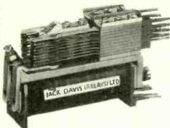
Twin coils and armatures.
