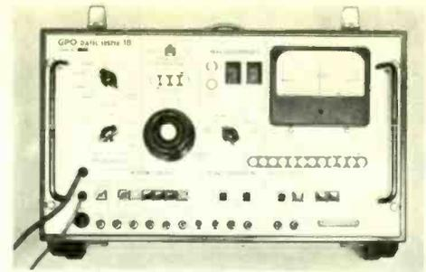
error. These are totaled and the stored count displayed up to a maximum of 2,047 counts. The error counter may be switched to display element counts or 511-bit pseudo random blocks in error. Trend Electronics Ltd, St. John's Works, Tylers Green, Nr. High Wycombe, Bucks.
