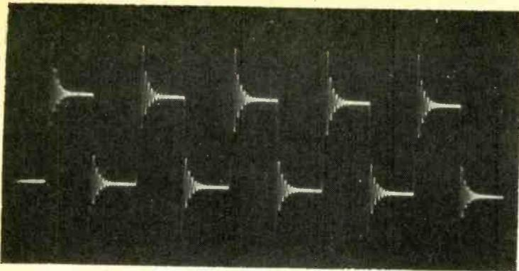
Fig. 12. Square-wave response, 10kHz and 0.1- $\mu$ F load.
