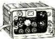
Oscillator Test No. 2. A high quality precision instrument made for the Ministry by Airmeq. Frequency coverage 20-80 Mc/s. AM/CW/FM. Incorporates precision dial, level meter, precision attenuator 1µV-100mV. Operation from 12 volt D.C. or 0/110/200/250 v. A.C. Size 12 x 8 1/2 x 9 in. Supplied in brand new condition complete with all connectors, fully tested, £45. Carr. 20/-.
