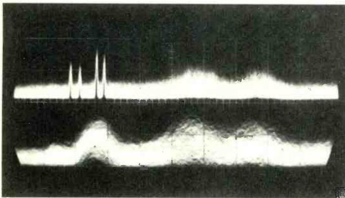
*Fig. 4. With and without pulse compression; the upper pair are of a snowstorm approaching a group of targets and the lower pair taken 10 minutes later, are with the storm over the same area as the target. (Crown copyright).*
