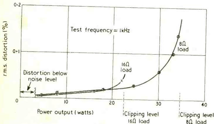
Fig. 7. Variation of distortion with output power level.
