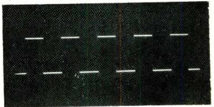
Fig. 11. Square-wave response, 50kHz and 8-ohm load.
