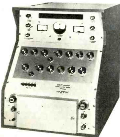
tact resistance. No critical resistors are used. Internal power supplies provide currents of one and two amperes respectively, and an external power supply delivering up to 100A is provided. Claude Lyons Ltd., Instruments Division, Hoddesdon, Hertfordshire. WW 303 for further details
