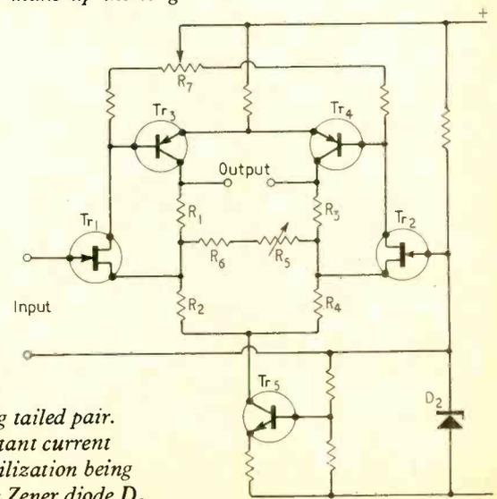
Fig. 2 The long tailed pair.  $Tr_5$  forms a constant current source, base stabilization being performed by the Zener diode  $D_2$ .
