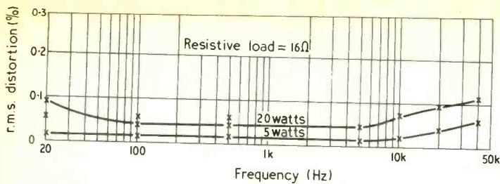
Fig. 5. Distortion characteristics of amplifier with 16-ohm load.
