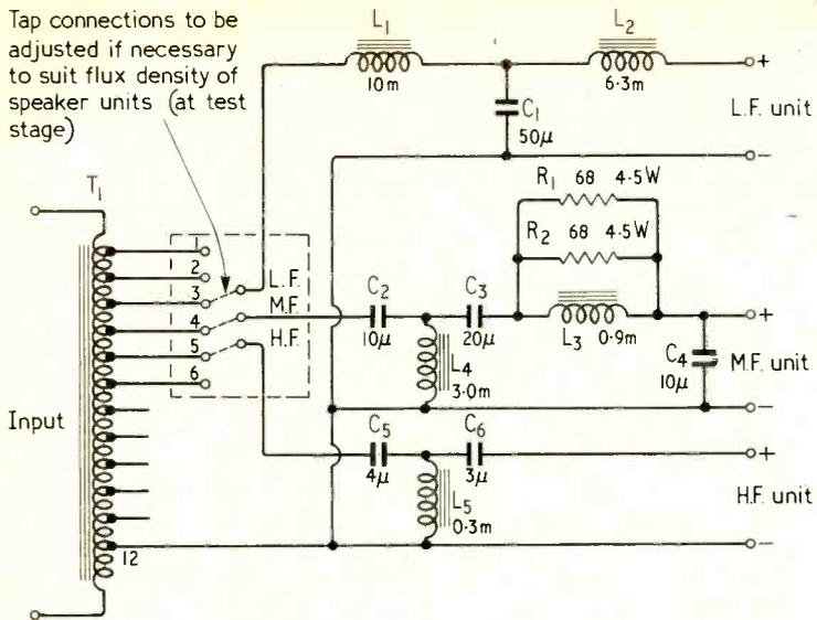
Fig. 30. (Left) Circuit diagram of crossover network of LS5/5 and LS5/6 loudspeakers. All component values are  $\pm 2\%$ .
