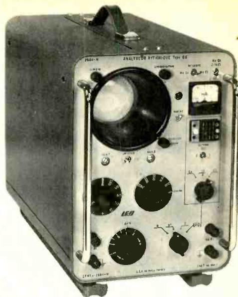
Instrument for measuring distortion on telegraph circuits, including a signal generator for signal speeds of 50-2400 bands (Laboratoire Electro-Acoustique of Paris).
