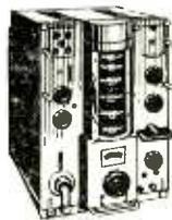
Just released by the Ministry. High quality 10 valve receiver manufactured by Murphy. Coverage in 5 bands 520 Kc/s-30 Mc/s. I.F. 500/Kc/s. Incorporates a R.F. and 3 I.F. stages, bandpass filter, noise limiter, crystal controlled 400 Kc/s. B.F.O. calibrator, I.F. output, etc. Built-in speaker, output for phones. Operation 150/230 volt A.C. Size 19 1/2" x 10 1/2" x 10 1/2".
