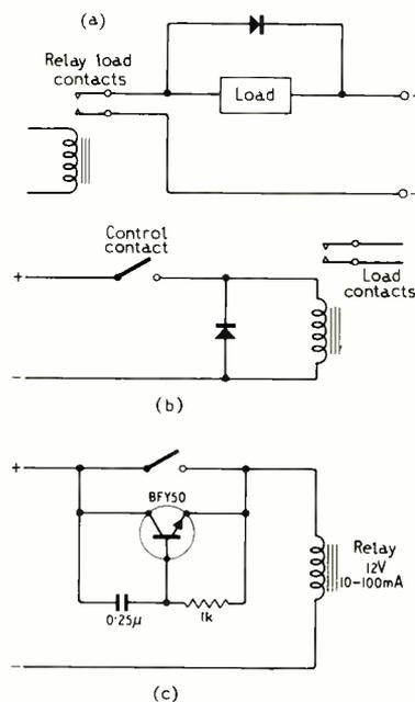
Fig. 1. Relay switching transient suppression circuits: (a) Load contacts—diode across load. (b) Diode protecting drive coil control switch. (c) Transistor spike suppressor.
