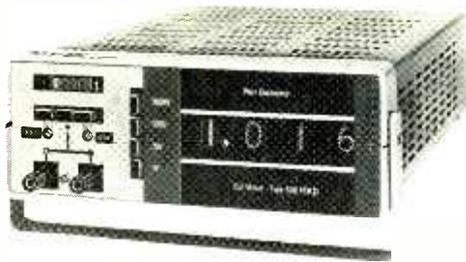
to 1100 on all ranges. Four ranges are incorporated from  $\pm 1$  V to  $\pm 1000$  V d.c., the input resistance is  $> 10$  M $\Omega$  ( $> 1$  M $\Omega$  on the 1 V range). An internal calibration standard has an accuracy of  $\pm 0.001\%$ /year. The price is £120. Weir Electronics Ltd, Durban Road, Bognor Regis, Sussex.
