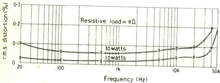
Fig. 6. Distortion characteristics of amplifier with 8-ohm load.
