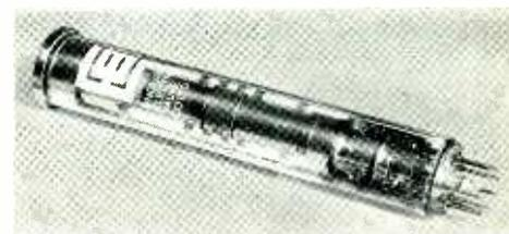
ciated with magnetic focusing, thus making this type vidicon suitable for multi-tube colour cameras. A uniform "beam landing" characteristic provides good signals from the whole picture area. An example of the tubes in this range is the 8134VB which has a high blue sensitivity intended to overcome the difficulties normally associated with tungsten filament lighting.
