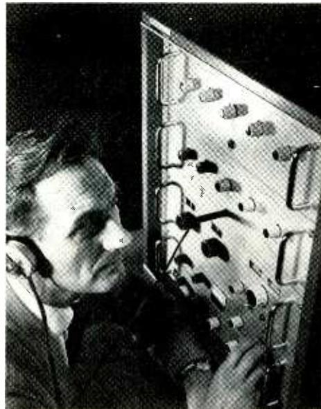
independent sideband facilities handling two separate channels, will cost approximately £3,500. Other standard versions cost less. The receiver covers the 1.5 to 30MHz band in four ranges. Tuning is by decade switches followed by a continuously variable final tuning control. A sophisticated a.f.c. system locks on to signals drifting up to  $\pm 250\text{Hz}$ . A.g.c. circuits operate over a 90dB variation of signal strength, controlling the output to within 6dB.
