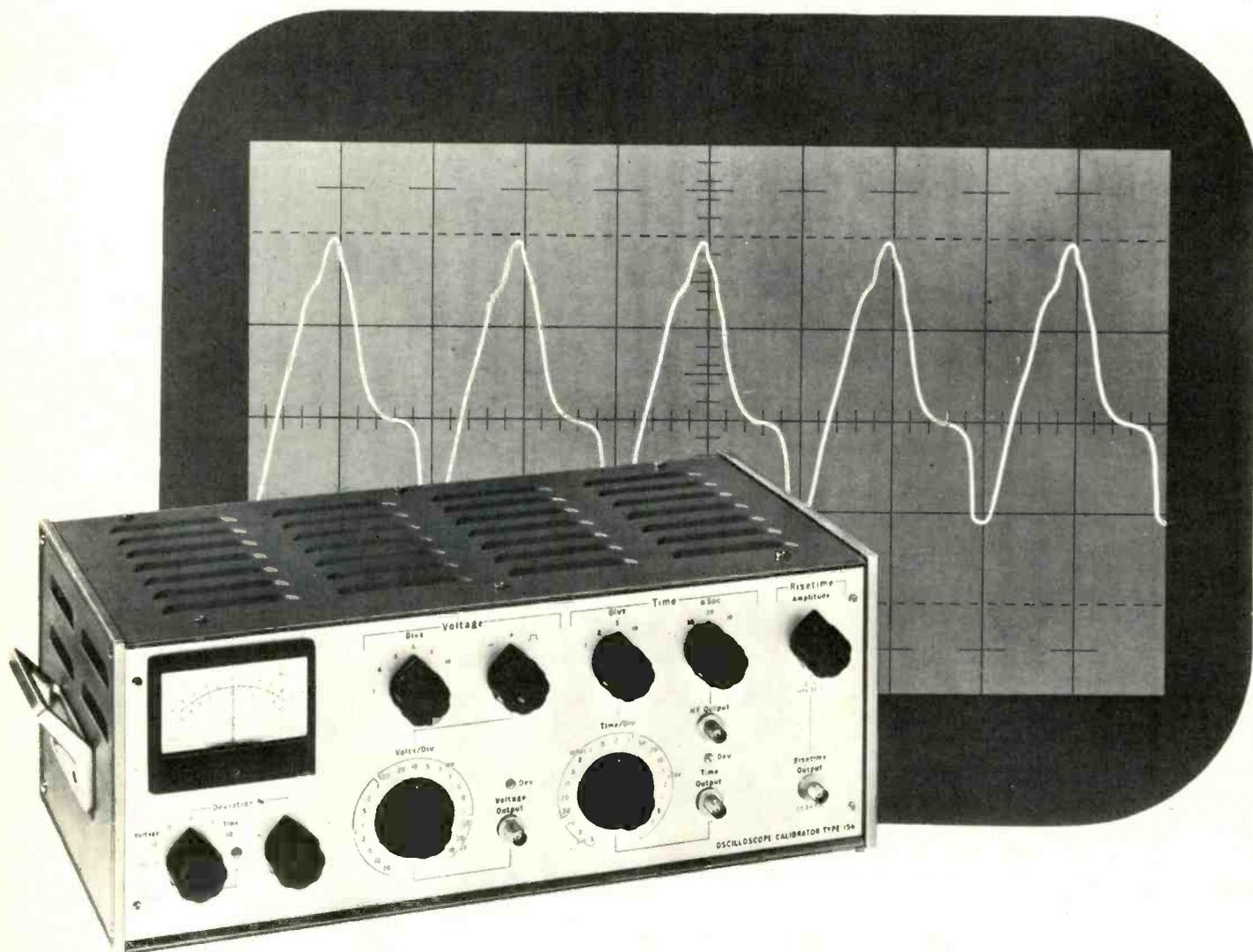
A new instrument, the BRADLEY Oscilloscope Calibrator 156 provides all the facilities required for the calibration of modern precision oscilloscopes. Simple to use, it is designed to calibrate vertical amplitude and sweep speeds, and to check risetime. A unique feature is the direct reading of percentage deviation from true values.
