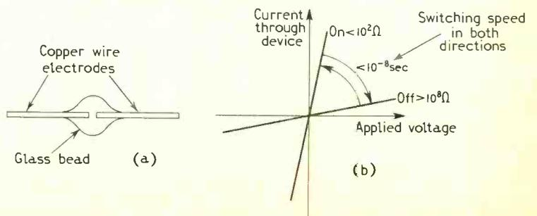
a critical value, typically 20V, and switching from the "on" to the "off" state is effected by a step-edged pulse from a low impedance source. Switching speed was given as being better than  $10^{-8}$  second in both directions. In its application as a memory element, the device will retain information indefinitely under open-circuit, short-circuit or load conditions.
