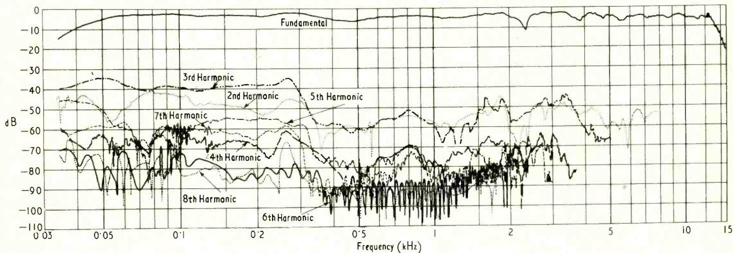
Fig. 32. (Below) Harmonic distortion of LS5/5 loudspeaker measured at 1 N/m<sup>2</sup> at 1.5m.
