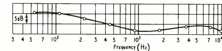
Fig. 28. (Left) Mean spherical response of LS5/5 loudspeaker measured in octave bands.
