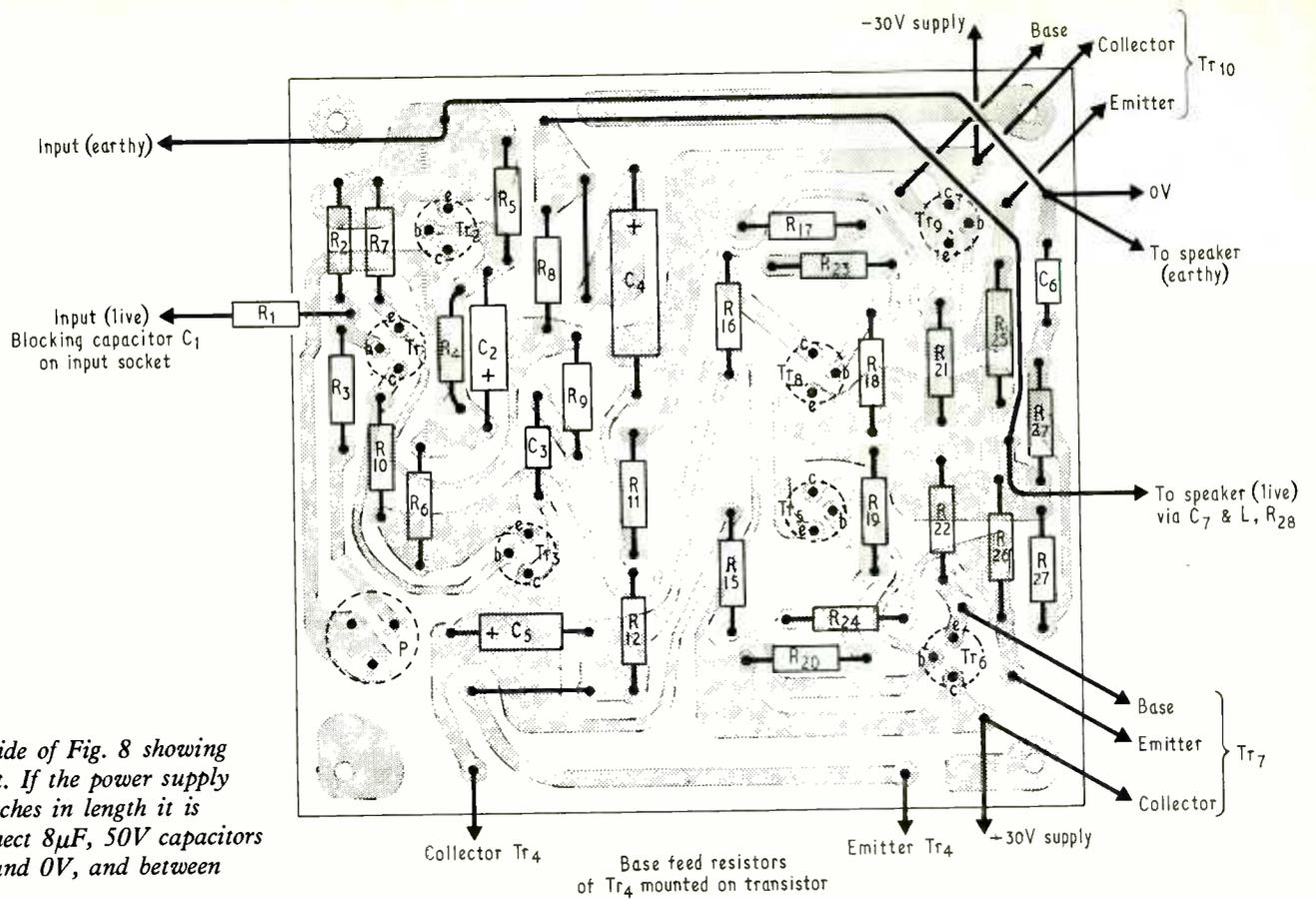
Fig. 9. Reverse side of Fig. 8 showing component layout. If the power supply leads exceed 6 inches in length it is advisable to connect  $8\mu\text{F}$ , 50V capacitors between +30V and 0V, and between -30V and 0V.
