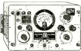
High quality 17 range instrument which measures A.C. and D.C. Voltage, Current, Resistance and Power output. Ranges D.C. volts 250mV-10,000 v. (10 megohm input). D.C. current 10µA-25 amps. Ohms: 0-1,000 megohm. A.C. volt 10mV-250 v. (with R.F. measuring head up to 250 Mc/s). Current 10µA-25 amps. Power output 500 micro-watts-5 watts. Operation 0/110/200/250 v. C. Supplied in perfect condition complete with circuit lead and R.F. probe £25. Carr. 15/-.
