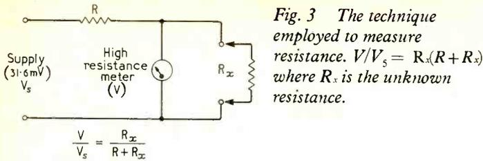
Fig. 3 The technique employed to measure resistance.  $V/V_s = R_x/(R + R_x)$  where  $R_x$  is the unknown resistance.
