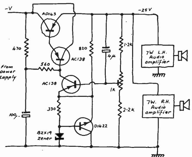
Fig. 4. Voltage stabilization circuit used in H.M.V. stereo radiograms. A 15-volt source for the varicap tuner is provided from the junction of the  $820\Omega$  resistor and the emitter of the D1422 transistor.
