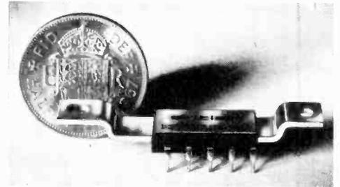
Sinclair IC-10 monolithic integrated circuit power- and pre-amplifier in dual-in-line package measuring 2.5 × 1 × 0.5cm. Output of 5W r.m.s. (continuous) is claimed. Price: £2 19s 6d.
