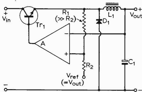
Fig. 7. Basic principle of self-oscillating switching d.c. voltage regulator using monolithic i.c.
