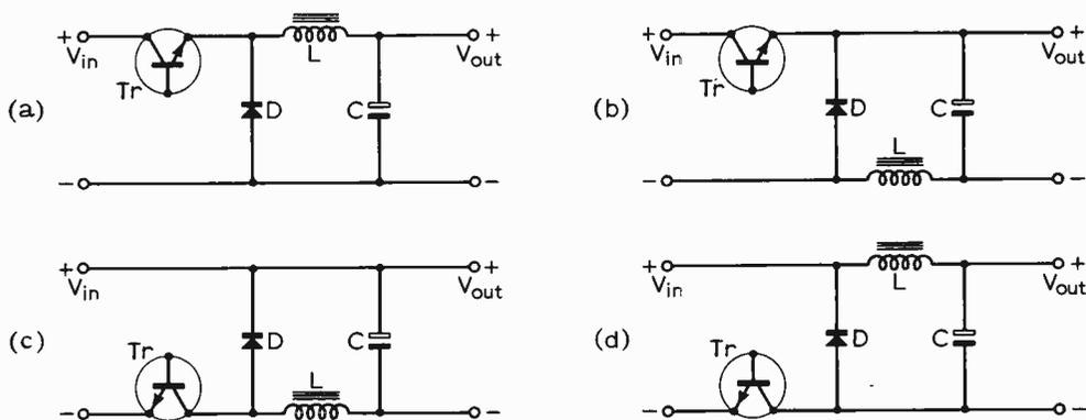
Fig. 2. Types of filters used after series switching transistor in switched d.c. voltage regulators: (a) In emitter circuit with choke in positive lead; (b) as (a) but with choke in negative lead; (c) in collector circuit with choke in negative lead; (d) as (c) but with choke in positive lead.
