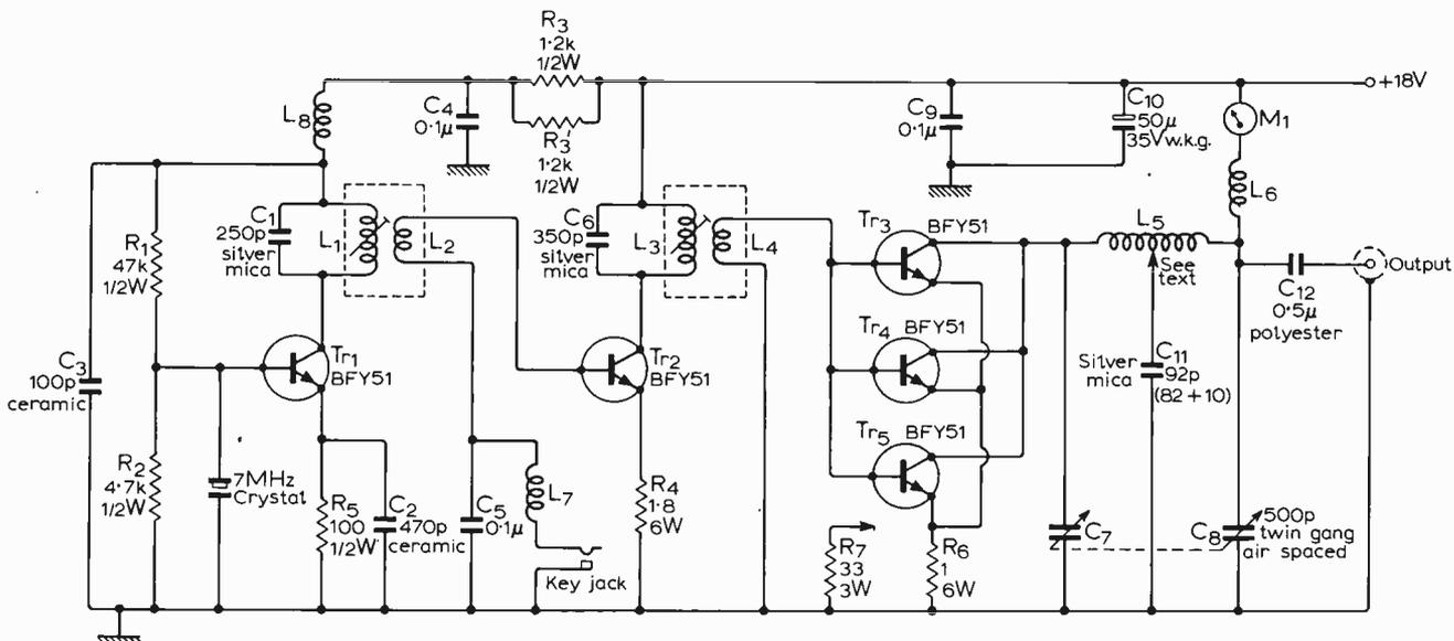
with keying ("chirp") is obviated. The filter,  $L_7 C_5$ , prevents r.f. from appearing on the key leads.
