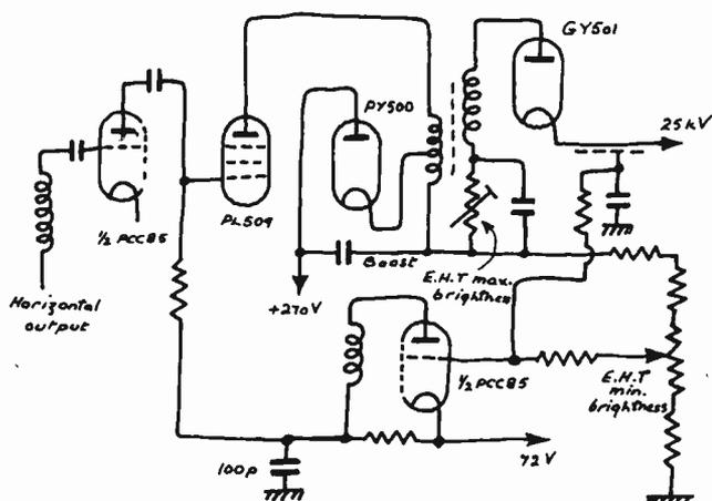
Fig. 1. Simplified circuit diagram of the e.h.t. generator employed in the Bang & Olufsen single-standard colour tv receiver, Beovision 3000.
