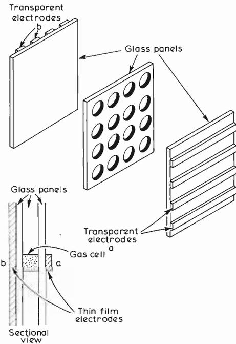
Fig. 5 Plasma display panel. A rectangular array of gas cells with external X and Y addressing electrodes.
