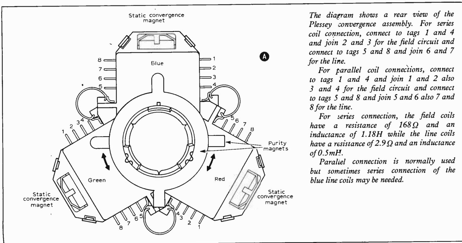
The diagram shows a rear view of the Plessey convergence assembly. For series coil connection, connect to tags 1 and 4 and join 2 and 3 for the field circuit and connect to tags 5 and 8 and join 6 and 7 for the line.
