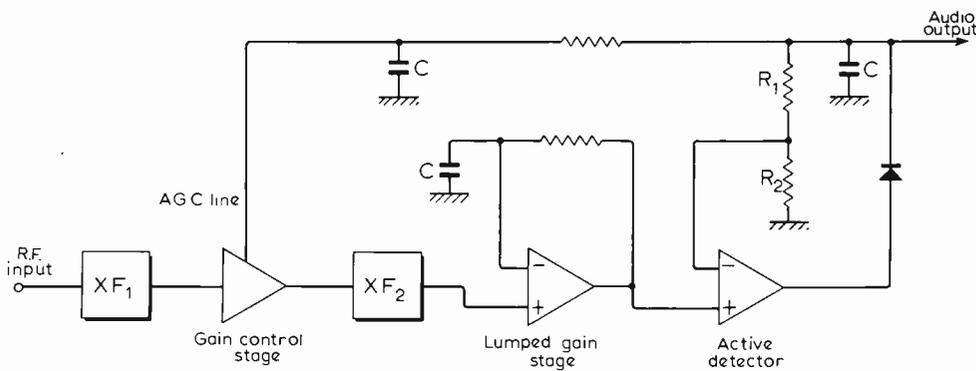
Fig. 2 Block diagram of the LM172—a complete a.g.c. stage, i.f. amplifier and a.m. detector. The capacitors and ceramic filters ( $XF_1$ ,  $XF_2$ ) are external to the chip.
