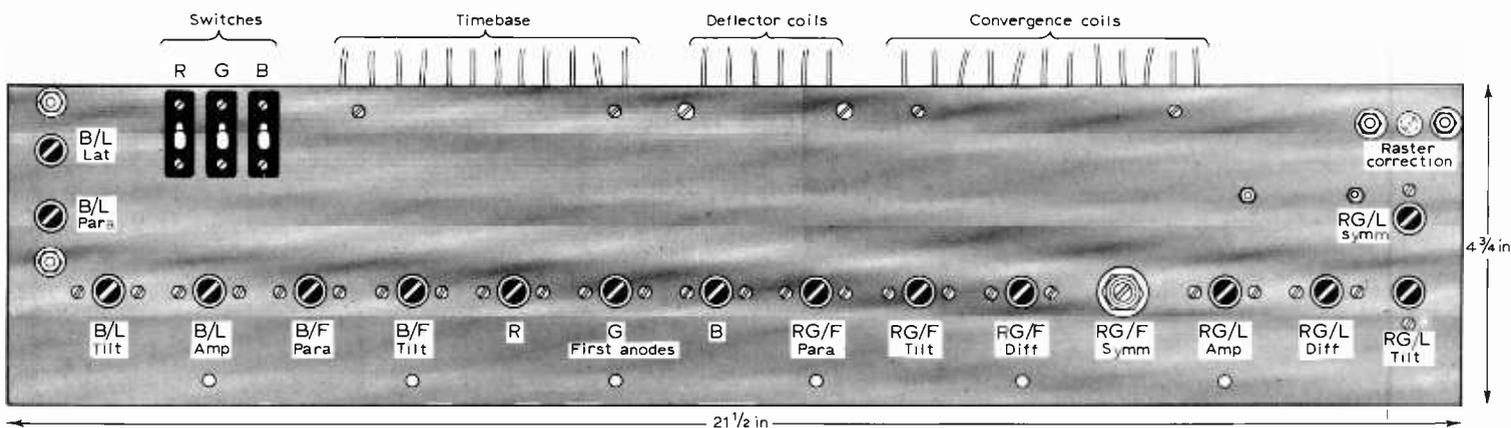
This photograph shows the underside of the convergence panel and indicates the positions of some of the chief components. The layout is far from critical.
