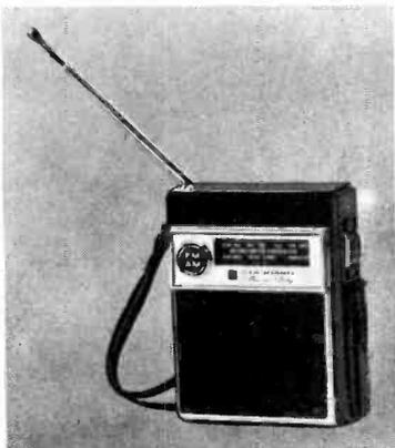
**Standard model SR-K466F** a.m./f.m. pocket radio receiver employing 11 transistors, and featuring a.f.c. on f.m. Output 200mW; speaker 4.5cm diameter. Power source: three mercury batteries. Dimensions: 79 x 62 x 31mm. Price: 23gn.
