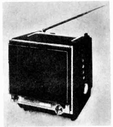
*KB model CK 400 colour TV receiver employing 48cm type tube. Hybrid chassis featuring manual tint control. Removable decoder board. Solenoid-operated system switch. Solid state e.h.t. unit. Price: 275gn.*
