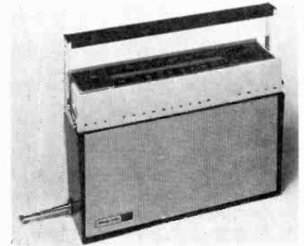
**Philco-Ford model T993** portable radio receiver covering medium-wave and v.h.f. Ten transistors and eight diodes employed. Features include a.f.c. on v.h.f. Price: 14gn.
