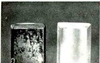
A section of a typical cast solder bar. Note the surface dross and general contamination.
