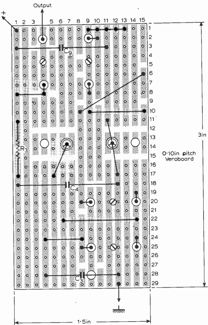
Fig. 7 Underside of the Vero circuit board.
