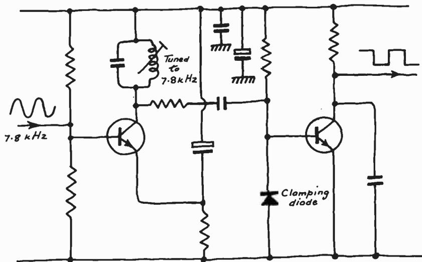
Fig. 2. An outline of the 7.8kHz switching wave generator employed in the Baird colour television model 718.
