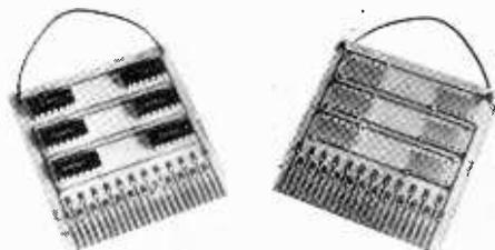
glass laminate with printed power supply tracks to each i.c. It is fitted with 24 input/output edge-connector terminations at 2.54mm (0.1in) pitch and provision is made for the attachment of a nylon cord loop to assist card removal. Size of the card is 68mm (2.7in) square and the price is 7s. 6d. Cards are also available as part of the components for a complete 6-way mounting framework. A.P.T. Electronic Industries Ltd., Chertsey Road, Byfleet, Surrey.
