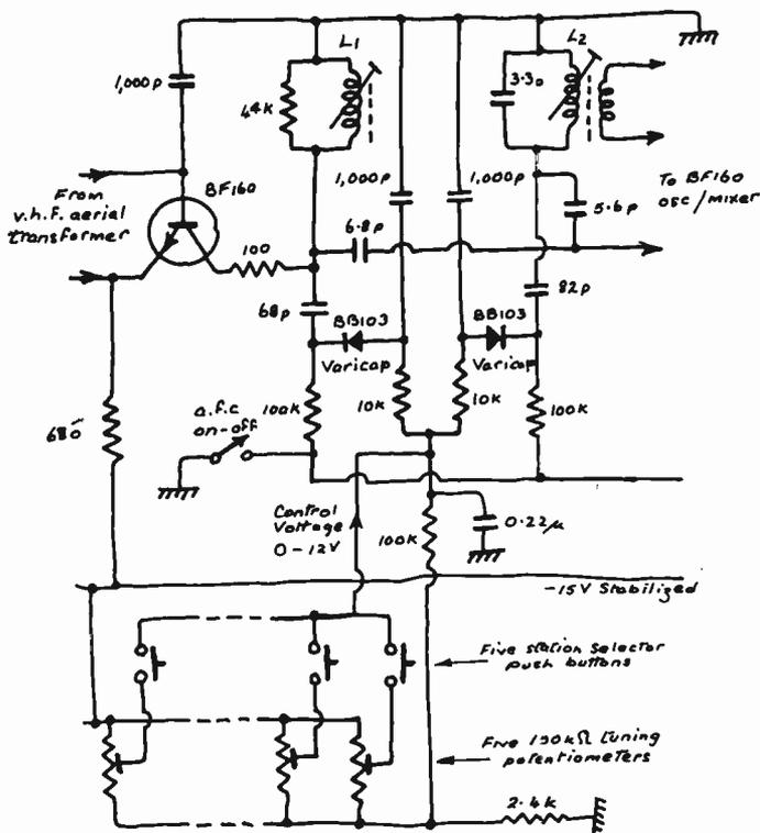
Fig. 5. Section of v.h.f./f.m. tuner in British Radio Corporation stereo radiograms, showing use of varicap diodes for tuning between the r.f. amplifier and the mixer/oscillator.
