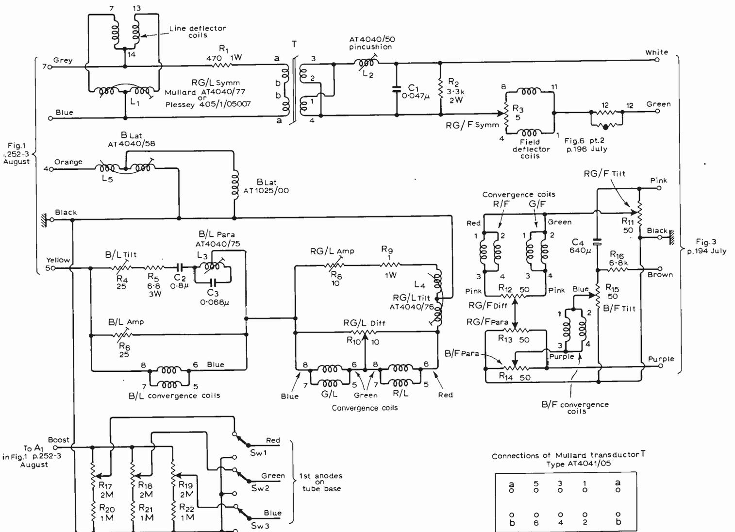
Fig. 1. Complete circuit diagram of the convergence unit. The switches employed are Rendar Instruments miniature slide type, model R 53005 (Electroniques stock number 168F27391D). They are d.p.d.t. switches, but only one pole in each is used.
