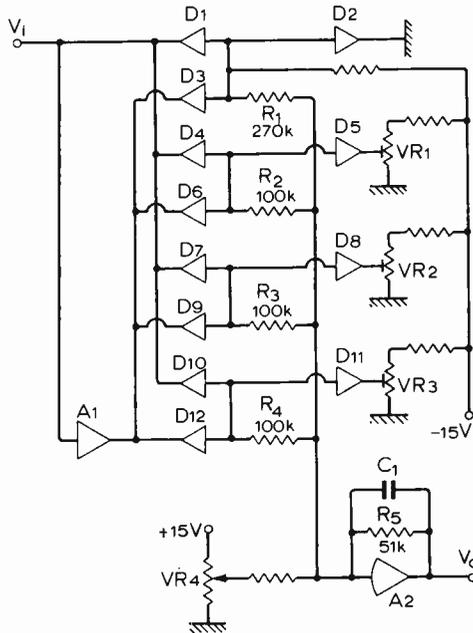
goes through  $D_{3,6,9,12}$ . The break point voltages are fed through diodes  $D_{2,5,8,11}$ , which provide compensation for the effect of temperature on the diode forward-conduction voltage, as pointed out by A. E. Crump. This balancing out of the voltages also means that the break-points can be set up by connecting an accurate voltmeter, most conveniently a digital type, to the sliders of the potentiometers, and adjusting these to the calculated break point voltages.
