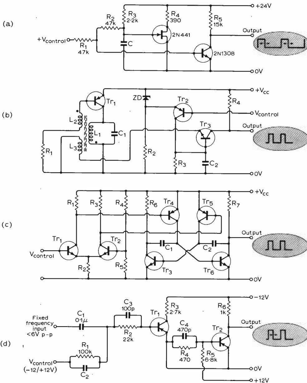
Fig. 3. Examples of constant-frequency pulse generators with mark-space ratio controlled by d.c. signal (a) Unijunction oscillator; (b) LC oscillator with output modulator transistor; (c) Astable multivibrator with long-tail control pair; (d) Schmitt trigger control with fixed frequency input.
