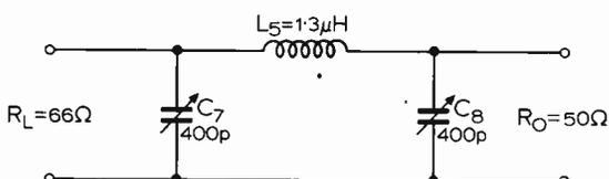
Fig. 3 Single  $\pi$ -network circuit.
