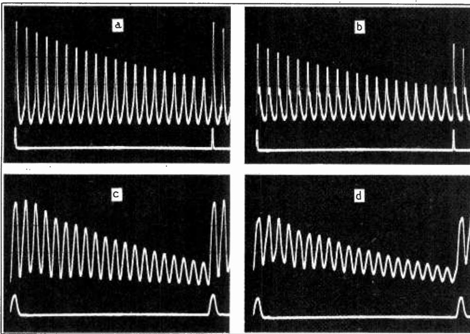
Fig. 2. Oscillograms from the double-beam c.r.o. (Fig. 1). Each shows the initiating pulse on the lower trace and the train of pulses resulting from recirculation on the upper trace.
