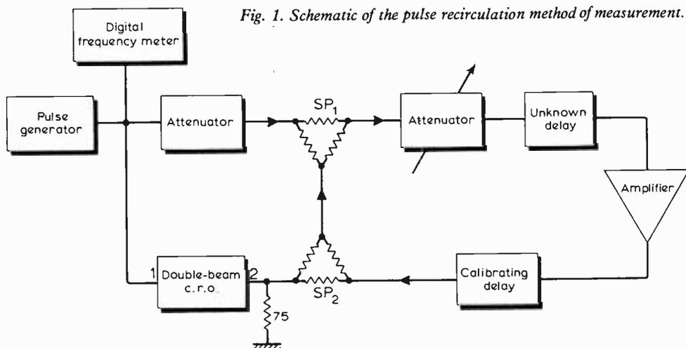
Fig. 1. Schematic of the pulse recirculation method of measurement.
