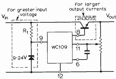
Fig. 4 Additional external components for increasing regulation range of WC109 device.
