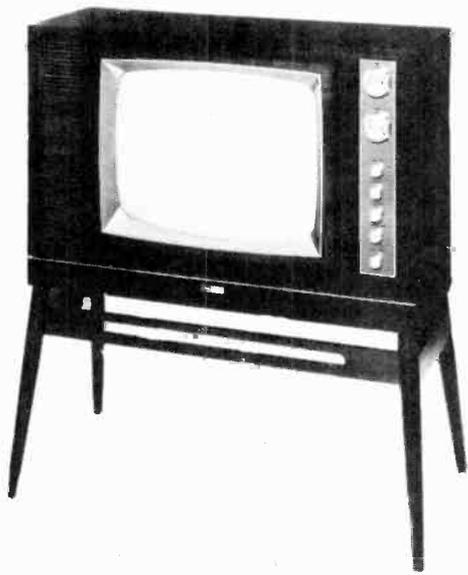
*Pye model 63 monochrome TV receiver with 51cm "squared" tube. Incorporates the 368 series hybrid chassis featuring solenoid-operated system switch. Forward facing 20 x 13cm loudspeaker. Price: £83.*
