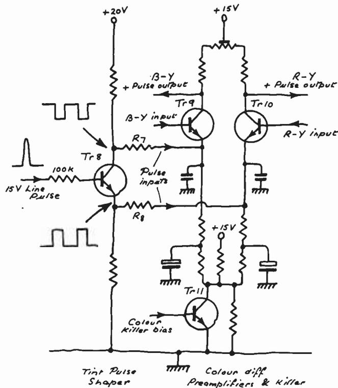
Fig. 3. Circuit diagram of part of the ITT/KB colour decoder panel showing the principle of operation of the automatic reference white correction circuit.
