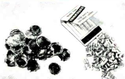
Solder chips which are usually made by dripping solder alloy on to a metal surface.
