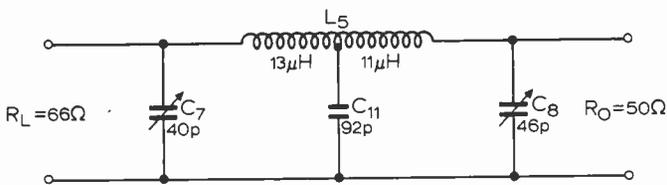
Fig. 5 Double π-network circuit.
