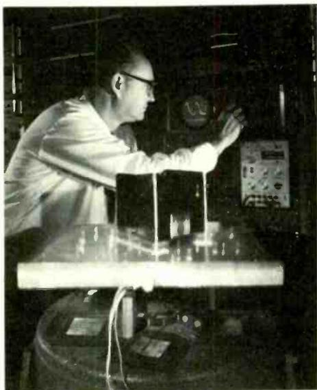
Showing the loose article detector in operation.
