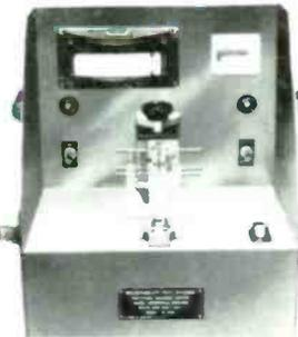
Incorporates many new features, including semi-automatic electrical timing, proportional temperature control, remote controlled specimen lowering system and a temperature meter calibrated to an accuracy of 0.25% full scale deflection at the test temperature. The machine can reduce production costs by instantly checking the solderability of components with wire terminations.
