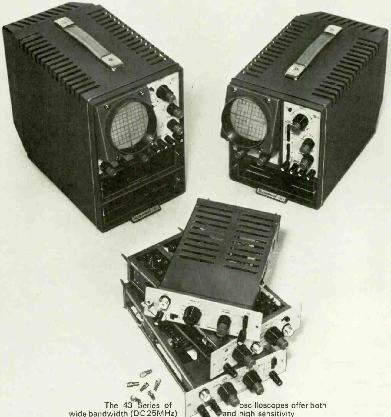
The 43 Series of oscilloscopes offer both wide bandwidth (DC 25MHz) and high sensitivity (100 $\mu$ V/cm) for general oscilloscope applications.
