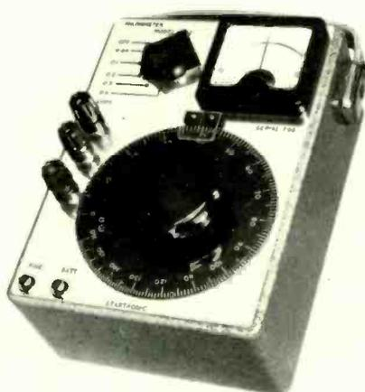
9-V dry battery, or any externally applied potential not exceeding 500V d.c. The BR1 is fitted with an isolating transformer enabling it to be used with a wide range of signal generators for measurements at frequencies other than 1kHz. Advance Electronics Ltd., Roebuck Road, Hainault, Essex.
