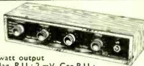
**SPECIFICATION:** Sensitivities for 10 watt output at 1 KHz. Tape Head: 3mV (at 3 1/2 i.p.s.). Mag. P.U.: 2 mV. Cer.P.U.: 80 mV. Radio: 100mV. Aux. 100 mV. Tape/Rec. Output: 100 mV. Equalisation for each input is correct to within ± 2dB (R.I.A.A.) from 20 Hz to 20KHz. Tone Control Range: Bass ± 13 dB at 60 Hz. Treble ± 14 dB at 15 KHz. Total Distortion: (for 10 watt output) < 1.5%. Signal Noise: < -60dB. AC Mains 200-250V. Size 12 1/2" long, 4 1/2" deep, 2 1/2" high. Teak finished case.
