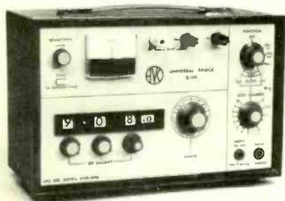
An inductance adaptor, type A151, is available to allow iron-clad inductors to be measured directly on the bridge with varying d.c. bias current and at different a.c. signals superimposed via the bridge. Avo Ltd., Avocet House, Dover, Kent.
