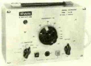
A general purpose, mains operated, solid state frequency generator with a frequency range of less than 1 Hz to 150 KHz in six switched ranges. Maximum output voltage is 2.2V r.m.s. into 600 ohms. Protection is by an internal 60mA fuse. On the front are a frequency range switch, ON/OFF output control, sweep frequency control with a large clear scale, 4 mm output sockets and a three-way socket to supply a separate 1/2 watt amplifier/loudspeaker (E.A.34 below).
