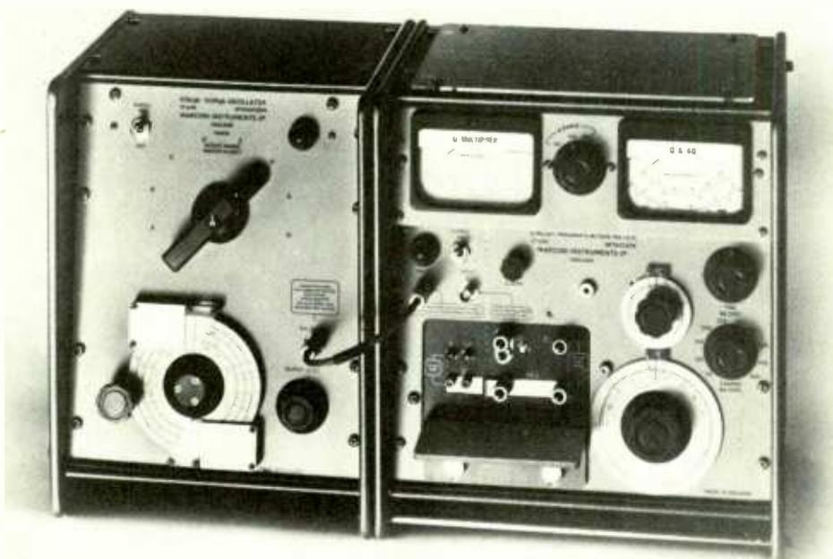
The new Marconi TF 1245A gives *gilt-edged* confidence in Q-measurement! By *gold-plating* the complete test-circuit and tuning capacitor, Marconi have cut inherent loss, increased long-term stability – factors which have always reduced the certainty of Q-measurement, especially at high frequencies.
