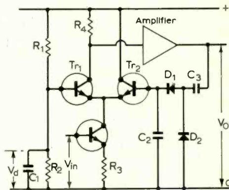
Fig. 11. Automatic gain control.
