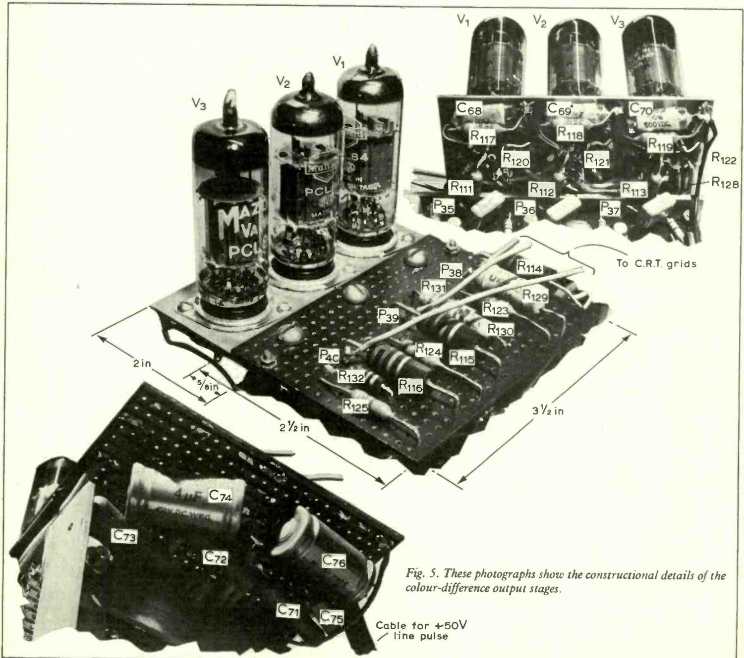
Fig. 5. These photographs show the constructional details of the colour-difference output stages.
