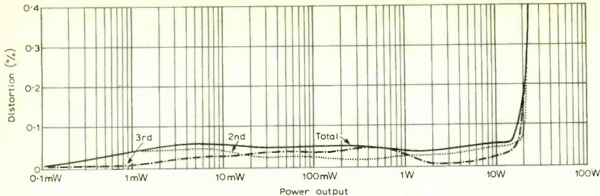
Fig. 5. Distortion characteristics of modified amplifier at 20mA quiescent current.
