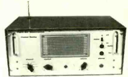
Details of a.g.c. performance state that for a change of input from  $2\mu\text{V}$  to 200mV it will produce a change of output not greater than 3dB with reference to 1W. Operation is from a.c. mains 100-115V and 200-250V. Size is 407  $\times$  305  $\times$  178mm. A number of optional extras are available including interchangeable block filters for changing channel spacing. Park Air Electronics Ltd., Red Lion Square, Stamford, Lincs.
