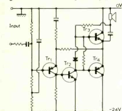
Fig. 2. Amplifier re-designed for common positive earth line
