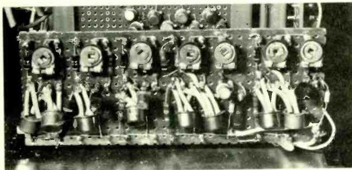
Fig. 20. A completed dian. Sharp-eyed readers may notice that one of the transistors has been substituted for a different type. This was only because we ran out of stock of the specified type.
