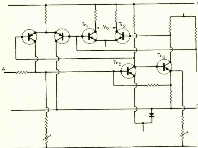
Fig. 9. Adding negative feedback to the multiplier circuit.
