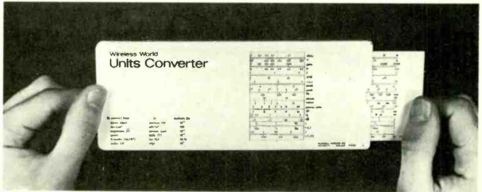
The units converter in use. The conversion scales are engraved on the slider and are read through a window carrying a "cursor" line.
