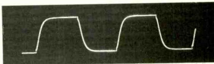
Fig. 3. Response to 1 kHz square-wave with 40,000 pF capacitor
