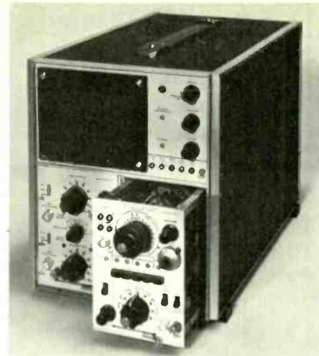
a 10-turn calibrated potentiometer to provide the delay of 0.2  $\mu$ s to 2s. Timebase B, with 18 calibrated sweep speeds from 100ms/cm to 0.2  $\mu$ s/cm provides the sweep in the delay mode. The gate and ramp waveforms from timebases A and B are available at sockets on the front panel. A x5 magnifier expands the sweep length to effectively five screen diameters and provides a maximum sweep speed of 40ns/cm. Advance Electronics Ltd., Roebuck Road, Hainault, Essex.
