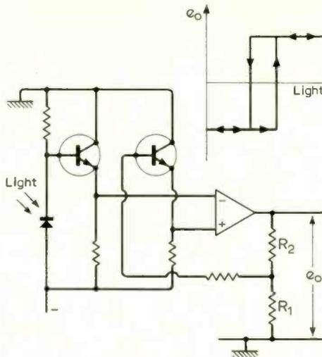
saturation. If the light intensity is reduced a regenerative action returns the amplifier to its negative saturation value. The circuit exhibits hysteresis.
