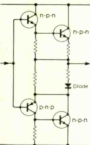
Fig. 2. Modified quasi-complementary output stage.
