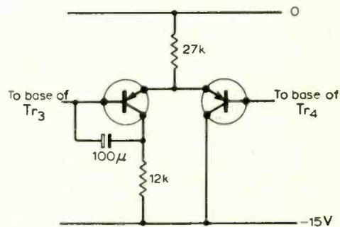
Fig. 13. Amplifier to reduce effect of rectifier ripple in Fig. 11.
