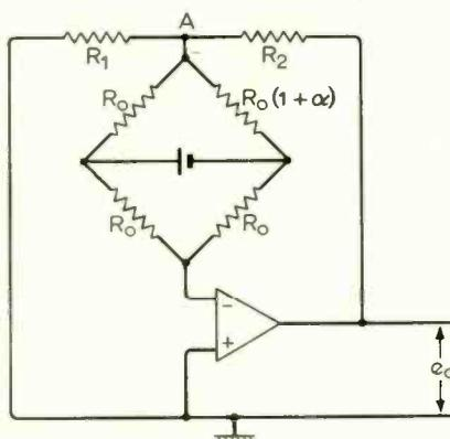
The feedback circuit forces the amplifier to develop a voltage at the point A which is equal and opposite to the unbalance voltage developed across the bridge. The bridge unbalance voltage is
