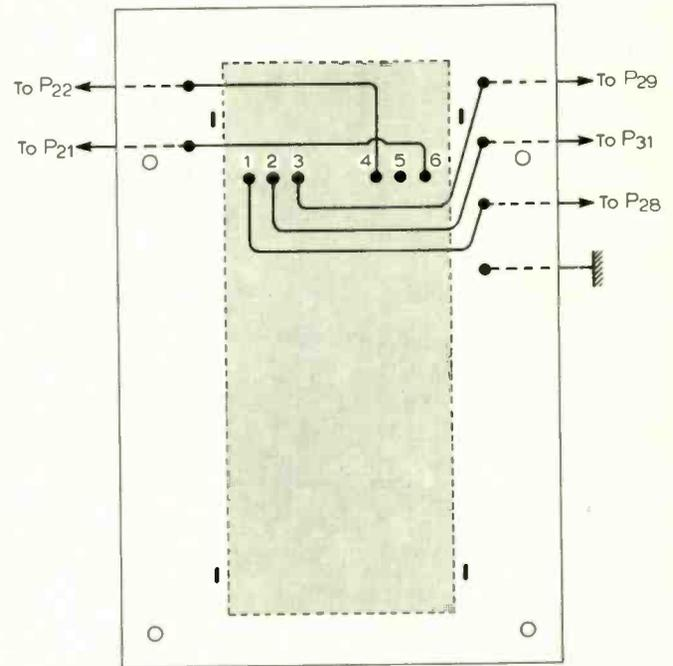
Fig. 3. Details of the delay-line mounting board are given here, viewed from the rear. This is for the original model of the Mullard delay line.
