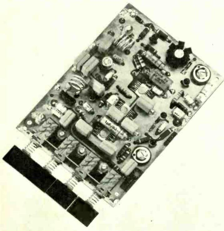
Fig. 4. Completed prototype of the f.m. tuner
