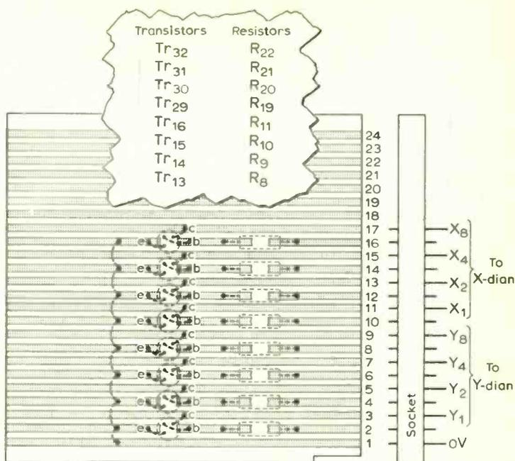
Fig. 23. Construction of board 1 containing the buffer amplifiers. The vacant space will be used for other components later on in the construction.
