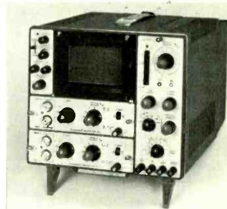
more than a minute; and as a storage oscilloscope capable of storing traces for periods of up to ten minutes. Variable sweep delay is also provided and a choice of plug-in Y amplifiers is available. Display area is 6 x 10cm and 22 calibrated sweep speeds range from 5s to 0.5 $\mu$ s/cm. Telequipment Ltd., 313 Chase Road, Southgate, London N.14.
