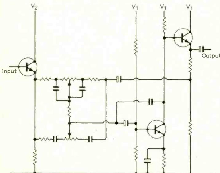
Fig. 5. Tone control stage of Leak 'Stereo 30 Plus'.
