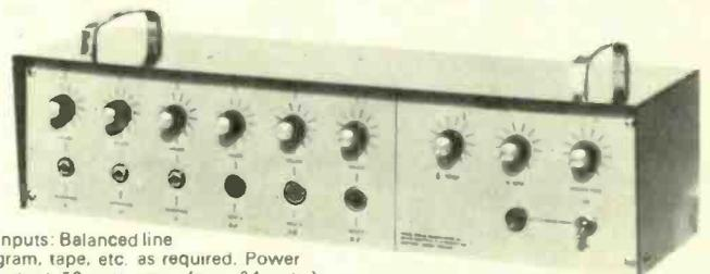
Inputs: Balanced line gram, tape, etc. as required. Power output: 50 watts r.m.s. (max. 64 watts). Output impedance and voltage: 15 ohms (other taps available), 156 ohms C.T. giving 50-0-50 volts or 100 volts. Harmonic distortion: Approx 1% at full power. Frequency response: plus or minus 2dB 20 c/s (Hz) to 35 Kc/s (KHz). Weight 38lb. Models available: M50/4, M50/6, M50/8 (suffix refers to channels)
