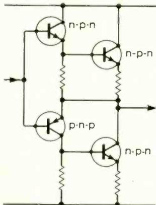
Fig. 1. Typical quasi-complementary output stage.
