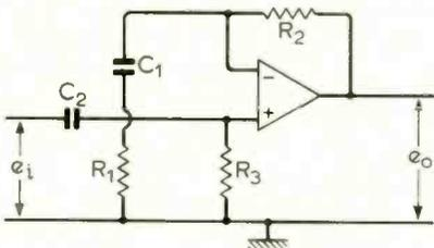
Basically the follower with gain with the addition of blocking capacitors and the d.c. bias path  $R_3$ . The gain of the amplifier is  $(1 + R_2/R_1)$  with low frequency 3 dB frequency determined by the shorter of the two time constants  $C_1R_1, C_2R_3$ . The input resistance is  $R_3$ .
