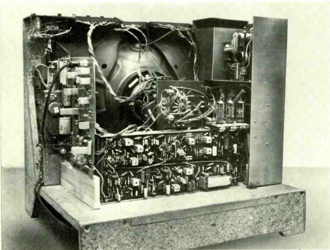
*Rear view of the complete receiver with the complete decoder in its closed position at the rear.*
