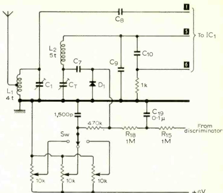
Fig. 5. Modifications to the circuit to allow electronic tuning to be used
