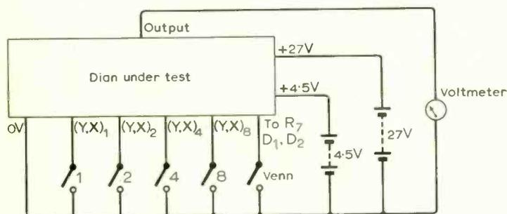
Fig. 21. A dian test circuit.
