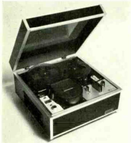
claim to make the bandwidth 50% wider than a normal v.t.r. Tape width is 12.7mm and its length 915m. Speed is 240mm/s. Two video heads are used and horizontal resolution is 350 lines for black and white; 250 lines for colour. The recorder measures 480 x 480 x 250mm and weighs 25kg. Victor Company of Japan Ltd., 12,3-chome, Moriyacho, Kanagawa-ku, Yokohama, 221, Japan.
