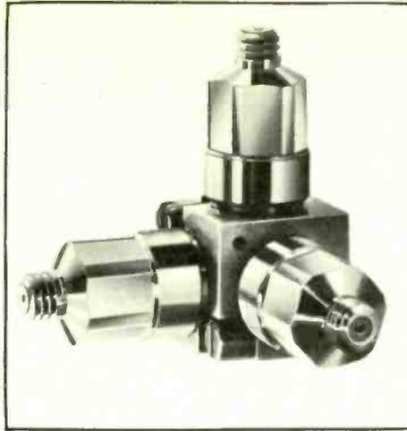
to 20,000g in three axes can be measured. Kistler Instruments Ltd., The Ridges, 2 Clockhouse Road, Farnborough, Hampshire.
