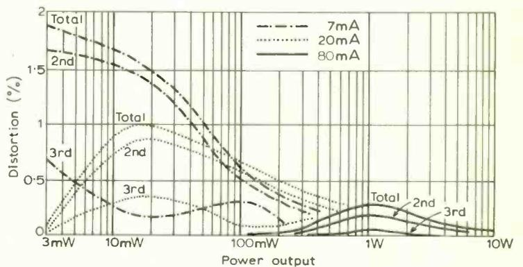
Fig. 3. Distortion characteristics of conventional amplifier with 7mA, 20mA, and 80mA quiescent current.
