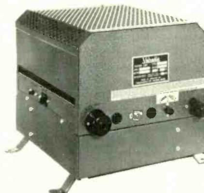
units working from any input voltage and providing a variety of output voltages. The conversion principle is static and noiseless in operation. Frequency stability is claimed to be better than  $\pm 1\%$ . The two types available are FCA230/100W at £32.6s.9d. (£32.34) and FCB230/200W at £52. Special units providing 400-1000Hz for testing marine and aircraft equipment can be supplied to order. Valradio Ltd., Browell's Lane, Feltham, Middx.
