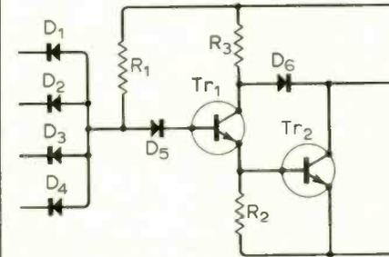
Fig. 28. Circuit of a Micronor-2 NAND gate.
