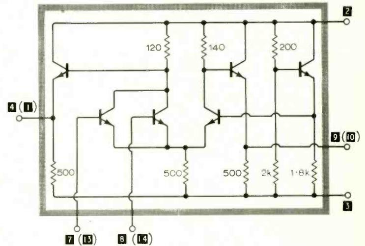
Fig. 2. Circuit of the type E3016 i.c. used in the i.f. section of the tuner
