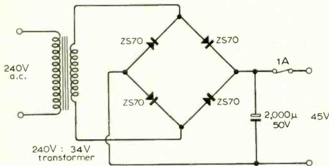
Fig. 6. Simple power supply used with amplifier.
