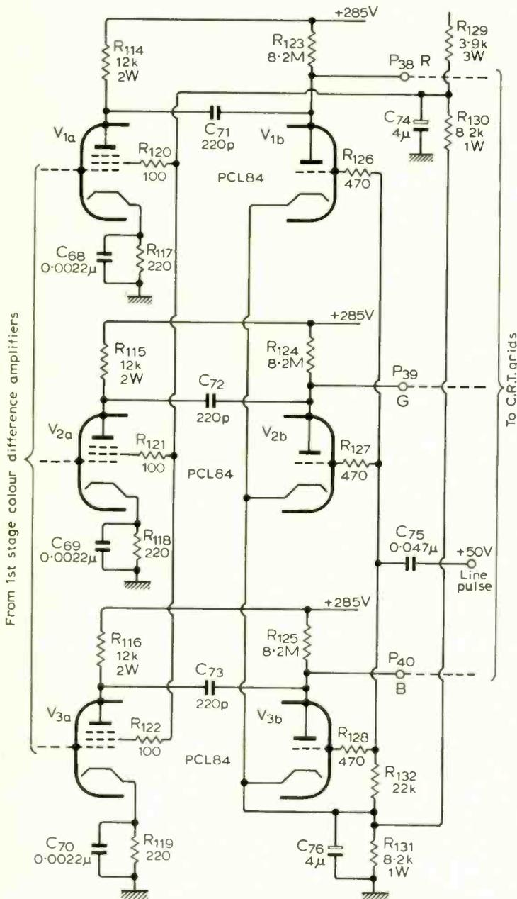
Fig. 1. Circuit diagram of the output stages of the colour-difference video amplifiers and black-level clamps.
