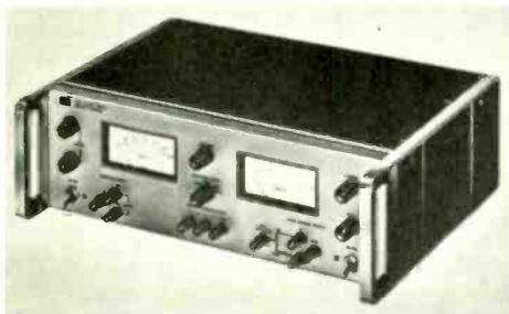
10A max. The output voltage changes less than 0.1% +5mV with a change from no load to full load and the transient recovery time is such that the output returns to within 25mV of the selected voltage within 50 $\mu$ s of the step change from no load to full load or vice versa. Dimensions: 16 x 42 x 33mm. Weight: 10kg. Price: £240. Hewlett-Packard Ltd., 224 Bath Road, Slough, Bucks.
