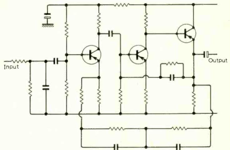
Fig. 2. Input stage of Radford SCA-30.
