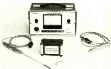
recorder operation. Supplied with the magnetometer is a calibration magnet and two Hall probes; one for transverse field and the other for axial field measurement. Accuracy is quoted as  $\pm 2\%$ . The unit measures 229 x 152 x 127mm and weighs 1.95kg. Price £98. Scientifica & Cook Electronics Ltd., 40-48 High Street, Acton, London W.3.
