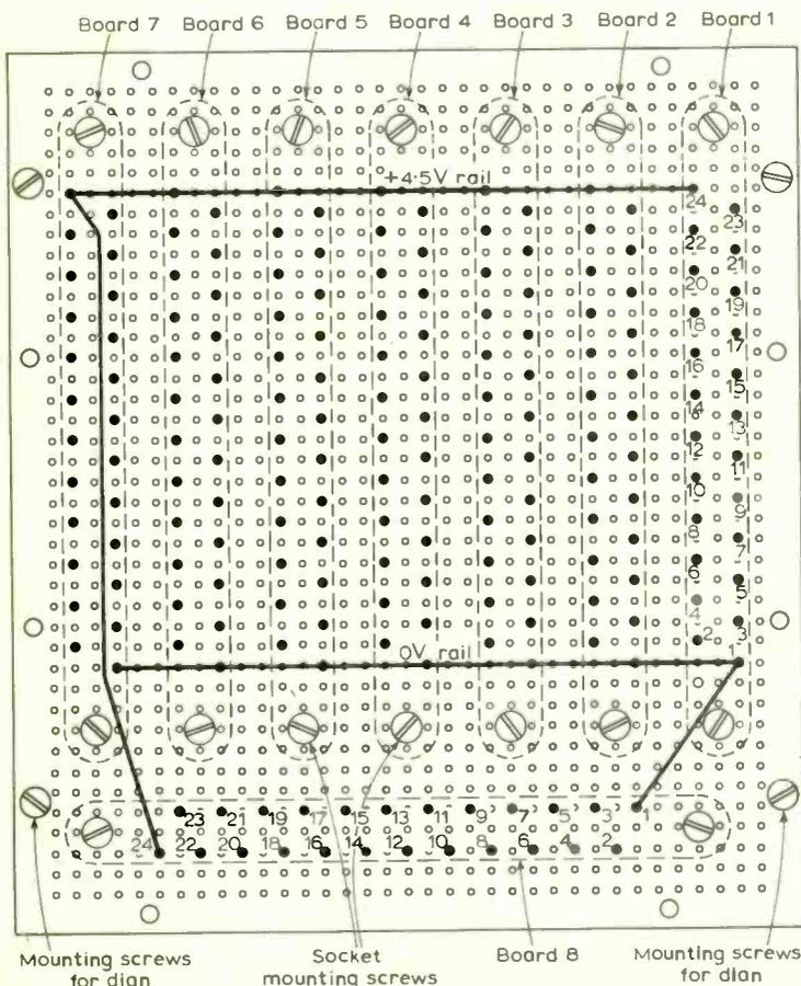
Fig. 22. The layout of the circuit board sockets in the main logic unit.
