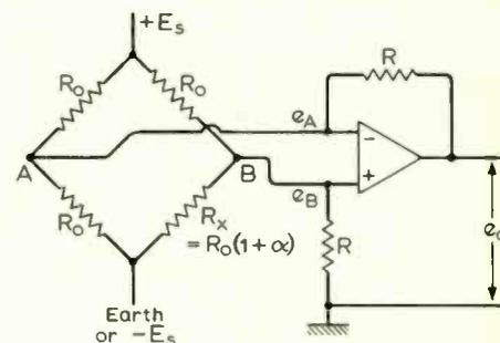
Feedback maintains the opposing corners of the bridge at equal potential; the amplifier output voltage establishes the differential current needed to balance the bridge. Using a single supply with the lower end of the bridge earthed:
