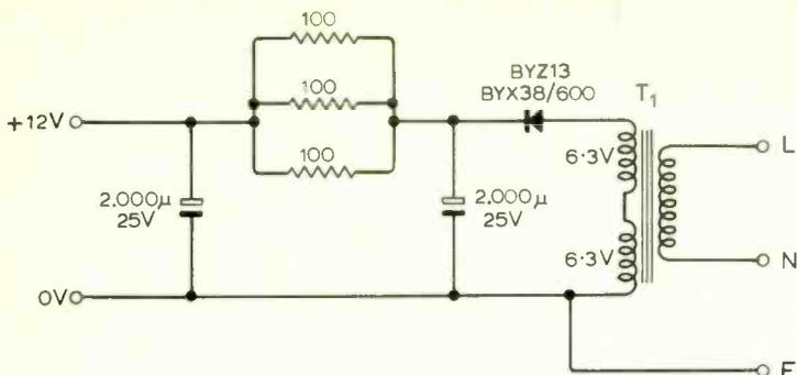
Fig. 6. A suitable power supply for the tuner.  $T_1$  is a Radiospares Ltd "Hygrade" filament transformer
