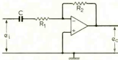
The basic inverter amplifier with capacitor C in series with the input. The gain of the amplifier is  $R_2/R_1$  with the low frequency 3 dB fall in gain occurring at a frequency  $1/(2\pi CR_1)$ . The upper frequency limit of the amplifier will be dependent on the loop gain and the compensated open-loop frequency response (see March article). The input resistance is  $R_1$ .
