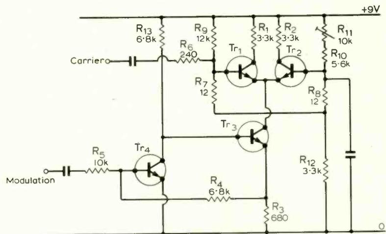
Fig. 5. Circuit to give up to 100% modulation.
