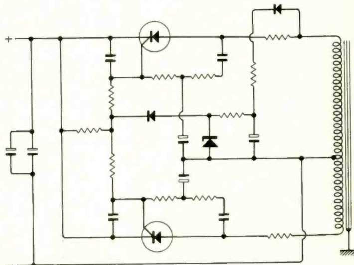
Fig. 7. One half of the power supply in the Radford SCA-30.
