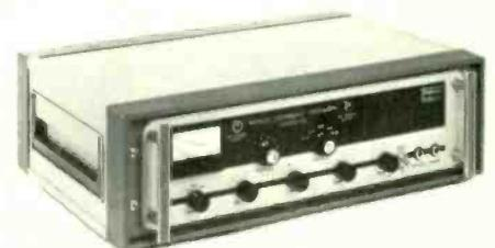
failure is automatic. Any aerial with a 75  $\Omega$  transmission line may be employed with the receiver or a long wire in conjunction with an aerial tuning unit. A socket is provided for the connection of headphones or an external loudspeaker. When this facility is in use the internal loudspeaker is muted. A second socket terminated at 600  $\Omega$  allows an a.f. signal to be fed to external equipment such as an amplifier or teleprinter. Price £190. Labgear Ltd., Cromwell Road, Cambridge.
