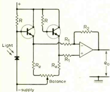
general purpose op. amp. is normally not high enough to allow it to be connected directly to this circuit. A transistor capable of operating at low currents and acting as an emitter follower can be used to increase the input resistance. A balanced input stage is used to reduce temperature drift. The gain of the amplifier is set by the choice of  $R_2/R_1$ .
