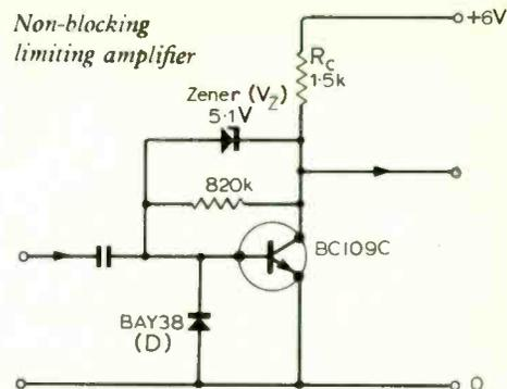
the current from the signal source exceeds a value of about  $(V_{CC} - V_Z)/R_C$ ; the transistor is then cut off. Diode  $D$  prevents the negative part of the signal waveform being passed on to the next stage through the zener diode.
