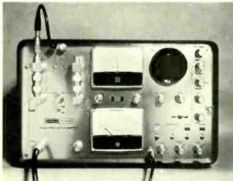
included. Single- and two-tone signals are provided for driving the microphone input of a.m. and s.s.b. transmitters. Price £290. Green Electronic and Communication Equipment Ltd., 79-91 Braemar Road, London N.15.
