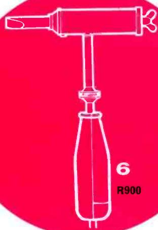
1. 1/8" DIA.—3.2 mm dia detachable bit. Standard temp. 360 c at 19 watts. Special temps. from 253 c 400 c. Weight 4.5 ozs. 127 grms.
