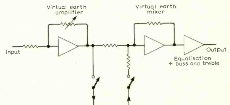
Fig. 3. Input stage of Cambridge Audio P40 and P80.
