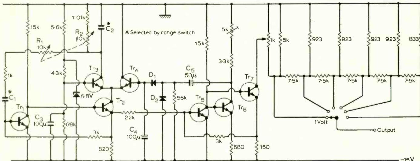
Fig. 12. Wien network signal generator with a.c.
