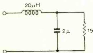
Fig. 7. Test circuit equivalent to Quad electrostatic speaker.
