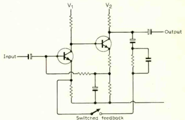
Fig. 1. Input stage of the Heathkit TSA-12.
