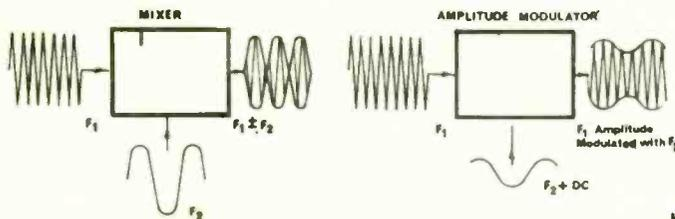
New, versatile Hatfield Modulators Types MD4 and MD6 have been designed using the latest Schottky barrier diodes. The superior wideband match and low noise characteristics of these components enable a very high performance to be obtained. The diagrams below illustrate some of the typical uses for these new units, which also have applications in phase lock loops.
