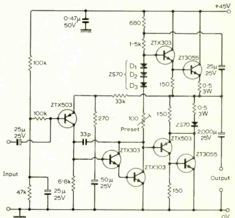
Fig. 4. Complete circuit diagram of modified power amplifier.
