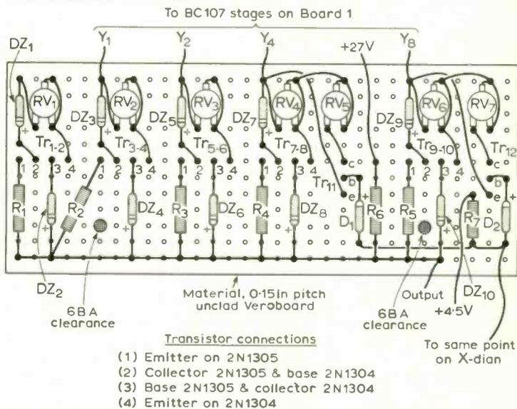
Fig. 19. The position of the dians on the main logic assembly.
