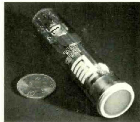
attainable with the target voltage set to produce 0.02  $\mu$ A dark current. This new fibre-optic vidicon is ideal for applications involving coupling to other devices having fibre-optic window outputs, such as image intensifiers. By using fibre-optic windows on both devices and coupling them together in direct optical contact, the optical efficiency can be improved by as much as 50 times compared with a normal lens system. English Electric Valve Co. Ltd., Chelmsford, Essex.
