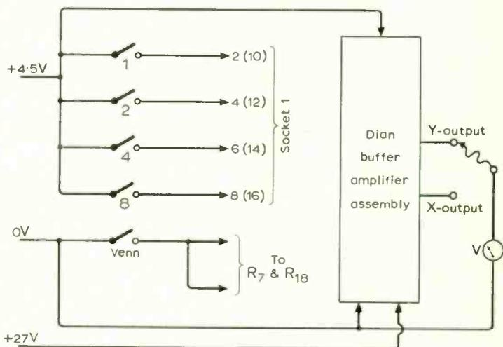
Fig. 24. Buffer amplifier/dian test circuit.
