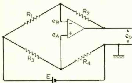
$$e_B = e_0 + \frac{(E - e_0)R_2}{R_1 + R_2}$$
