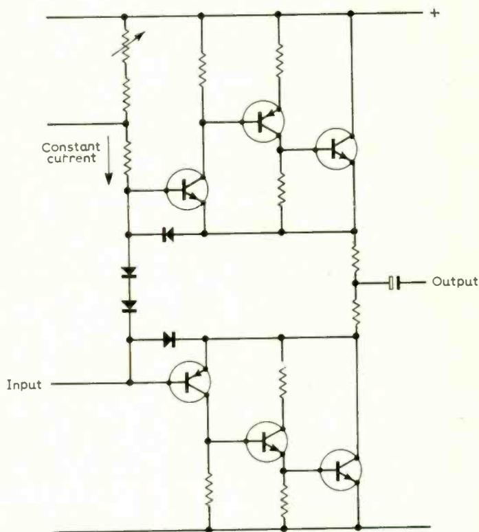
Fig. 6. Output section of Quad 303 power amplifier.
