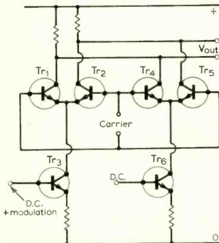
Fig. 4. Modulator with suppression of carrier and modulation frequencies.
