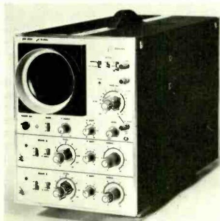
0.5s/div with continuous adjustment of setting. Sweep can be expanded up to five times. The input selector switch features a "0" position which earths the Y amplifier input enabling the d.c. reference level to be found without disconnecting the probe. Pye Unicam Ltd., York Street, Cambridge.
