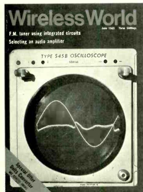
This month's cover picture shows crossover distortion occurring in a class B output stage. The low-level high-order harmonics contained in the apparently clean sinusoid are quite audible although amounting to less than 0.1% distortion.
