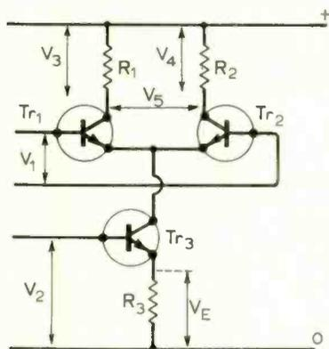
Fig. 1. The basic circuit of the multiplier.
