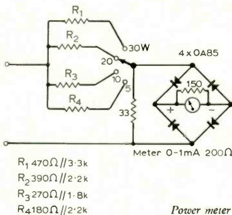
$R_1$ , 2, 3, 4, it may be adapted for other impedances and powers, provided that no more than 1.4V is applied to the bridge input.
