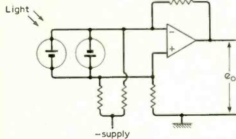
**Features.** In the circuit shown the polarity of the output voltage is dependent on the relative intensity of the light falling on the two cells. Circuits of this type are useful in measuring small deflections of a beam of light.
