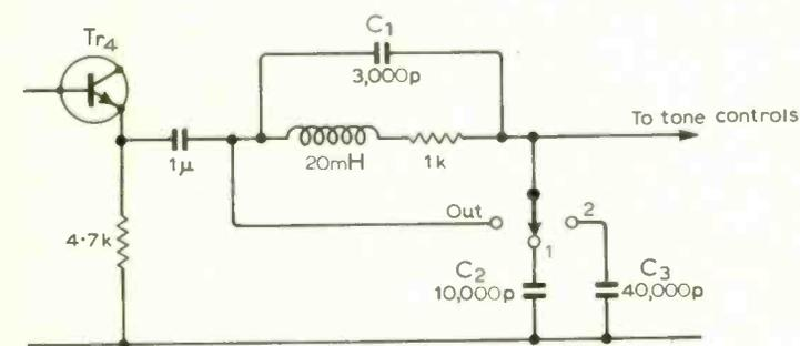
Fig. 1. Modified treble-filter circuit.
