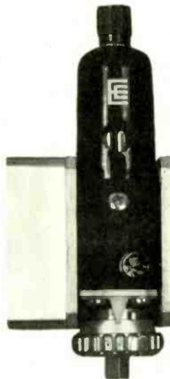
of the limiter stage gives added protection against spike leakage, which in turn reduces noise deterioration and limits crystal burn-out. For use in marine radar applications the BS908 is tunable over the frequency range 9250 to 9550MHz, and will work in duplexers with up to 75kW transmitted power. Overall dimensions are height 96.85mm, width across mounting flange 41.28mm and depth 39.5mm. Net weight is approximately 250g. English Electric Valve Co. Ltd, Chelmsford, Essex.
