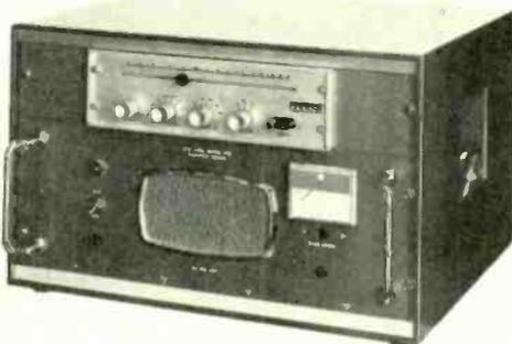
PPA120VA, complete in its own free-standing cabinet, can be used as a general purpose laboratory power supply to provide any frequency between 40Hz and 10kHz. The output voltage is continuously variable between zero and 100%.
