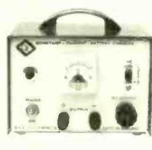
**CONSTANT CURRENT BATTERY CHARGER TYPE R41.** The adjustable constant-current nickel-cadmium cell charger will deliver 1-20 mA indicated on a front panel meter. This battery charger will accommodate at least 10 cells in series, having capacities up to 1Ah. The instrument is completely safe and cannot be damaged by short-circuiting the output terminals or reversed battery connections. Dimensions: 6inx4inx3in deep. **PRICE: £10.0.0.** Carr. 10/- (U.K. only).
