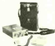
**Pye 'Bantam' Portable VHF Radiotelephone**
