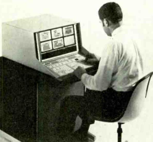
*Ampex v.t.r. controller allowing random access to material on one or more video tape recorders. Television frames are individually addressed to allow automatic searching.*
