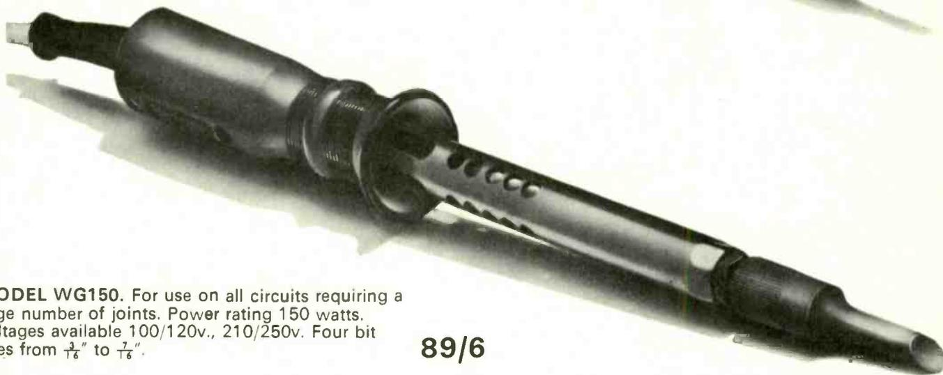
**MODEL WG150.** For use on all circuits requiring a large number of joints. Power rating 150 watts. Voltages available 100/120v., 210/250v. Four bit sizes from  $\frac{3}{16}$ " to  $\frac{7}{16}$ ".
