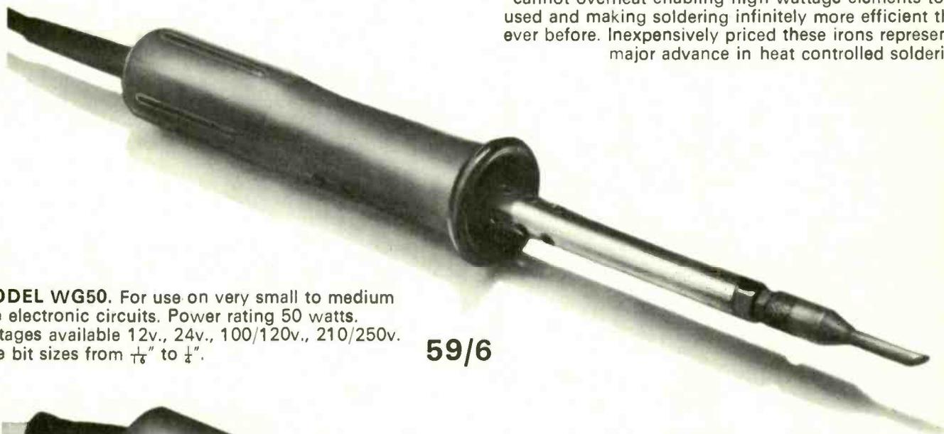
**MODEL WG50.** For use on very small to medium size electronic circuits. Power rating 50 watts. Voltages available 12v., 24v., 100/120v., 210/250v. Five bit sizes from  $\frac{1}{16}$ " to  $\frac{1}{4}$ ".
