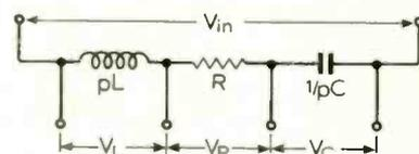
Fig. 9. Showing the voltages across each of the three elements.
