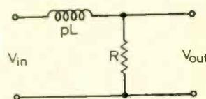
Fig. 2. 1st-order LR low-pass filter, or simple-lag network.
