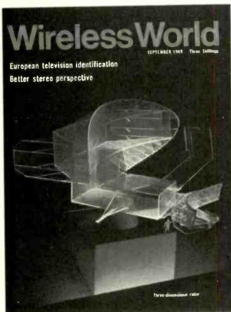
This month's cover. A Perspex model of a three-dimensional radar scanner developed by R.R.E. (see p. 422) illuminated by ultra violet light.
