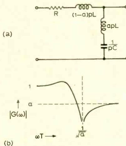
Fig. 19. 2nd-order filter giving unsymmetrical notch response (low-pass type),
