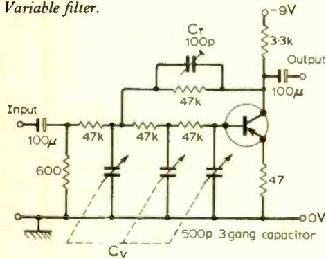
this type of circuit. The range may be altered by fixed capacitors across  $C_v$  although this practice will reduce the range.
