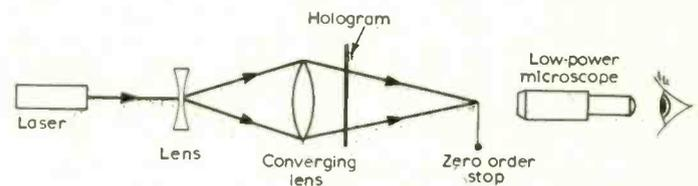
Fig. 4. Optical system for reconstructing a three-dimensional image.
