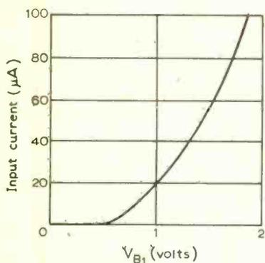
Fig. 5(a). Input characteristic for upper (Darlington) pair of Fig. 2.
