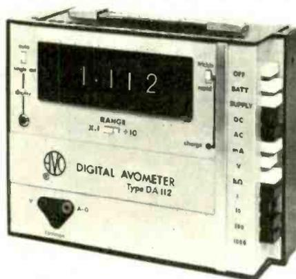
tinuous operation. The meter may also be operated from a 12V car battery. The measured value is presented on a  $3\frac{1}{2}$  digit display with automatic decimal point and over-range indication. A print-out socket (parallel BCD 1248 code) is available as an optional extra. Avo Ltd, Avocet House, Dover, Kent.
