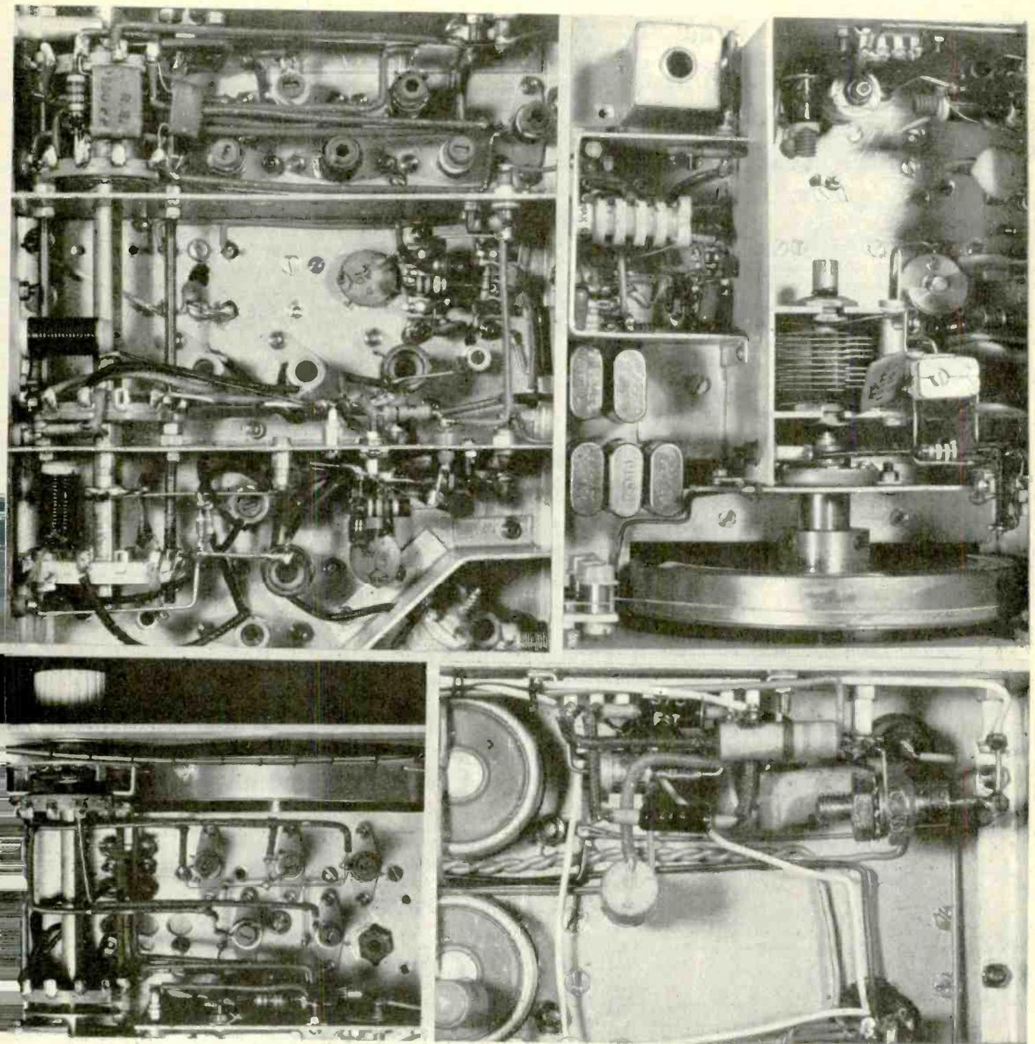
Fig. 26. Various sections of the completed receiver; top left from top to bottom — local oscillator synthesizer, receiver mixer and r.f. stage; bottom left — h.f. crystal oscillator; top right — v.f.o. amplifier, and h.f. oscillator crystals; bottom right — underside of power supply.
