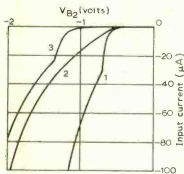
Fig. 5(b). Input characteristics for lower (conjugate) pair of Fig. 2. Curve 1,  $S$  closed; 2, circuit as shown; and 3,  $S$  closed, power diode in series with  $R_s$  (Mr. Shaw's scheme).
