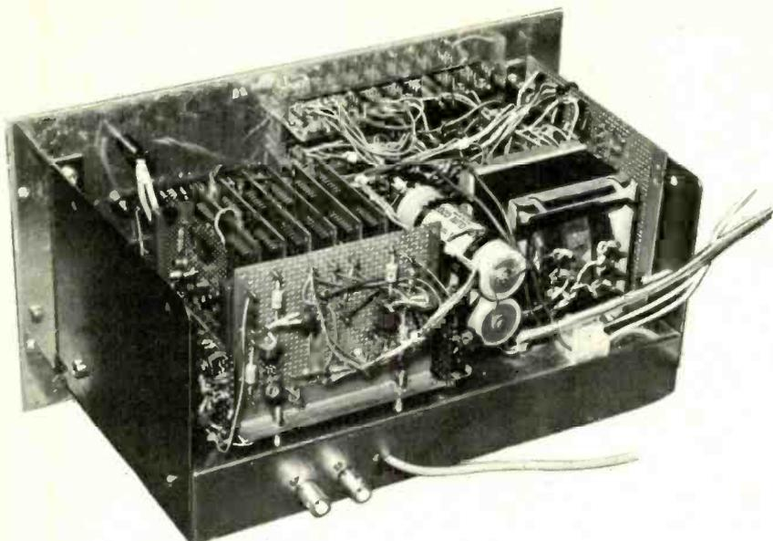
(above) Fig. 73. Rear chassis view of the prototype. The extra board mounted on the rear of the main logic unit contains the parts for one of the modifications to be described later in the series. The board on the right, behind the mains transformer, is also associated with a modification.
