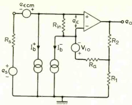
It is assumed that  $R_s \ll R_{cm}$ . Common mode error voltage
