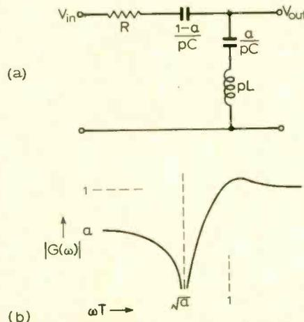
Fig. 20. 2nd-order unsymmetrical notch filter (high-pass type): (a) network, (b) amplitude response.
