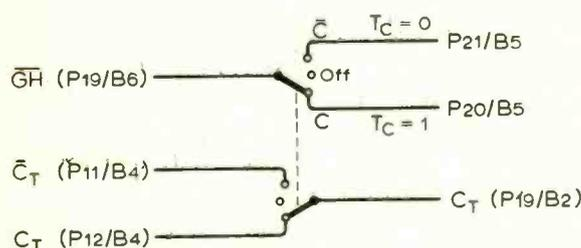
Fig. 67. Wiring of the Truth table column C control switch
