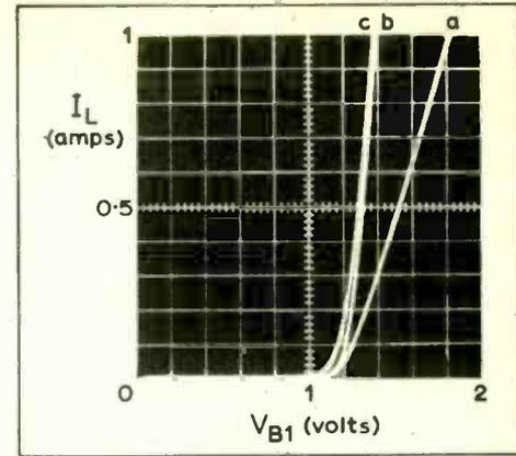
Fig. 3. Characteristics for upper (Darlington) pair of Fig. 2. Curve (a) circuit as shown; (b)  $R_2$  short-circuited; and (c)  $R_1$  omitted,  $R_2$  short-circuited.
