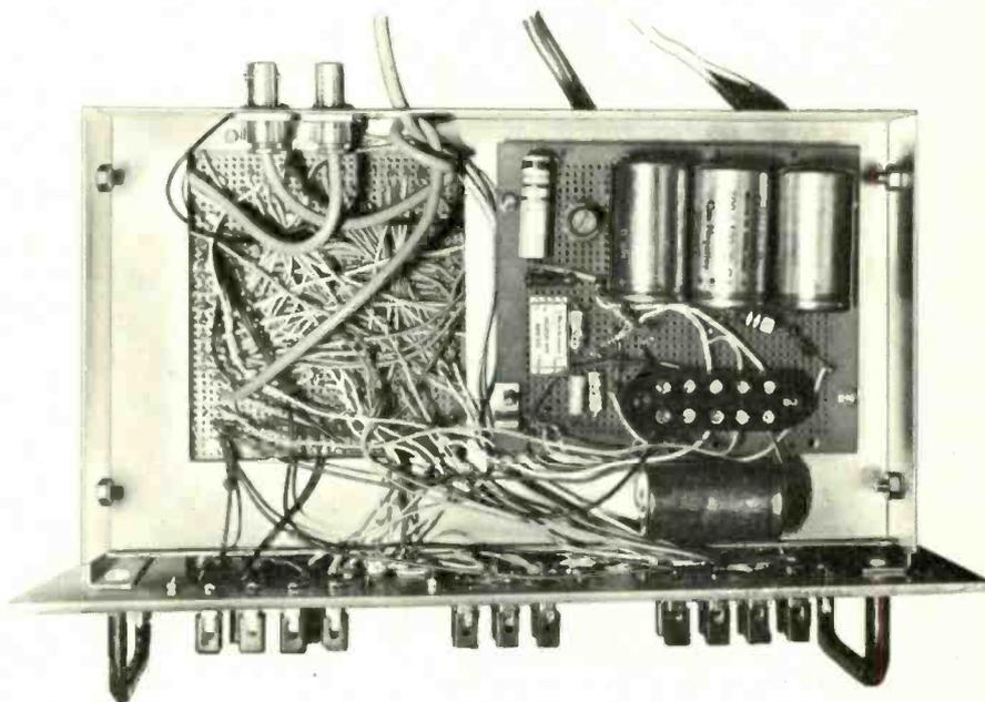
(below) Fig. 72. Under chassis view of the complete instrument. On the left, through the cutout in the chassis, the underside of the main logic assembly can be seen. On the right is a board containing the small components of the power supply.
