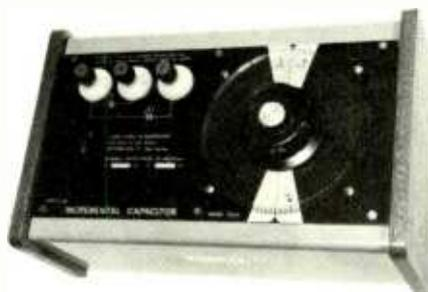
Accuracy of calibration at 20°C is  $\pm 1\%$ . The maximum d.c. working voltage is 500V, and the maximum recommended frequency is 10MHz. J. J. Lloyd Instruments Ltd, Brook Avenue, Warrasash, Southampton SO3 6HP.
