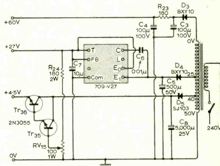
Fig. 71. The power supply
