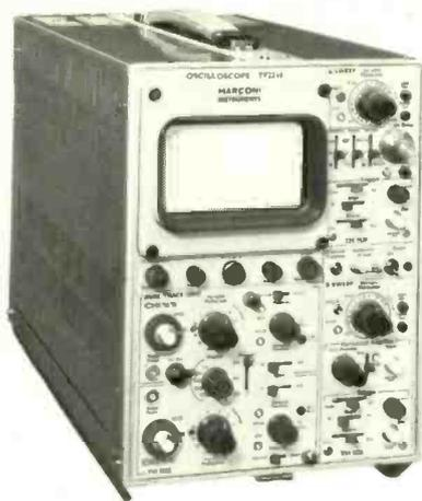
combined with the dual trace Y input system to view each of two incoming waveforms at two sweep speeds, giving a display comprising four separate traces. Marconi Instruments Ltd, St. Albans, Herts.
