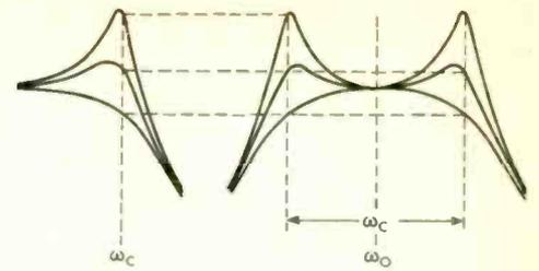
Fig. 15. Comparison of 2nd-order band-pass with corresponding 2nd-order low-pass responses.
