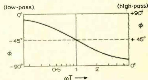
Fig. 4. Phase response of 1st-order filters: l-p (left-hand scale); h-p (right-hand scale).
