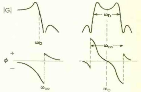
Fig. 16. Showing low-pass response transformed into band-pass response.
