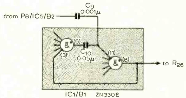
Fig. 69. The monostable which provides the gating pulses for the video amplifier
