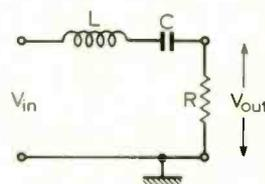
Fig. 11. 2nd-order LCR series network connected for "tuned-circuit", or 1st-order band-pass, response.
