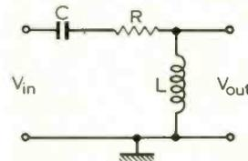
Fig. 10. 2nd-order LCR series network connected as h-p filter.
