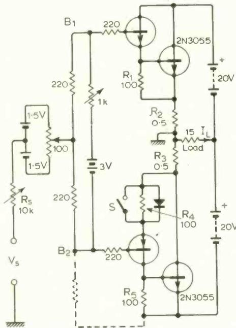
Fig. 2. Experimental circuit with shifted earth point. The broken-line resistor represents the effect of finite output resistance in  $Tr_1$  of Fig. 1. The 220-ohm base resistors are to prevent parasites; the writer's rather straggly version also required a series combination of 33 ohms and 100pF between base and collector of the top driver transistor only.
