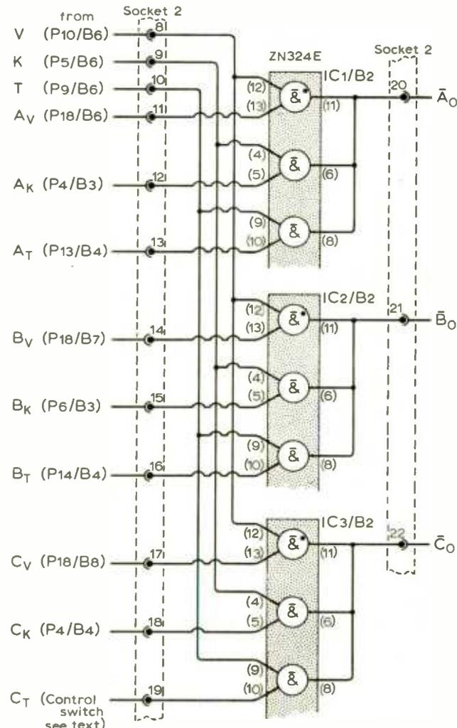
Fig. 66. Circuit which allows the control signals to select the correct output variables
