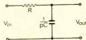
Fig. 1. 1st-order CR low-pass filter, or simple-lag network.
