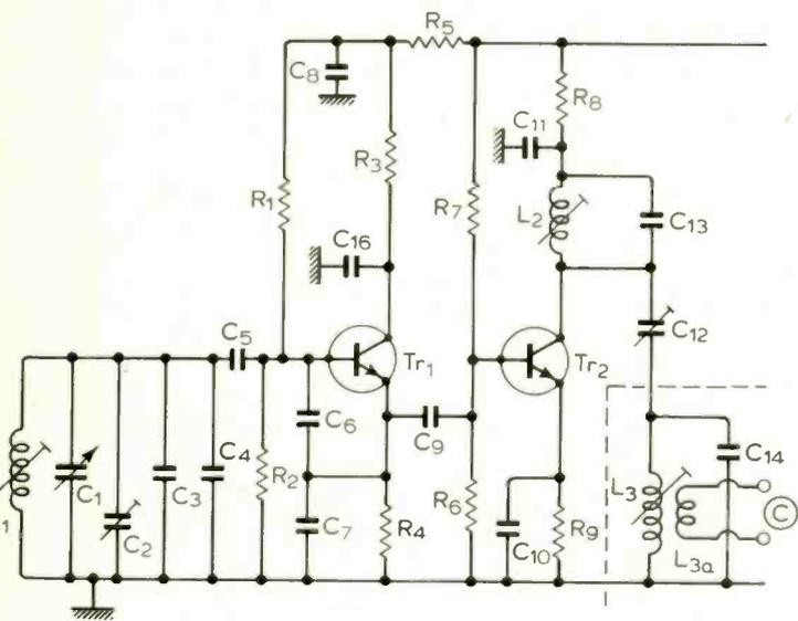
Fig. 22. The v.f.o. section of the local oscillator synthesizer.
