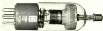
is a direct electrical equivalent to the KU82/7583, capable of handling peak pulse currents up to 35A at a peak forward anode voltage of up to 8KV, advance production techniques and the inclusion of an internally connected hydrogen reservoir give a much improved life expectancy. Warranty is for 1000 hours operation. English Electric Valve Co. Ltd., Chelmsford, Essex.
