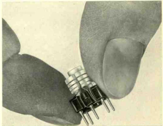
Available in 5, 7, and 10mm cans to meet AM and FM requirements, with frequency range from 100KHz to 100MHz. High packaging density, low cost with high reliability (reject rate 0-01). The unique construction of the bobbin enables close tolerance windings to within a quarter of a turn, and prevents shearing of wires on alignment.
