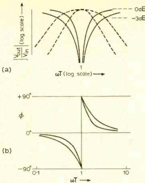
Fig. 18a. Symmetrical notches, normalised amplitude responses, together with tuned-circuit responses of equal  $Q$  factor.
