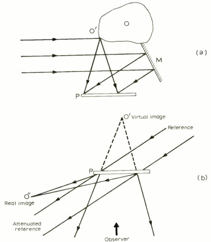
Fig. 1. The holographic process: (a) making the hologram; (b) reconstructing the three-dimensional image.
