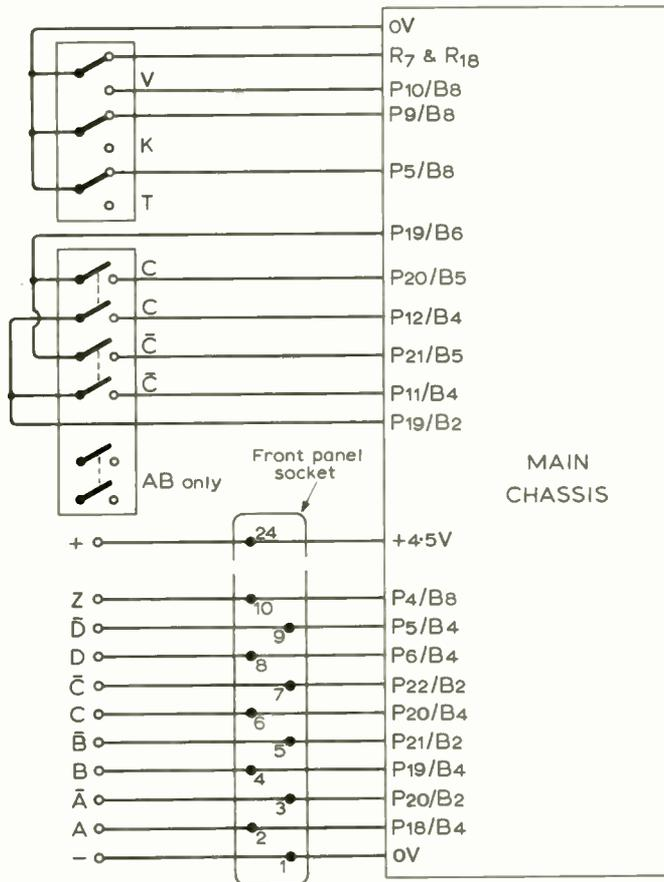
Fig. 75. Front panel components to main chassis connection diagram
