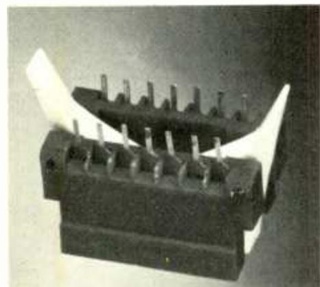
profile mounted units. Gold plated beryllium upper contacts are used to minimize contact resistance which is normally less than 5 milliohms. The unit is moulded Kemetal with Delrin spring claws. The unit is also supplied without clips for mounting in multiples on p.c. boards when production printed circuit assemblies require multi function check and test. The price is 20s each for 100 or more. W.E.L. Components Ltd, 5 Loverock Road, Reading, Berks.
