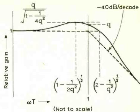
Fig. 8. Relative positions of some of the characteristic points on a 2nd-order low-pass amplitude/frequency response curve.
