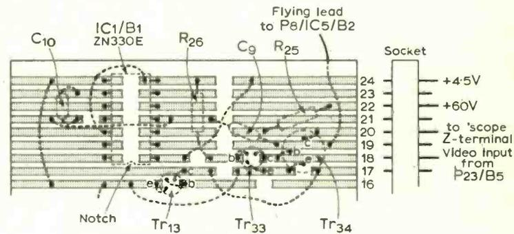
Fig. 70. Practical details of the video amplifier and monostable circuits
