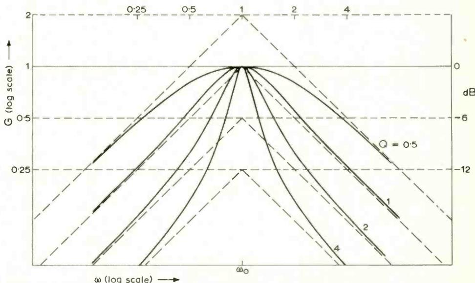
Fig. 12. Tuned-circuit response as defined by eqns. (27) and (28).
