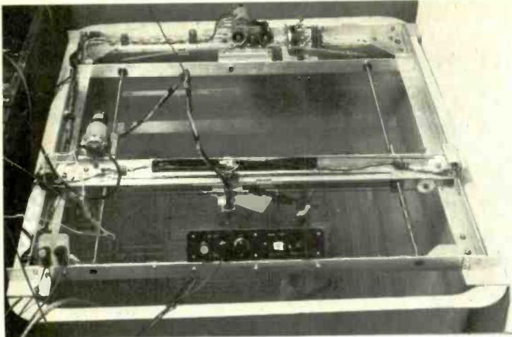
Fig. 5. Mechanical scanning frame used to produce holograms.
