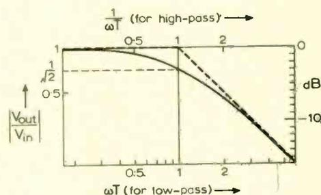
Fig. 3. Amplitude, or gain, characteristic of 1st-order l-p filter (lower scale), and 1st-order h-p filter (upper scale).
