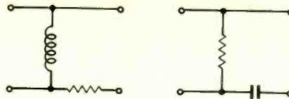
Fig. 5. 1st-order high-pass filters or simple-lead networks.
