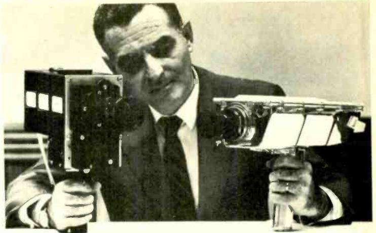
*The two television cameras used on the mission: left, the colour camera carried in the command module to televise activities in flight; right, the black-and-white camera carried in the lunar module and used to televise scenes on the surface of the moon.*
