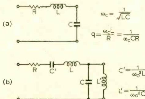
Fig. 14. Low-pass to band-pass transformation.
