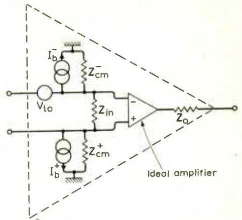
Fig. 1. Simplified equivalent circuit for real amplifier.
