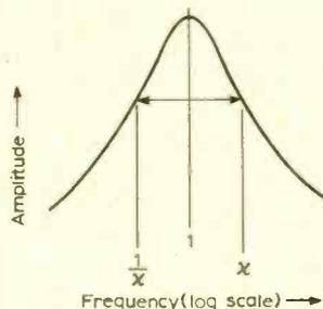
Fig. 13. Showing the symmetry of "tuned-circuit" response when plotted to a logarithmic scale.
