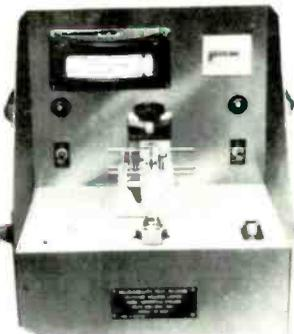
Incorporates many new features, including semi-automatic electrical timing, proportional temperature control, remote controlled specimen lowering system and a temperature meter calibrated to an accuracy of 0.25% full scale deflection at the test temperature. The machine can reduce production costs by instantly checking the solderability of components with wire terminations. It complies with B.S.I. and proposed M. of D. and International Solderability Test Specifications.
