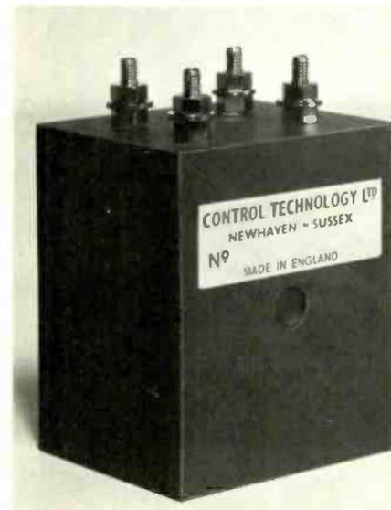
resistance. Thus only one basic unit need be stocked to cover a variety of applications. The output is 0-10V at 10mA and the input impedance is typically 1.25k $\Omega$ . It is intended for use where an isolated d.c. signal voltage is required for measurement or control, in particular for applications such as thyristor drives and motor control. The unit is fully resin encapsulated and measures 44 x 51 x 63 mm. Control Technology Ltd, Meeching Road, Newhaven, Sussex.
