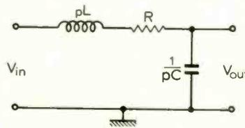
Fig. 6. 2nd-order LCR series network connected as 1-p filter.
