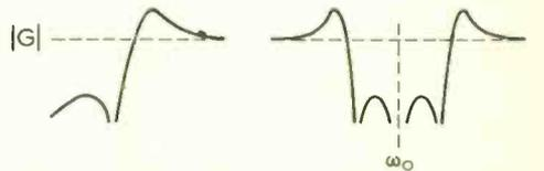
Fig. 17. High-pass response transformed into band-stop response.
