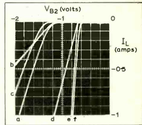
Fig. 4. Characteristics for lower (conjugate) pair of Fig. 2. Curve (a) circuit as shown; (b) diode removed; (c)  $S$  closed, power diode inserted in series with  $R_3$  (Mr. Shaw's scheme); (d)  $S$  closed, otherwise as shown; (e)  $S$  closed, no diode,  $R_3$  short-circuited; and (f) as for (e) but with  $R_3$  removed.
