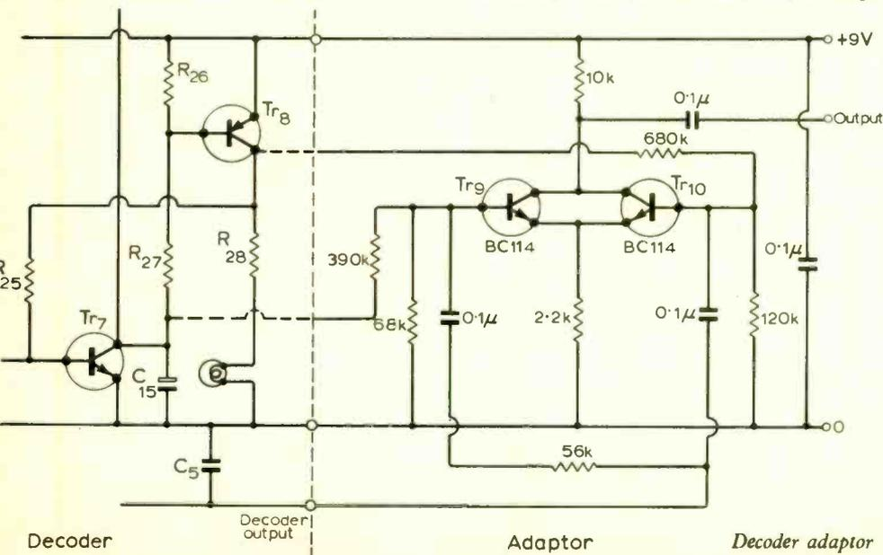
disadvantage in that the voltage gains for mono and stereo were about 0.5 and 0.25 respectively. By adding the circuit below to the decoder, unity gain for both mono and stereo is obtained.
