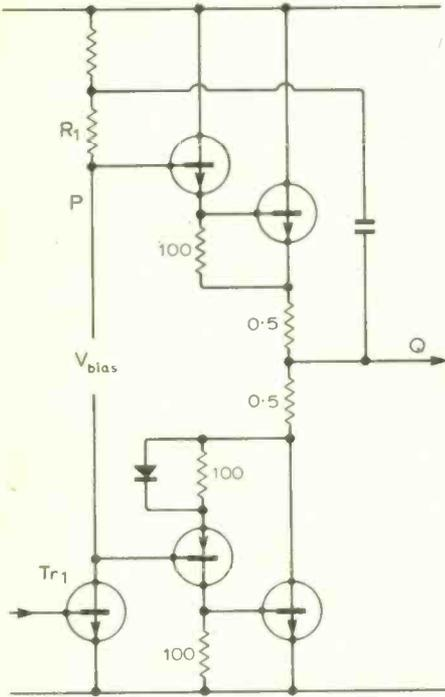
Fig. 1. An effective modification for reducing crossover distortion.
