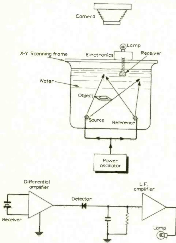
Fig. 2. Typical acoustical holograph recording process.
