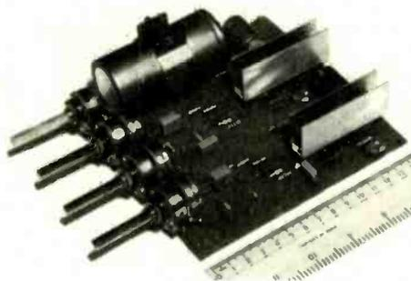
is 30dB. A printed circuit board only 152 x 140mm (6 x 5.5in.) in size supports all the components of the amplifier, controls, power supply rectifier and smoothing circuit. A.C. at 16V is required. Britmac Electrical Company Ltd, Electronics Division, Shelley Road, Preston, Lancs.
