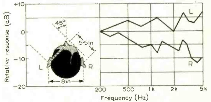
Fig. 1. Graph of level differences for a sound source located at 45° to the left of the listener.
