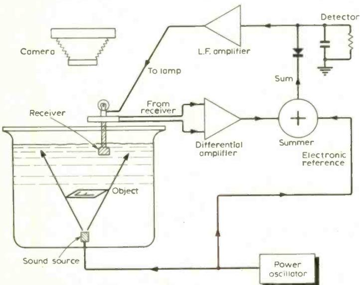
Fig. 6. System using a reference beam from an oscillator.
