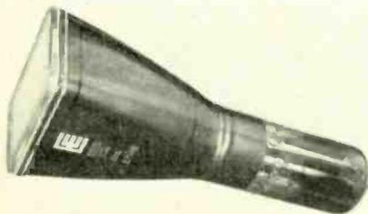
tube has a writing speed in the storage mode of  $0.5\text{cm}/\mu\text{s}$ , a deflection sensitivity of approximately 12V/cm in both axes, at a writing beam voltage of 1.5kV, a typical line width of 0.4mm in the c.r.t. mode. The English Electric Valve Co. Ltd, Chelmsford, Essex.
