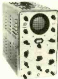
Bandwidth 10mc/s. Triggered and free-running time base. Pulses from .1 to 3,000 microseconds can be observed. Max. overshoot of 1 microsec. pulse 5%. Built-in time base calibrator and amplitude calibrator. Sensitivity from .3 to 25 Vrms/mm. Telescopic viewing hood.
