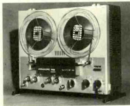
This recorder has a frequency range of 30Hz—20kHz at 7½ i.p.s. At 3¼, and 1⅞ i.p.s. the upper limit is 15 and 8kHz respectively. Each channel amplifier can deliver 4W into 4Ω. Bosch Ltd., Rhodes Way, Radlett Road, Watford, Herts.
