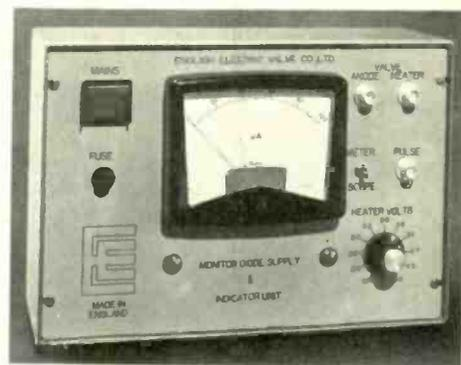
panel of the instrument. A heater-voltage control, also on the front panel, provides for adjustment of the diode heater-voltage for all conditions of r.f. input. The correct diode load-resistance is built into the unit. English Electric Valve Co. Ltd, Chelmsford, Essex.
