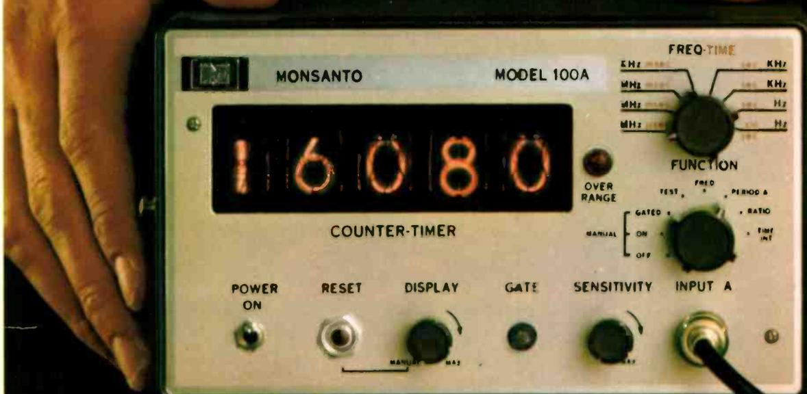
The Monsanto Model 100A Counter/Timer measures frequency up to 12.5 MHz, single period or frequency ratio ; or counts total events. It has a crystal controlled clock and integrated circuits . . . Its price is £300.
