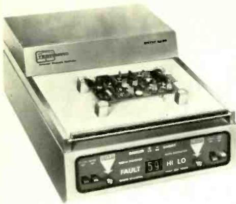
tests is d.c. voltage checks and any subsidiary signals, circuits or supplies can be fed into the TM60 at the rear of the unit or embodied in the programme board.
