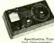
Specification. Type: Moving Coil Galvanometer. Ranges: 1. 0.05 to 5 ohms. 2. 0.5 to 50 ohms. 3. 5 to 500 ohms. 4. 50 to 5,000 ohms. 5. 500 to 50,000 ohms. Scales: Switched. Bildivire: 0.5. Case: Moulded plastic. Internal Source: 4V. Dry battery. Dimensions: 200 x 110 x 65mm. Weight: 0.9 kg. List price £25. Our price £9/19/6.
