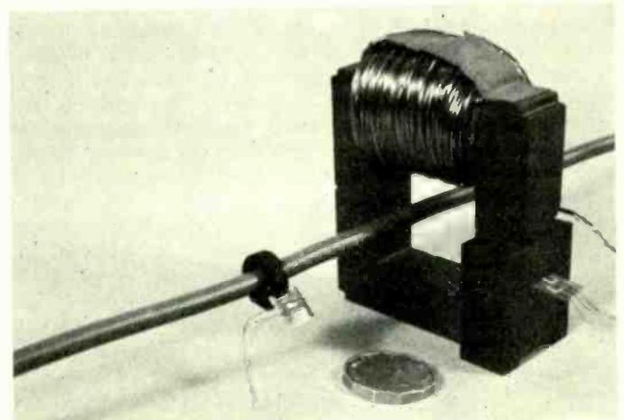
The magnetic circuits for the mean-square ammeter (left) and the d.c. transformer (right) are shown here. The magnetoresistances are also visible, but in operation one would be in the air gap.
