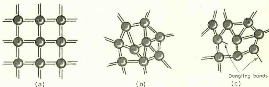
Fig. 1. Covalent binding (schematic) (a) crystalline state (b) amorphous state (c) amorphous state indicating dangling bonds.
