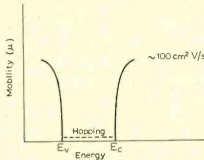
density of electron states throughout the energy 'gap' in amorphous materials, none the less the mobility of any electrons filling those states can probably be ignored. The idea is shown schematically in Fig. 4.
