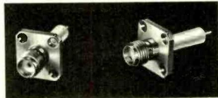
50-645-4520-31, the receptacle is constructed of gold plated stainless steel, Teflon, and gold-plated beryllium copper. It meets all requirements of MIL-C-39012 regarding contact and dielectric torque and captivation. R. F. Components Division, Sealectro Ltd, Walton Road, Farlington, Portsmouth, PO6 1TB.
