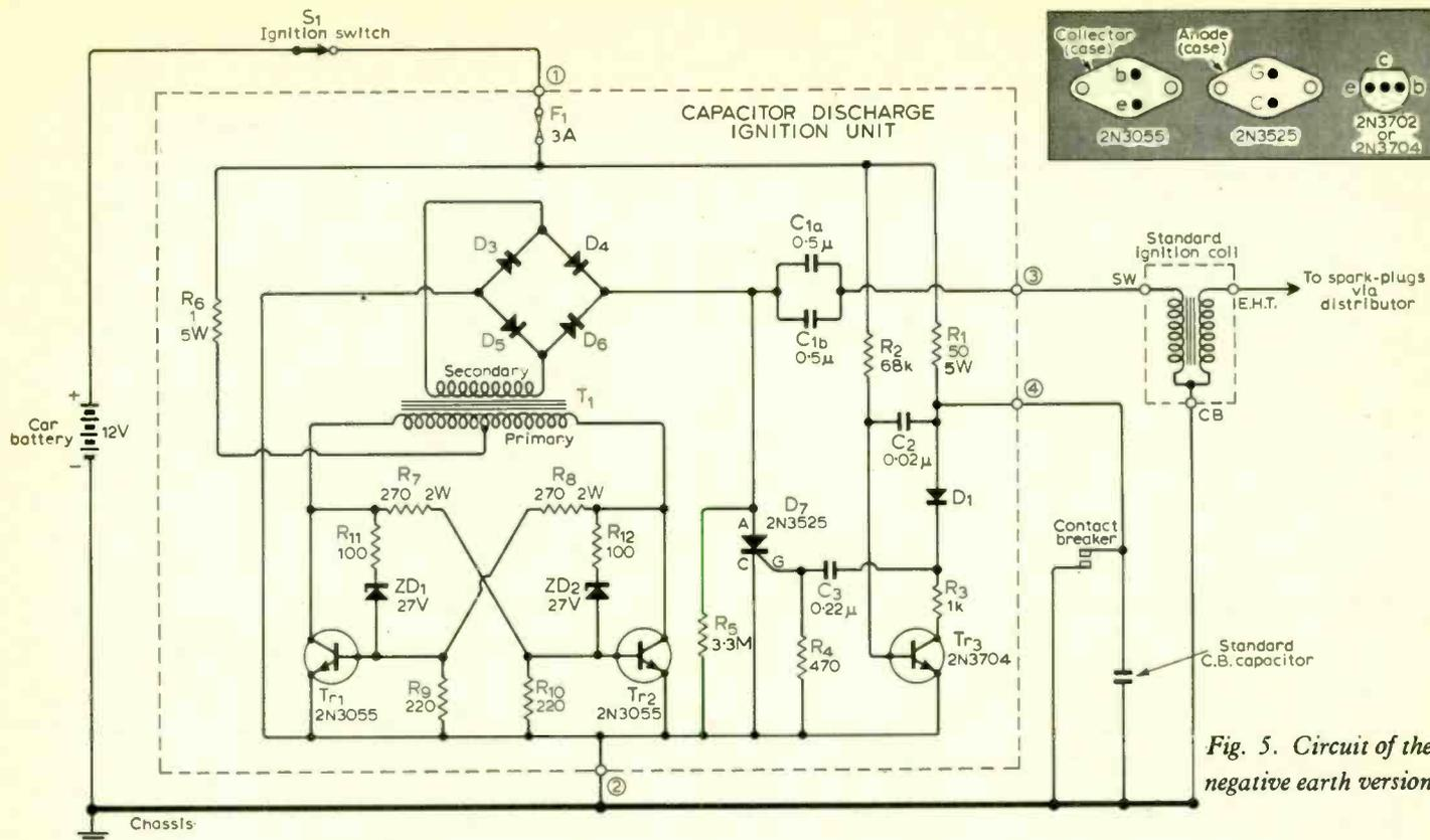
Fig. 5. Circuit of the negative earth version.
