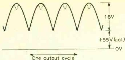
Fig. 5. Waveform across tail resistor. 'Dents' in the peaks indicate that the collectors are bottoming.
