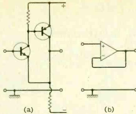
Fig. 3. Possible amplifier configurations for  $K \rightarrow 1$ .
