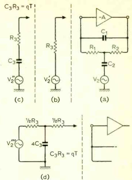
Fig. 13. Derivation of band-pass filter and an alternative form of low-pass filter from the standard l.p. filter (Fig. 4).
