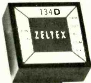
plastic/epoxy case can be mounted directly on a p.c. board or plugged into a mating connector. Specification includes an output of  $\pm$ V at 4mA, a d.c. gain of 50,000, and a gain/bandwidth product of 1.3 MHz. Frequency at full output is 100kHz. The slew rate is 6V/s and operating temperature  $-25$  to  $+85^{\circ}$ C. Price is £8 5s. Advance Institute Electronics, Raynham Road, Bishops Stortford, Herts.
