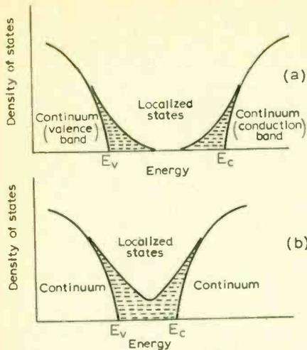
(Left). Fig. 3. Density of electron states in amorphous semiconductor (a) non-overlapping localized states (b) overlapping localized states.
