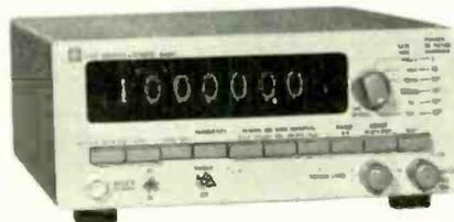
500MHz. Models are available with 5, 6 or 7 digit presentation. When measuring frequency from d.c. to 32MHz, the counting gate times are 100 $\mu$ s to 10s, and Hz, kHz and MHz can be displayed with positioned
