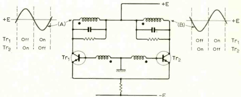
Fig. 3. Diode of Fig. 2 replaced by second transistor.
