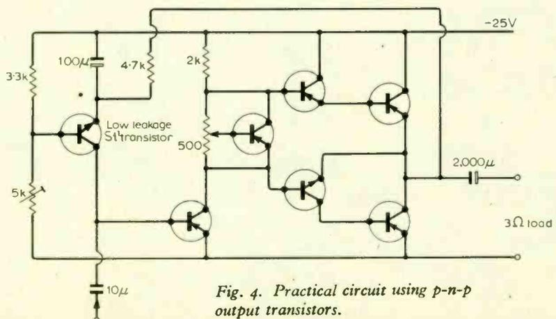
Fig. 4. Practical circuit using p-n-p output transistors.
