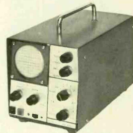
to  $100\text{kHz}$ . The instrument costs  $\pounds 24.10\text{s}$ . (discount for schools) and features a Y sensitivity of approximately  $100\text{mV/cm}$  at maximum gain with full Y shift. The timebase range covers approximately  $100\text{ms/cm}$  to  $10\ \mu\text{s/cm}$  and is automatically synchronized. The X input required is  $1\text{V/cm}$  with full X shift when the timebase is switched off. Flyback suppression and access to Y plates
