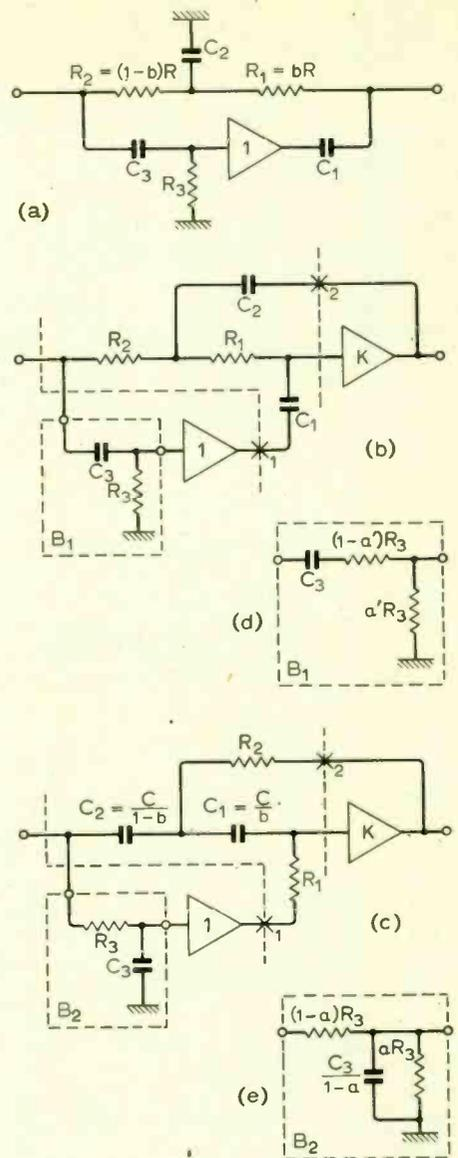
Fig. 11. Modifications for obtaining a notch (or zero): (a) Effectively passive symmetrical notch filter with buffer amplifier in h.p. path; (b) the same made active; (c) similar circuit with buffer in the l.p. path; (d) a method of putting attenuation in the h.p. path of (b); (e) in the l.p. path of (c).
