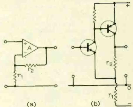
Fig. 5. Feedback less than 100%.
