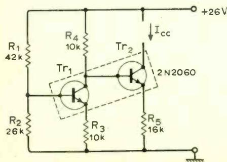
The measured temperature coefficient of  $I_{cc}$  is typically 0.0015%/°C over the temperature range 0 to 100°C.
