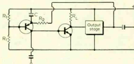
Fig. 3. Use of common-base stage to control d.c. level of amplifier output.
