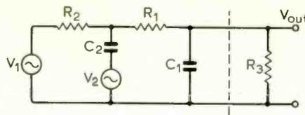
$$T_2 = \frac{C_2 R_2 R_1}{R_1 + R_2}, \quad T_1^* = k_1 C_1 (R_1 + R_2)$$
