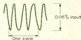
Fig. 8. Residual waveform at the base winding after passing through the twin-T filter.
