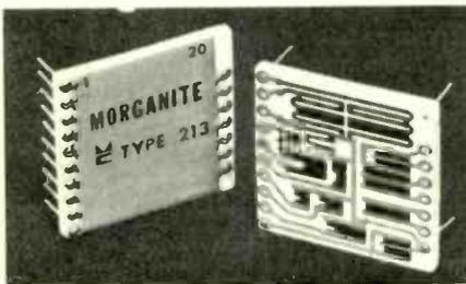
fier summation. Model 213 is a 10-bit binary resistor array designed to be compatible with the Fairchild  $\mu$ A 722 current source for D/A and A/D applications. Resistance values correspond directly with those specified on the A 722 data sheet. The resistance temperature coefficient is 0 to -200 p.p.m./°C with resistance tolerance of  $\pm 2\%$  over the temperature range -20 to +85°C. Morganite Resistors Ltd, Bede Industrial Estate, Jarrow, Co. Durham.
