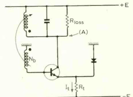
Fig. 2. Tail current is switched between the transistor and the diode.
