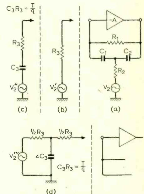
Fig. 14. Similar derivations from the standard h.p. filter (Fig. 10).
