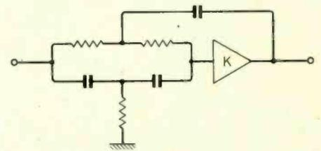
Fig. 12. Notch filter without buffer.
