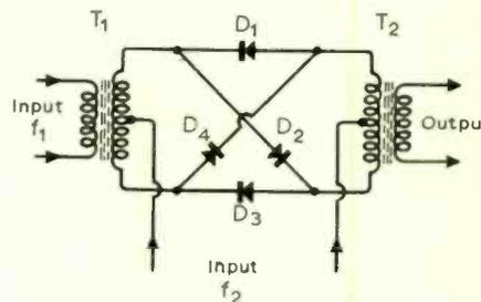
Fig. 3. Basic ring modulator circuit.
