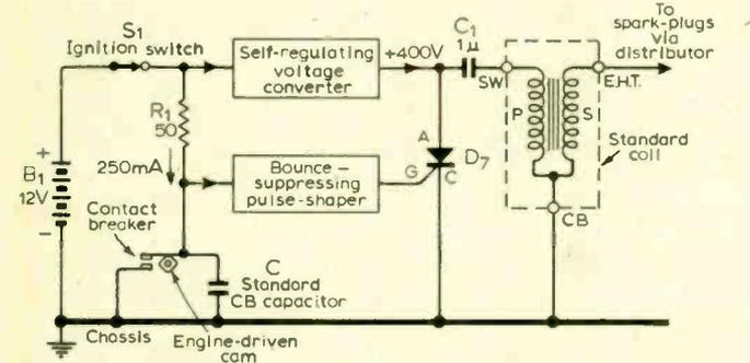
Fig. 3. Block diagram of the capacitive discharge ignition system described in the article.
