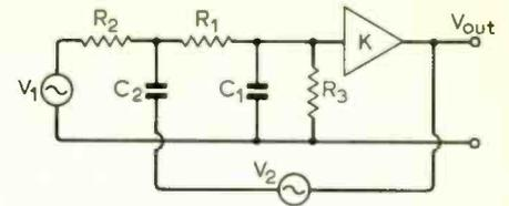
Fig. 7. Resistance-loaded network in active filter.
