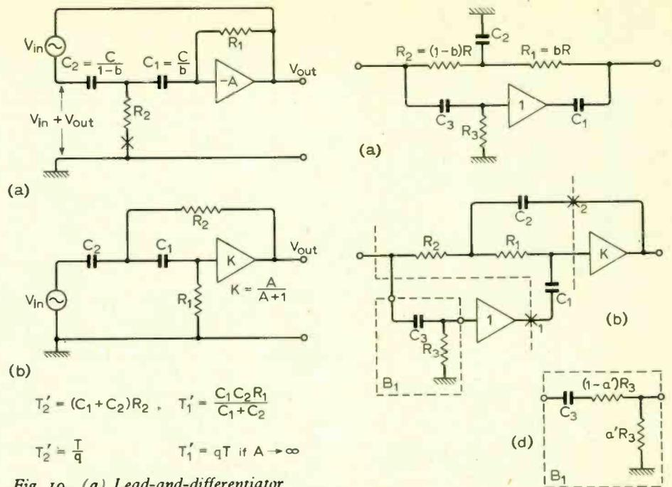
Fig. 10. (a) Lead-and-differentiator loop with series feedback; (b) the same converted by change of earth point to Sallen-and-Key h.p. filter.
