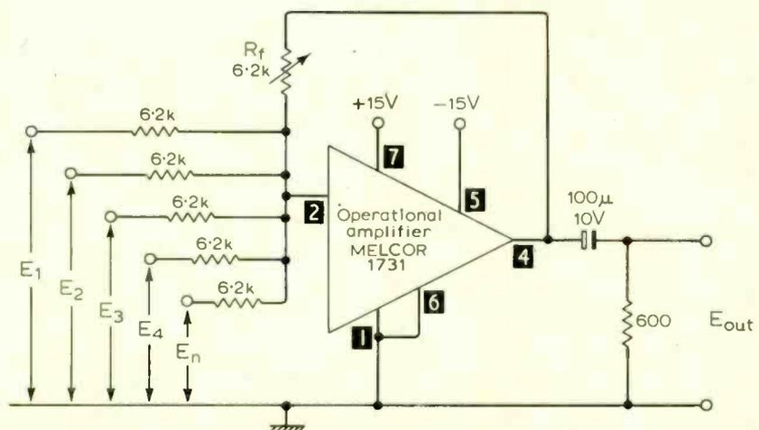
Fig. 2. Mixer using operational amplifier.
