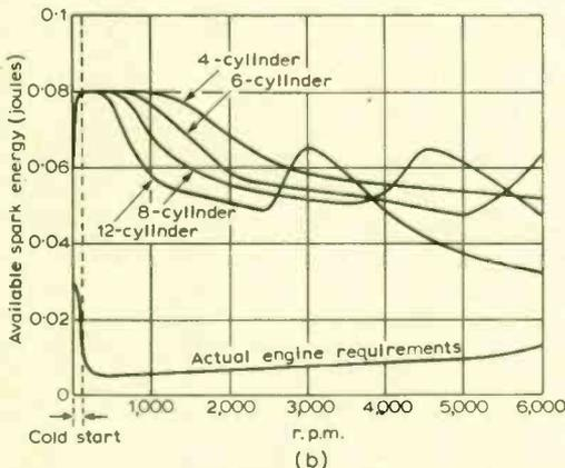
Fig. 4. Curves showing the measure performance of the capacitive discharge ignition system with the same battery voltage conditions as Fig. 2.
