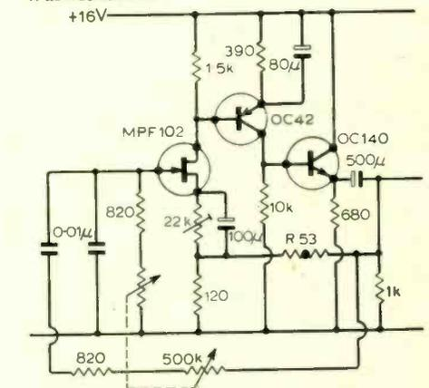
Wien bridge oscillator covering audio range with no capacitor switching.
