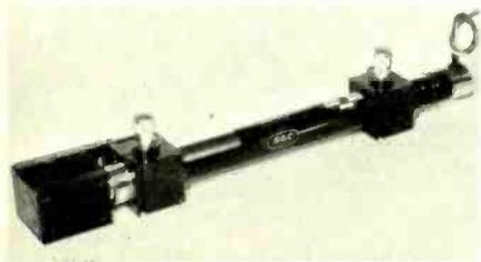
obtain power outputs of over 20 watts at spot frequencies. The tube is packed in a permanent magnet focusing mount, and r.f. coupling is by means of a type N 50 connector. Cooling may be by either conduction or convection, according to specification. The M-O Valve Co. Ltd, Brook Green Works, London W.6.
