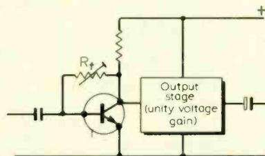
Fig. 1. Arrangement where driver stage  $Tr_1$  controls d.c. level of output pair.
