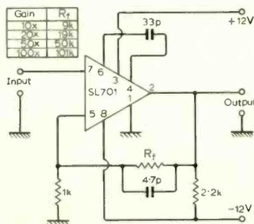
$50k \Omega, \times 100, R_f = 101k \Omega$  Typical drift is quoted as  $15\mu V/^\circ C$ . Extracted from Plessey Technical Communication No. 7.
