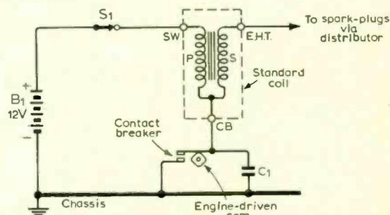
Fig. 1. Circuit of a conventional inductive discharge ignition system.
