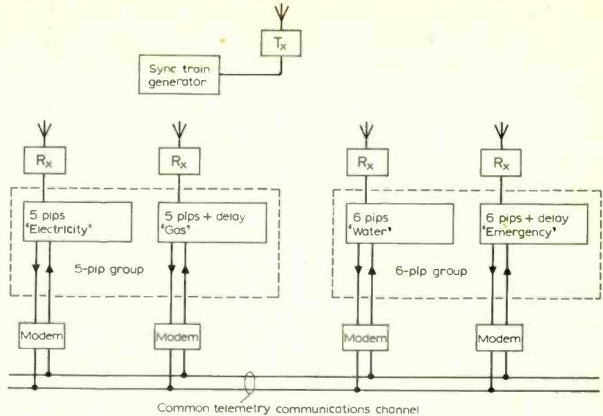
Fig. 1 "Telegrid" diagrammatic network arrangement.
