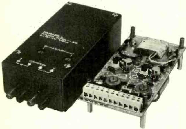
The A.15 is intended for driving operational amplifiers and the twin output, nominally 15V, can be varied between 12-17V or connected in series to provide 24-34V. Both ganged control and independent adjustment of one output enable precise setting of output voltages.
