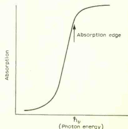
Fig. 2. Absorption edge (schematic). Absorption of light by a crystal against light frequency.
