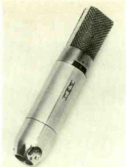
signal cable powering system, which permits the use of a screened twin cable to carry the microphone current (0.5 to 0.7mA) and the output signal current. Suitable for all broadcasting and recording use, the unit measures 150 × 31mm, has stand adaptation or can be hand-held. Jagor Interelectric Ltd, Mercury House, Hanger Green, Ealing, London W.5.
