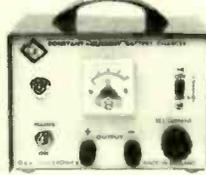
CONSTANT-CURRENT BATTERY CHARGER TYPE R41. The adjustable constant-current nickel-cadmium cell charger will deliver 1-20 mA indicated on front panel meter. This battery charger will accommodate at least 10 cells in series, having r-packets up to 1Ah. The instrument is completely safe and cannot be damaged by short-circuiting the output terminals or reversed battery connections. Dimensions: 6inx4inx3in deep. PRICE: £10.0.0. Carr. 10/- (U.K. only).
