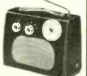
**TRANSONA FIVE, MEDIUM, LONG AND TRAWLER BAND WITH SPEAKER AND EARPIECE.** 5 transistors and 2 diodes. ferrite rod aerial, moving coil speaker. 6 1/2 x 4 1/2 x 1 1/2 in. Total Building Costs 47/6. P. & P. 3/6. Plans and Parts list 1/6 (free with parts).
