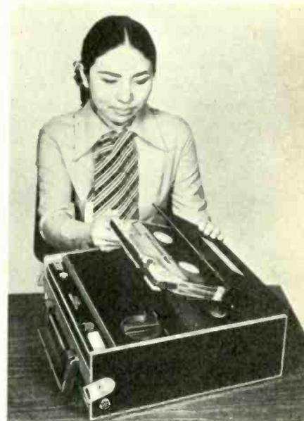
The Panasonic (Matsushita) magazine loading v.t.r. The unit is built to the specifications laid down in the Japanese Type I Standard for  $\frac{1}{2}$ -inch video tape recorders. The magazine illustrated contains enough tape for recording and reproducing a 30-minute programme.
