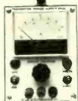
TRANSISTOR STABILIZED POWER SUPPLY TYPE R31/A Output Voltage: 0 to +30V, 0 to -30V, continuously variable. Output Current: up to 1.5A. Automatic overload and short circuit protection. Current and Voltage metered. Output Resistance: less than 0.08 ohm. Regulation: Full load to no load better than 0.1%. Ripple less than 1mV p/p. Dimensions: 6inx4inx2in. PRICE: £28.10.0. Carr. 17/6 (U.K. only).
