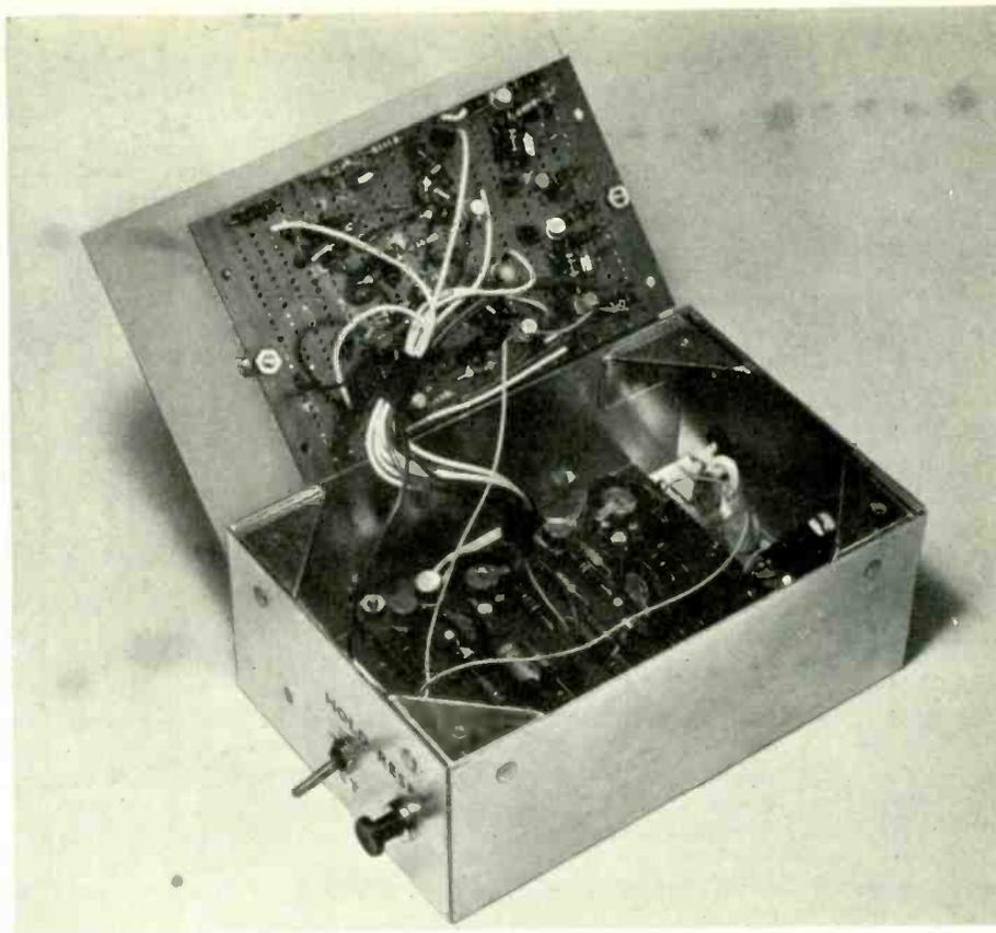
The components of the digitally-controlled pre-amp. need take up little space—the aluminium case shown measures only 6in × 4in × 2½in. The bistables are mounted on the board attached to the lid of the container, the other board carrying the amplifier and the peak-level sensor. Amplifier input and output are carried by screened leads. The bunch of unscreened leads joining pulse counter to the amplifier carries switching signals only. The power supply is external.
