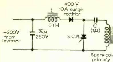
Fig. 1. Inductive charging circuit.
