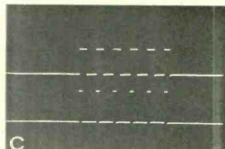
Fig. 1. (a) Output pulses with channel A delayed (vertical gain: 2V/div.; timebase: 10μ s/div.). (b) Rise time of both channels showing that time coincidence can be achieved (Vertical gain: 2V/div.; time base: 50ns/div.). (c) The action of the inhibit pulse (vertical gain: 2V/div.; timebase: 0.5ms/div.).
