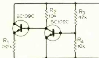
Transistor circuit operating as a tunnel diode.
