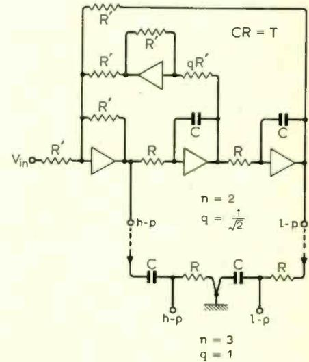
Fig. 7. Two-integrator system as crossover filter.
