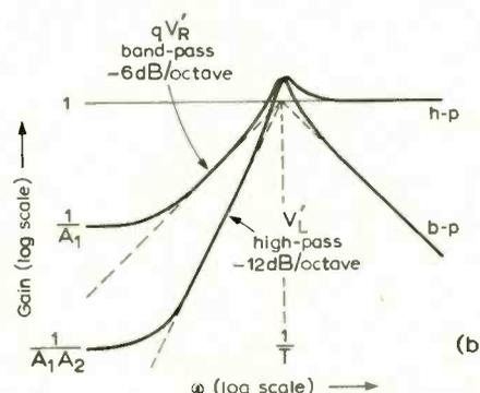
Fig. 4. (a) Equivalent circuit of system with finite-gain integrators. (b) Uncompensated responses.
