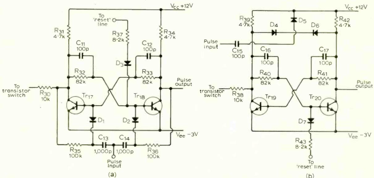
Fig. 4 (a). First bistable. Diodes are germanium types, e.g. OA81, OA91, IN914.  $Tr_{17}$  and  $Tr_{18}$  can be 2N3708, BC108, etc. (b). Circuit for remaining five bistables. Diodes and transistors as for first bistable.
