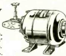
**Motor Driven Variable Voltage Transformers by Ohmite (U.S.A.).** Input 120/240v., 50/60 c.p.s. Output 0-240v. at 480 v.a. A reversible 115v. a.c. geared motor drives the contact sweep arm in the direction required. There is a micro switch mounted at each end of the track which is cam-operated and intended to be connected as a safety-stop. First class condition. £8.15.0. P. & P. 10/-.
