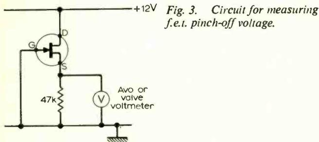
Fig. 3. Circuit for measuring f.e.t. pinch-off voltage.
