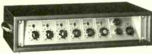
The MXT/6 series of Audio Mixer assemblies offer complete flexibility for pre-amplifier/mixing of microphones, gramophones, tape recorders, tuners, tone signal generators, etc. Utilising a modular construction any number of channels can be incorporated up to 14 in standard assemblies for cabinet or rack mounting.
