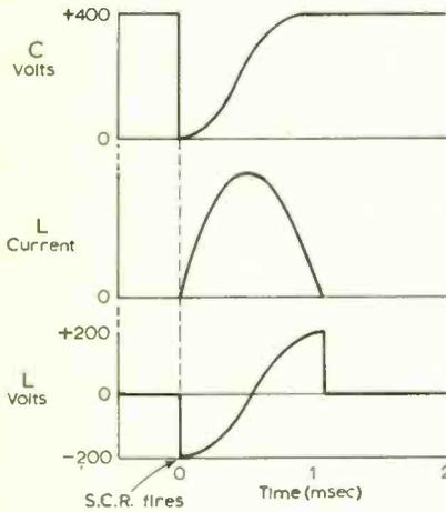
Fig. 2. Waveforms in above circuit.
