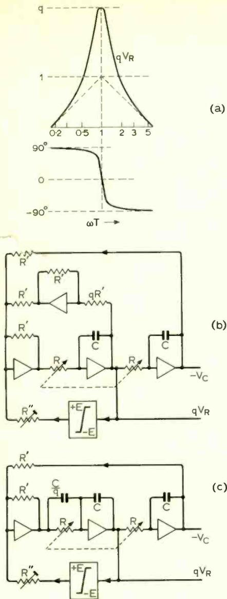
Fig. 8. Two-phase low-frequency oscillator.
