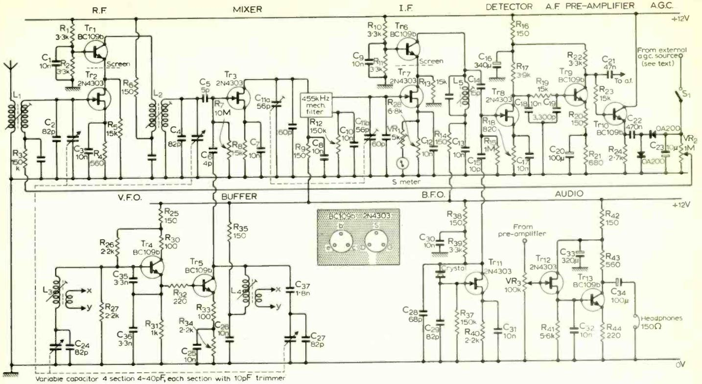
Fig. 2. The circuit. A power supply is not included in this description, but a car battery or almost any mains 12V power pack will suffice.
