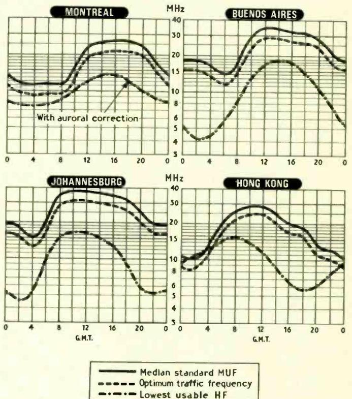
The charts show median standard MUF, optimum traffic frequency (FOT) and lowest usable frequency (LUF) for reception in this country. LUFs were calculated by Cable & Wireless Ltd for specific point-to-point telegraph circuits. LUFs for domestic reception of high-power broadcast transmissions would be slightly higher and those for the amateur bands considerably higher, especially during daylight.
