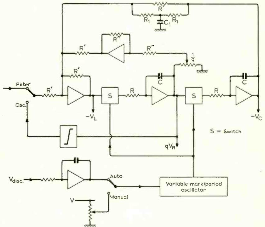
Fig. 12. Electronic tuning applied to a two-integrator system.
