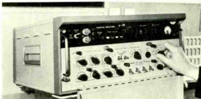
*The Omega navigation receiver fitted to the Q.E.2 which provides position fixing to an accuracy of two miles*
