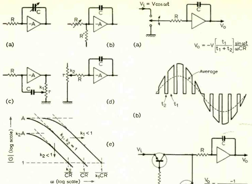
Fig. 10. Some methods of tuning an integrator.
