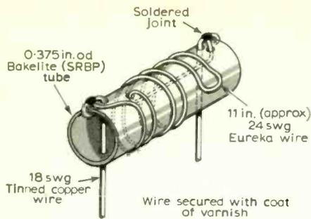
Fig. 6. Construction of 0.56 Ω 5% non-inductive resistors.
