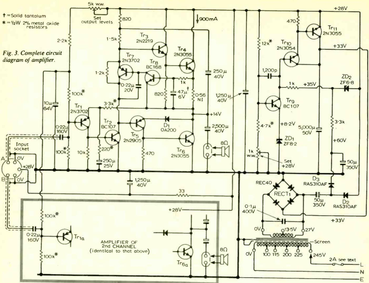
Fig. 3. Complete circuit diagram of amplifier.
