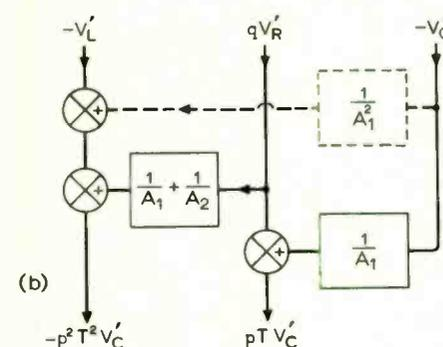
Fig. 3. (a) Analysis of system with finite-gain integrators. (b) Method of compensation.
