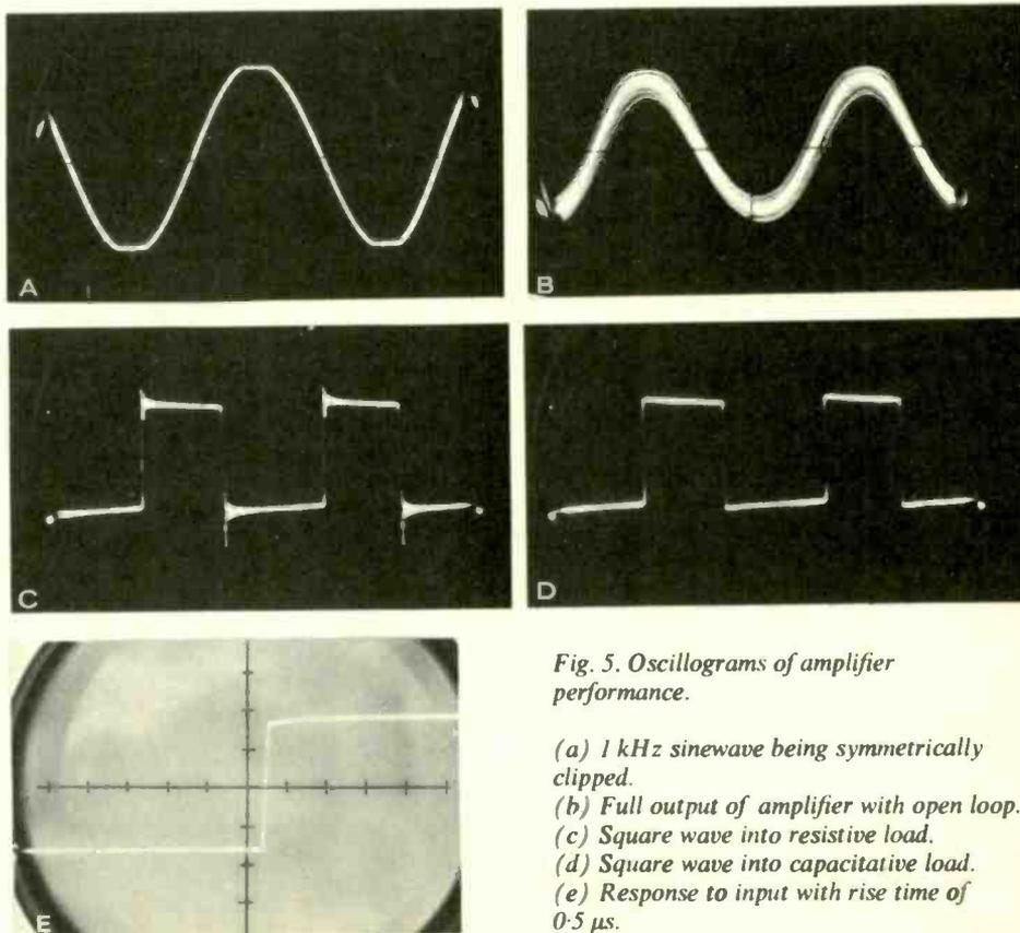
Fig. 5. Oscillograms of amplifier performance.
