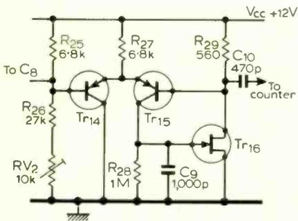
Fig. 3. Peak-level sensor circuit.  $Tr_{14}$  and  $Tr_{15}$  can be 2N3702 or 2N4289; and  $Tr_{16}$ —TIS43 or 2N2646.
