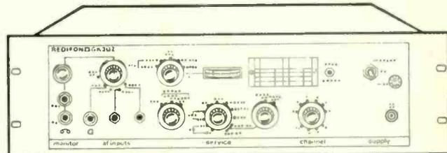
GK.202. 10-channel drive unit for frequency and service generation, 1.5-30 MHz. 17 modes of transmission, including ISB if required.
