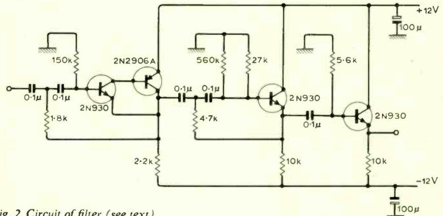
Fig. 2. Circuit of filter (see text).
