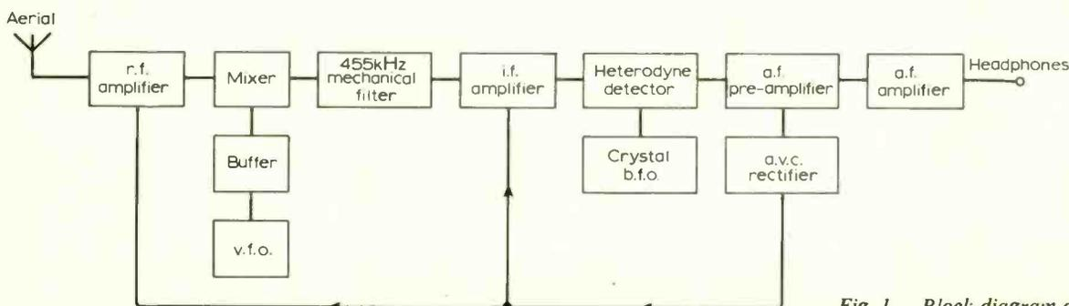
Fig. 1. Block diagram of the complete receiver.
