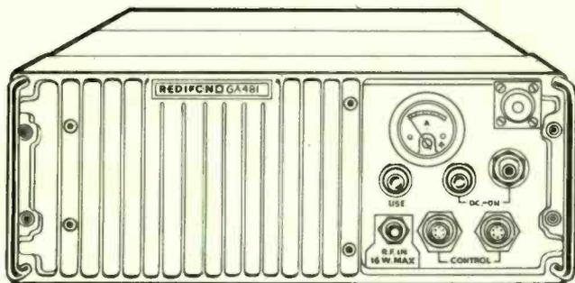
GA.481. 100-watt linear amplifier, broad-band 1.5-30 MHz. No tuning or loading. Automatic protection against any mismatch (from open- or short-circuit aerial) or excessive drive. Easily portable, will operate direct from vehicle supply.
