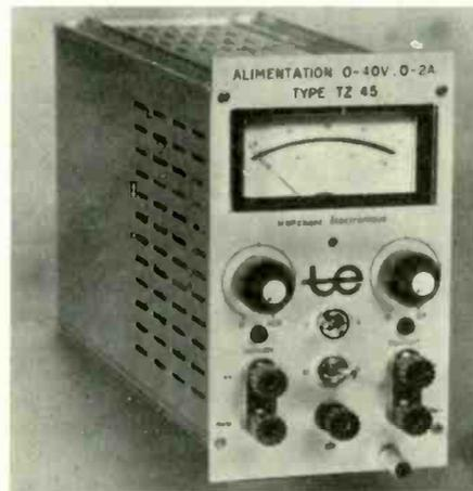
and fine adjustment controls. Unit measures 4 $\times$ 7 $\times$ 11 $\frac{1}{2}$ in. An over-voltage crowbar with operating time of less than 20 $\mu$ s, operating temperature range of 0-60 $^{\circ}$ C, ripple 300 $\mu$ V r.m.s. and load and line regulation 1 part in 10,000 is available as an optional extra. Tranchant Electronics (U.K.) Ltd, 17 Charing Cross Road, London. W.C.2.
