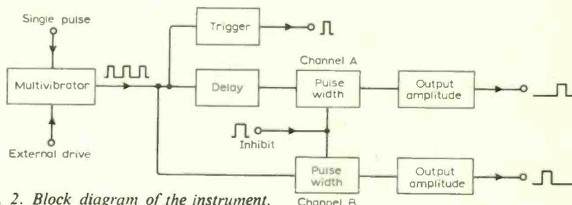
Fig. 2. Block diagram of the instrument.
