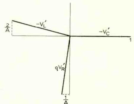
Fig. 2. Relative phases of three primary responses at  $\omega_c$ .
