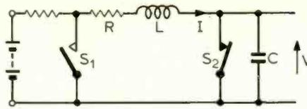
Fig. 2. The circuit of Fig. 1, with resistance added.
