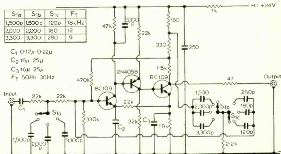
Low-pass and high-pass filter circuit.
