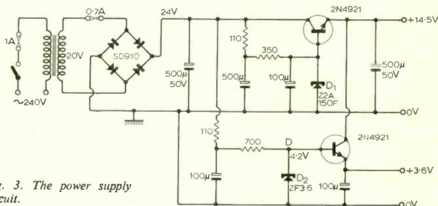
Fig. 3. The power supply circuit.
