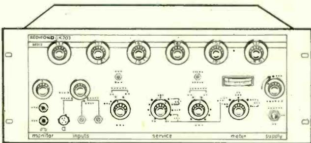
GK.203. Frequency synthesis drive unit. 1.5-30 MHz in 100 Hz increments. 17 modes of transmission, including ISB if specified.
