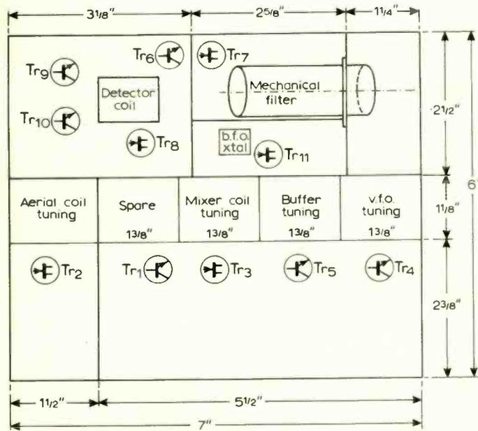
Fig. 4. Skeleton mechanical layout showing position of main components.
