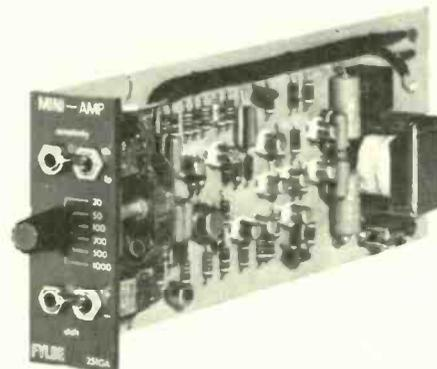
Output capability is  $\pm 8\text{V}$  at up to 1.5mA and common mode rejection is greater than 100dB. Full shift of the output is possible, and wideband noise is less than 10mV pk-pk, referred to output. Bandwidth may be adjusted, from d.c. to between 100Hz and 100kHz. A monolithic input stage produces drift performance better than  $5\mu\text{V}/^\circ\text{C}$ , referred to input. Fylde Electronic Laboratories Ltd, 6/16 Oakham Court, Preston, PR1 3XP.
