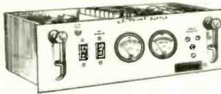
Regulation between 7-15 volts D.C. at 20 amps. Fitted 0-30 D.C. ammeter, 0-15 D.C. voltmeter and overload protection switch. Built to a very high specification. Bench or rack mounting. Size 19 x 8 x 17 ins. A.C. input 110v. 50 cycles. Ex equipment but guaranteed in perfect condition. Maker's price in excess of £200. Our price £29.10.0. Carr. 30/- 240/110 volt, 400 watts, Mains Transformer available if required. £3 extra
