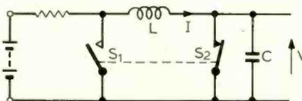
Fig. 1. At  $t = 0$ ,  $S_1$  is closed and  $S_2$  opened.
