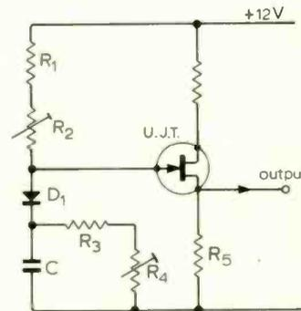
Modified unijunction transistor oscillator.
