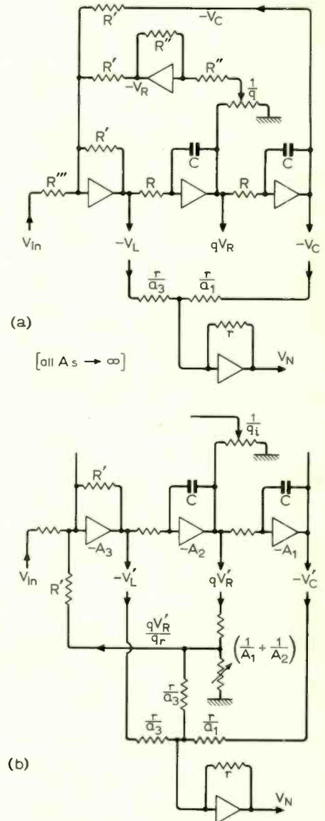
Fig. 1. (a) Ideal two-integrator system. (b) Showing a method of correcting  $Q$  factor and notch response when integrators have finite gain.
