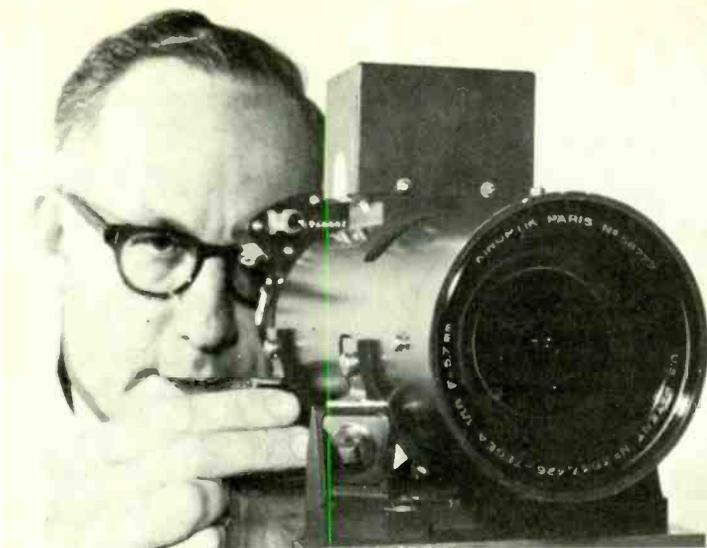
*One of the TV cameras used in the satellite TIROS-M which is now providing weather information for the world's meteorological centres. TIROS-M was built by R.C.A. under the direction of N.A.S.A.'s Goddard Space Flight Centre*
