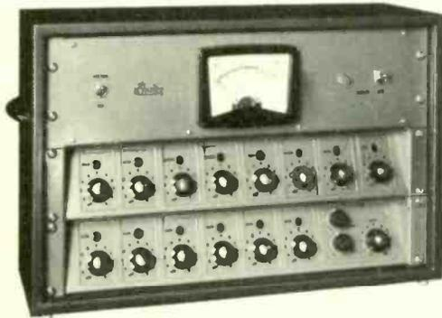
The combiner unit mixes the module outputs and amplifies the composite signal to drive either power amplifiers or 600Ω output stage. A master gain control and treble and bass controls are provided. Power requirements are modest and a typical 6 way assembly requires only 15mA at 12v DC.
