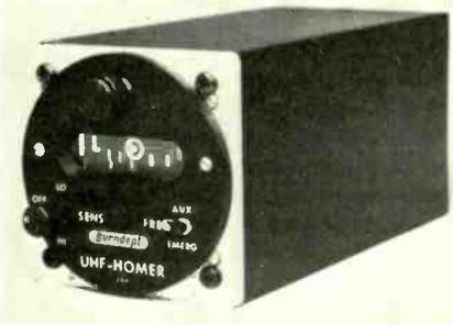
operation, the emergency channel is preset to the v.h.f. or u.h.f. international aviation distress frequency; an auxiliary channel can be used to within  $\pm 2.5$ MHz (v.h.f.) or  $\pm 5$ MHz (u.h.f.) for training and/or tactical purposes. The homer provides 'left/right' indications from the received signal. Audio outputs to the aircraft intercom system are provided. The unit costs under £500, plus installation. Burndept Electronics (E.R.) Ltd, St. Fidelis Road, Erith, Kent.
