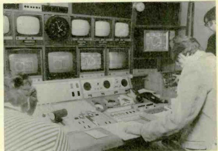
The master control desk at Thames Television's new centre in Euston is boomerang-shaped and has positions for the lines engineer (top left), the engineer in charge who performs a quality control function (top right), and the network switcher (bottom left). The monitor bank facing the desk has a row of 14-in. monochrome monitors and a row of colour monitors underneath. These preview incoming sources, check the passage of signals
