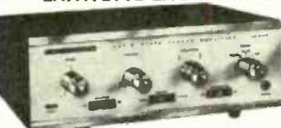
19 transistors, 8 diodes. I.H.F music power 30 watts at 8 ohms. Res. 30-20,000 ±2 dB at 1 w. Distortion 1% or less. Inputs 3 mV and 250 mV. Output 3-16 ohms. Separate L and R volume controls. Treble and bass controls. Stereo phone jack. Brushed aluminium, gold anodised extruded front panel with metal case. Size 10 1/2 in. x 3 1/2 in. x 7 1/2 in. Operation 115/230 volt A.C. £28. Carr. 7/6.
