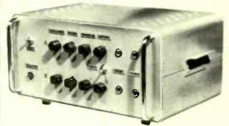
The March issue of Practical Electronics presents a wonderful new series showing you how to construct your own high power solid state audio amplifier. It's a twin channel 50 plus 50 watt design with a hi-fi specification and all purpose capability ranging from paging and public address to instrumental and other forms of music reproduction systems.
