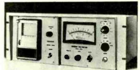
low frequency and where unwanted high-frequency noise is present. Voltage ranges are 0.3, 30, 100, 1000V to 30kV with optional probes. Input impedance is 10MΩ to 30kΩ depending on the range and accuracy ±3% of full scale. Sintrom Electronics Ltd, 2 Castle Hill Terrace, Maidenhead, Berks.
