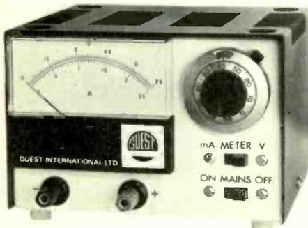
ability. A built-in meter enables the output voltage or current to be monitored. Ripple noise is less than 0.5mV pk-pk and overload protection limits the output current to 110% of maximum. Reset is automatic. The model 606 is available in current ranges from 0-500mA up to 0-2.5A. Dimensions are 156 × 152 × 102mm and prices from £34 15s to £42 15s. Guest International Ltd, Nicholas House, Brigstock Road, Thornton Heath, Surrey.
