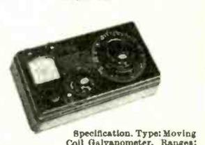
Specification. Type: Moving Coil Galvanometer. Ranges: 1. 0.05 to 5 ohms. 2. 0.5 to 50 ohms. 3. 5 to 500 ohms. 4. 50 to 5,000 ohms. 5. 500 to 50,000 ohms. Scales: Switched. Slidewire: 0.5 to 50. Galvanometer Scale: 10-0-10. Case: Moulded plastic. Internal Source: 4V. Dry battery. Dimensions: 200 x 110 x 65mm. Weight: 0.9 kg. List price £25. Our price £29/19/6.
