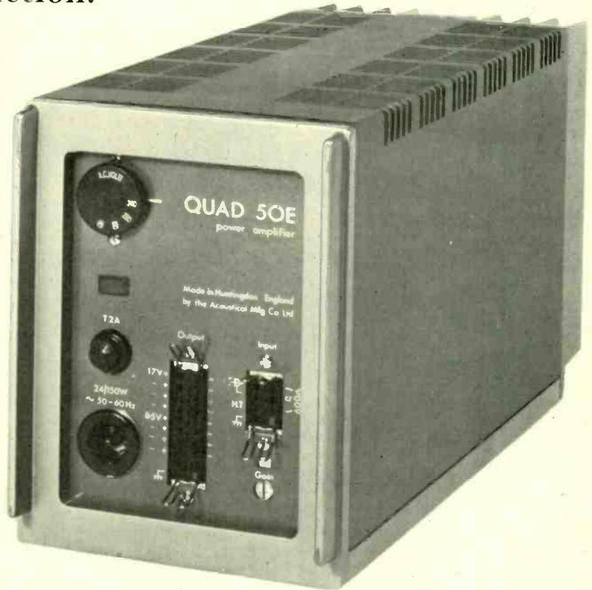
**INPUTS** - 0.5 Vrms unbalanced with provision for an optional plug-in transformer for bridging 600 ohms lines.
