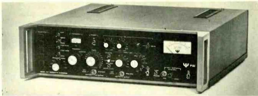
This carrier servo generator introduced by Prosser Scientific Instruments has a frequency range of 0.0008Hz to 200kHz and provides a two phase modulated output.
