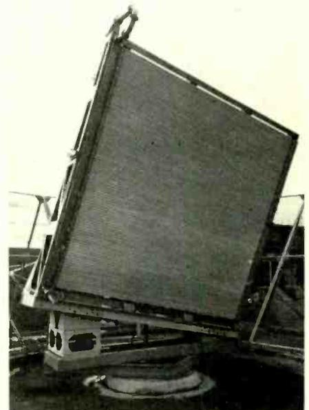
Fig. 9. Three-dimensional air surveillance radar aerial.
