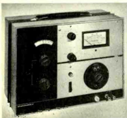
external. This can be measured in three ranges without the need for an external voltmeter. Frequency range is 86-108MHz with  $\pm 0.5\%$  accuracy. Output is 0.1-100,000 $\mu$ V and modulation 400, 1,000 and 10,000Hz (internal). Deviation is in three metered ranges of 0-30kHz, 0-100kHz and 0-300kHz, and deviation response is within 1dB from d.c. to 75kHz. Wessex Electronics Ltd, Royal London Buildings, Baldwin Street, Bristol 1.
