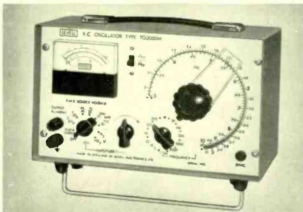
One of the Levell TG200 series of RC oscillators covering 1Hz to 1MHz in 12 ranges.
