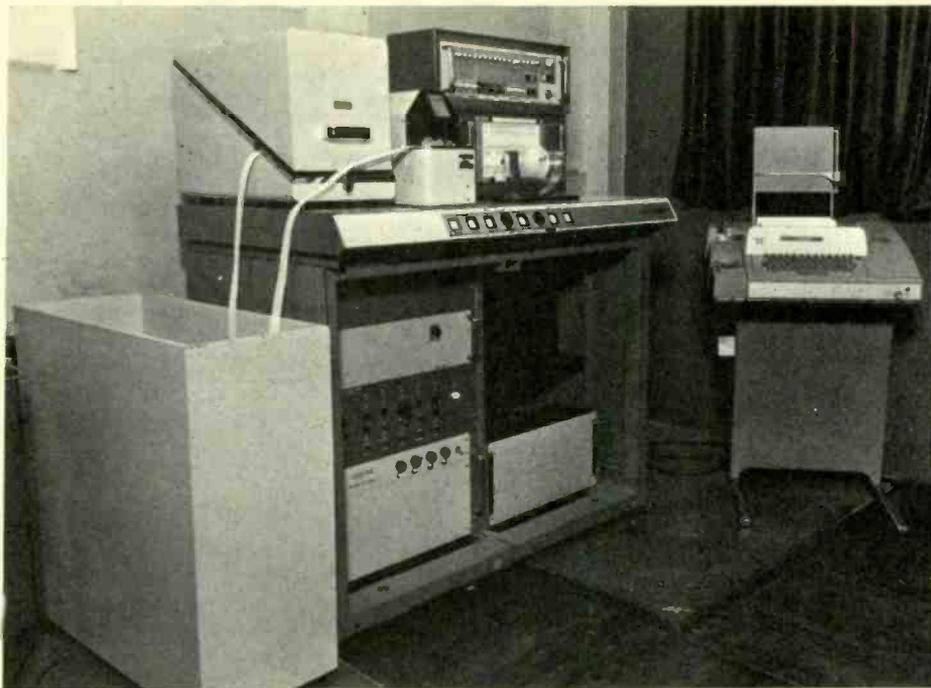
Fig. 10. The Elliott computer installation used in the track-while-scan system. The 920M micro-miniature computer employs a 16k word store.
