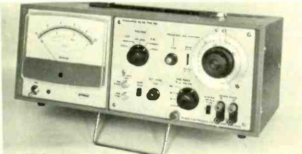
Dymar modulation meter, type 785, for narrow deviation mobile v.h.f. and u.h.f. radio telephone transmissions.
