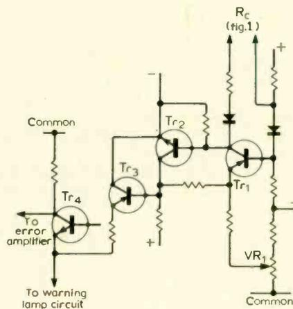
Fig. 4. Simplified current limit circuit.
