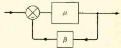
Fig. 13. Standard diagram of feedback loop.
