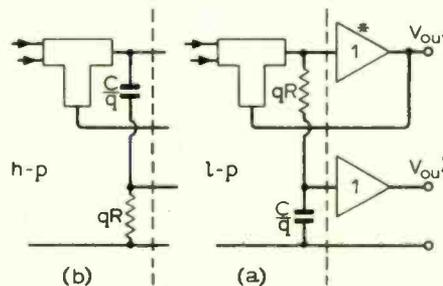
Fig. 2. Use of damping branch to give 3rd-order response.
