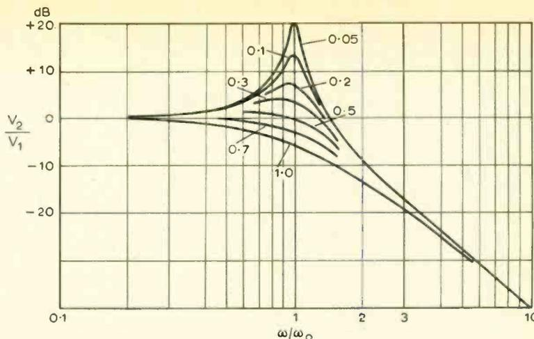
Fig. 10(a).  $\frac{V_2}{V_1} = \frac{P_1 P_2}{(p-p_1)(p-p_2)}$  for various values of  $1/2Q_0$ .
