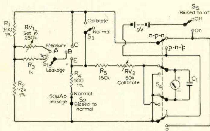
Fig. 3. Complete circuit diagram.
