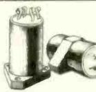
**DIAMOND "H" SEALED RELAY Type BR 115 C.I.T.**—IC 26v. 150Ω 4 P.D.T. Completely encapsulated in heavy gauge brass case, glass sealed terminals, very robust. 17/6 each.
