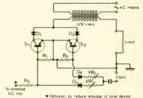
Control circuit with low power dissipation when off.
