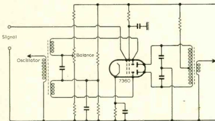
*Fig. 9. Balanced mixer using 7360 beam deflection valve can provide low-noise and extremely wide dynamic range.*
