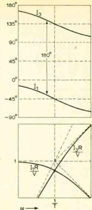
Fig. 7. Phase and amplitude plots when  $T_2' = T_2$ .
