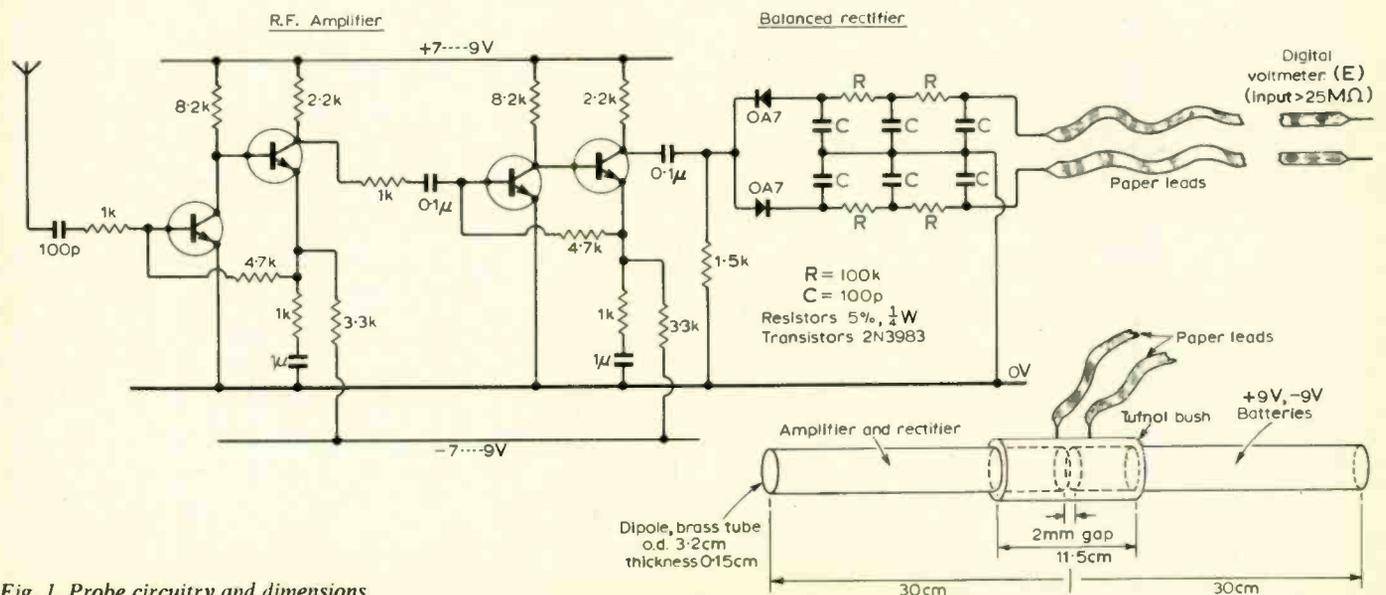
Fig. 1. Probe circuitry and dimensions.
