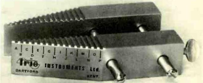
An easily adjusted hand tool for the accurate bending of resistor, capacitor, diode leads, etc., for printed circuits. Will bend leads to within 1/16" of ends of components and up to 3 1/4" centres.
