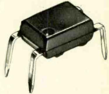
be used either as a general-purpose a.f. amplifier or as an i.f. amplifier at 465kHz. Typical output noise is 1mV r.m.s. Maximum power supply potential is 18V and typical current drain is 3mA. This i.c. contains three transistors and five resistors. Motorola Semiconductors Ltd, York House, Empire Way, Wembley, Middx.
