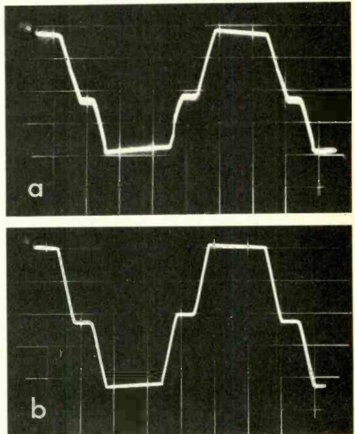
Fig. 4. Amplifier performance using 10kHz test waveform. (a) Response of amplifier showing inadequate stability with reactive load. (b) Response of improved amplifier with reactive load.
