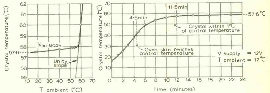
Fig. 5. Warm-up curves for the oven, obtained with a calibrated thermistor.
