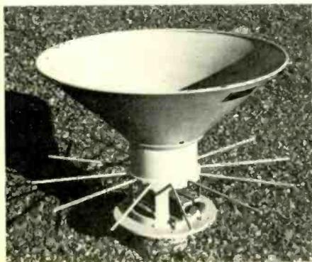
vertex of the cone for structural strength and waterproofing. It is supplied with a base flange for mounting. The frequency range is 250-1000MHz, radiation pattern omnidirectional, input impedance  $50\Omega$ , input power 750W, and weight 4kg. Microwave International (U.K.) Ltd., 33-37 Cowleaze Road, Kingston upon Thames, Surrey. WW 304 for further details
