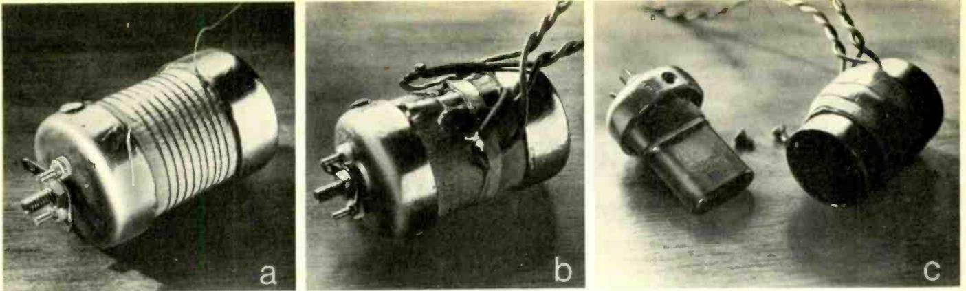
Fig. 4. (a) The oven with the heater winding in place over the insulating paper tape. (b) The heater and thermistor in place, with connecting wires attached. (c) Completed oven, opened to show the crystal in position in its socket.
