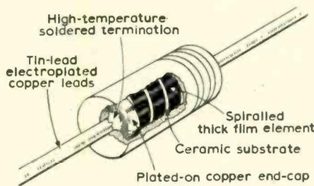
Fig. 1. The construction of a metal glaze resistor.
