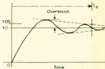
Fig. 11. Response of second order circuit to a step input.
