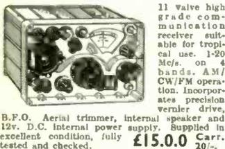
11 valve high grade communication receiver suitable for tropical use. 1-20 Mc/s. on 4 bands. AM/CW/FM operation. Incorporates precision vernier drive, B.F.O. Aerial trimmer, internal speaker and 12v. D.C. internal power supply. Supplied in excellent condition, fully tested and checked. £15.00 Carr. 20/-.
