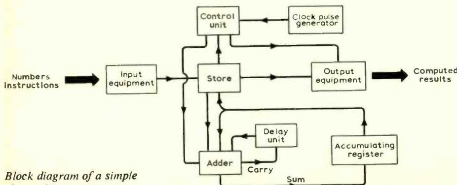
Block diagram of a simple electronic computer.
