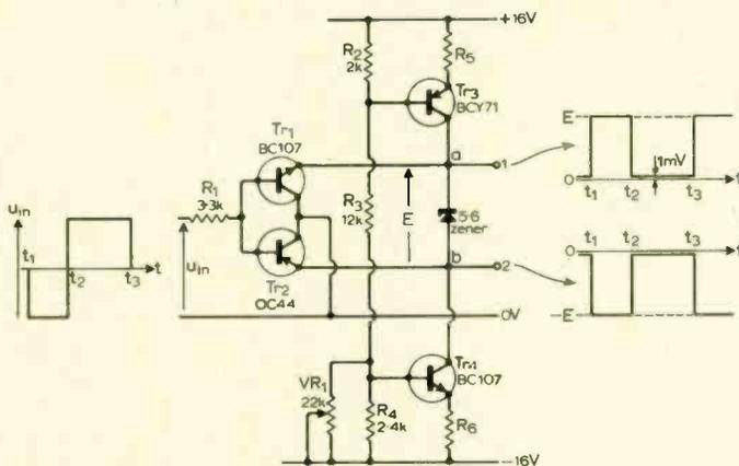
Fig. 1. Circuit of complementary pulse generator.
