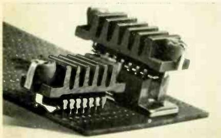
ensure good thermal contact between the sink and the module. The DIP14/1 and DIP14/4 are rated at 30°C and 28°C per watt respectively. Redpoint Ltd, Lynton Road, Cheney Manor, Swindon, Wilts.
