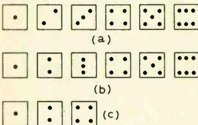
Fig. 1. (a) Classical dice patterns; (b) amended dice patterns; (c) the three patterns required to form (b).
