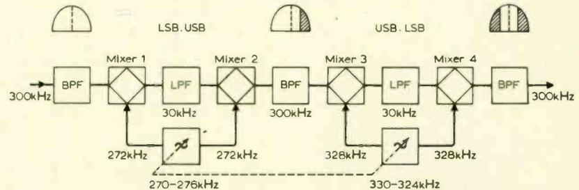
Fig. 8. Rohde & Schwarz variable-bandwidth i.f. filter shown set for ±2kHz bandwidth.
