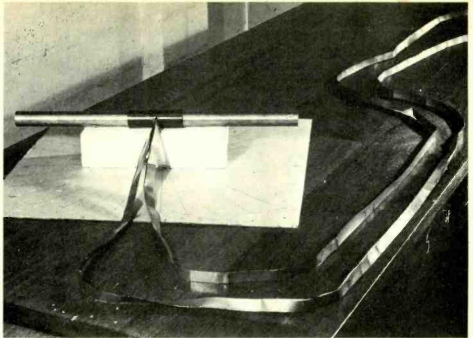
Fig. 5. The probe with its "paper" leads ( $\theta = 270^\circ$ ). The assistance given by J. Bruce in constructing the probe is gratefully acknowledged.
