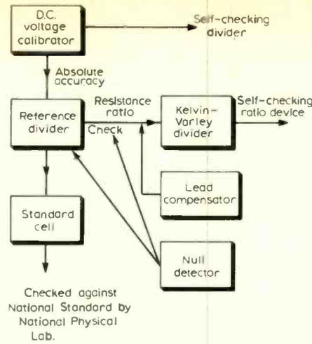
Fig. 9. Tracing measurement to the national standard of voltage.
