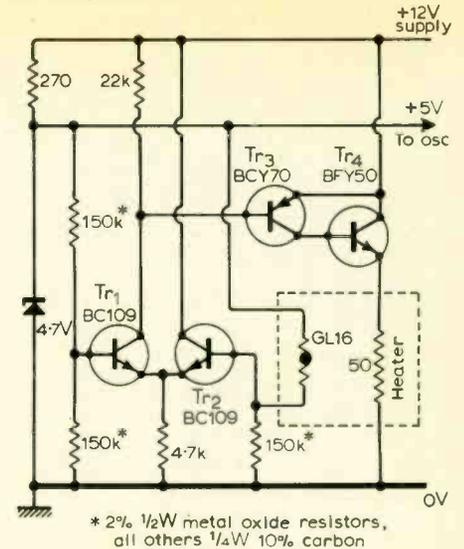
Fig. 1. Initial experimental temperature control circuit for the crystal oven.
