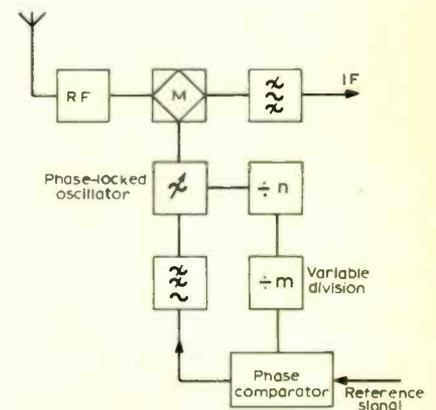
Fig. 5. Phase-locked synthesizer using digital techniques.
