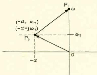
Fig. 5. One root and its effect for sinusoidal excitation.
