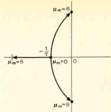
Fig. 12. Movement of three roots.
