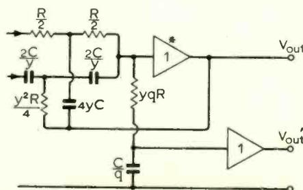
Fig. 3. Network in which  $T_1 \neq T_2$ .
