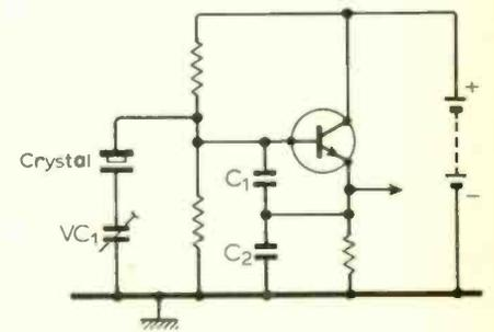
Fig. 6. Basic circuit of the oscillator.
