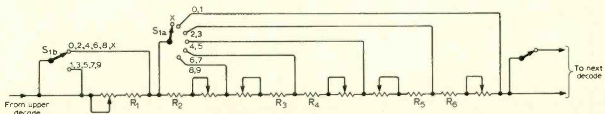
Fig. 2. Typical decade—voltage control feedback resistor.
