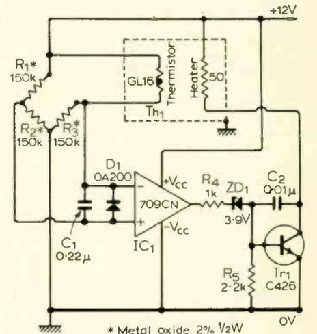
Fig. 2. Temperature control circuit actually used. Improved performance is obtained because of the higher loop gain.
