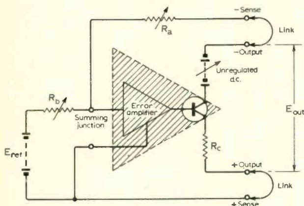
Fig. 1 (left). Voltage control block diagram—voltage calibrator.
