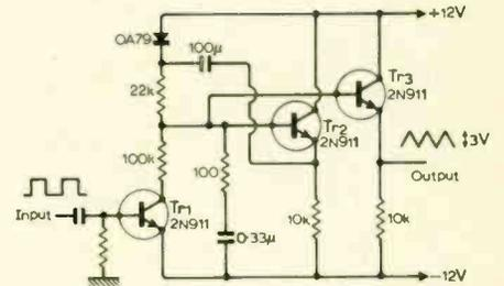
Generator circuit with charge time equal to flyback time.
