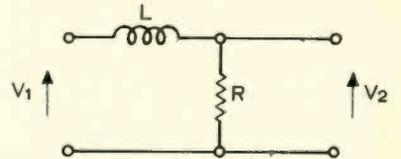
Fig. 7. The simple LR circuit, which has only one root.
