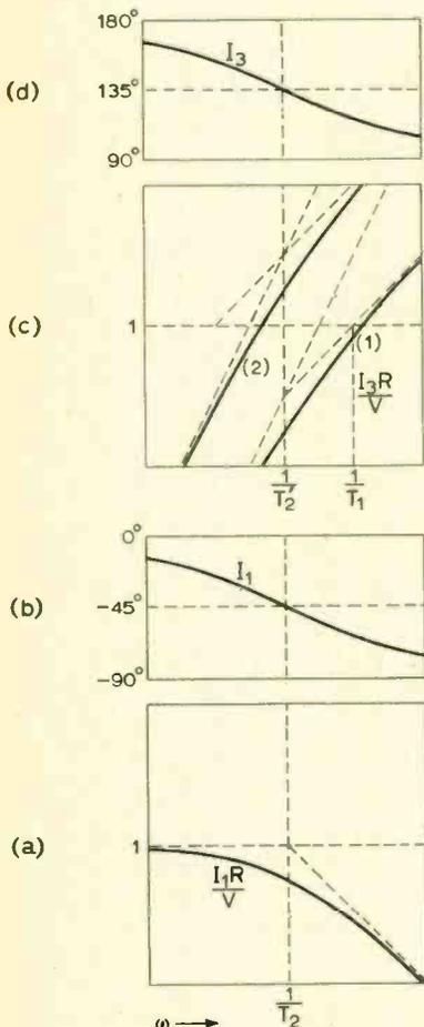
Fig. 6. Phase and amplitude plots of the short-circuit output currents of the two tees for constant input voltage.
