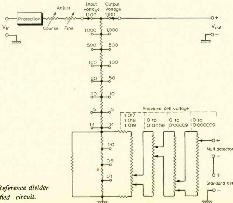
Fig. 6. Reference divider—simplified circuit.
