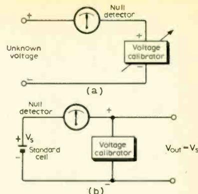
Fig. 5. Voltage calibrator and null detector used as (a) high resolution differential voltmeter (b) power standard cell.
