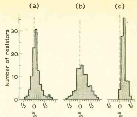
Fig. 3. Typical test results showing the percentage change of resistance for given conditions. (a) Conditions as per DEF5115/RFG5F at rated volts at  $70^\circ\text{C}$  for 2000 hours; spec. limit  $\pm 3\%$ . (b) Same conditions as (a) but for 10,000 hours. (c) Tropical exposure with light load for 1,344 hrs; spec. limit  $\pm 1\%$ .
