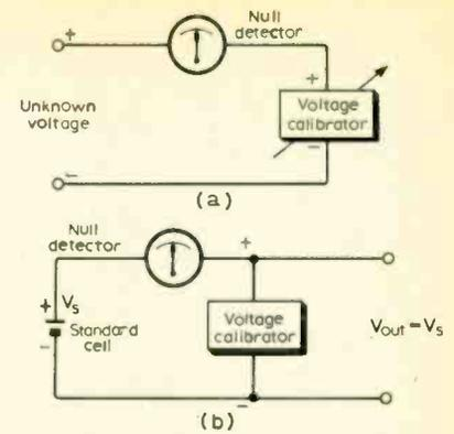
Fig. 5. Voltage calibrator and null detector used as (a) high resolution differential voltmeter (b) power standard cell.
