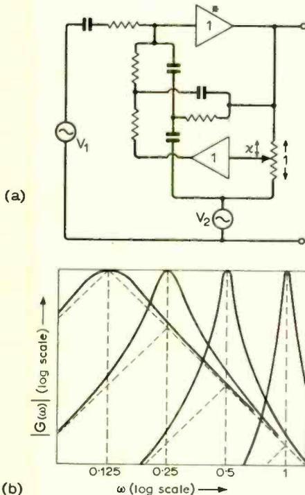
Fig. 1. Use of a potentiometer to give variable tuning with constant bandwidth.
