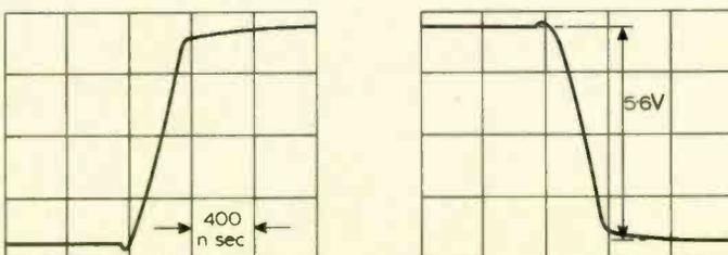
Fig. 2. Rise and fall times of the circuit.
