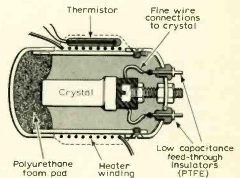
Fig. 3. Cross-sectional diagram of construction of the oven.
