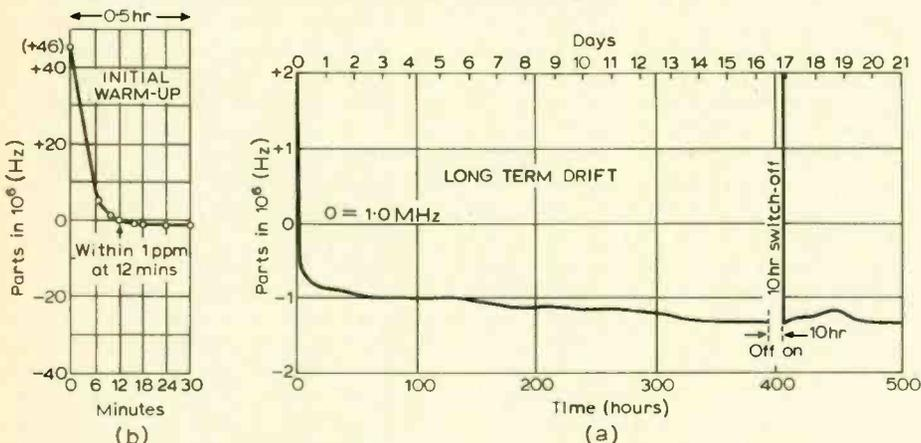
Fig. 8. Results of a 500-hour frequency drift test on the frequency standard (a), showing in detail the initial warm-up phase (b).
