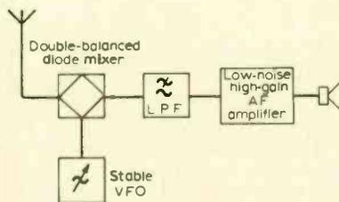
Fig. 13. Basic outline of simple homodyne (direct conversion) receiver for s.s.b./c.w. reception.
