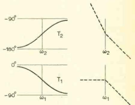
Fig. 14. Phase and asymptotic gain diagrams for the two portions of the loop.
