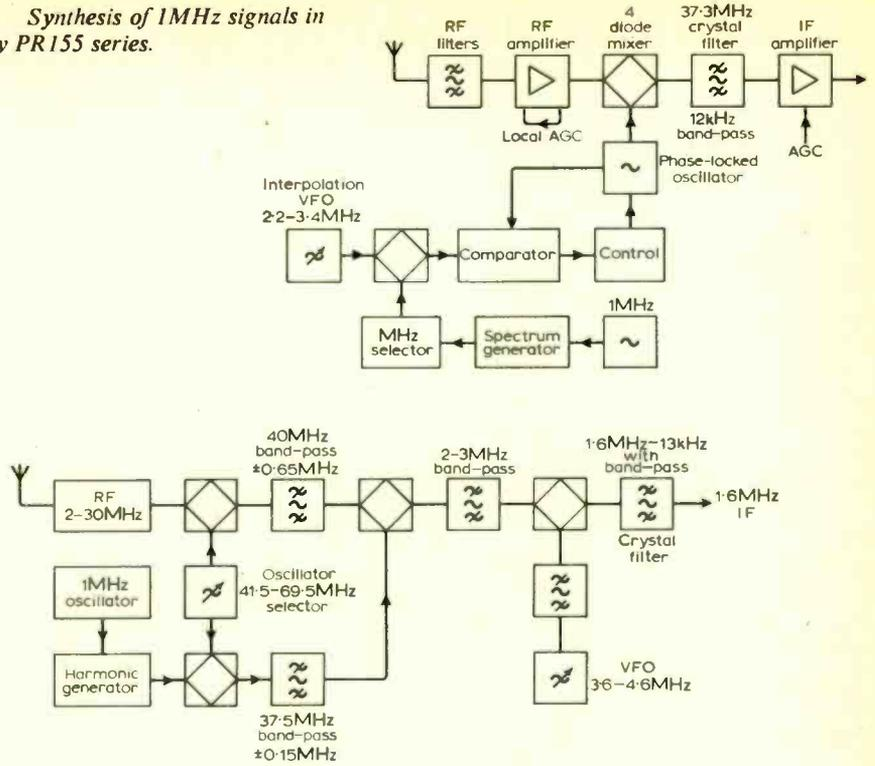
Fig. 4. Wadley drift-cancelling loop technique as used in many Racal receivers.
