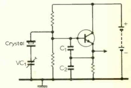
Fig. 6. Basic circuit of the oscillator.
