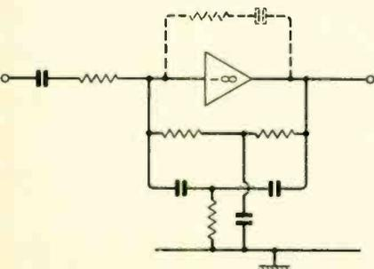
Fig. 11. Parallel-T selective amplifier.
