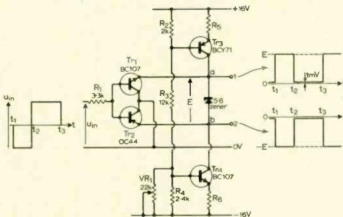
Fig. 1. Circuit of complementary pulse generator.
