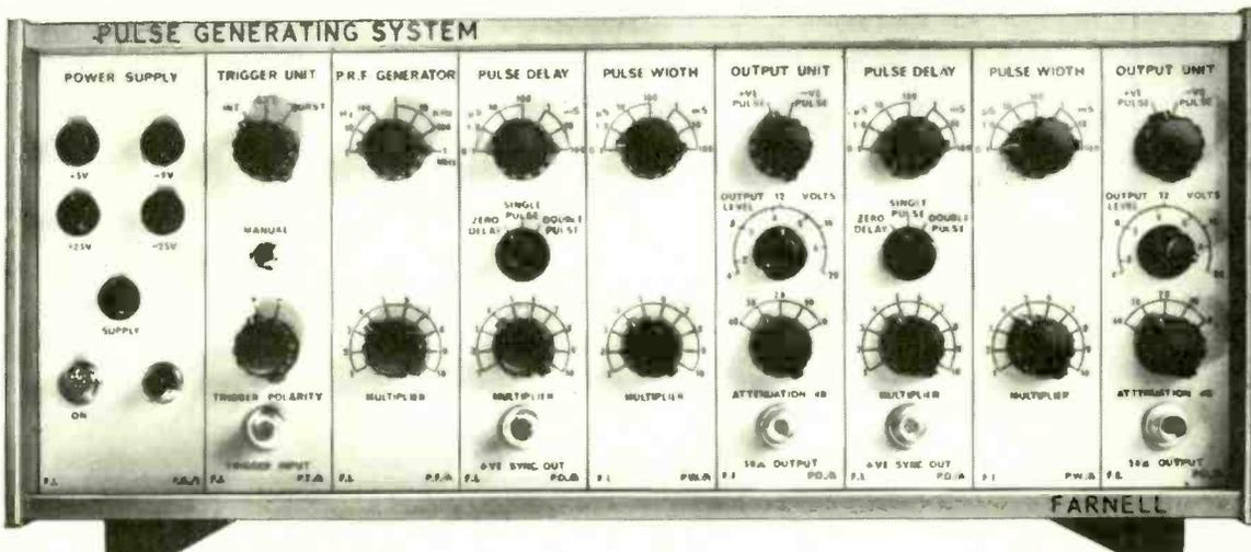
\* SINGLE OR DOUBLE PULSE OUTPUT \* TRUE DOUBLE PULSE OPERATION with independent control of output width, delay, amplitude and polarity. \* RISE TIME 10 NANOSECONDS. \* MAXIMUM PULSE AMPLITUDE is 20V into 'open circuit', or 10V into 50Ω \* PRICES FROM £118.
