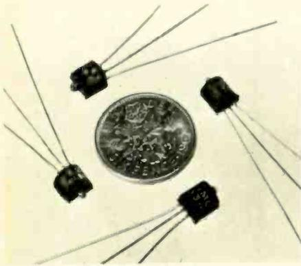
dimensions of 5mm. The circuit contains one transistor, one diode and two resistors and is designed to operate from a 5-V 4-mA supply. It indicates logic states of "0" (0.5V lamp off) and "1" (2.5V lamp on) with input currents of  $5\mu\text{A}$  and  $30\mu\text{A}$  respectively. Newmarket Transistors Ltd, Exning Road, Newmarket, Suffolk.
