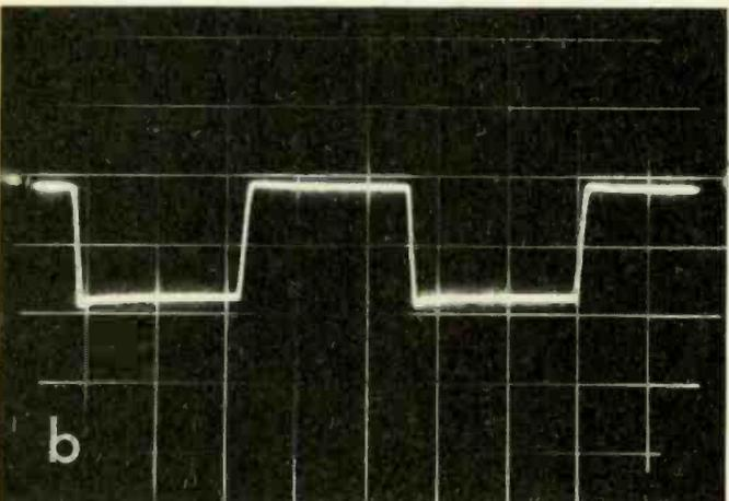
Fig. 5. Amplifier response driving a reactive load ( $15\ \Omega$ ,  $0.47\ \mu\text{F}$ ) with a  $10\text{kHz}$  square wave. (a) The ringing gives evidence of instability. (b) No transient ring indicates better stability.
