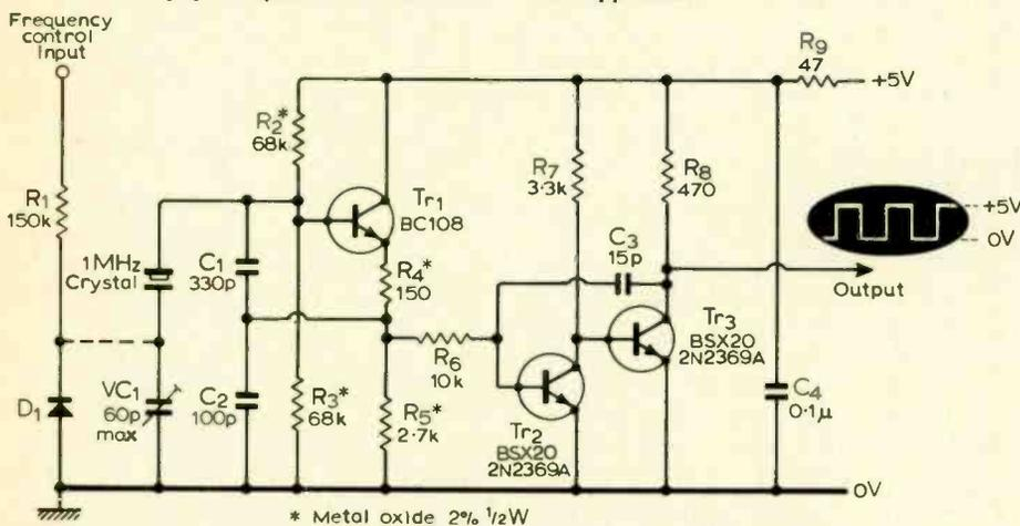
Fig. 7. Complete circuit of the 1MHz oscillator. The final two transistors form a shaping circuit to provide the required square-wave output.
