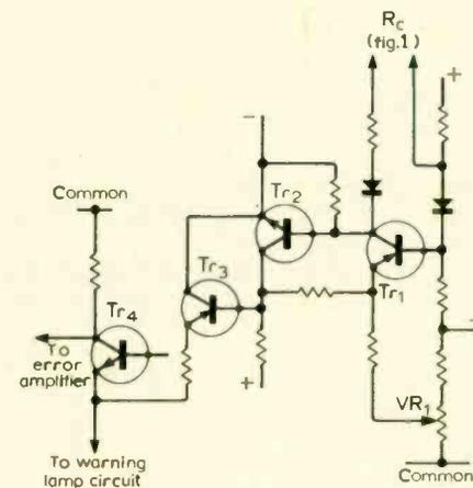
Fig. 4. Simplified current limit circuit.
