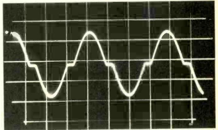
Fig. 3. Test waveform for providing arrested transient input.
