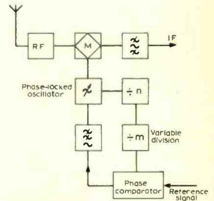
Fig. 5. Phase-locked synthesizer using digital techniques.
