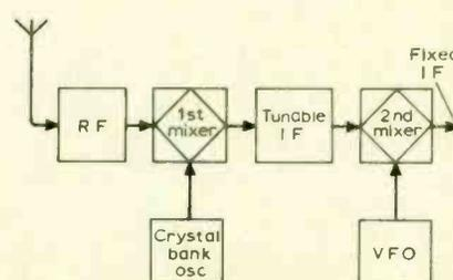
Fig. 2 Multi-conversion superhet having crystal-controlled first oscillator.
