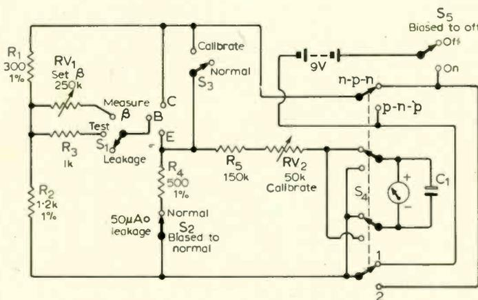
Fig. 3. Complete circuit diagram.
