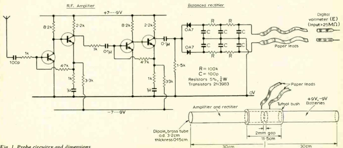
Fig. 1. Probe circuitry and dimensions.
