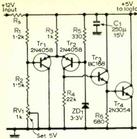
Fig. 9. Circuit of +5V shunt stabilizer for oscillator supply and for d.t.l. or t.t.l. logic of a counter-timer.
