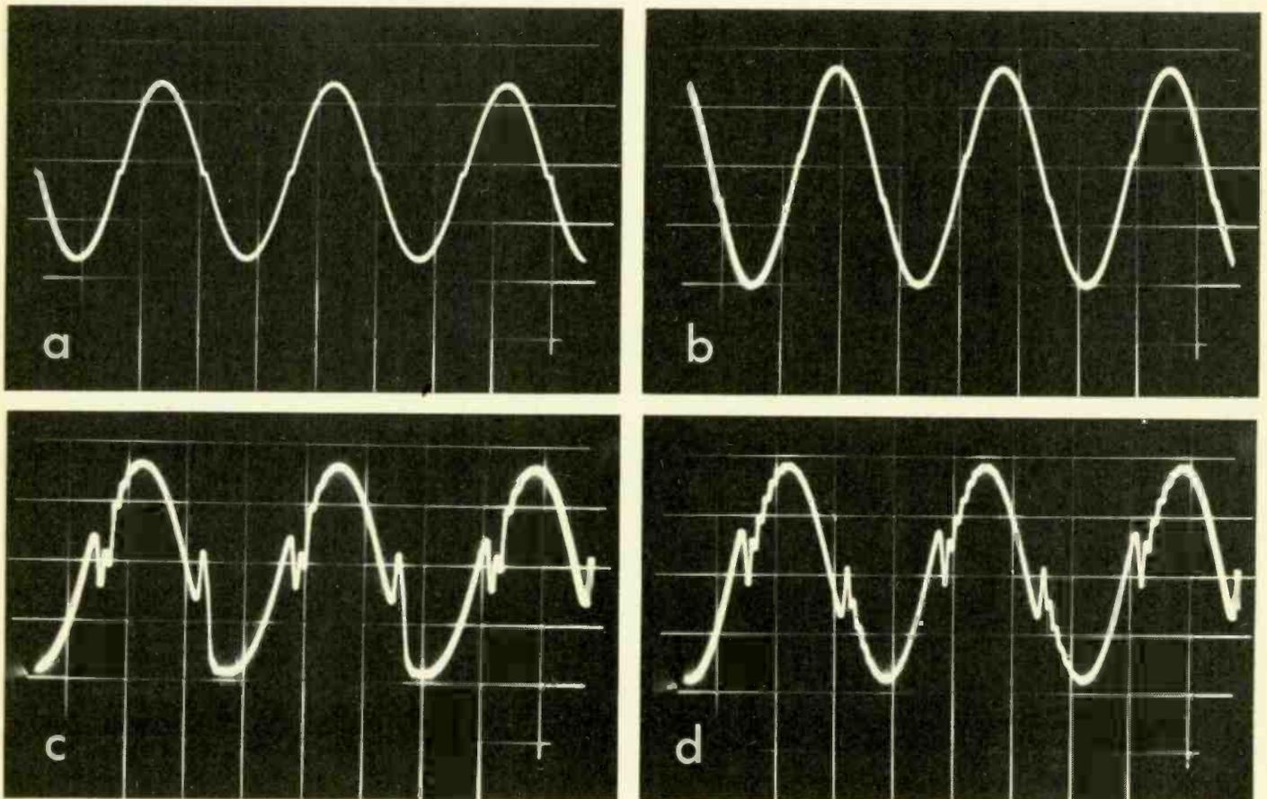
Fig. 1. Crossover distortion in a class B stage employing transistors with an  $f_T$  of about 2MHz. (a) Low frequency sine wave at 10mA. (b) High frequency sine wave showing the effect of hole storage on the crossover discontinuity under light load conditions. (c) Influence of hole storage and n-p-n/p-n-p asymmetry under high current conditions at 200kHz. (d) Improvement of conditions in (c) by reducing source impedance.
