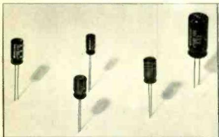
are fitted with insulating sleeves which, together with the single-ended design, allow close arrangement on printed circuit boards. Temperature rating is from  $-25^{\circ}$  to  $+85^{\circ}$ C. ITT Components Group Europe, Capacitor Product Division, Brixham Road, Paignton, Devon.
