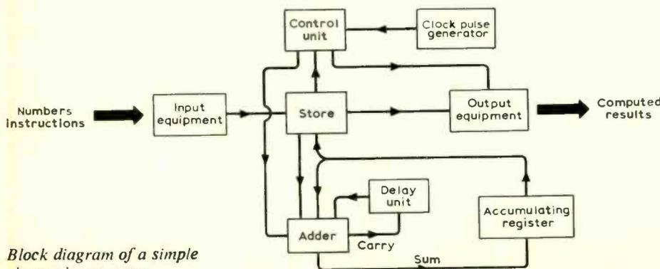
Block diagram of a simple electronic computer.
