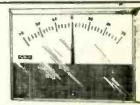
**Ernest Turner 5" x 4" 0-1 Ma. meter** calibrated 0-10 in 50 divisions mirrored scale, handsome chrome escutcheon for flush mounting. A quality instrument. £6.10.0.
