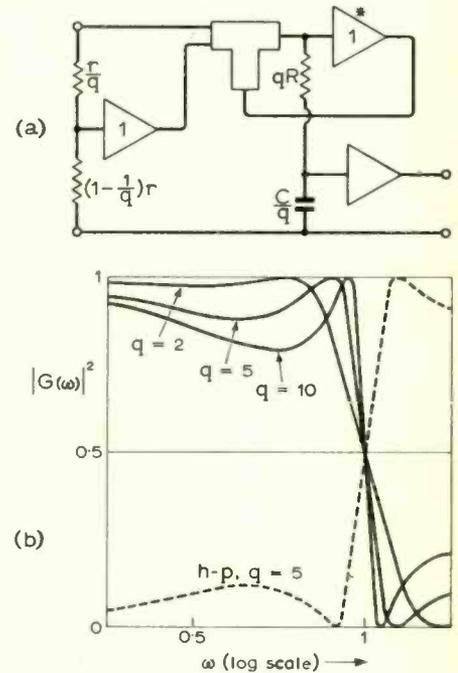
Fig. 4. 3rd-order responses obtainable from active parallel-T system. Note linear power scale.
