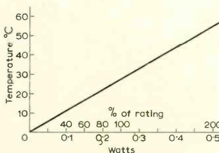
Fig. 2. Typical temperature rise with power dissipation for the RGO7 resistor.
