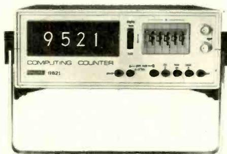
puting counter is expected to find wide application in the process control industry where it can provide accurate indication of gallons per minute, r.p.m. or similar parameters. Capabilities include frequency measurement (5Hz-10MHz) on either of two channels, frequency ratio, time interval and totalize. Racal Instruments Ltd, Duke Street, Windsor, Berks.
