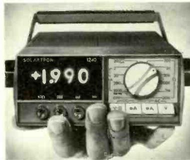
type LM1240. The new instrument has 26 ranges and is capable of measuring a.c. and d.c. voltage and current, and resistance. It is priced at £195 and is claimed to incorporate features regarded as standard in high-priced d.v.m.s. These include automatic polarity, high input resistance, an integration technique to
