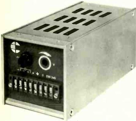
line regulation of 0.01%+1mV; load regulation of 0.03%+3mV (0 to full load); 1.5mV ripple voltage; re-entrant protection; input a.c. voltages of 220 or 240V a.c.  $\pm 10\%$ , with a frequency range of 45 to 400Hz; a temperature coefficient of 0.02%+2mV per  $^{\circ}\text{C}$ ; and nominal d.c. outputs variable  $\pm 10\%$ .
