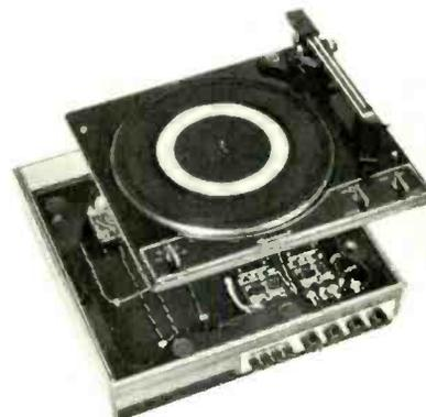
The illustration here shows quite clearly how easily Project 60 can be contained in one of today's slim, modern plinths. Very little space is required to house these Sinclair units, and within the space of the motor plinth, you can install a stereo amplifier of the very highest quality. If, for example you have already put together an assembly as illustrated here, adding the Active Filter Unit would be very easy.
