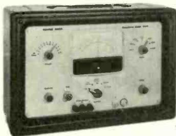
**Autobalance Capacitance Bridge** gives direct readout from 0.1pF to 10 $\mu$ F and will follow a changing value. Comprehensive facilities for 'zero suppression' and comparative measurements. Analog voltage and current outputs. Accuracy 0.25%. Internal 1kHz source, detector. A.C. or battery operation.
