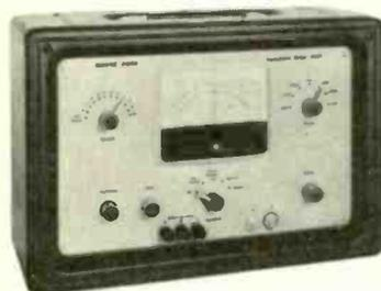
**Autobalance Capacitance Bridge** gives direct readout from 0.1pF to 10μF and will follow a changing value. Comprehensive facilities for 'zero suppression' and comparative measurements. Analog voltage and current outputs. Accuracy 0.25%. Internal 1kHz source/detector. A.C. or battery operation.
