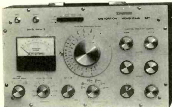
A sensitive instrument for the measurement of total harmonic distortion, designed for speedy and accurate use. Capable of measuring distortion products as low as 0.002%. Direct reading from calibrated meter scale.
