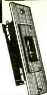
**NEW HYSTERESIS MOTORS BY WALTER JONES.** Type 14050/12, 240v. 50 c/s 1500 RPM cont. rating, output 2.0 oz./in. Size: Length (less spindle)  $3\frac{1}{2}$ ". Width  $2\frac{1}{2} \times 2\frac{1}{2}$ ". Spindle 1" x 3/16". Weight 3 lb. Maker's price in region of £22.10.0. Our price £6.10.0. each. Carr. Paid.
