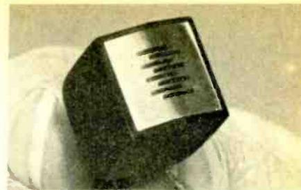
DHM/030, has a track width of 0.5mm and track spacing of 0.81mm. Inductance at 1kHz is 30mH ±20%. Playback full level is 85μV ±1.5dB. Crosstalk from a tape recorded to saturation level on seven tracks, measured on the unrecorded track, is better than -20dB. Signal current is 300μA r.m.s. and peak bias 1.7mA at 50kHz. Phi Magnetronics (Sales) Ltd, Penwerris Lane, Falmouth, Cornwall.
