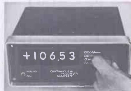
Weston standard cell. Zero offset current and voltage are automatically corrected between each reading. Series-mode rejection at mains supply frequency and its harmonics is greater than 85dB, and common-mode rejection 100dB at mains frequency and d.c. with  $1k\Omega$  imbalance in the input leads. The price is £25. International Electronics Ltd, Ewood Bridge, Haslingden, Lancs.
