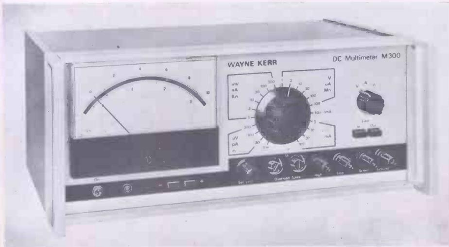
Wayne Kerr stand during the I.E.A. exhibition earlier this year, also measures direct voltage and resistance. Amplifier uses photochopper stabilization with 40-Hz switching to avoid beats with the 50-Hz supply. Instrument also features a small reverse scale for null detection, overload protection, one set-zero control for all ranges, a recorder output of 0.1mA at 1k $\Omega$ , and a hum rejection filter which rejects hum equivalent to 50  $\times$  f.s.d.
