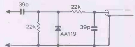
Fig. 2. Circuit for connection between earth and the last sound i.f. collector to view the overall response apart from the discriminator.
