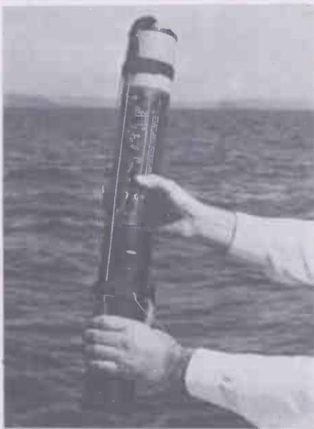
*This floating beacon manufactured by Burndept, which has already captured orders worth £50,000 from Norway, operates on a primary battery and transmits on both the civil and military aviation distress frequencies (121.5 and 243MHz) for a minimum of 48hrs at 0°C. It measures 670 x 85mm and weighs 2.89kg.*
