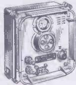
Small portable crystal controlled wavemeter. Size 7in. x 7in. x 4in. Frequency range 500 Kcs-10 Mc/s (up to 30 Mc/s on harmonics). Calibrated dial. Power requirements 300 V.D.C. 10mA and 12 V.D.C. 0.3A. Excellent condition. 89/8. Carr. 7/8.
