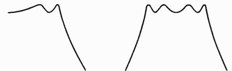
Fig. 7. The band-pass response has twice as many ripples as the low-pass response used as model.
