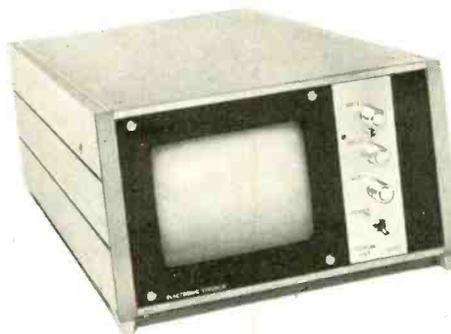
a simple blanking amplifier or an optional wideband linear amplifier. The vertical amplifier has a bandwidth of d.c. to 10MHz and all inputs are compatible with t.t.l. and d.t.l. levels. The unit can be supplied in various case types and is suitable for 19in rack-mounting. Electronic Visuals Ltd, P.O. Box 16, Staines, Middx.
