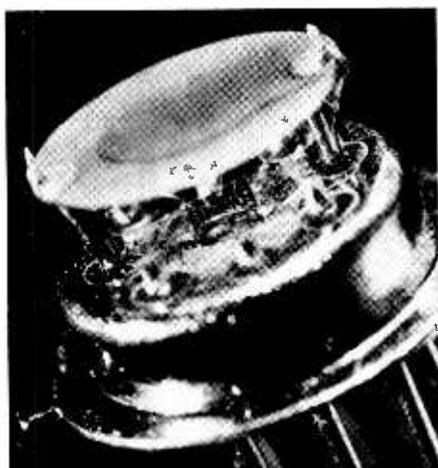
Quartz crystal and integrated circuit comprise new Marconi oscillator housed in a TO-5 package (type F3187).
