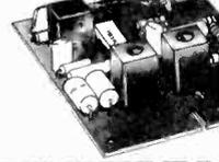
Two transistor plus integrated circuit design. 9-12 volt operated, 50mV sensitivity, lamp output direct. Auto switching plus many other features. Size 2 1/2" x 2 3/8" x 3/8" Standard 0-1 connector or solder connections. Output 1 volt per channel. Price ready to use £6.50 (Leaflet No. 7 on request).
