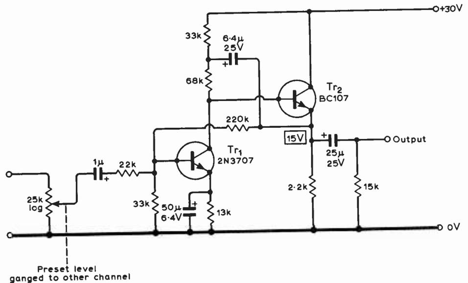
Fig. 15. Single-ended line amplifier. Distortion 0.1% at  $2\text{V}$  r.m.s. into  $600\Omega$ ; 0.05% at  $5\text{V}$  into high impedance. Residual noise  $-82\text{dB}$  w.r.t.  $500\text{mV}$  output ( $20\text{kHz}$  bandwidth).
