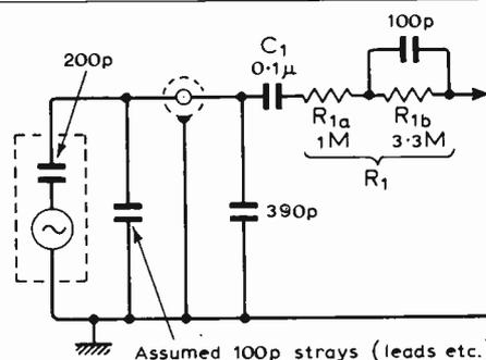
As an example of the suggested modifications the pickup input circuit for each channel of a Connoisseur SCU1 will be as shown here.
