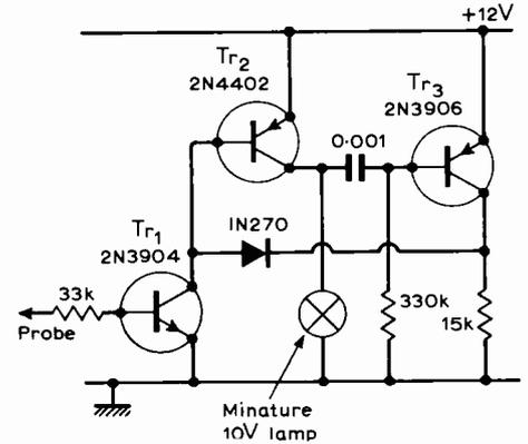
( $Tr_2$  and  $Tr_3$ ) lighting the lamp momentarily. Steady inputs above 0.7V hold the lamp on. The circuit can be housed in 3/8in diameter plastic tube with a probe attached.
