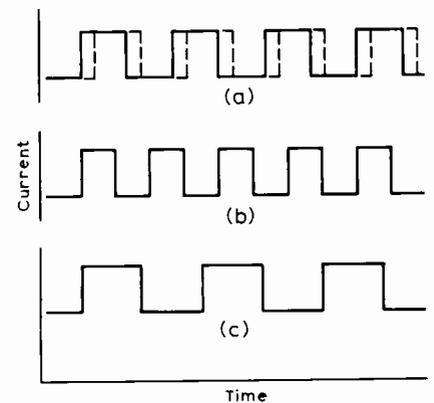
Fig. 2 Square-wave oscillations illustrating (a) phase difference, and frequency difference between (a), (b) and (c).
