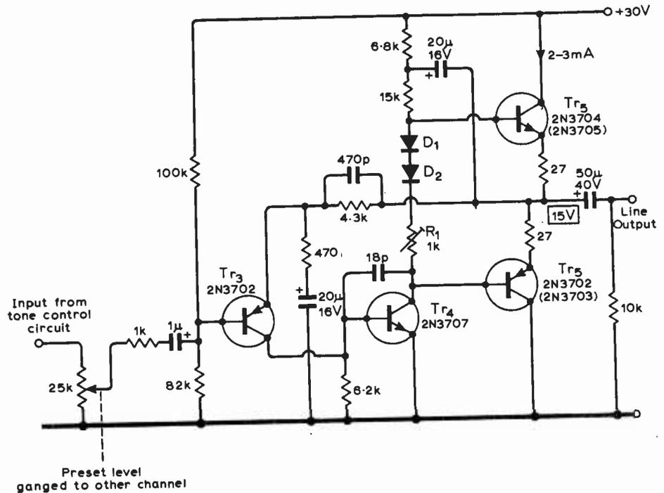
Fig. 16. Push-pull line amplifier. Distortion 0.03% at  $+20\text{dBm}$  ( $8\text{V}$  into  $600\Omega$ ) at  $1\text{kHz}$  and  $10\text{kHz}$ , and at lower powers ( $20\text{kHz}$  bandwidth).  $D_1$ ,  $D_2$  1N914.
