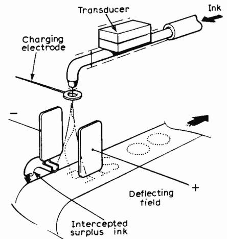
Fig. 4. To avoid using special paper a charged ink jet can be used, deflected electrostatically. Pulsed operation is achieved by attaching a transducer to the ink feed pipe.
