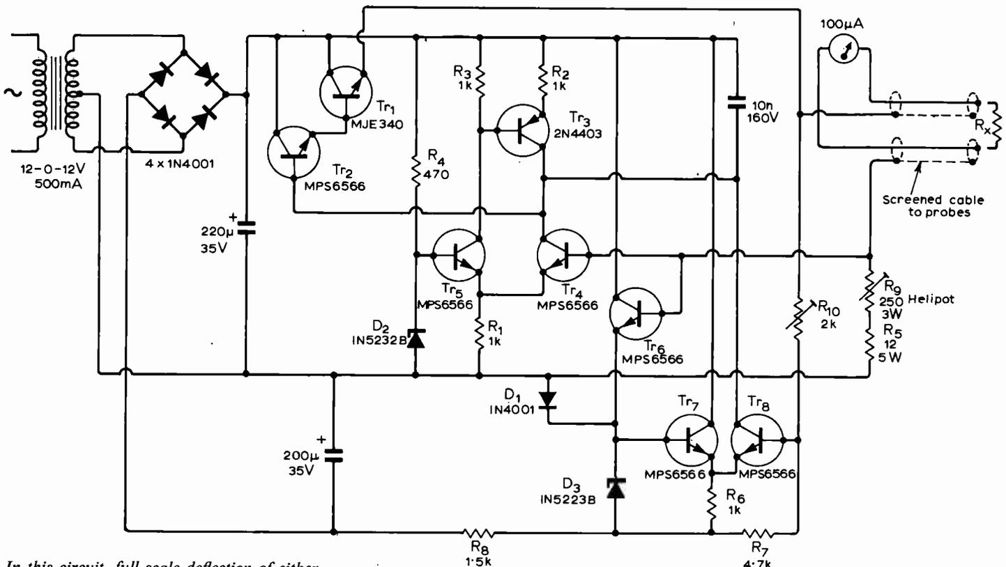
In this circuit, full scale deflection of either 500 milliohms or 5 ohms is set by  $R_9$ . Resistors should be  $\frac{1}{2}$ -watt types with  $\pm 5\%$  tolerance unless shown otherwise.
