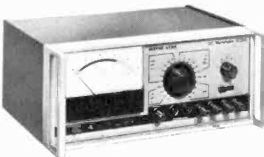
DC Multimeter – full-scale ranges  $30\mu\text{V}$ -300V, 30pA-100mA and  $10\Omega$ - $1\text{G}\Omega$ . Switched filter. Constant  $100\text{M}\Omega$  for 1% voltage measurements. Analog output. Ask for M300 Data Sheet.
