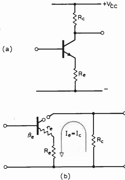
Fig. 9. Calculation of open-circuit voltage gain with addition of an external emitter resistor is easily done as  $R_e$  is merely added to  $r_e$ .
