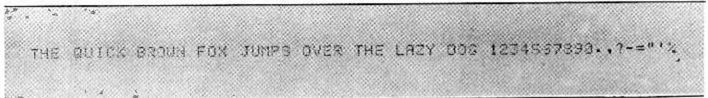
Fig. 3. To print electrostatically on continuously moving paper, the voltage to the printing heads is in the form of  $30\text{-}\mu\text{s}$  pulses. In this example the paper speed was  $125\text{cm/s}$  giving a printing rate of 500 characters a second.
