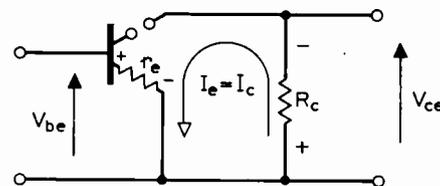
Fig. 8. Simpler circuit of common-emitter amplifier with d.c. source omitted and the approximation  $I_e = I_c$  made so that it can be immediately seen that  $\mu$  is the ratio of the two resistors, and that there is a change of polarity.
