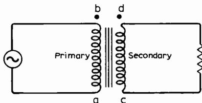
Fig. 1. An ideal transformer. Is the secondary voltage in phase with the primary voltage, or phase-reversed?
