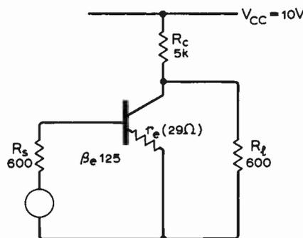
Fig. 10. Example used to illustrate calculation of voltage gain according to equation 1. This method of calculation shows that of the available gain of 173, 85.9% is transmitted by the input coupling and only 0.7% by the output coupling. It also shows that effect of using a transistor of four times the gain is an increase in voltage gain of only 12%.
