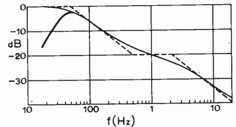
Fig. 2. Overall R.I.A.A. equalization with and without the rumble filter (either circuit).
