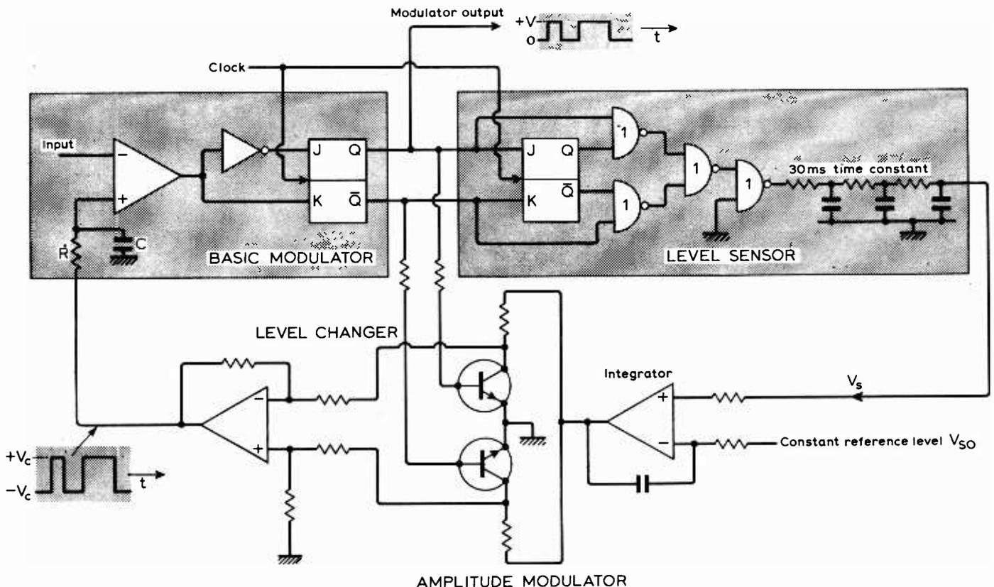
Fig. 5. Adaptive delta modulator using full width pulses.
