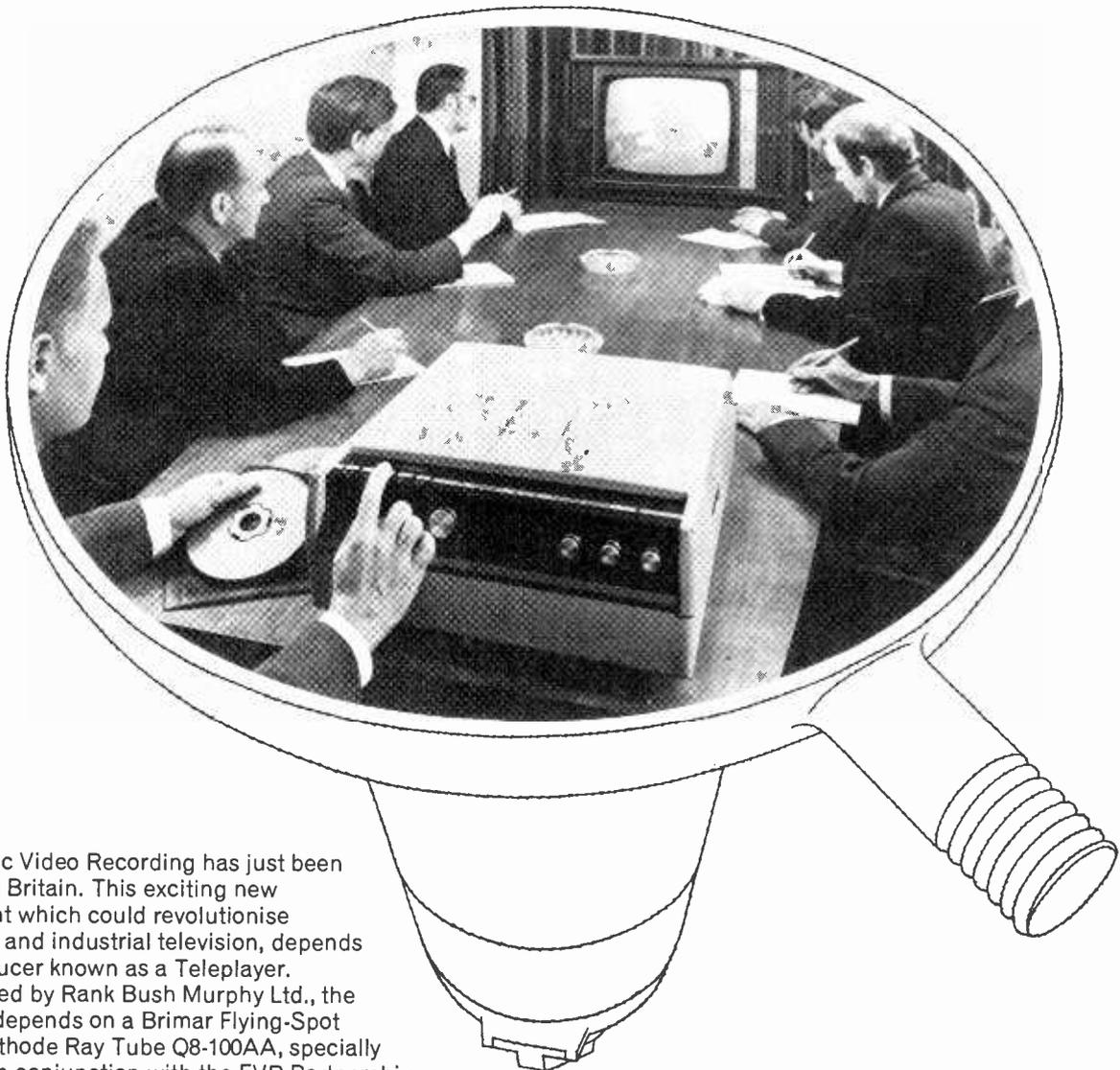
Electronic Video Recording has just been launched in Britain. This exciting new development which could revolutionise educational and industrial television, depends on a reproducer known as a Teleplayer. Manufactured by Rank Bush Murphy Ltd., the Teleplayer depends on a Brimar Flying-Spot Scanner Cathode Ray Tube Q8-100AA, specially developed in conjunction with the EVR Partnership.
