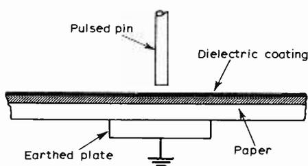
Fig. 1. Electrostatic printing can be achieved by applying an electric field across dielectric coated paper.
