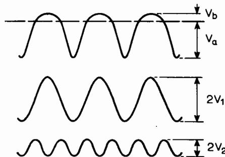
Fig. 6. Demonstrating the effect of negative feedback.
