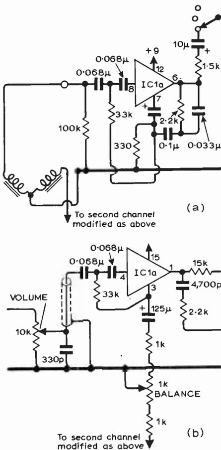
Fig. 1. Alternatives for incorporating the filter network: (a) in gram' input and (b) in second stage where it is effective on all inputs and reduces the 1/f noise of the first stage. The 0.068µF capacitors are 10% polyester and each should be matched with its corresponding number in the other channel. The 33kΩ resistor should be 5%, or better, 0.25W high stability carbon film or metal oxide.
