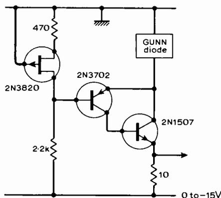
Fig. 4. The constant voltage bias circuit used so that the current could be monitored.
