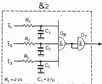
Fig. 3. It may be necessary to connect the sum output gate like this.
