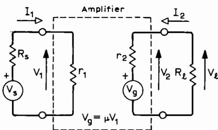
Fig. 2. Equivalent circuit of a source-amplifier-load enables overall gain to be expressed as a product of input coupling gain (from Fig. 1), internal amplifier gain  $\mu$  and output coupling gain.
