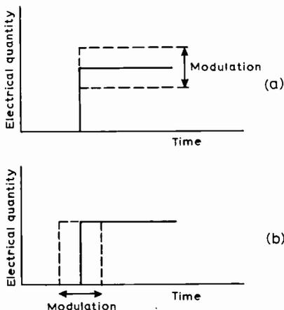
Fig. 1 How a periodic change can be used to carry information: (a) by modulation of amplitude; (b) by modulation in time.
