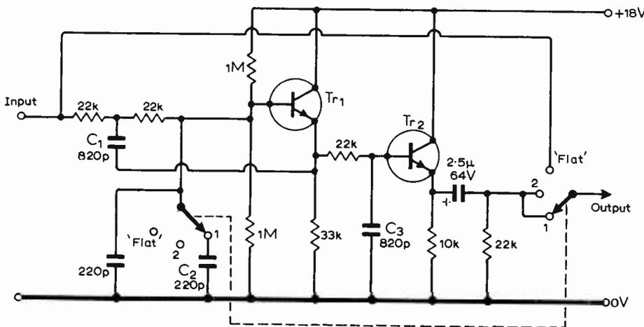
Fig. 13. High-frequency filter.  $Tr_1$ ,  $Tr_2$  BC109 etc.
