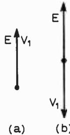
Fig. 5. Voltage phasor diagram (a) is sometimes seen for Fig. 4, but (b) is much commoner.
