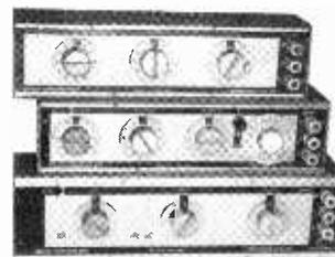
VARIABLE LOW PASS ACTIVE FILTERS over the range of :1 Hz to 11 kHz
