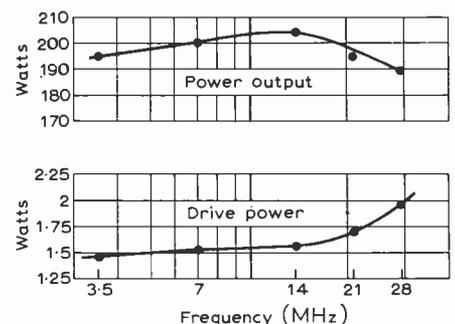
Fig. 3. Performance in terms of output and input power against frequency.
