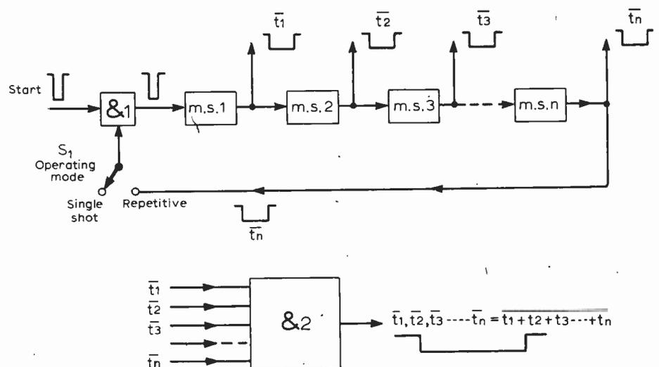
Fig. 1. Block diagram. With  $S_1$  in the repetitive position the cascade is self sustaining.
