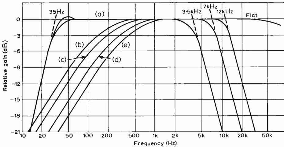
Fig. 1 Performance of unmodified pre-amplifier with three different ceramic cartridges. (a) pre-amplifier alone; (b) Sonotone 9TAHC; (c) Decca Deram; (d) Connoisseur SCU1 plus 100pF strays; and (e) Connoisseur SCU1, no strays.
