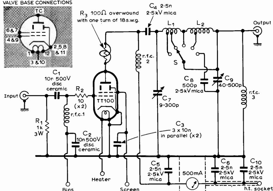
Fig. 1. Circuit of the linear amplifier capable of producing 200W up to 30 MHz.
