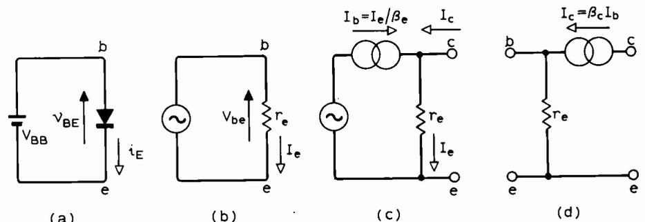
Fig. 5. Partial transistor model (a) can use  $r_e$  in place of base-emitter diode for small signals (b). Adding current generator with  $I_e$  as control variable (c) is invalid because it prevents input voltage appearing across  $r_e$  and allows  $V_{ce}$  to appear across  $r_e$ . It is avoided by making  $I_b$  the control variable (d).
