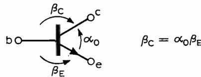
Fig. 4. Summary of transistor parameters are contained in the symbol. Numerical values are added in some positions in following circuit diagrams.
