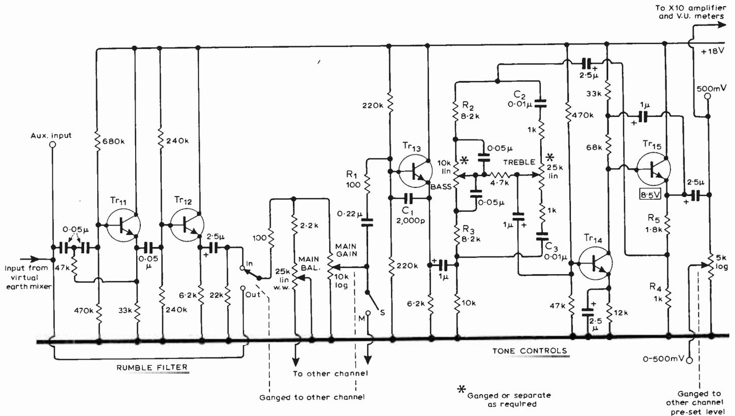
Fig. 11. Tone-control and filter circuit. Residual noise -98dB. Tr<sub>11</sub>-Tr<sub>15</sub> BC109 etc.
