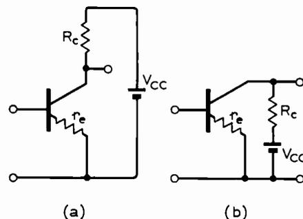
Fig. 7. Common-emitter amplifier circuit used to calculate open-circuit voltage gain  $\mu$  ( $\approx R_c/r_e$ ).
