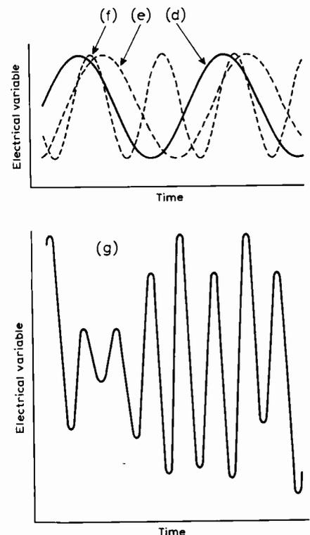
Fig. 3 Sine-wave oscillations differing in phase, (d) and (e), and in frequency, (d) and (f); also a sine-wave oscillation modulated in amplitude (g).
