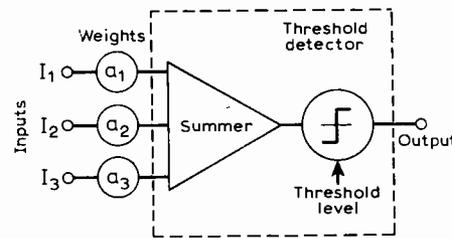
Fig. 2. Threshold gate.
