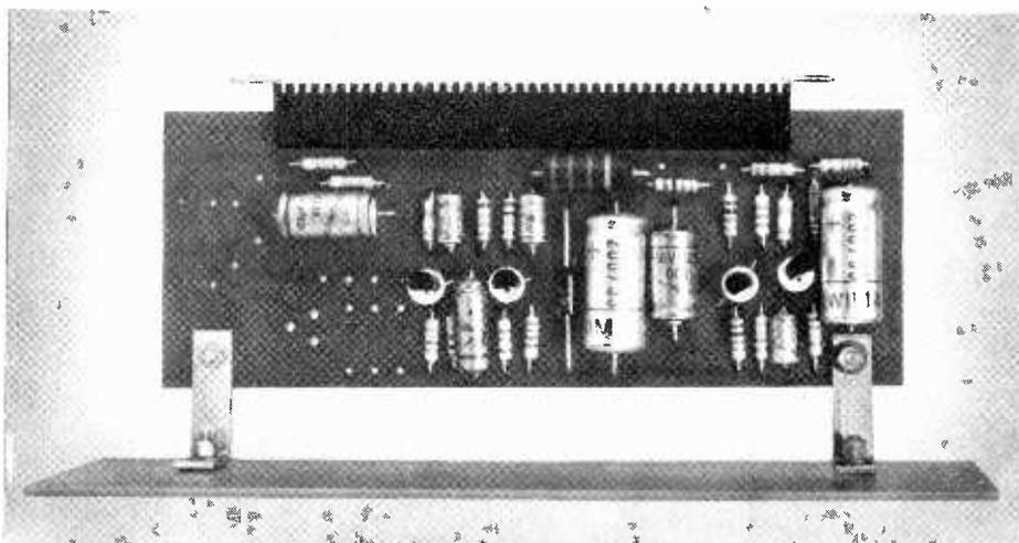
and with a control range of  $\pm 12\text{dB}$ . The filters can be used for either cut or lift in response depending on which way each filter 'card' is plugged in. The module is also useful in music reproduction systems where acoustic properties of the environment alter tonal balance. Astronic Ltd, Dalston Gardens, Stanmore, Middx HA7 1BL.
