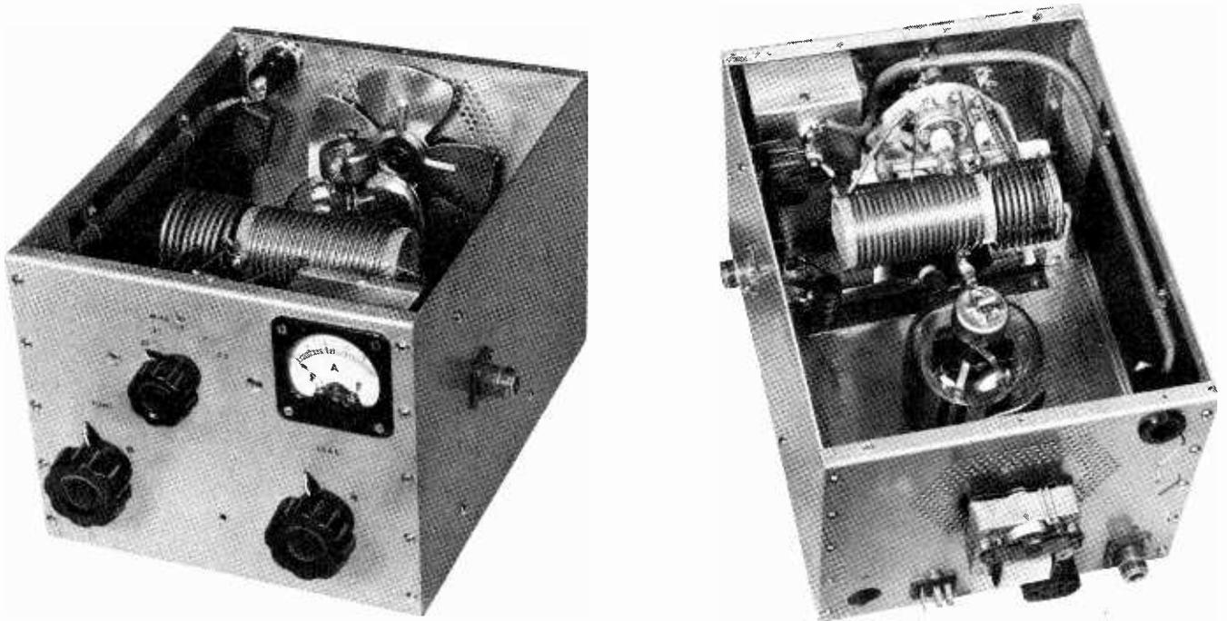
Two views of the completed prototype. In the left-hand photograph the h.t. decoupling capacitor can be seen in the top left-hand corner
