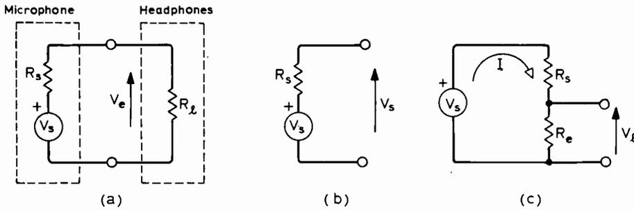
Fig. 1. To introduce transistor amplifier theory an understanding of voltage transfer is necessary—often misunderstood. Simplest way to find signal transfer from source to load (a) under no-load conditions (b), is to treat the two resistances as a potential divider (c).
