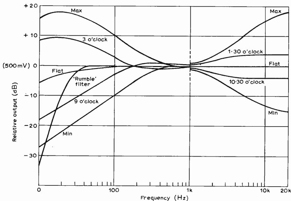
Fig. 12. Characteristics of filter and tone controls.
