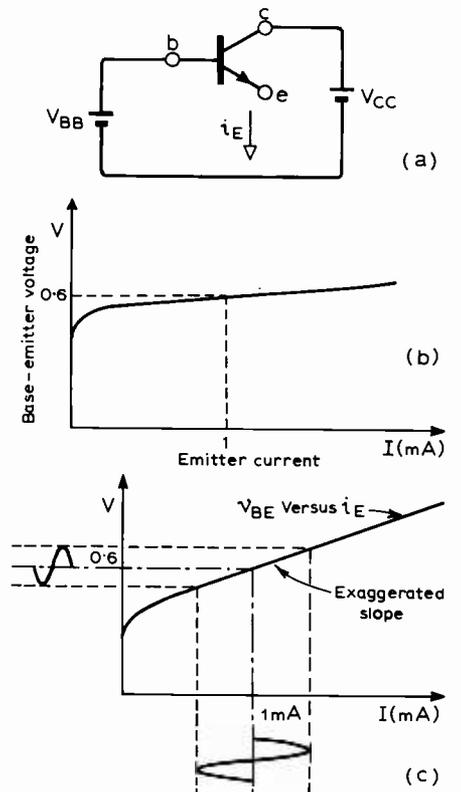
Fig. 3. To help find  $r_1$ ,  $r_2$ , and  $\mu$  in Fig. 2 and in equation 1, a model is needed in terms of simple components. To provide this the bipolar transistor (a) must be understood, in particular the  $i_E$ - $v_{BE}$  relationship (b) whose slope is the important thing (c), and which is approximately constant if  $v_{CE}$  is greater than 1 V.
