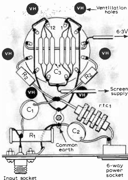
Fig. 2. Under-chassis layout of components.
