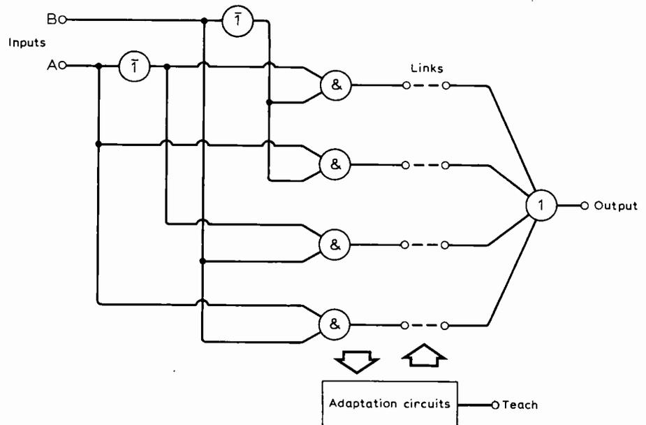
Fig. 4. Universal gate with adaptation circuits.
