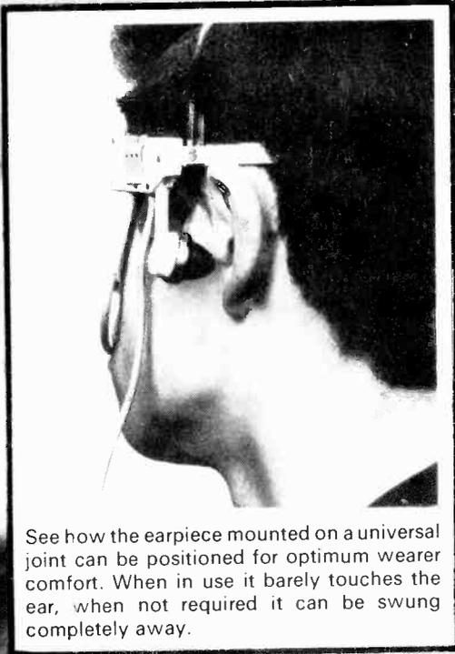
See how the earpiece mounted on a universal joint can be positioned for optimum wearer comfort. When in use it barely touches the ear, when not required it can be swung completely away.
