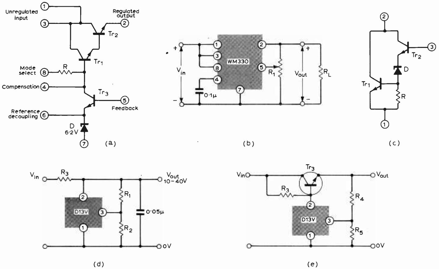
Fig. 2. Simple voltage regulator microcircuits. (a) Westinghouse WM330; (b) connection of WM330 in practical circuit; (c) G.E. (U.S.A.) D13V utility voltage regulator; (d) the D13V as a shunt regulator; (e) the D13V as a series regulator.
