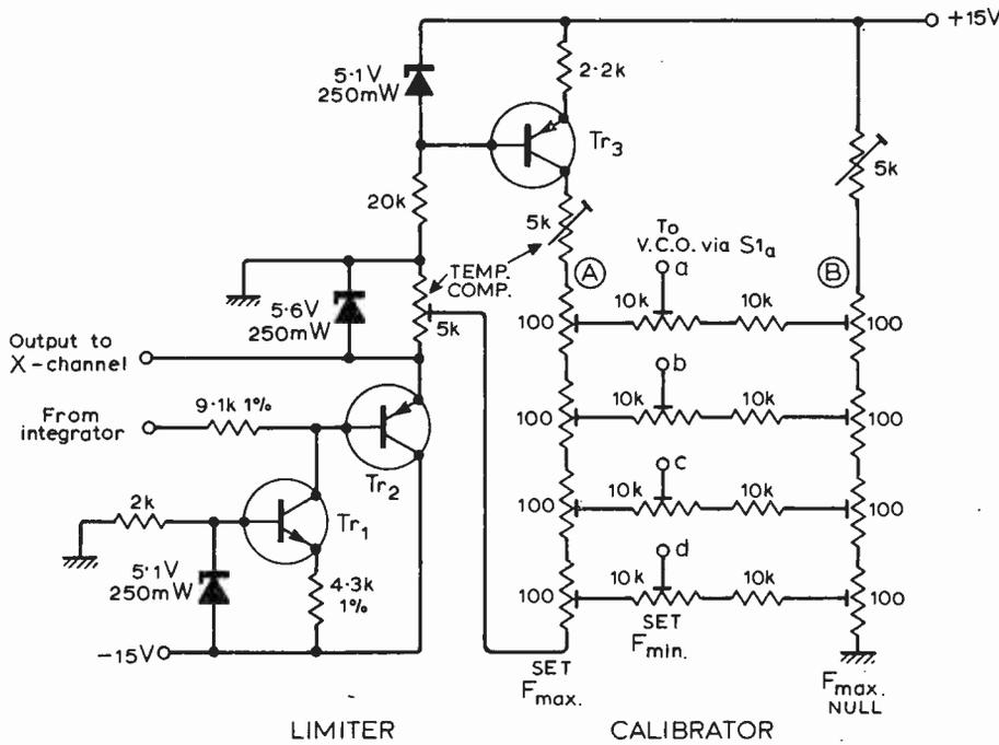
Fig. 3. Limiter and range calibrator includes three pre-set potentiometers for each range to set maximum and minimum frequencies. Null potentiometers allow minimum frequencies to be adjusted without affecting maximum frequency. (Potentiometers can be skeleton pre-set or, for greater precision, multi-turn pre-set types.)
