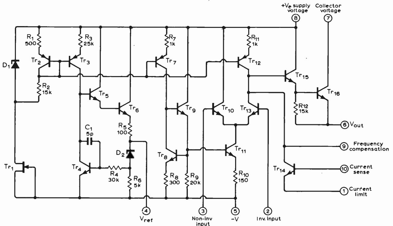
Fig. 3. Internal circuitry of industry-standard Fairchild Semiconductors  $\mu$ A723 voltage regulator microcircuit.
