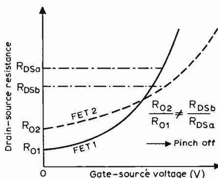
Fig. 1. Automatic gain control offsets 'dynamic mismatch' which occurs when f.e.ts are used in a Wien network. This 'mismatch' is caused by the ratio of the drain-source resistances varying with gate-source voltage as shown.
