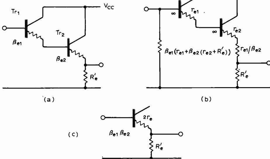
Fig. 18. Because both a.c. and d.c. quantities can be mixed in the same equation with the beta-barrier model it is easy to show that the Darlington pair (a) has a current gain equal to the product of individual gains and an emitter resistance of twice the usual value (c). Voltage gain is calculated by first transferring  $r_{e1}$  to  $Tr_2$  emitter and then transferring all resistances to the base of  $Tr_1$  (b) and using the relation  $I_{E1} = I_{E2}/\beta_{E2}$ .
