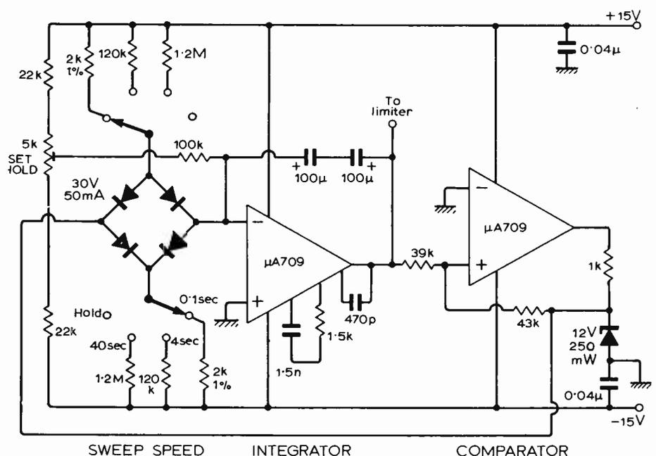
Fig. 2. Ramp generator uses Miller integrator switched at selected rates by a comparator in the feedback loop. (Resistors in all circuits should be  $\frac{1}{4}$ -watt,  $\pm 5\%$  tolerance unless shown otherwise. Compensation capacitors should be polystyrene dielectric.)
