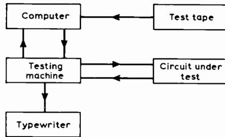
Fig. 3. Automatic test system.
