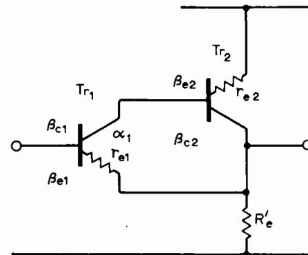
Fig. 19. Analysis of the complementary pair shows equivalence to a single transistor of current gain  $\alpha_{o1}\beta_{e1}\beta_{e2}$  with emitter resistance  $r_{e2}$ .
