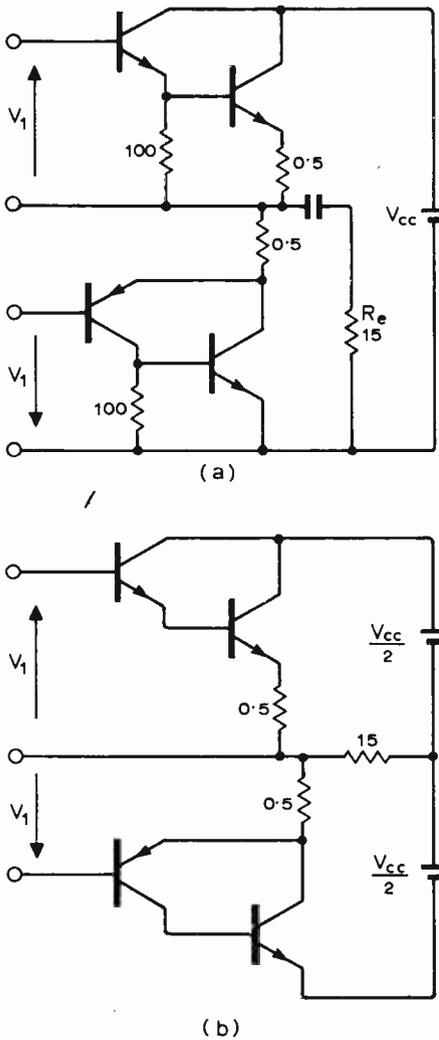
Fig. 21. For d.c. and large-signal analysis emitter resistors must be replaced by diodes. This Lin circuit (a) consisting of a Darlington pair and a complementary pair is equivalent to circuit (b) and is separated for analysis into Figs 22 and 23.
