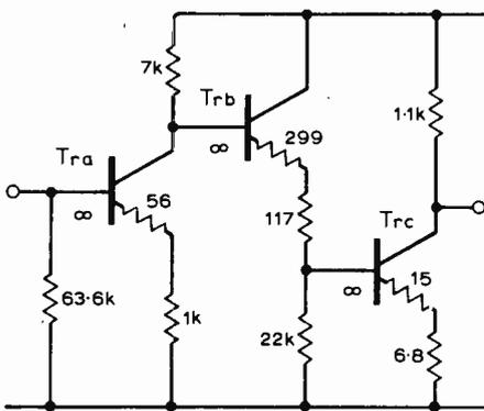
Fig. 14. Open-circuit gain of Fig. 12 circuit can be calculated more quickly using referred resistance technique of Fig. 13. Emitter resistance of  $Tr_a$  is transferred to base;  $Tr_b$  and  $Tr_c$  base resistances are transferred to their emitters; collector resistance of  $Tr_a$  is transferred first to  $Tr_b$  emitter by dividing by  $\beta_{cb}$  and then—with emitter resistance of  $Tr_b$ —to  $Tr_c$  emitter by dividing by  $\beta_{ec}$ .
