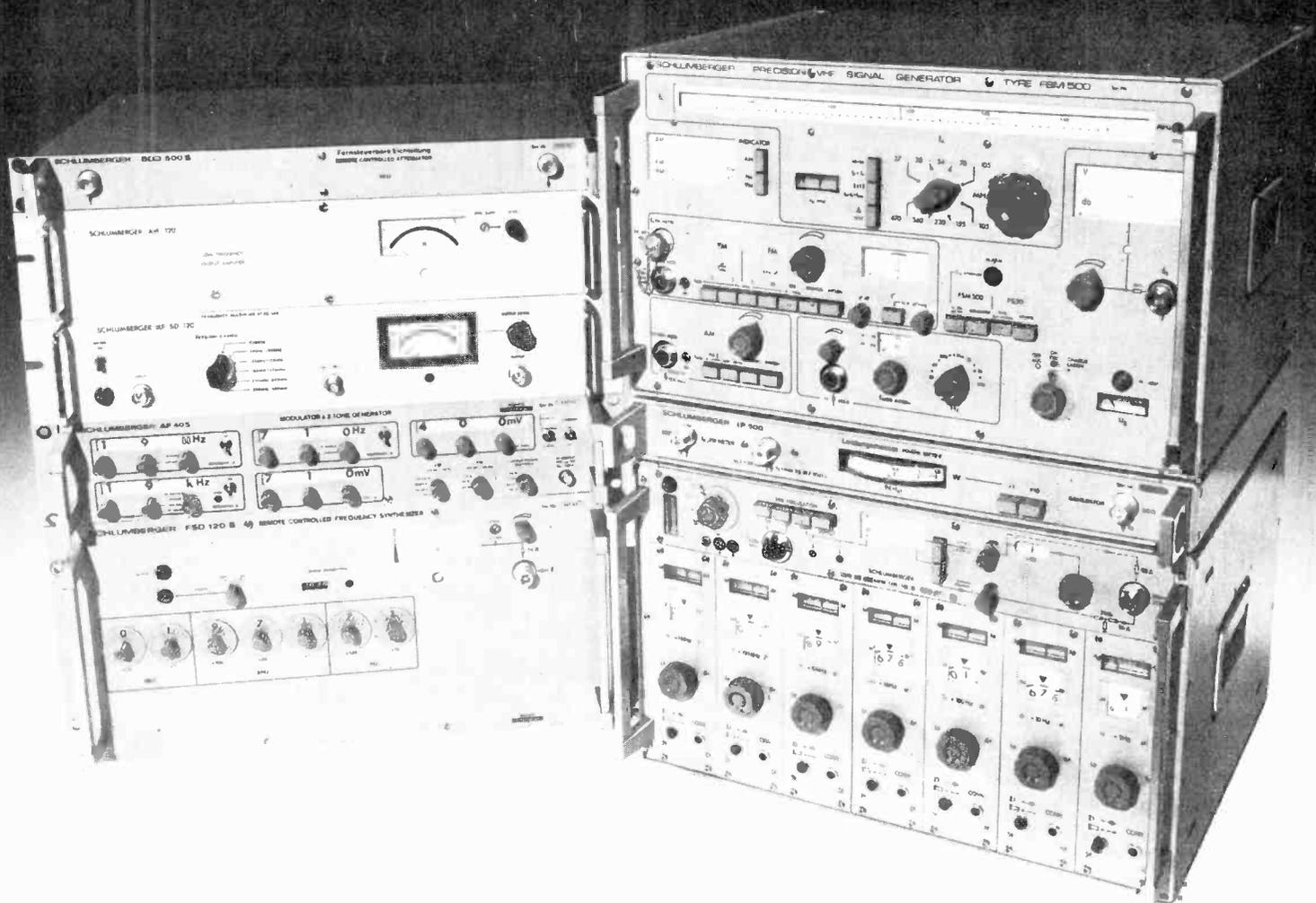
Solartron's synthesizer signal generator eliminates those three operator headaches: keeping the signal generator within the bandwidth of the RX that's being checked; having to reset output levels with each modulation change; and having to readjust controls with every frequency change.
