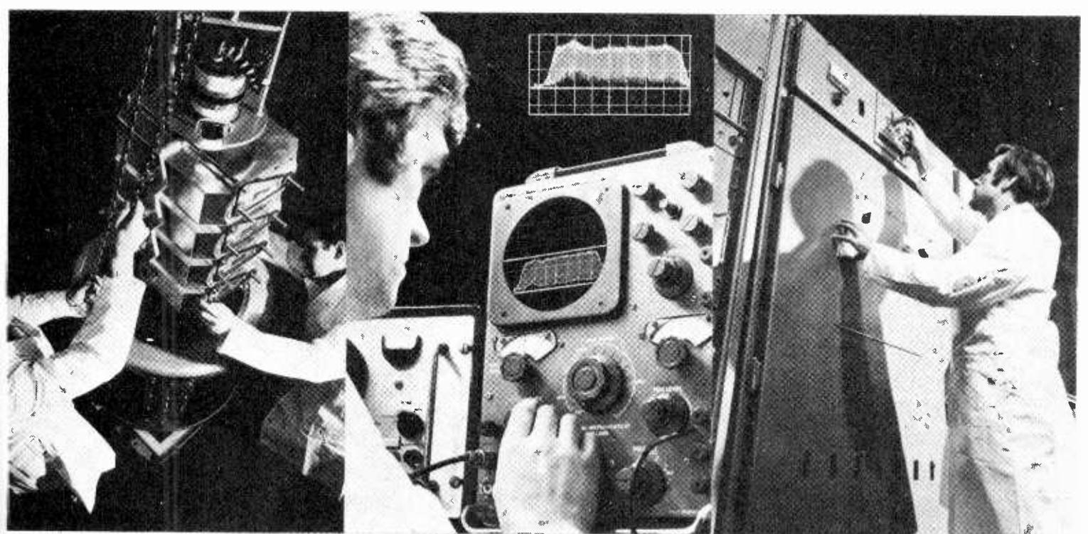
is also easy to lower the klystron to the circuit assembly because there are guide rails on the internal structure of the magnetic frame. The assembly is then pushed back to the transmitter.
