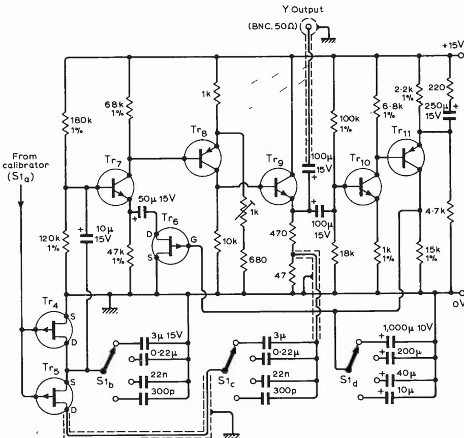
Fig. 4. Voltage-controlled oscillator with f.e.t.s as resistors in Wien network uses another f.e.t. for a.g.c. Allow circuit to settle for one minute before starting sweep. (Non-polarized capacitors in the range switching should have polyester or polystyrene dielectrics.)
