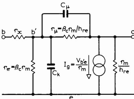
Fig. 15. To find how the beta-barrier model compares to this hybrid- $\pi$  circuit it is transformed to the circuit of Fig. 16.
