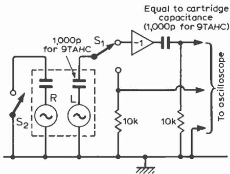
Fig. 5. Test circuit for high/low impedance loads.
