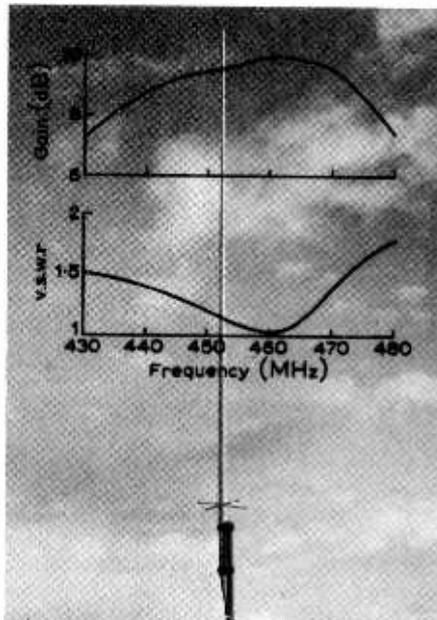
giving a frequency range of 450-470 MHz with a maximum v.s.w.r. of 1.5. Impedance is 50ohms and half-power beam-width  $8^\circ$ .
