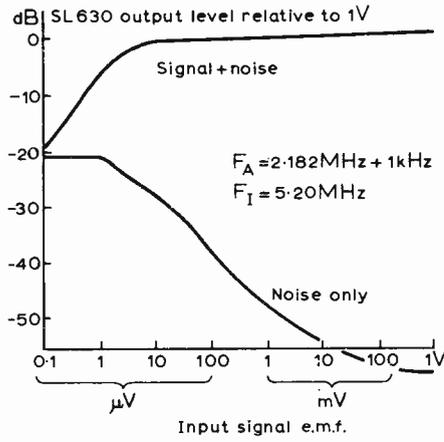
Fig. 7. Signal-to-noise and a.g.c. performance of circuit of Fig. 4.
