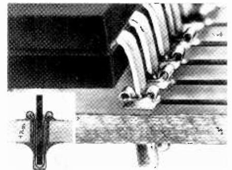
claimed) more reliable connection than presently available circular cups. A spring, soldered to the board, allows round leads from 0.014 to 0.022in diameter and flat leads 0.008 to 0.01in thick by 0.025in wide to be accepted. The sockets, called Minisert, are available separately or in strip form for use with an inserter machine. Berg Electronics Inc, New Cumberland, Pennsylvania 17070.
