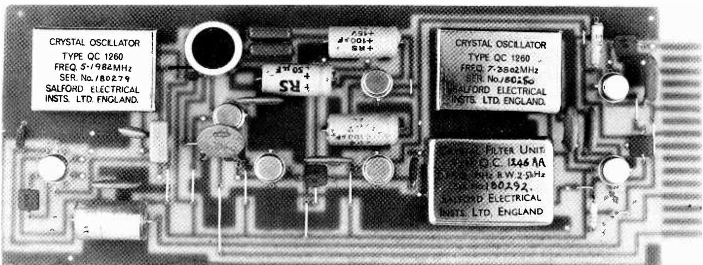
Fig. 6. A printed circuit board construction.
