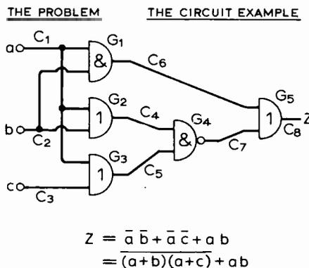
Fig. 4. The circuit used to illustrate the various techniques of diagnosis.
