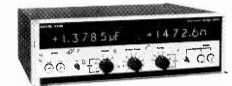
has twin displays reading up to 19999. Either or both displays can be used as a four-range d.v.m. In addition a reciprocal capacitance facility provides a linear distance/readout relationship for checking capacitive transducers. Wayne Kerr Co., Roebuck Rd, Chessington, Surrey.
