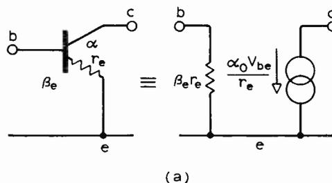
given by adding the feedback and output resistances of Fig. 16 to the beta-barrier model as in Fig. 17(b). This is now as accurate as the hybrid- $\pi$  circuit for low-frequency work.
