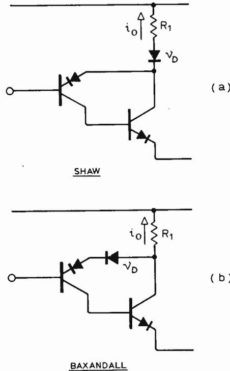
Fig. 24. Modification of complementary pair due to I. M. Shaw (a) and to P. J. Baxandall (b). Text shows how balance is improved.
