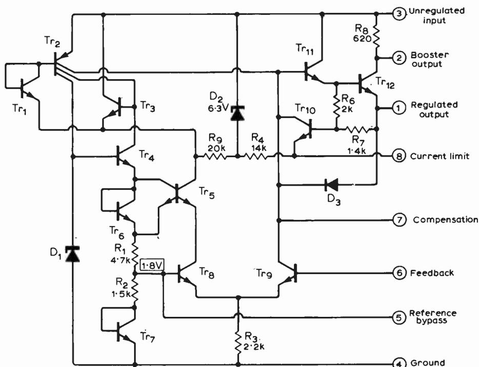
Fig. 6. Internal circuitry of industry-standard National Semiconductors LM100 voltage regulator microcircuit.
