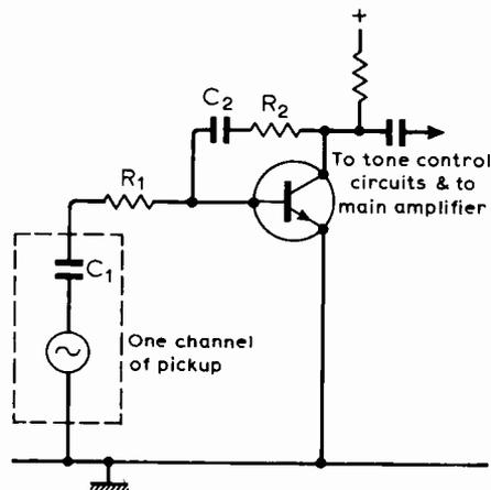
Fig. 7. Basic circuit for equalizing any ceramic pickup.
