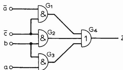
Fig. 1. Fault masking through redundancy.
