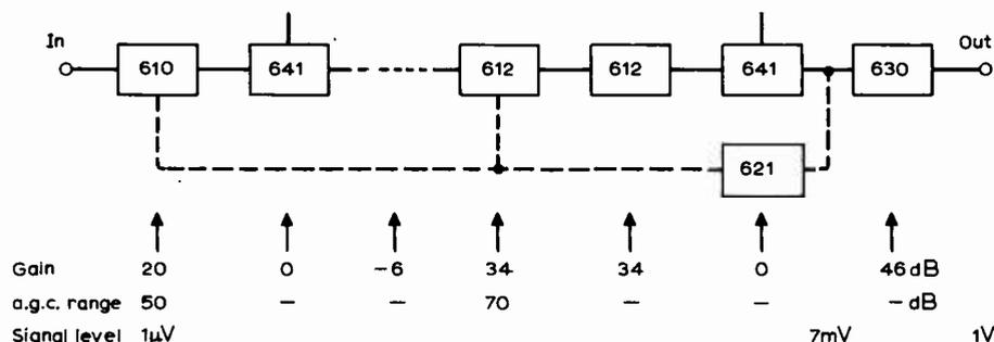
Fig. 4. Device and gain structure of receiver module.
