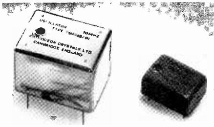
loop. The oscillators are based on the FS5901 and FS5951, the latter having compensation for temperature effects and allowing for frequency stability of  $\pm 0.1$  p.p.m. between  $0^\circ$  and  $60^\circ\text{C}$ . Linearity for both packages is better than  $\pm 5\%$  on the control range 0.5V to 5.0V, and the output is a 0-2.8V minimum square wave. Cathodeon Crystals Ltd., Linton, Cambridge.
