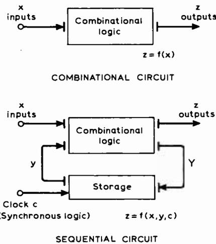
Fig. 2. Models for combinational and sequential circuits.
