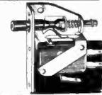
**"HONEYWELL" V3 SERIES.**—Flush micro-switch 10 amp. c/o. The side panel is insulated. End-plate size: 2" x  $\frac{3}{4}$ ". £1.50 per dozen.
