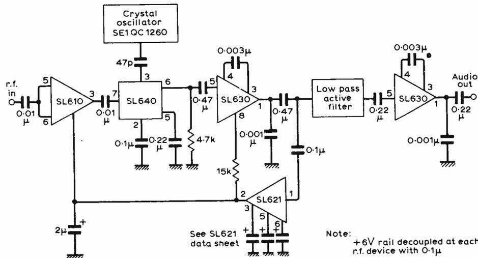
Fig. 9. Circuit diagram for direct conversion s.s.b. receiver.
