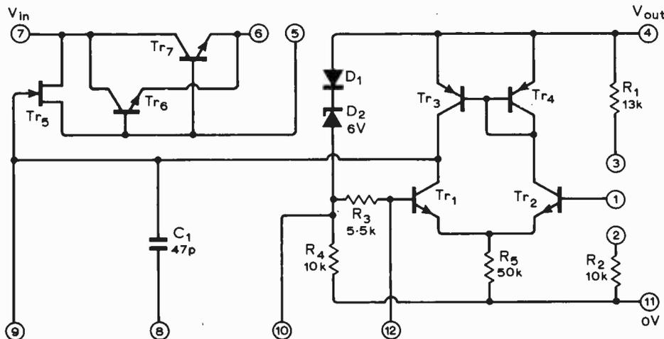
Fig. 8. Circuit of hybrid voltage regulator, General Instruments NC562.
