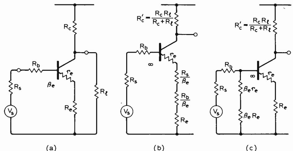
Fig. 13. In calculating the overall gain of the common-emitter circuit (a), resistances in the base circuit can be referred to the emitter circuit by dividing by  $\beta_e$  (b), or resistances in the emitter circuit can be referred to the base by multiplying by  $\beta_e$  (c).
