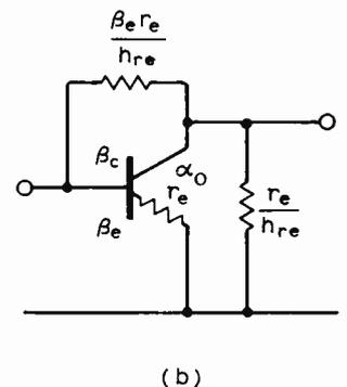
Fig. 17. Circuit of Fig. 16 is equivalent to the beta-barrier model by using only  $r_{be}$  and the current generator of Fig. 16 and replacing  $r_e'$  by  $r_e$  (a). A beta-barrier model (b) as accurate as the hybrid- $\pi$  circuits for low frequencies is thus derived by adding feedback and output resistances of Fig. 16 to (a).
