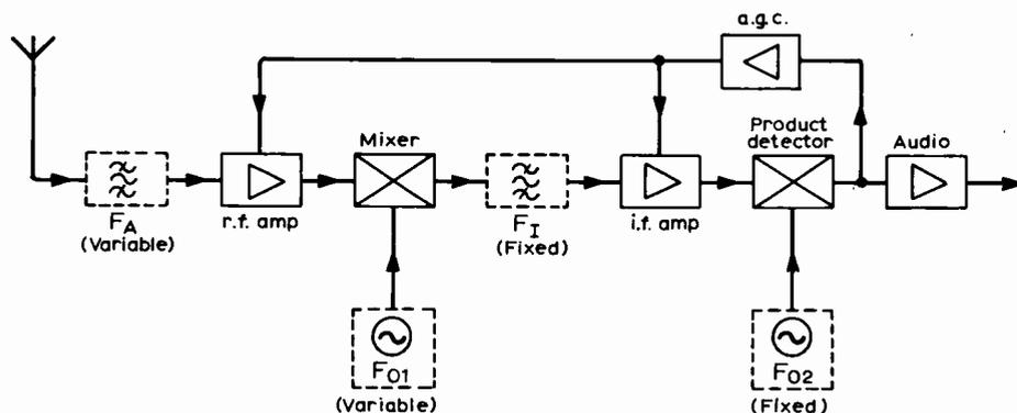
Fig. 2. Basic block structure of an s.s.b. receiver.
