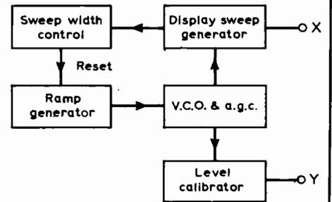
Although the unit described has proved very useful, its performance can be improved to allow accurate measurement of network response. Disadvantages are the calibration procedure (to compensate for f.e.t. spreads), the display sweep generator is not very linear with frequency, and the output level is not fully adjustable.
