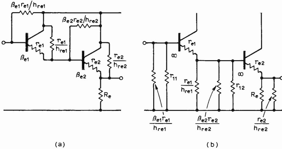
Fig. 20. To compare simple and more exact beta-barrier models for the Darlington pair, circuit is redrawn (a) using model of Fig. 17(b). Circuit (b) is equivalent to (a) with emitter resistances of each stage transferred to the base circuits as  $r_{11}$  and  $r_{12}$ . Two models give input resistances differing by a factor of five, but simple model gives more accurate result when  $Tr_1$  collector and  $Tr_2$  emitter are bootstrapped.
