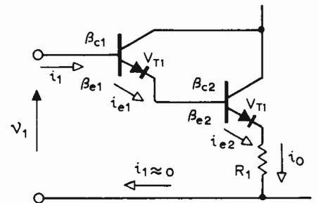
Fig. 22. Large-signal model of Darlington pair used to calculate expression for  $v_1/i_o$ . Comparing with expression for the complementary pair - derived from Fig. 23 - shows the two circuits are unbalanced.
