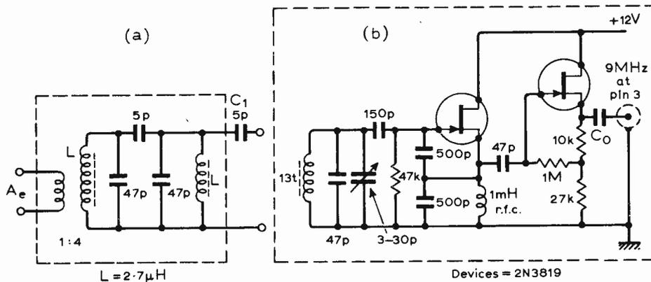
Fig. 8. Aerial pre-selection and local oscillator for 20-metre band.
