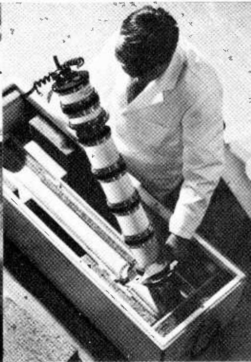
This 10 kW klystron can be easily removed from its pack. It's then ready to be dressed with the pre-tuned cavities which have been removed from the other klystron.
