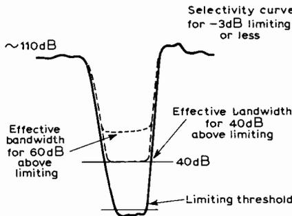
This results in an effectively wider bandwidth as shown in the graph, so that at the minimum signal strength at which stereo reception would give anything like an acceptable signal-to-noise ratio, the effective bandwidth is approximately 400 kHz, or more. It was partly for this reason that the limiting threshold of  $0.18\mu\text{V}$  was set so low.
