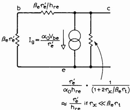
Fig. 16. Equivalent of hybrid- $\pi$  circuit of Fig. 15 where  $r_e'$  is  $r_e$  plus a measurable correction term.
