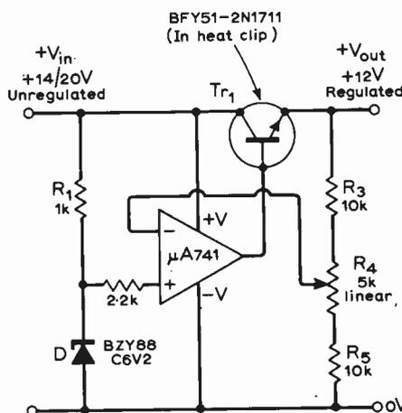
Fig. 1. Using a standard monolithic op-amp ( $\mu A741$ ) to make up a 12V, 100mA stabilized d.c. supply.
