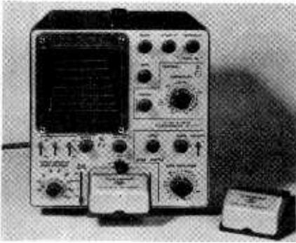
transistor and diode characteristics at currents of up to 2A, reverse currents down to 5nA and reverse voltages up to 1kV. Two different characteristics can be displayed on the  $10 \times 10$ cm screen. Price £195. Telequipment, 313 Chase Road, London, N14 6JJ.
