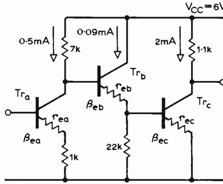
Fig. 12. Derivation of open-circuit voltage gain of ring-of-three amplifier used to illustrate emitter follower analysis. With no feedback and source and load unconnected gain is 328.
