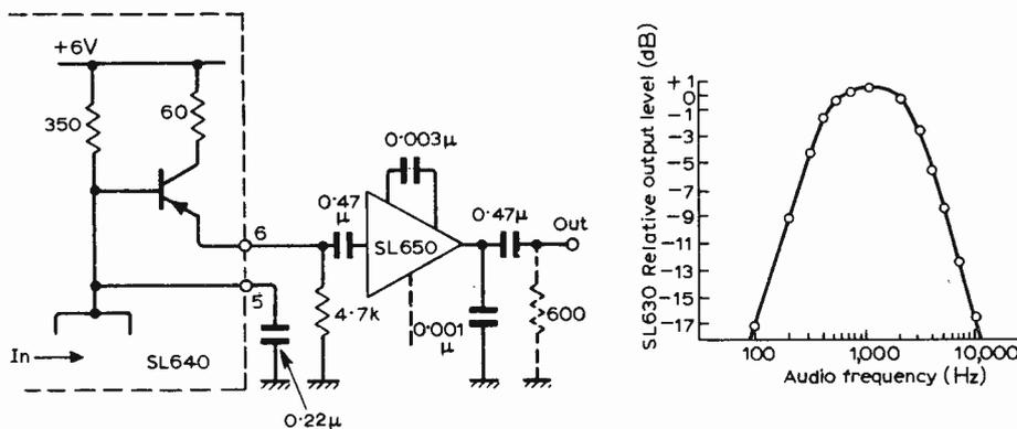
Fig. 10. Audio filtering within circuit of Fig. 9.
