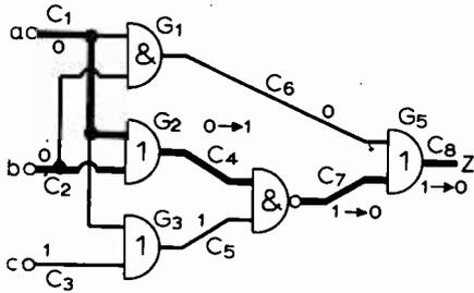
Fig. 7. The sensitive path and fully assigned circuit for  $C_4$  s-a-1.
