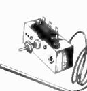
**"GOYEN" PRESSURE SWITCH.**—Incorporating differential adjustment between 2" and 12" water gauge (a max. of approx.  $\frac{1}{2}$  p.s.i.). A single pole change-over switch rated 15 amps. 250v. is actuated. Air inlet tube  $\frac{1}{8}$ " dia. Projection  $\frac{1}{4}$ ". Overall size: dia. 3 $\frac{1}{2}$ ", depth 2" plus  $\frac{1}{4}$ " (air tube). £1.25.
