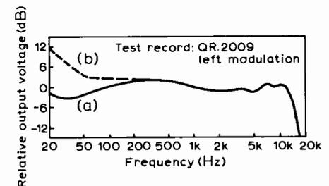
Fig. 2. Sonotone 9TAHC frequency response curve. (a) voltage across 2M $\Omega$  load shunted by 100pF. (b) internal pickup e.m.f. Curve (a) can be derived from (b) by calculating the bass cut due to the 2M $\Omega$  load—which gives 3dB down at 88Hz.
