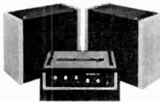
*Output Power:* 45 watts R.M.S. (Sine wave drive). *Frequency response:* -3 db points 30 Hz at 18 KHz. *Total distortion:* less than 2% at rated output. *Signal to noise ratio:* better than 60 db. *Speaker Impedance:* 3, 8 or 15 ohms. *Bass Control Range:* ±13 db at 60 Hz. *Treble Control Range:* ±12 db at 10 KHz. *Inputs:* 4 inputs at 5 mV into 470 K. Each pair of 2 inputs at 200 mV into 470K.
