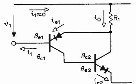
Fig. 23. Large-signal model of complementary pair.
