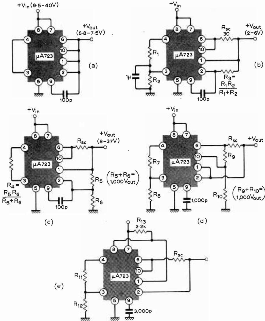
Fig. 4. Versatility of commercial voltage regulator microcircuits illustrated in typical circuit connection options for standard  $\mu A723$ . (a) Nominal 7.15V output with only one external capacitor; (b) low voltage (+2 to +6V) output; (c) high voltage (+8 to +37V) output; (d) foldback current limiting arrangement; (e) pre-regulated low voltage output.
