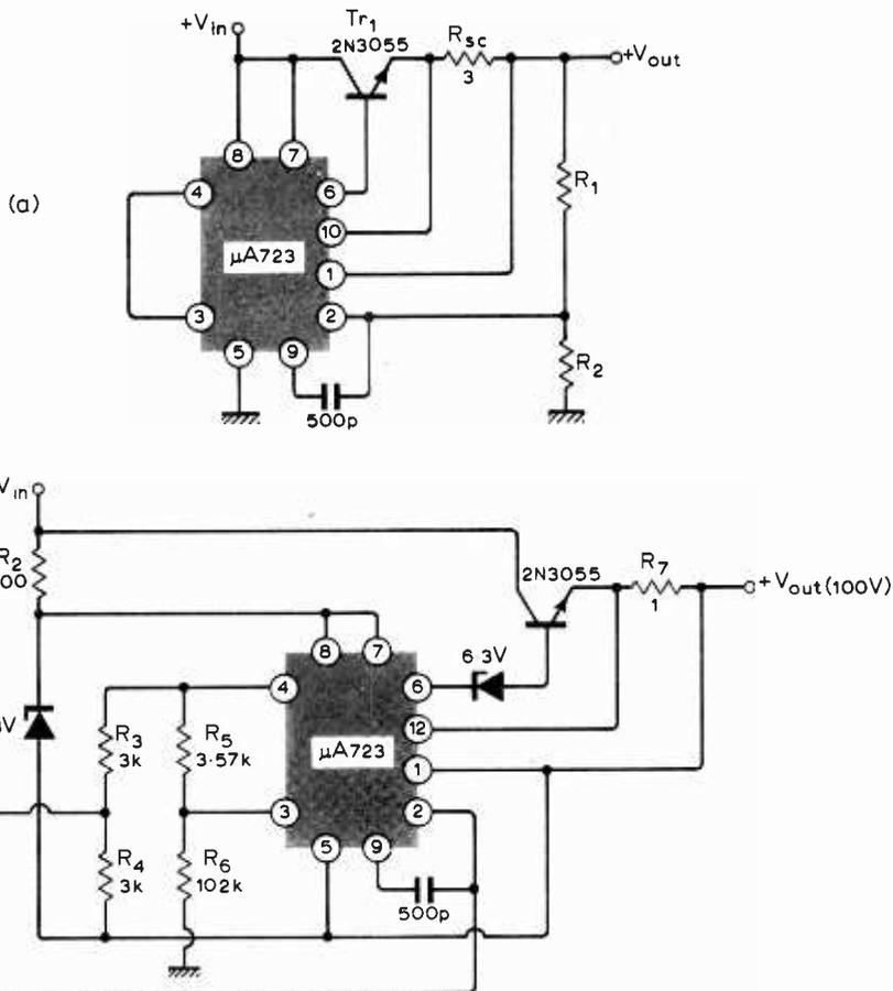
Fig. 5. Typical uses of external transistors to extend output capabilities of standard voltage regulator microcircuit (μA723). (a) high-current series-pass external transistor; (b) 'floating' high voltage (100V, 50A) output.
