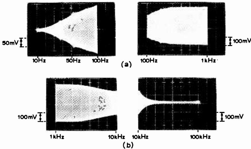
Application of sweep generator. Lower traces show envelope response of 2nd-order low-pass filter with 10kHz 'break' frequency. Generator set to 4s sweep time. Upper traces show envelope response of 2nd-order high-pass filter with 100Hz 'break' frequency. Generator is uncalibrated and set to 40 sweep time. Spikes at 50Hz are due to hum on the signal.
