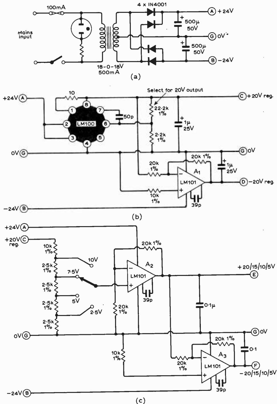
Fig. 7. Application of LM100 in regulated double (±) rail bench power supply for use with linear microcircuits: (a) rectifying-smoothing giving ±24V unregulated; (b) fixed ±20V regulated section; (c) switchable ±5, 10, 15, 20V section.
