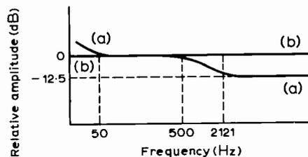
Fig. 1. Recording correction curves. (a) R.I.A.A. (b) constant amplitude.
