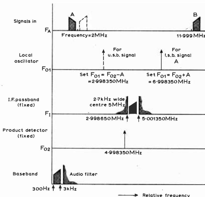
Fig. 1. Frequency chart for s.s.b. demodulation.
