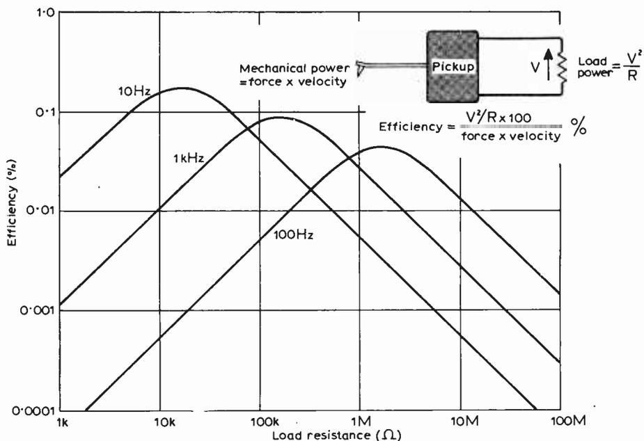
Fig. 4. Power conversion efficiency of a stereo ceramic pickup (9TAHC).
