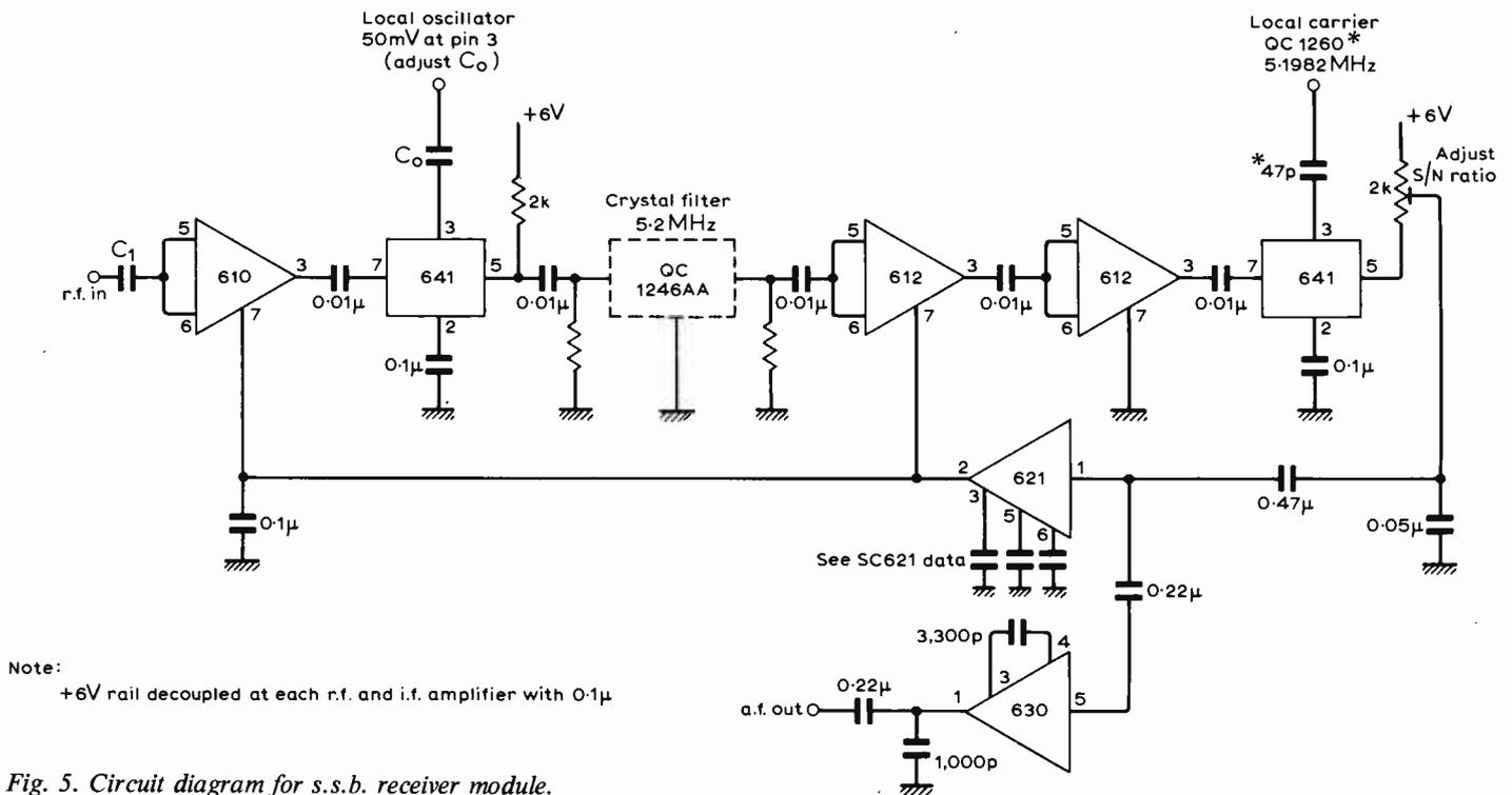
Fig. 5. Circuit diagram for s.s.b. receiver module.
